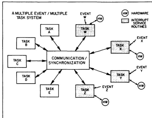
1. In a real-time multitasking system, task modules (A through F) can often perform their functions only after hardware-generated interrupts are serviced (highlighted). The executive in such a system provides intertask communications and synchronization.
