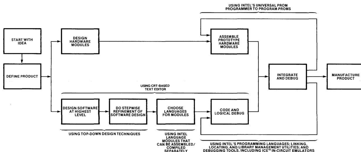
Figure 1-1. Microcomputer System Development Process
