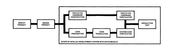
Figure 1-3. Typical Development Cycle with ICE<sup>™</sup> Module
