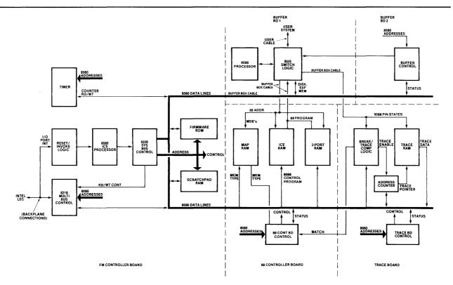
Figure 1-2. ICE-88<sup>™</sup> Functional Block Diagram
