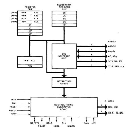
Figure 1-1. 8088 CPU Functional Block Diagram
