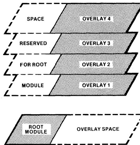
Figure 4-1. Memory Configuration of Program With Overlays
