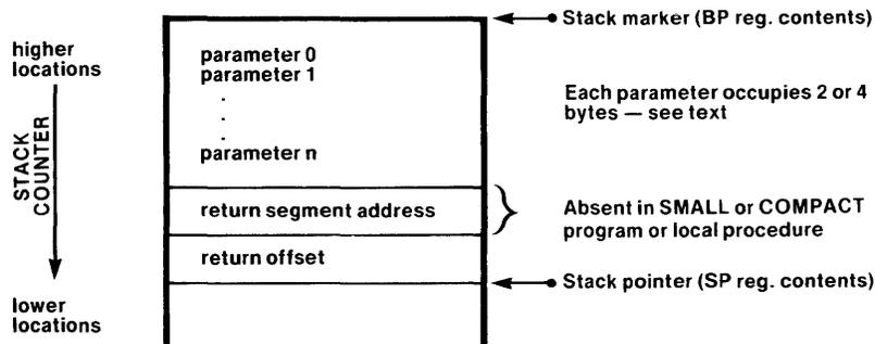
Figure H-1. Stack Layout at Point Where a Non-Interrupt Procedure is Activated
