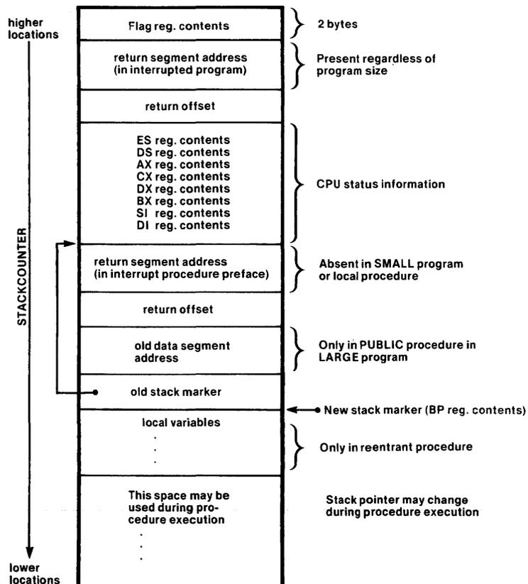
Figure I-3. Stack Layout During Execution of Interrupt Procedure Body
