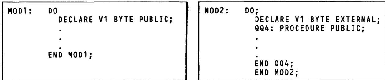
Both references to V1 will use the same definition (location) for V1, namely that in module MOD1. Similarly, if any module needed to call procedure QQ4, it would first need a declaration like
