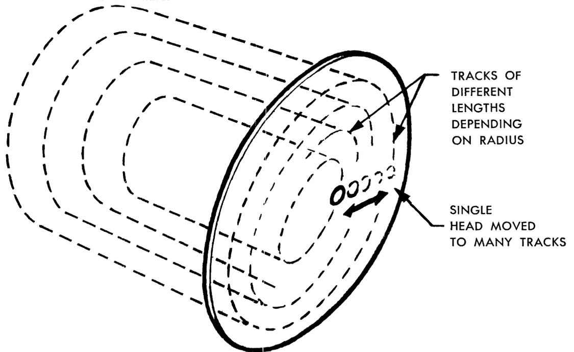
POSITIONING HEADS ON A DISC IS LIKE MOVING HEADS FROM ONE DRUM SIZE TO ANOTHER.
