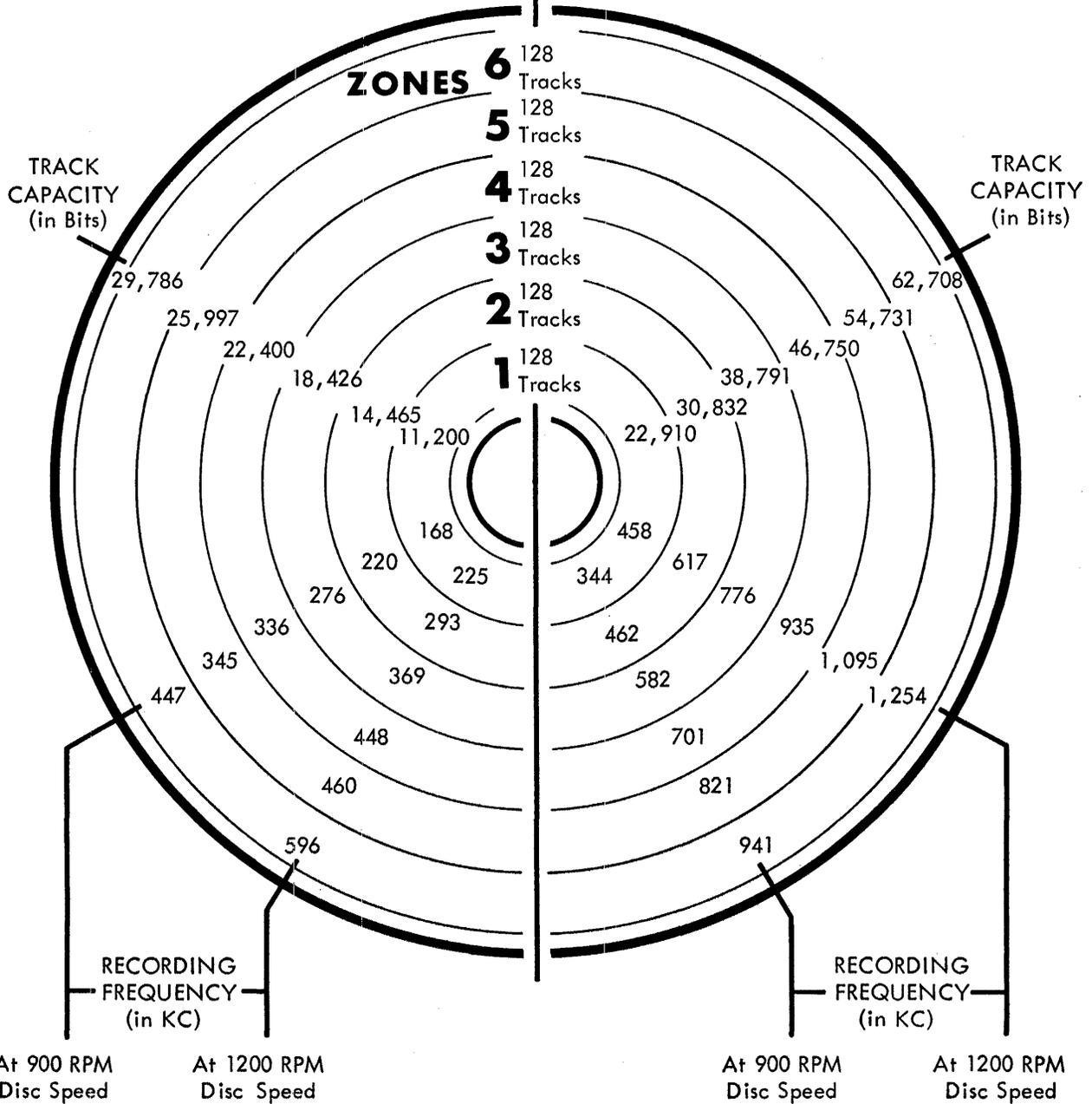
**Figure 5. MAXIMUM CAPACITIES OBTAINED WITH SIX-ZONE DISC FORMAT**
