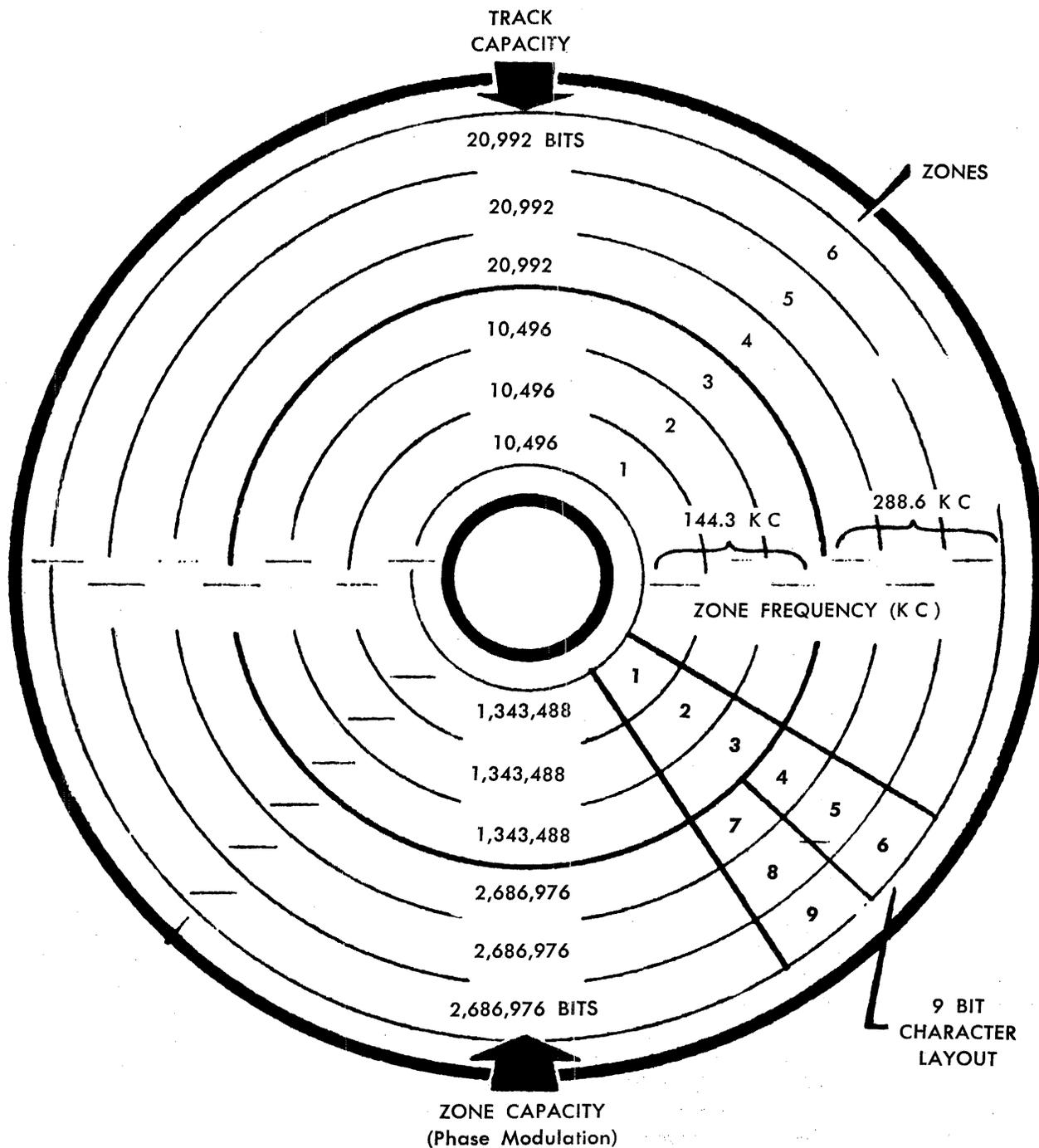
DISC SPEED: 900 RPM
