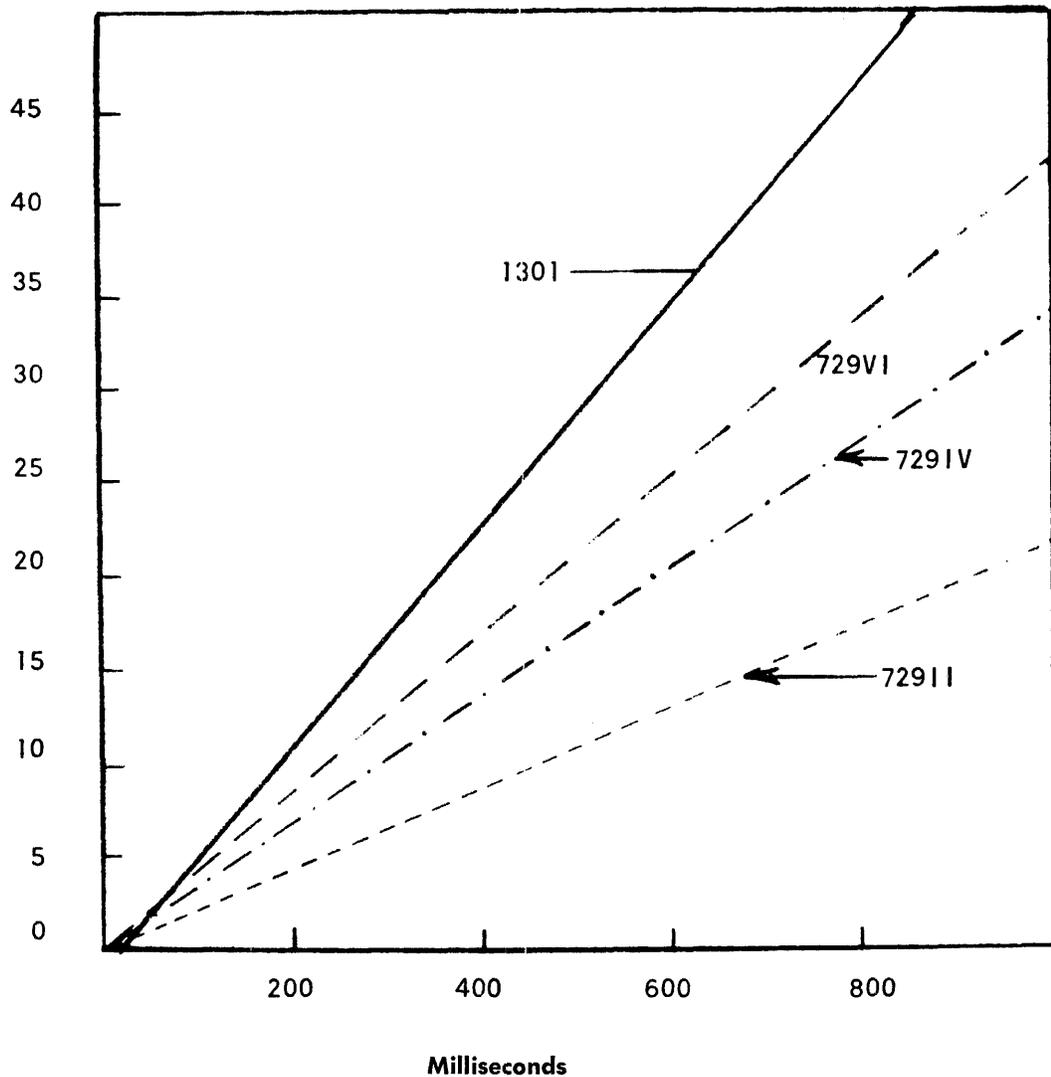
Figure 3. EFFECTIVE TRANSFER RATE OF IBM 1301 DISC AND IBM MAGNETIC TAPE UNITS FOR READING 256 IBM 7090 WORD BLOCKS
