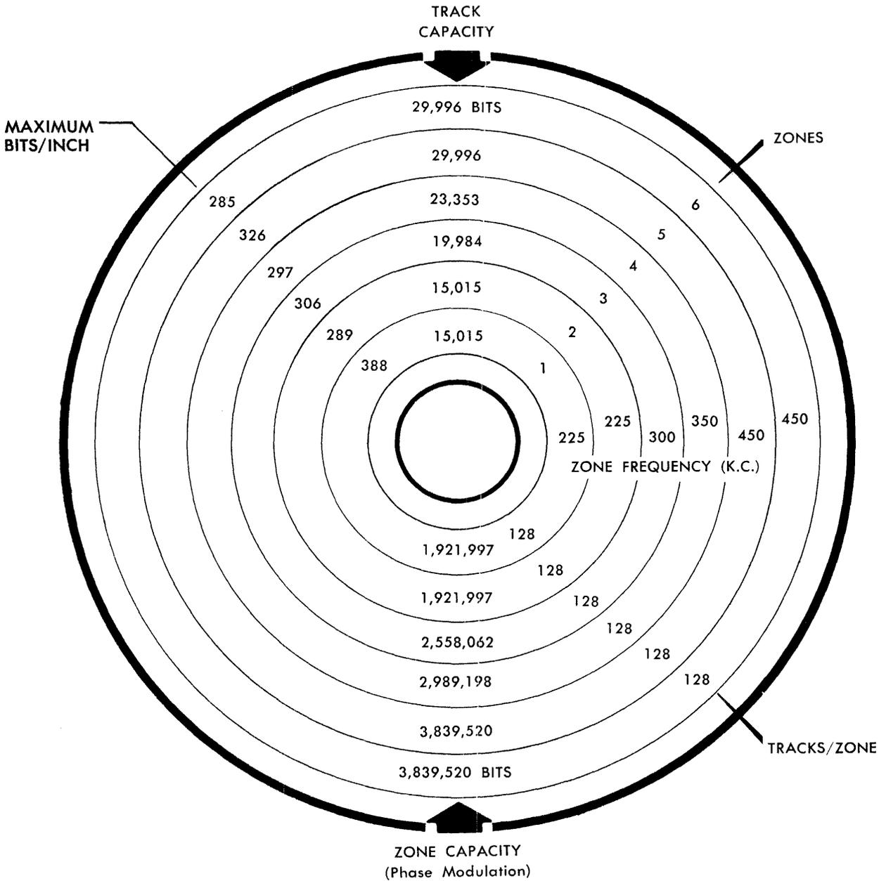
**DISC SPEED: 900 RPM**
