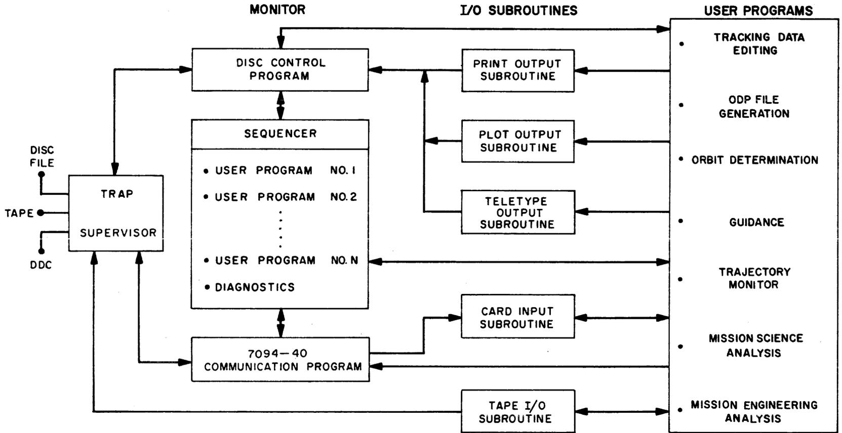
Figure 8. DISC PROGRAMMING SYSTEM
