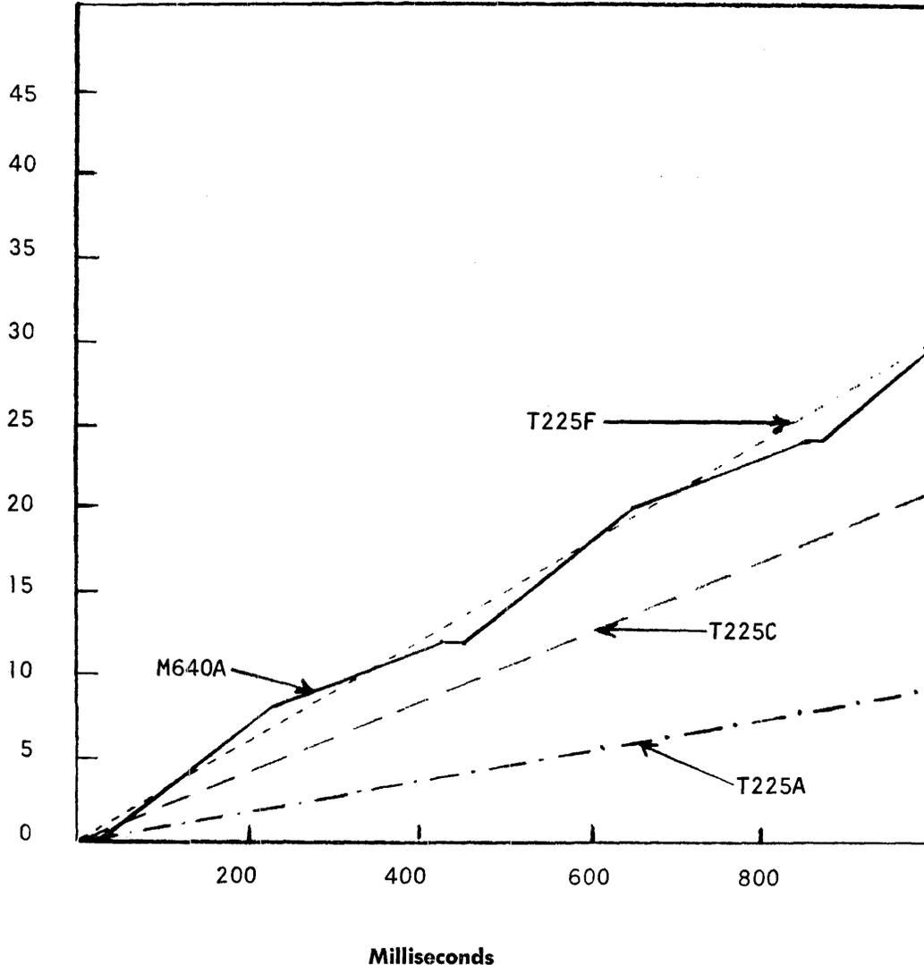
Figure 4. EFFECTIVE TRANSFER RATE OF GE 225 M640A AND GE MAGNETIC TAPE UNITS FOR READING 1536 CHARACTER BLOCKS
