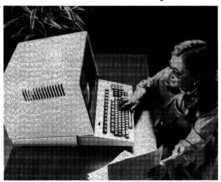
This view of the Inforex System 7000 CRT terminal shows the various key groupings on the keyboard. Immediately to the right of the alphanumeric keyboard is a full cursor control group. To the right of the cursor group is a numeric pad with plus, minus, and field termination keys. The row of elongated keys closest to the screen consists of user-programmable function keys. The elongated keys immediately above the typewriter keyboard numerics are predefined function keys.
