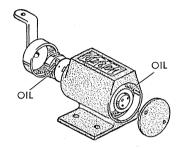
The counter ratchet assembly may be removed by removing the wire clip from the counter shaft. The assembly can then be washed thoroughly and re-lubricated. To lubricate the planetary gear system it is necessary to unscrew the end plate. This may be done by using a small punch and tapping the end plate counter. Care should be exercised not to over-lubricate as this will cloud the indicator window after use. If failing still occurs, the counter should be replaced.
