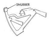
A 1/2" spring type clip (Part #1118847) is now being placed between the impression control shaft and the cam knockout bar to reduce the "hollow" sounding noise during normal typing. The clip makes the K.O. bar more rigid and, as shown by actual testing experiences, reduces noise to a more acceptable level.
