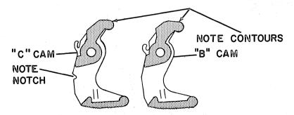
Model C cams used in Model B ET's result in a low tripping point and, in some instances, the keylever will bottom in the guide comb before tripping the cam.
