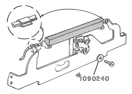
Retainer clips (Part #1110093, used to hold feed rolls in position on feed roll shaft) are now used on the Standard Model C spacebar shaft, in place of the neoprene sleeves, to reduce lateral motion of the spacebar keybutton. The retainers are placed on the inside of the bracket which supports the spacebar shaft. (See illustration above)
