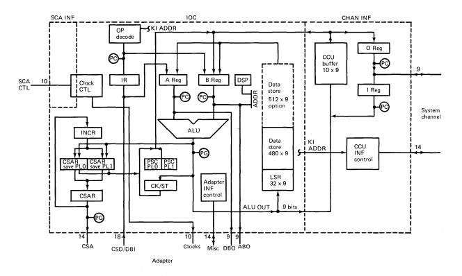
Figure 1 A data flow diagram of logic on the System/38 I/O controller card
