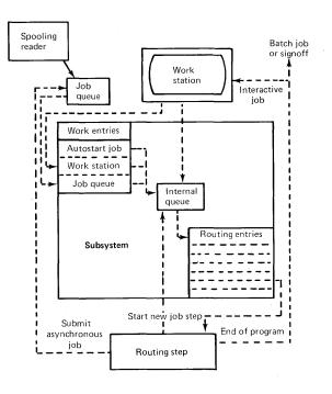
Figure 2 Work flow within an active subsystem
