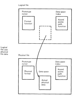
Figure 3 Machine object usage in implementing physical and logical files
