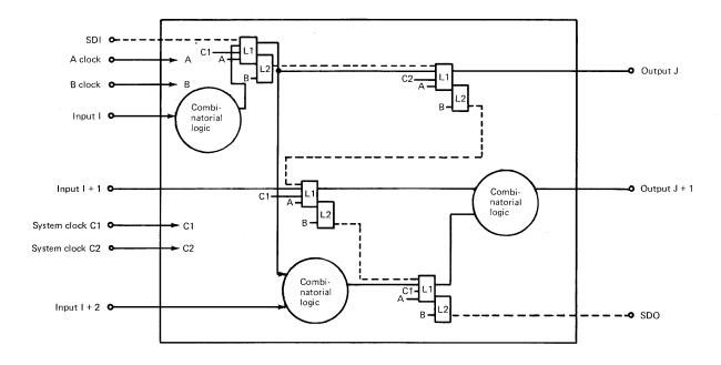
Figure 1 Typical LSSD LSI chip
