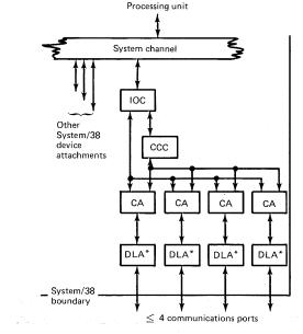
Figure 1 Communications subsystem hardware structure
