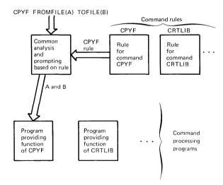
Figure 1 Processing a command in System/38
