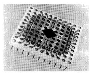
Figure 4 Single chip module before cover is added
