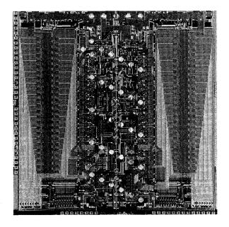
Figure 4 64K-bit array chip
