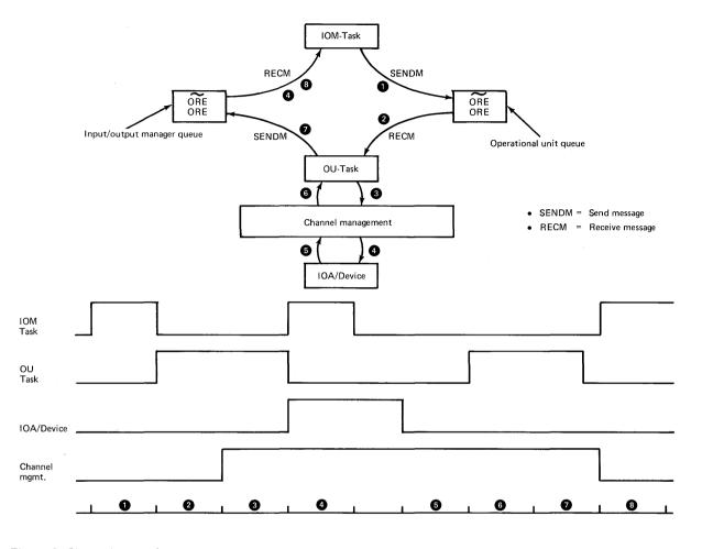
Figure 2 Channel operation
