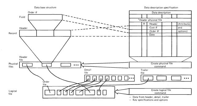
Figure 2 Relationship of the data base structure to the data description specification and creation interface
