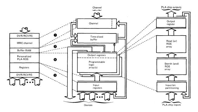
Figure 2 Magnetic media controller—functional data flow
