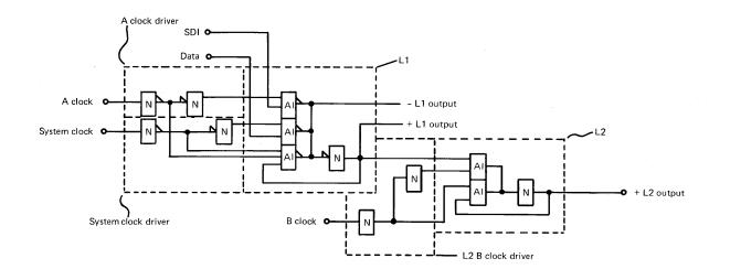
Figure 2 Shift register latch
