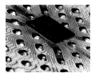
Figure 3 Closeup of mounted chip
