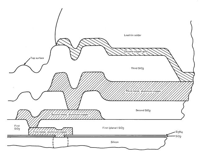
Figure 2 Three levels of metallization, showing silicon to solder ball electrical path
