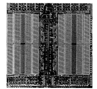
Figure 3 32K-bit array chip
