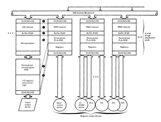
Figure 1 System/38 device attachments
