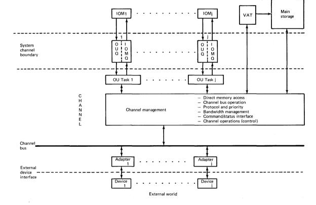
Figure 1 System/38 I/O structure
