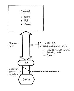
Figure 3 Channel dialog with device
