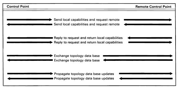
Note: This sequence will occur whenever a line is enabled on the CPSVCMG session between two networking nodes on the line and/or whenever the CPSVCMG session fails and is brought back up.
