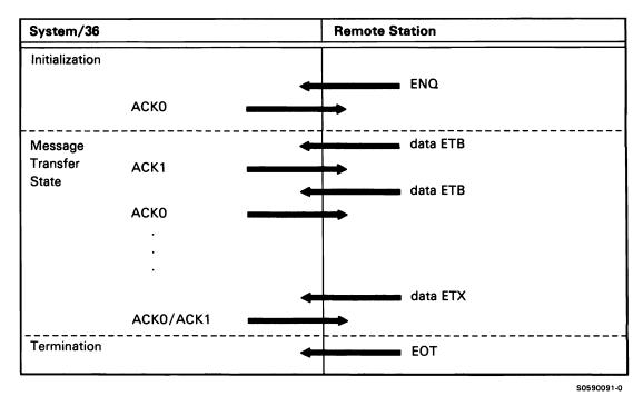
Figure A-1 (Part 6 of 13). Batch and SSP-ICF BSC Data Communications Line Protocols
