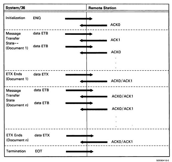
Figure A-1 (Part 13 of 13). Batch BSC (and BSCEL Subsystem) Data Communications Line Protocols
