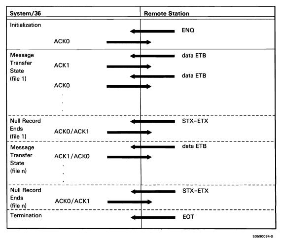
Figure A-1 (Part 10 of 13). Batch and SSP-ICF BSC Data Communications Line Protocols
