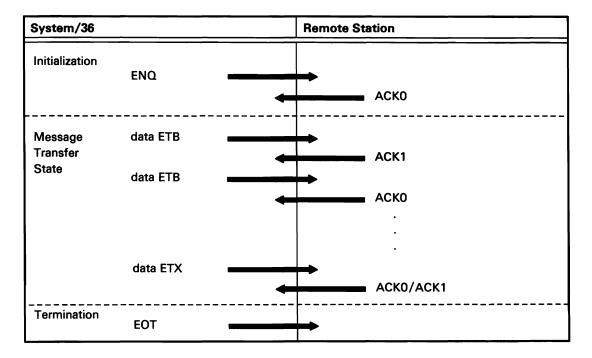
Note: If ENQs are simultaneously issued by the System/36 and the remote station, contention will continue until the remote station sends ACKO or the retry count is exceeded.
