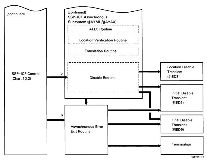
Chart 10.6.12 (Part 2 of 2) SSP-ICF Asynchronous Subsystem Control Flow
