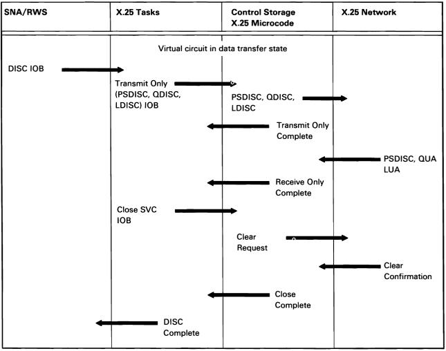
Figure A-13 (Part 5 of 7). Closing an X.25 Virtual Circuit
