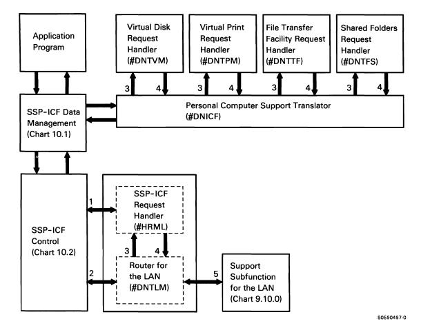
Chart 10.10.2 Personal Computer Support Subsystem Control Flow for an Environment of the LAN
