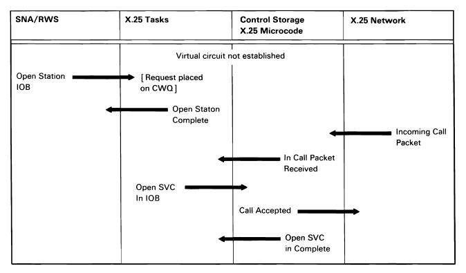
Figure A-13 (Part 3 of 7). Opening an X.25 Virtual Circuit
