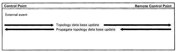
Note: External event is any action that affects the networks topology such as a node or link changing status, nodes becoming congested for routing, and disable pending. These will cause updates to flow throughout all the attached and communicating network nodes.
