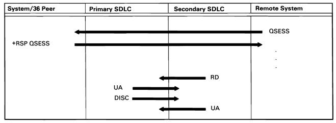
Figure A-10 (Part 7 of 31). Peer Subsystem Activation/Deactivation
