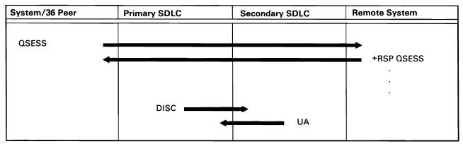
Figure A-10 (Part 5 of 31). Peer Subsystem Activation/Deactivation
