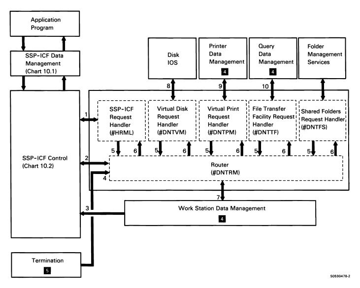
Chart 10.10.1 Personal Computer Support Subsystem Control Flow for a 5250 Environment
