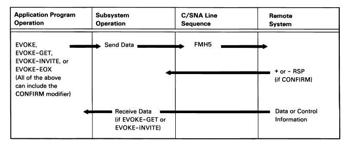
Note: The +RSP to confirm is not required if GET was specified. Instead, the data or control information is treated as a +RSP acknowledgment.
