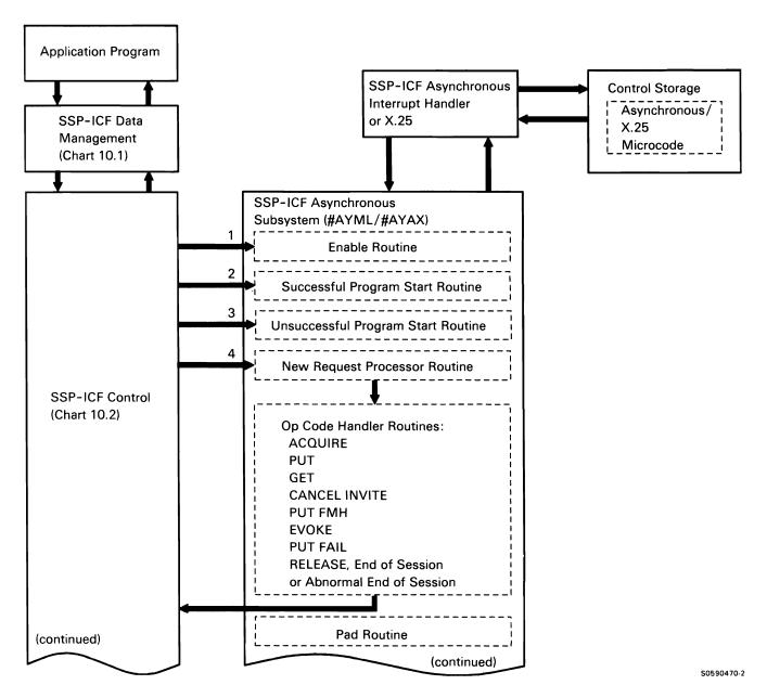
Chart 10.6.12 (Part 1 of 2) SSP-ICF Asynchronous Subsystem Control Flow
