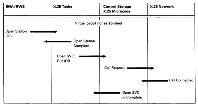
Figure A-13 (Part 4 of 7). Opening an X.25 Virtual Circuit
