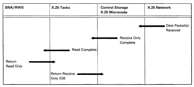
Figure A-13 (Part 7 of 7). X.25 Virtual Circuit Data Transfer
