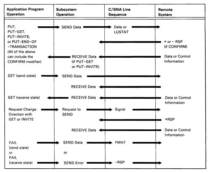
Note: The+RSP is not required if GET was specified. Instead, the data or control information is treated as a +RSP acknowledgment.
