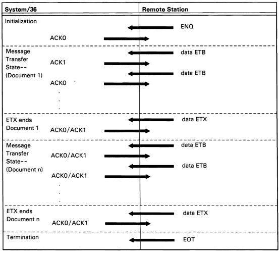
Figure A-2. SSP-ICF BSCEL Subsystem Line Protocols
