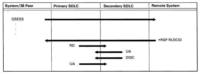
Figure A-10 (Part 6 of 31). Peer Subsystem Activation/Deactivation
