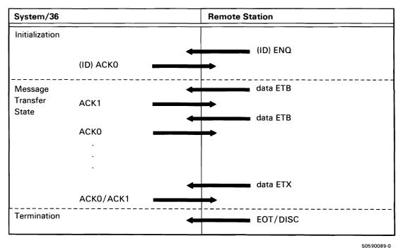
Figure A-1 (Part 4 of 13). Batch and SSP-ICF BSC Data Communications Line Protocols
