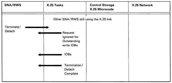
Figure A-13 (Part 2 of 7). X.25 Link Termination
