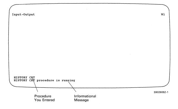
After the Input-Output display is shown, the system displays your history file. After you view your history file, press command key 7 to return to the display on which you typed the name of the procedure.
