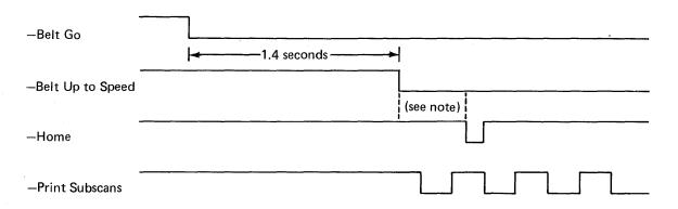
*Note:* The 'home' pulse may not always occur where shown in this timing chart. The time between an active 'belt up to speed' line and an active 'home' pulse may vary.
