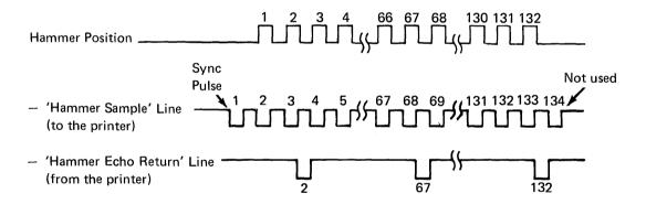
*Note:* Hammer 2 is the first failing hammer, and there are 3 failing hammers (2, 67, and 132).
