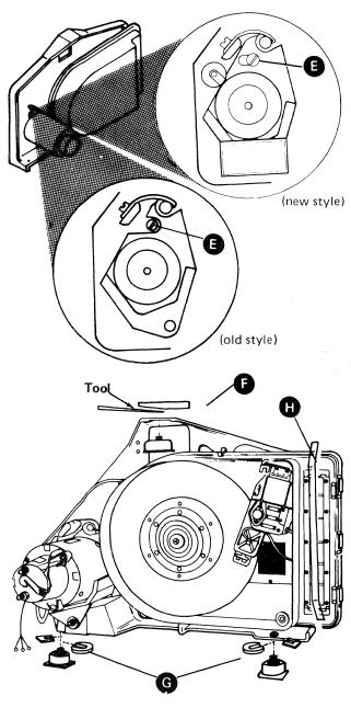
Place tape on the wood block (P/N 7354979) and wedge (P/N 7320154) and insert between disk casting and disk frame as illustrated. Attach tape to frame.
