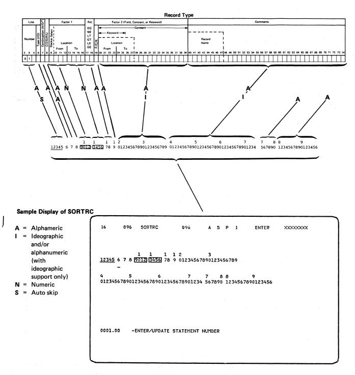
Figure 2-26. Sort Format: SORTRC, Record Type Constant Specification
