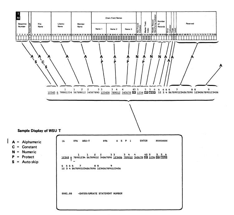
Figure 2-17. Work Station Utility Format: WSU T
