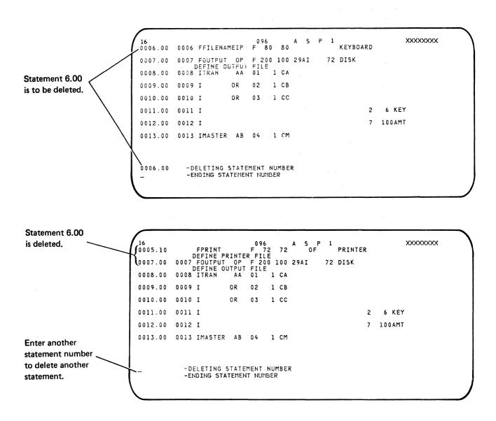
Figure 6-5. Sample Displays for Deleting a Single Statement
