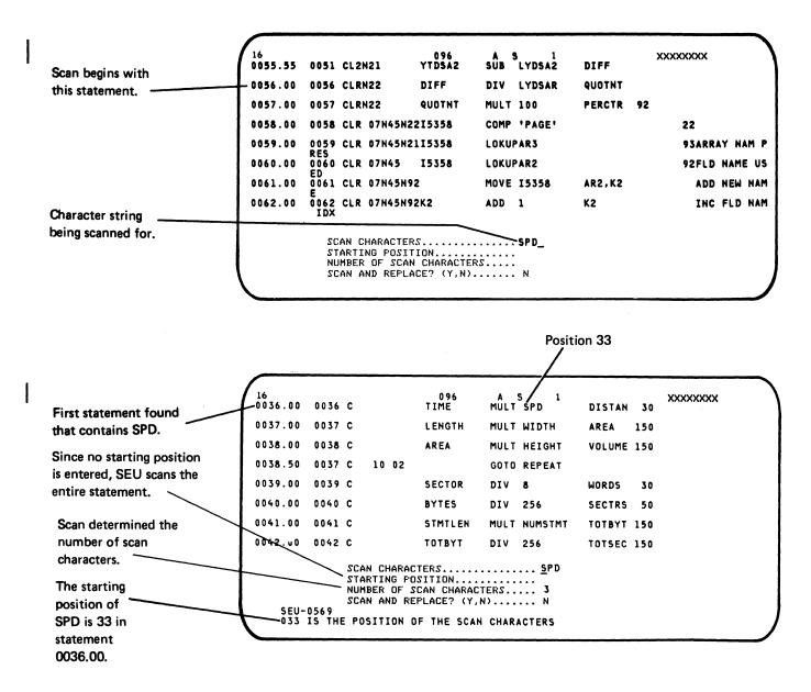
Figure 6-17. Example of Scan Mode
