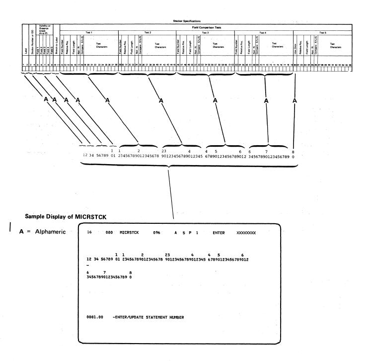
Figure 2-31. Magnetic Character Reader Format: MICRSTCK, Stacker Specification
