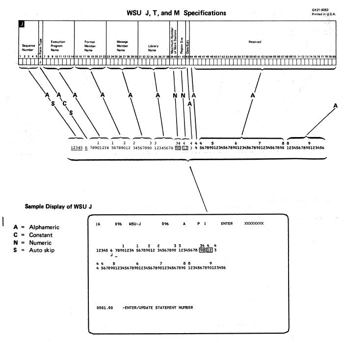
Figure 2-16. Work Station Utility Format: WSU J
