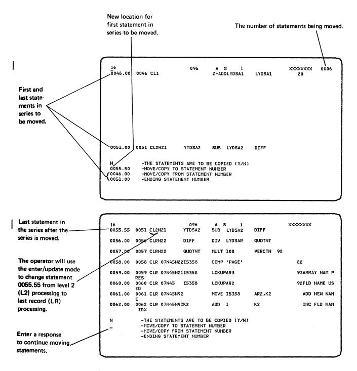
Figure 6-10. Sample Displays for Moving a Series of Statements
