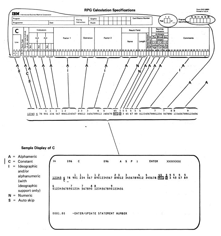
Figure 2-11. RPG II and Auto Report Format: C, Calculation Specification
