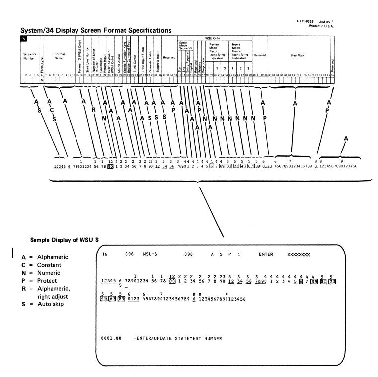
Figure 2-19. Work Station Utility Format: WSU S
