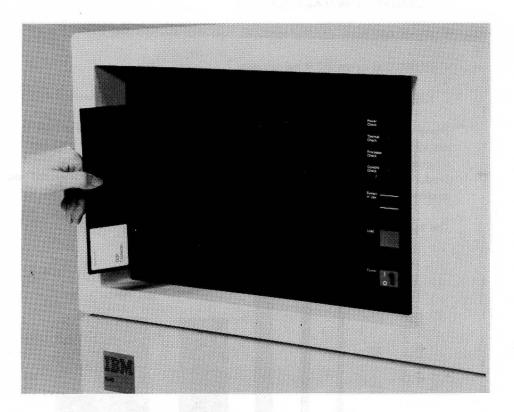
The diskette provides disk storage backup and separate storage of data that might otherwise take up needed space on the disk. Before you can process data or execute a program that is on diskette, you must move the data or program onto disk. Once you have moved the data or program onto disk you can leave it there. Diskettes can also provide input from another device or system that uses diskettes, such as a 3741 Data Entry Station.
