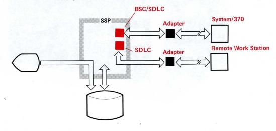
The communications adapters can use half-duplex communication (one direction at a time), with either two-wire or four-wire facilities. Each communications adapter supports data rates from 600 to 9,600 bits per second (8 bits equal 1 byte). The maximum data rate flow with both lines operating concurrently is 9,600 bits per second.
