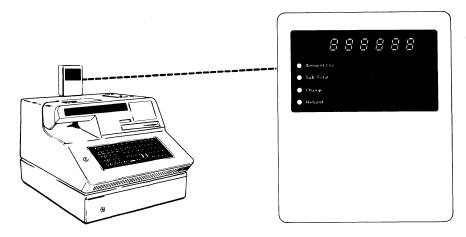
The IBM 5260 Retail System consists of point-of-sale terminals that help provide data processing answers for the operational and accounting areas of retailing. Point-of-sale terminals provide traditional cash register functions as well as data collection capabilities.
