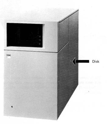
The disk provides quick-access magnetic storage for programs and data files. Disk storage has five *approximate* capacities:
