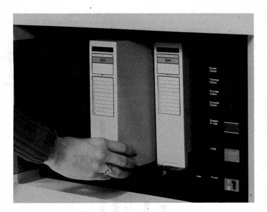
System/34 has an optional diskette magazine drive that can read from and write on Diskette 1 and Diskette 2D. The diskette magazine drive has five slots; two of them hold magazines and three hold individual diskettes. A magazine is a container that holds up to 10 diskettes.
