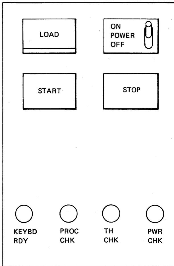
Figure 2-1. Operator's Console
