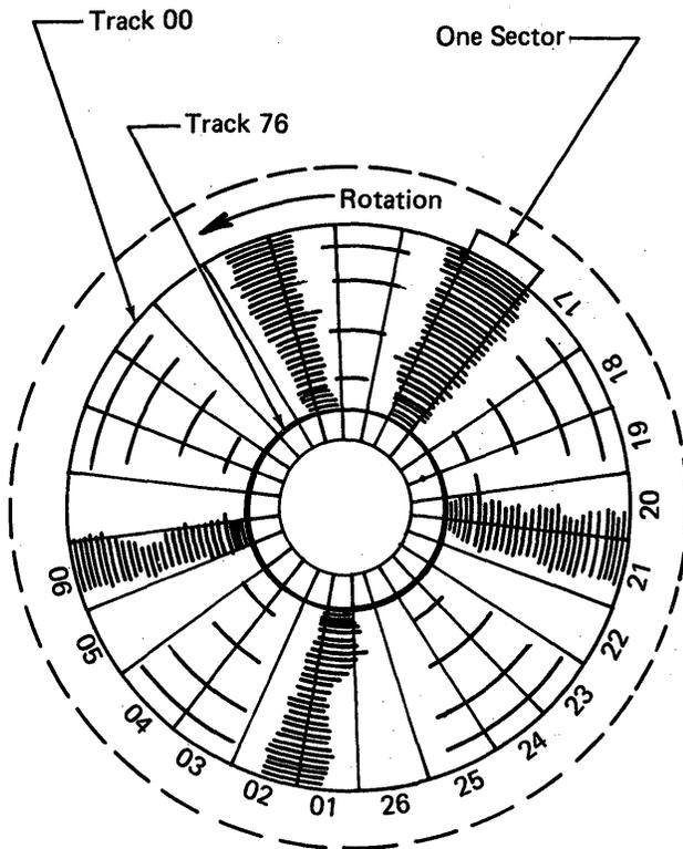
Figure 8-1. Standard Interchange Diskette Surface Recording Arrangement
