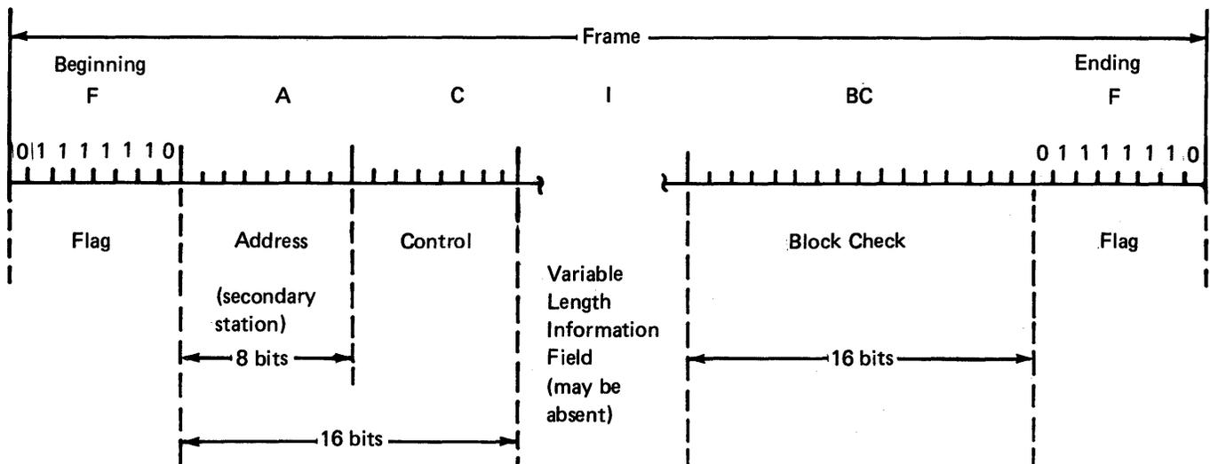
Figure 9-7. SDLC Transmission Frame
