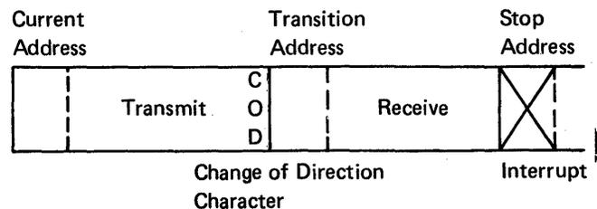
**Figure 9-4. I/O Area and Address Register Contents at Start of Transmit and Receive Operation**
