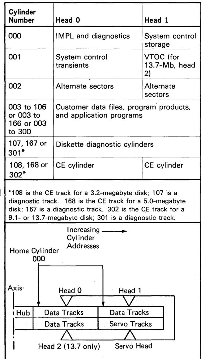
Figure 6-1. Disk Surface Partitioning Diagram
