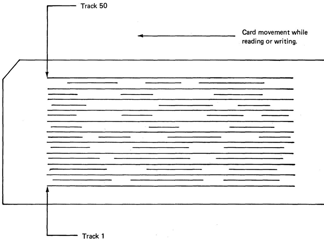
Figure 10-1. Magnetic Card Track Recording Arrangement
