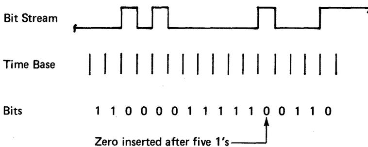
**Figure 9-14. NRZI Transmission Coding**
