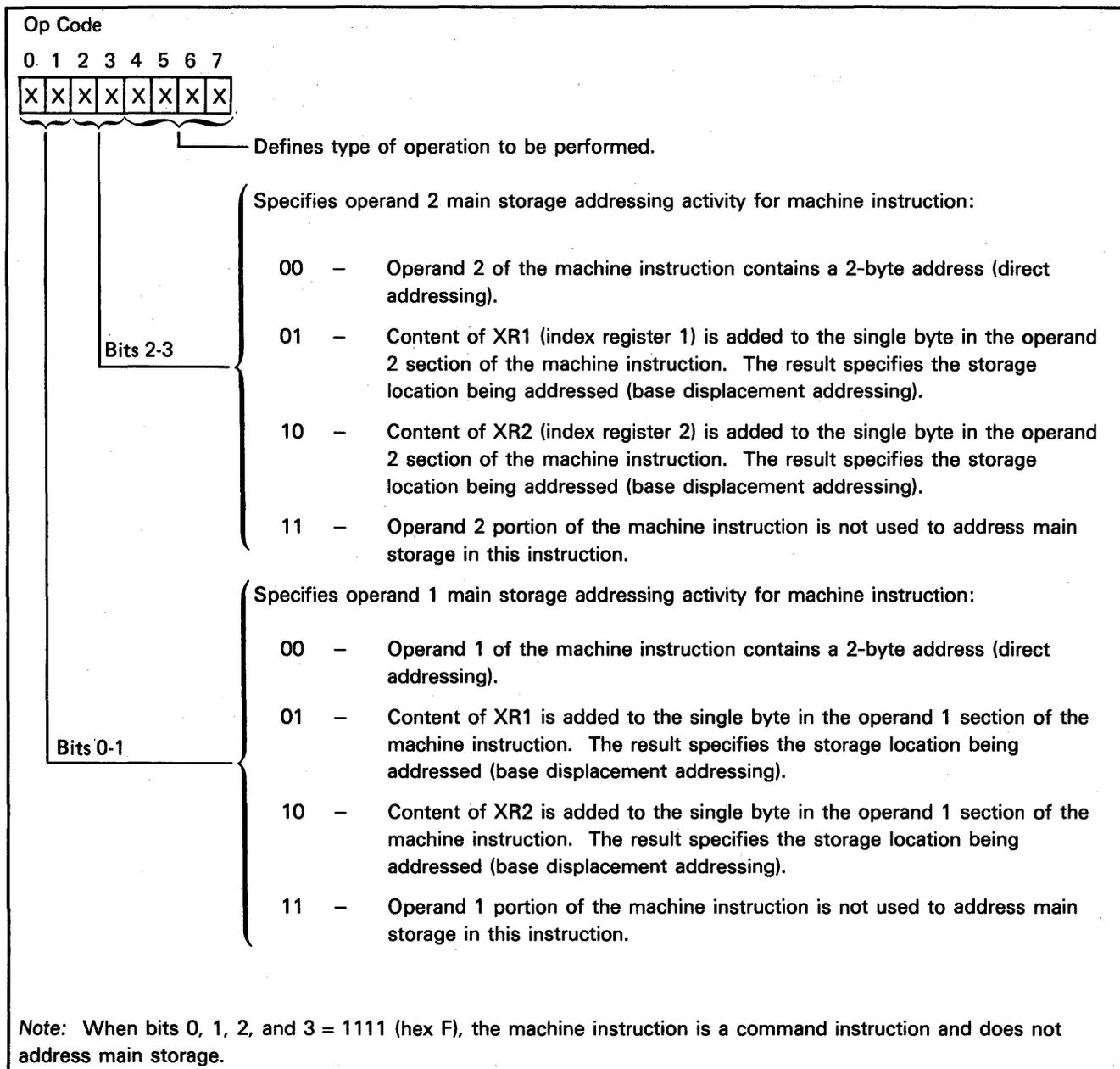
Figure 1-2. Op Code Function in Addressing Main Storage
