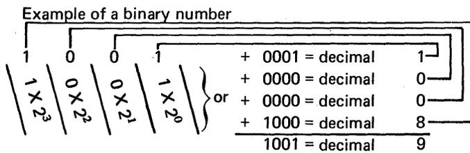
The decimal number system allows counting to 10 in each position, from units to tens to hundreds to thousands, etc. The binary system allows counting to two in each position. CE panel displays are in binary form: a bit light on is indicated by a 1; a bit light off is indicated by a zero.
