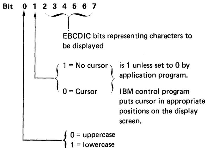
Bit 1 of each byte of data in the 240-byte display field determines if the cursor is displayed with that byte. For each EBCDIC character that has bit 1 = 0, a cursor is displayed directly below that character. All valid EBCDIC characters have a 1 in the bit-1 position unless set to 0 by a program. (See Appendix B for the EBCDIC displayable subset.)
