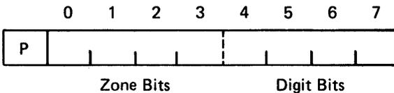
For decimal arithmetic operations, the zone bit of the rightmost byte in the field indicates the sign of the numbers. (The system ignores the zone bits in all other bytes during the operation.) Zones containing hex B or D (binary 1011 or 1101) designate a negative number. Any other hex digit in the zone designates a positive number.
