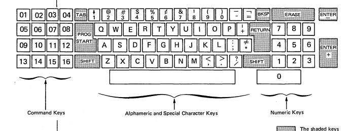
The operator keyboard is the device the operator uses most often for entering information into the Model 6. The operator can enter:
