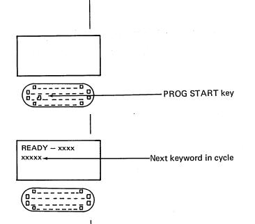
After typing in the name of the OCL cycle you want to use for the job, the operator presses the PROG START key.
