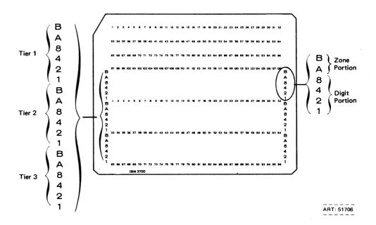
Figure B-1. Punch Positions in a Card
