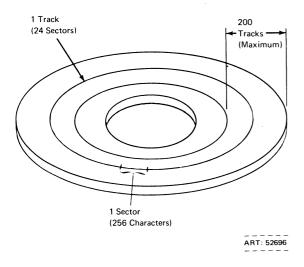
Figure 4-5. Tracks and Sectors on a Disk
