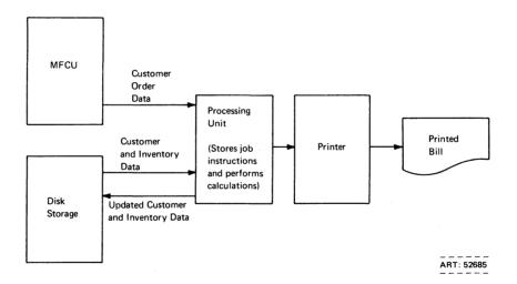
Figure 1-2. Input, Processing, and Output Functions
