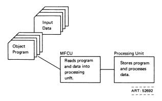
Figure 3-3. Loading a Program and Input Data
