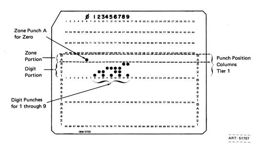
Figure B-2. Numeric Punches in a Card
