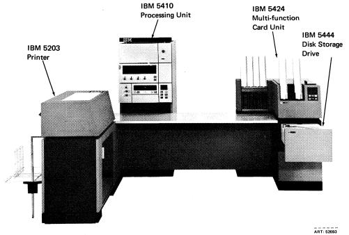
Figure 4-1. IBM System/3 Disk System
