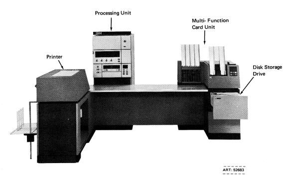
Figure 1-1. IBM System/3 Disk System
