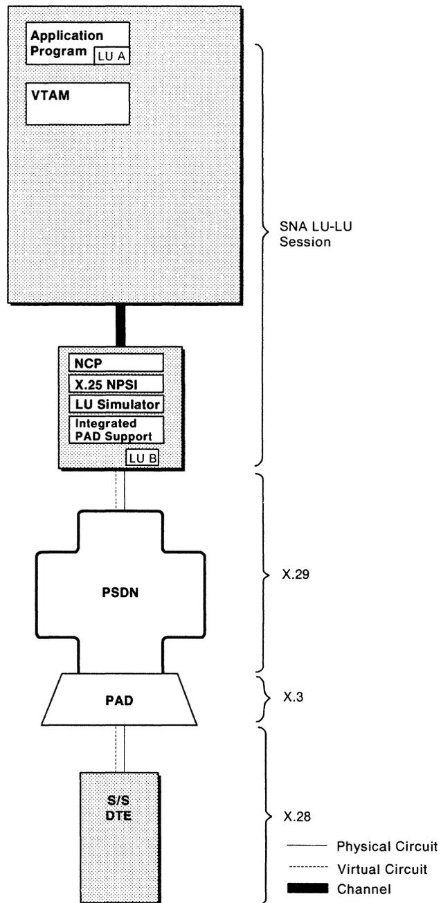
Figure 12. SNA Host Node to Non-SNA X.25 DTE (Integrated PAD Support)
