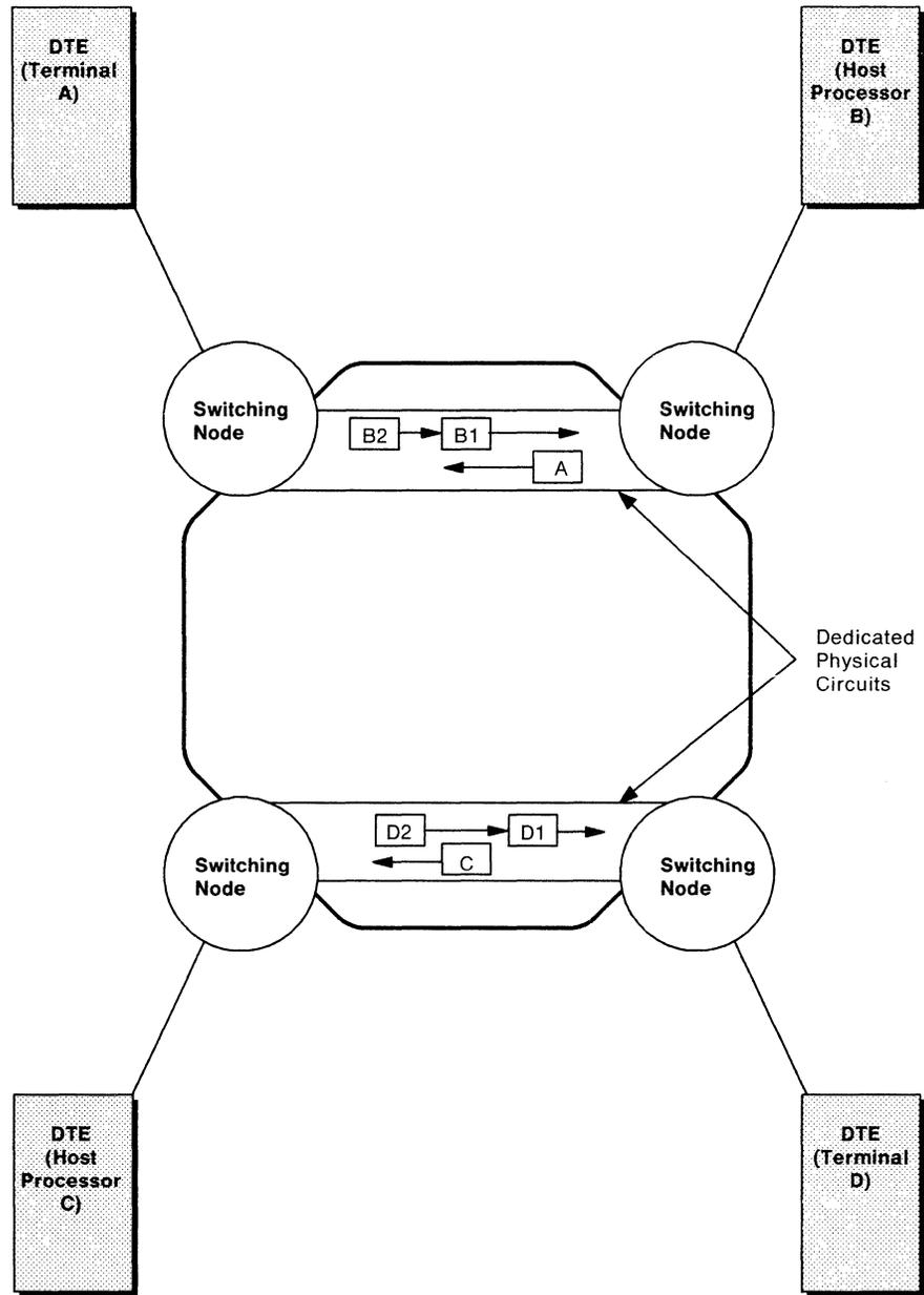
Figure 2. Circuit Switched Data Network (CSDN)
