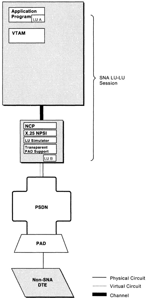
Figure 13. Host Node to Non-SNA X.25 DTE (Transparent PAD Support)
