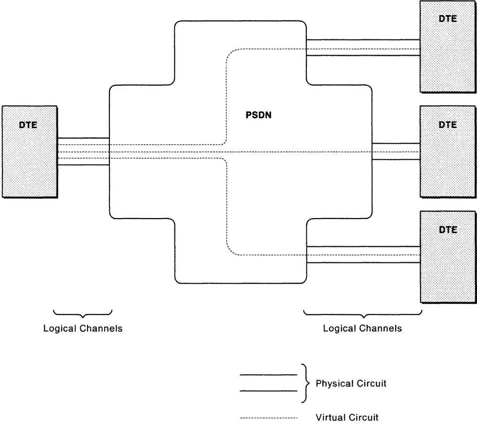
Figure 6. Logical Channels and Virtual Circuits through a PSDN
