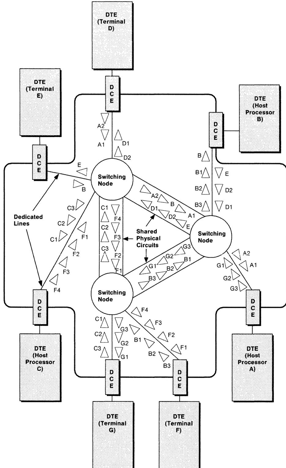
Figure 3. Packet Switched Data Network (PSDN)
