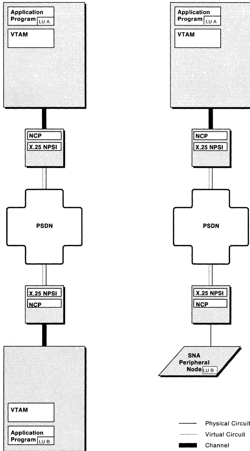
Figure 8. Communication between Subarea Nodes
