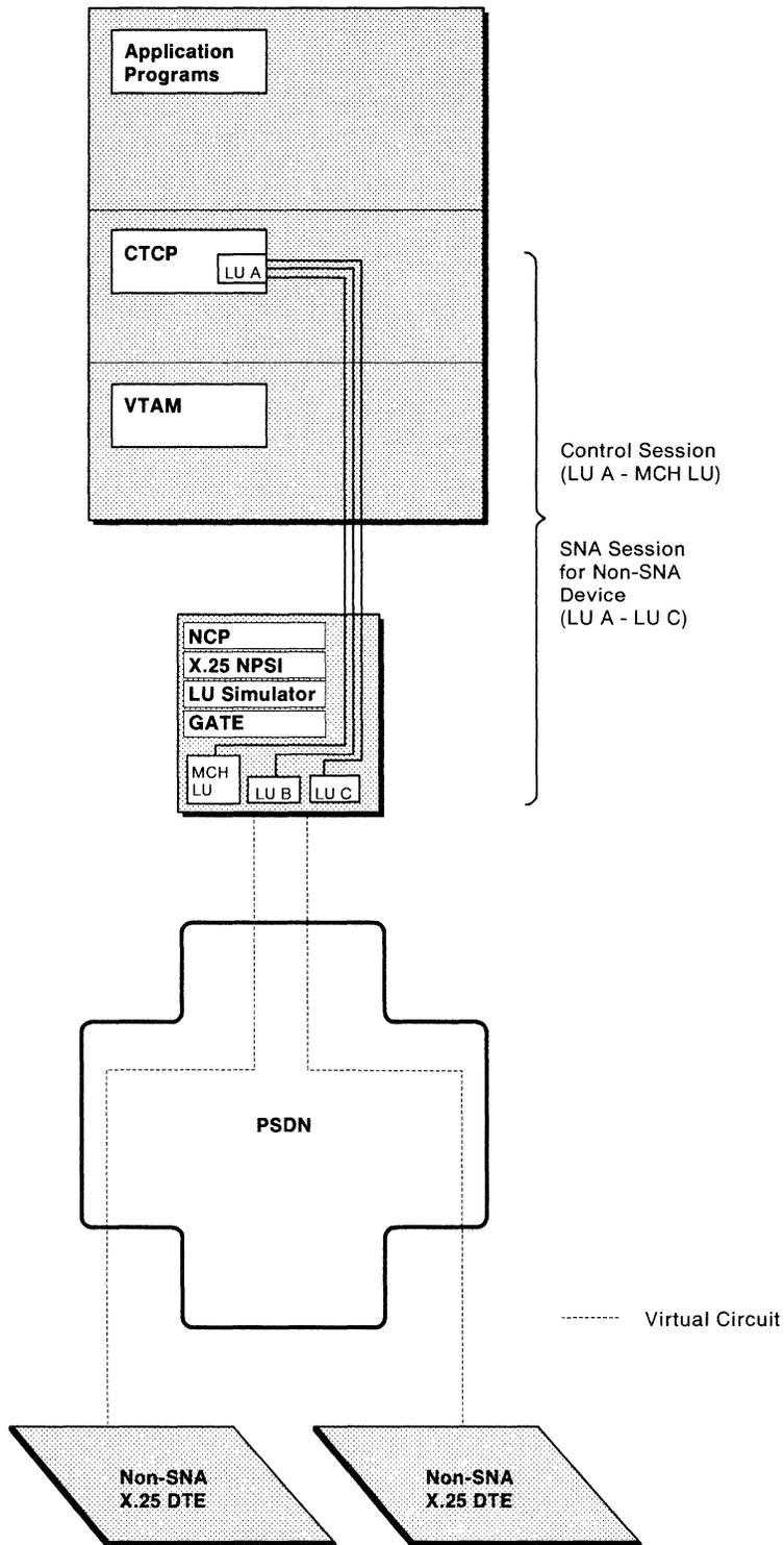
Figure 14. Host Node to Non-SNA X.25 DTE (GATE)
