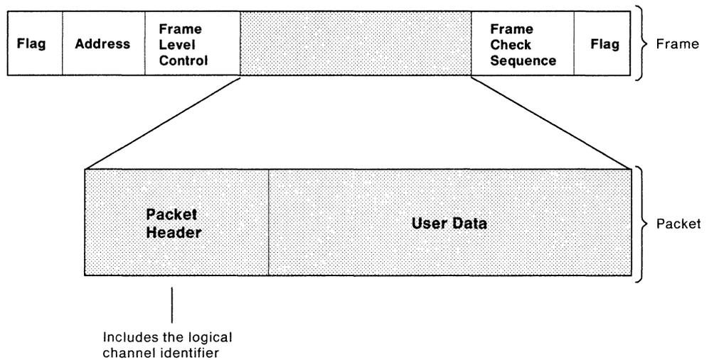
Figure 5. Frame and Packet
