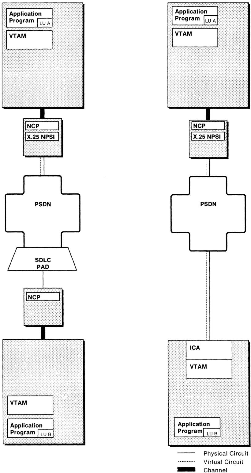
Figure 9. More Communication between Subarea Nodes
