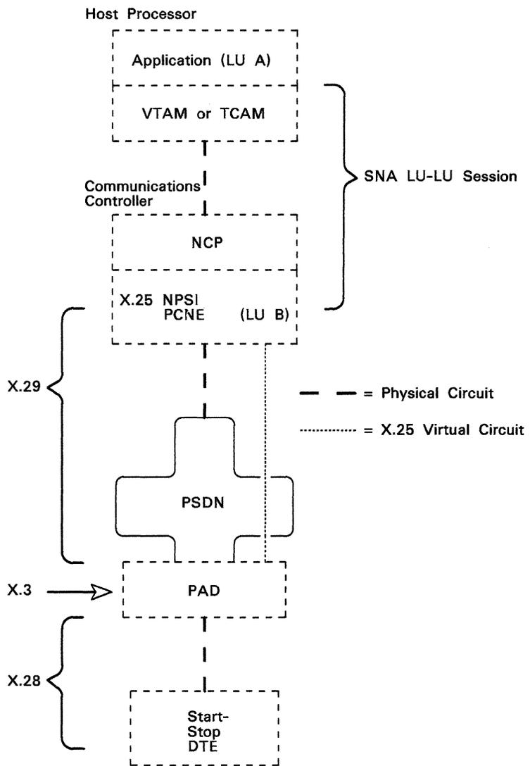
**Figure 2-4. Host Processor Communicating with an X.28 Start-Stop DTE Using the Integrated PAD Function**
