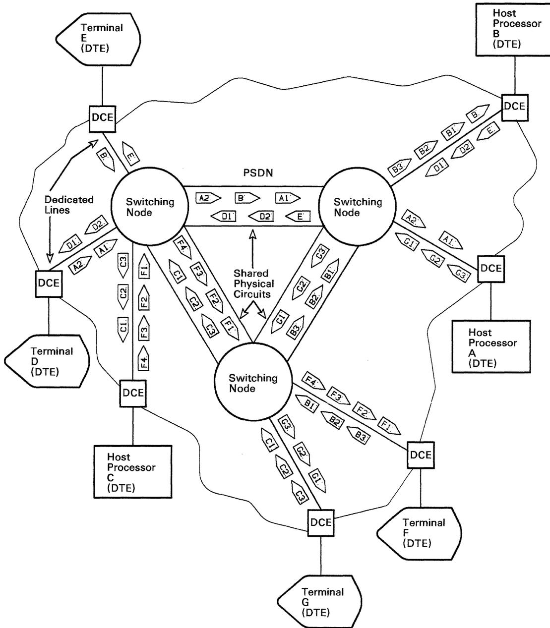
Figure 1-2. Transfer of Packets over a PSDN
