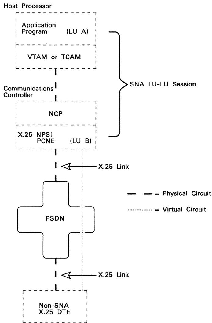
Figure 2-2. SNA Host Node Communicating with a Non-SNA X.25 DTE Using the PCNE
