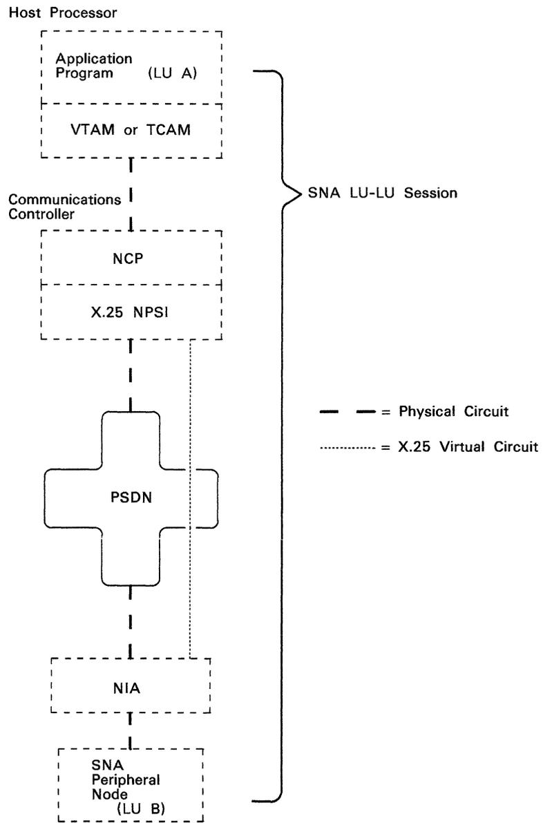
**Figure 2-1. SNA Host Node Communicating with SNA Peripheral Node over a PSDN**
