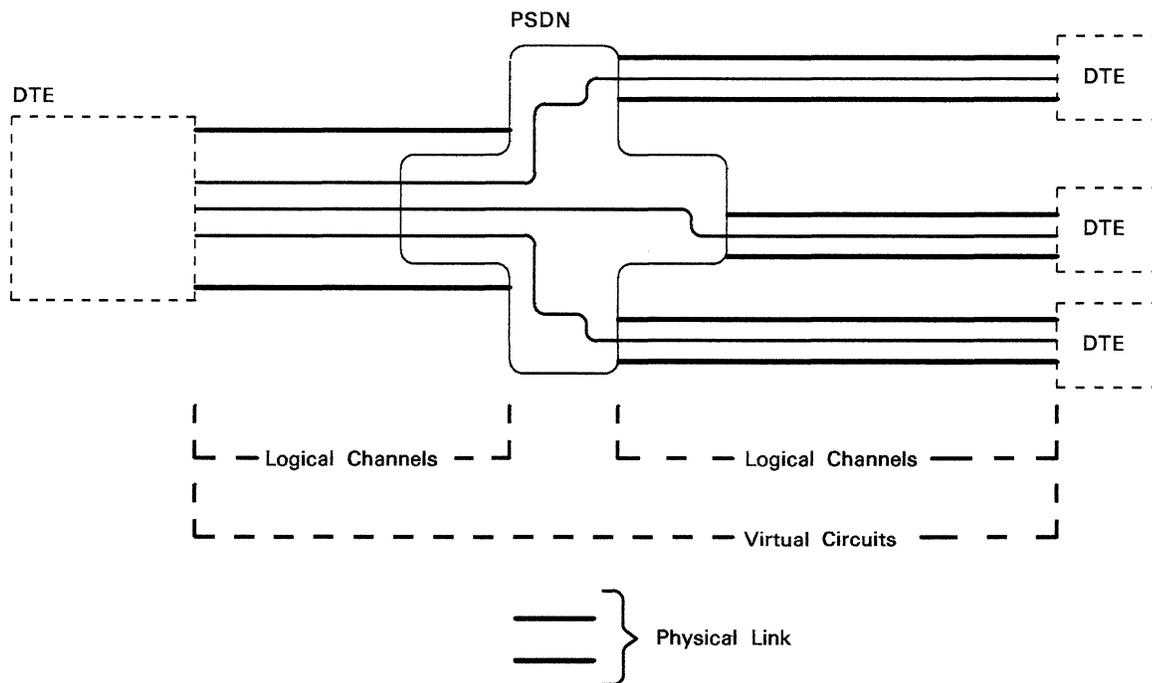
Figure 1-5. Logical Channels and Virtual Circuits through the PSDN
