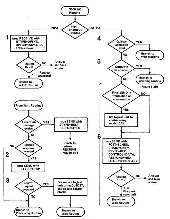
Figure 5-28. The Logic of the 3600 I/O Routine
