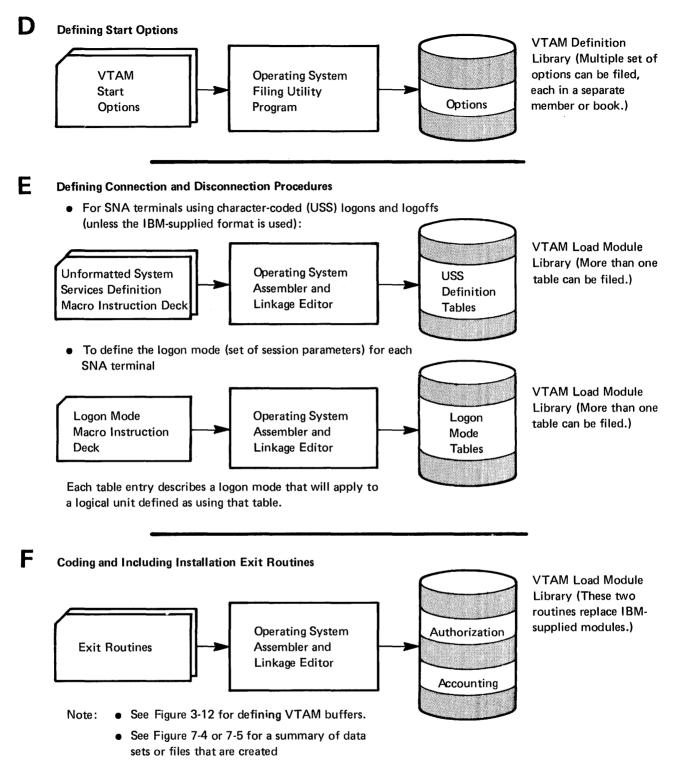
Figure 3-1 (Part 2 of 2). The Steps in Creating a VTAM Telecommunications System
