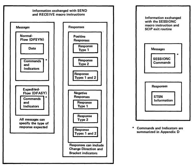
Figure 5-18. Types of Information Exchanged Between an Application Program and Logical Unit
