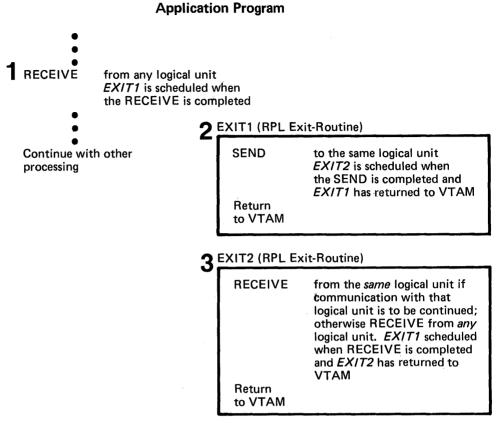
Figure 5-8. A Possible Processing Pattern When Asynchronous Requests Are Issued in RPL Exit Routines
