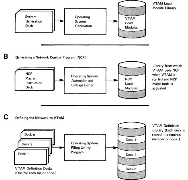
Figure 3-1 (Part 1 of 2). The Steps in Creating a VTAM Telecommunications System
