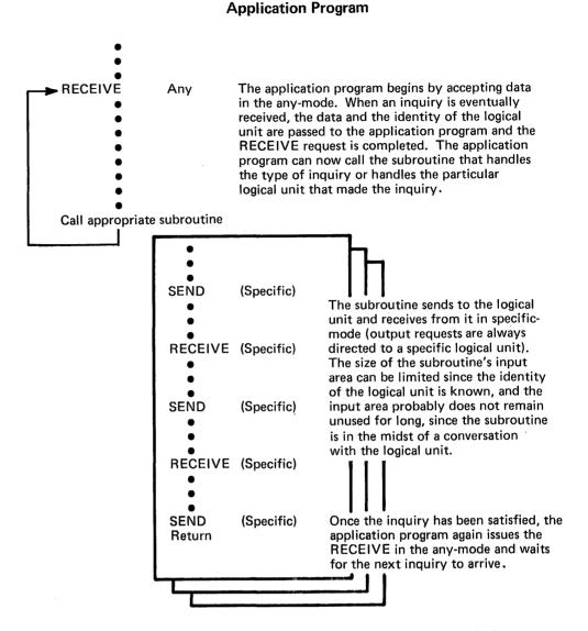
Figure 5-19. Using a Combination of Any-Mode and Specific-Mode to Obtain Data
