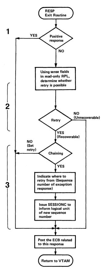
Figure 5-31. The Logic of the RESP Exit Routine
