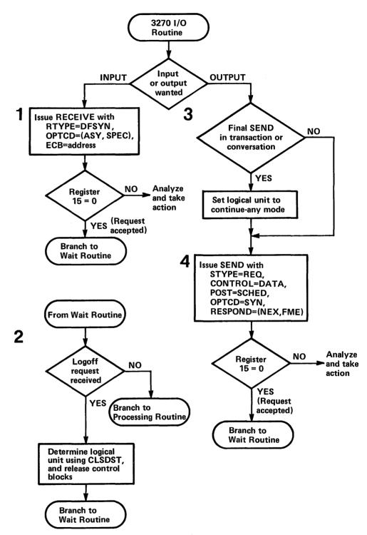
Figure 5-30. The Logic of the 3270 I/O Routine
