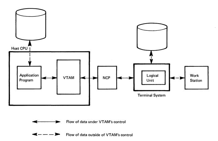
Figure 2-4. Data Flow Through a VTAM Telecommunication System
