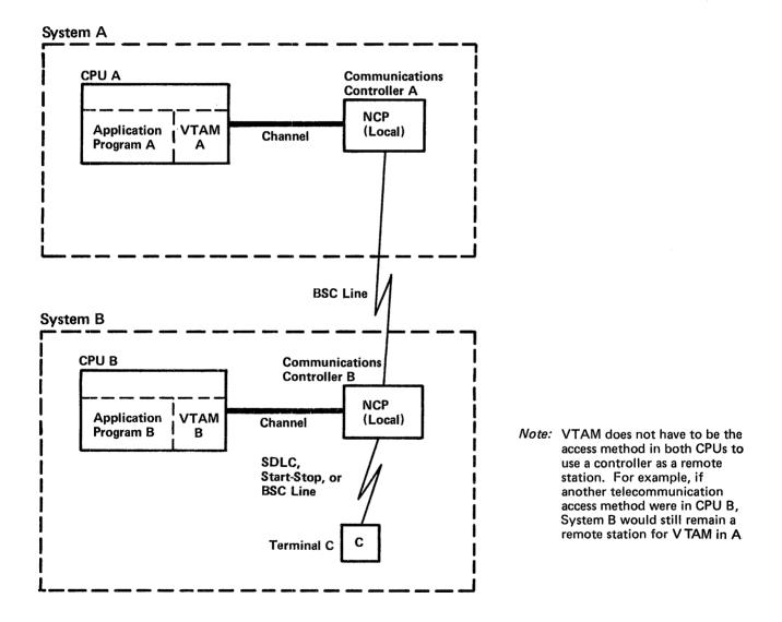
Figure B-2. Communications Controllers Attached as Part of Remote Stations
