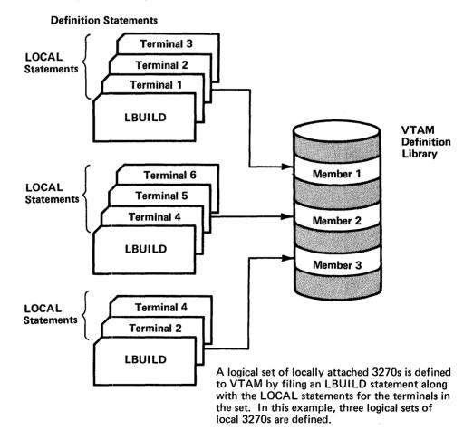
Figure 3-3. Grouping Locally Attached 3270s into Logical Sets
