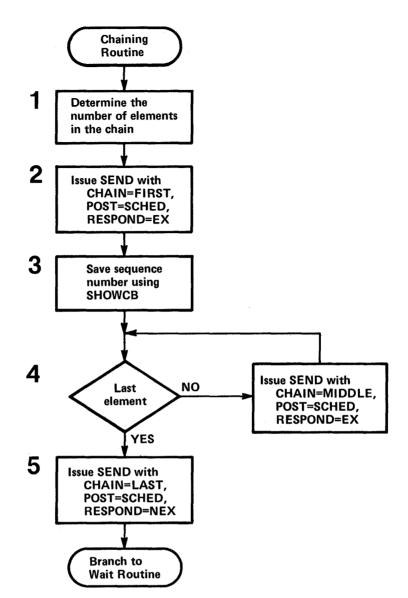
Figure 5-29. The Logic of the 3600 Chaining-Output Routine
