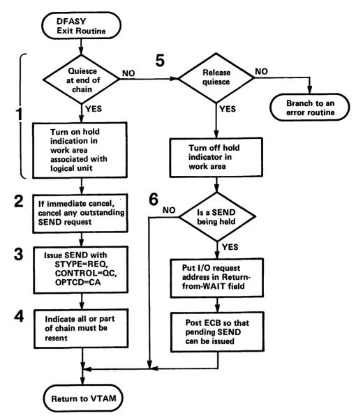
Figure 5-32. The Logic of the DFASY Exit Routine
