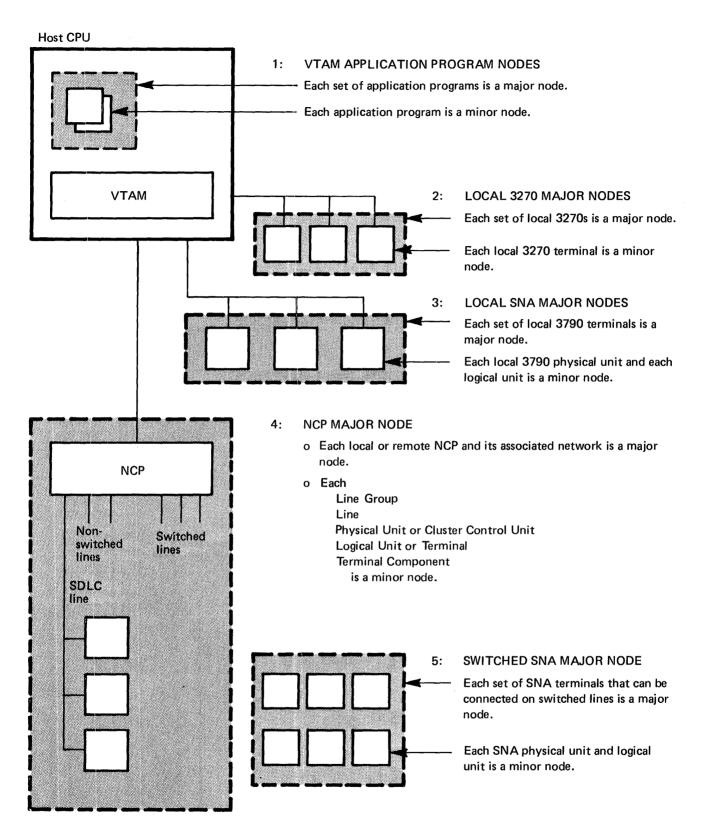
Figure 2-2. Major and Minor Nodes in a VTAM Telecommunications System
