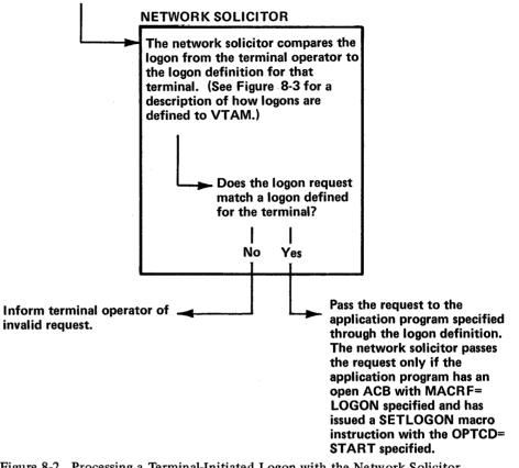
Figure 8-2. Processing a Terminal-Initiated Logon with the Network Solicitor
