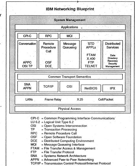
As indicated in the figure, CTS represents a common means for interfacing several applications or application programming interfaces (APIs) to a variety of transport protocols. MPTN, not shown explicitly in the figure, is one of the means to provide CTS. There are two main benefits of CTS and MPTN:
