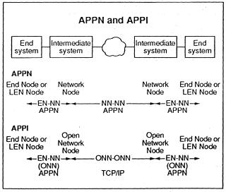
The APPN end nodes would register their resources to an ONN, as they would with an APPN network node, through the usual APPC general data stream (GDS) variables. APPI ONNs would also support the older LEN nodes, but these nodes and their resources would have to be statically configured in the ONN or a distributed directory server. An ONN could also support a network node by treating it as a LEN node and configuring a table of its resources.
