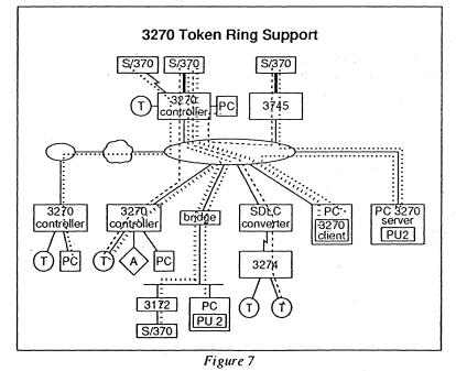
But many users are unaware that their controllers can be upgraded to access multiple SNA hosts, Digital Equipment Corporation (DEC) systems through local area transport (LAT) protocols, TCP/IP systems through telnet and tn3270, and AS/400 systems through 5250 emulation. Controllers can also be enhanced to connect to APPN, Ethernet, and ISDN networks and the ESCON channel. Even older controllers that do not support LAN adapters can access LANs through SDLC converters.
