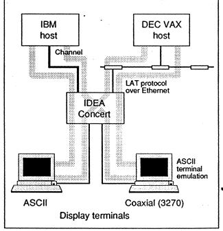
Controller replacement. Just as the 7100 offers capabilities not offered on the IBM 3174, so the 6100 offers more features than the 3172. In this article, we only consider its role as a device for connecting up to six Ethernet LANs to one or two IBM host channels.)
