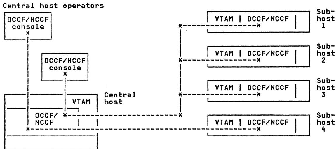
Figure 6. Multiple sub-hosts controlled through OCCF
