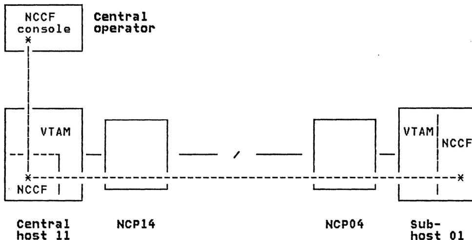
Figure 16. Configuration with a remote sub-host
