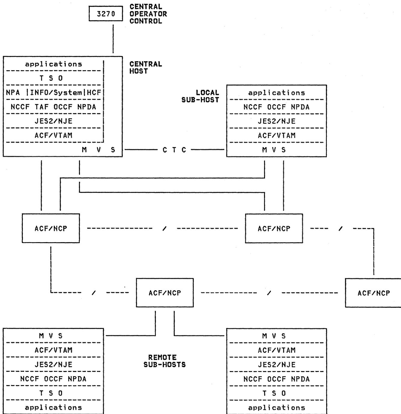
Figure 1. Sample of a centrally controlled configuration
