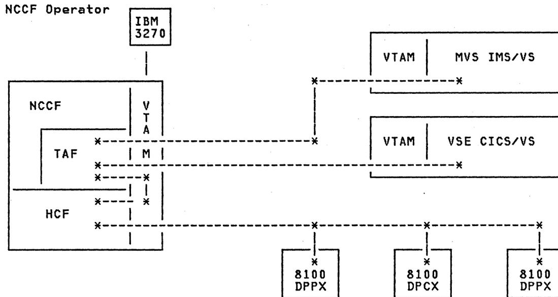
Figure 19. Centralized operation with NCCF/TAF: One NCCF operator controlling one IMS/VS, one CICS/VS, one IBM 8100/DPCX, and two IBM 8100/DPPX.
