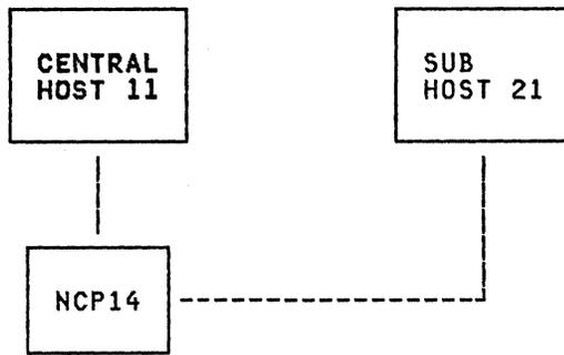
Figure 13. Sample Configuration: Two hosts share a single channel attached.NCP
