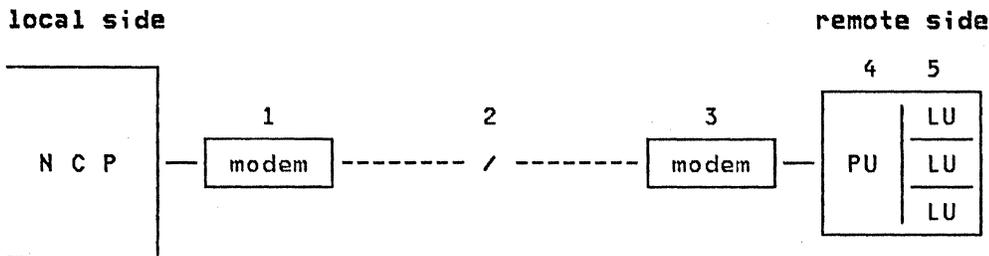
Figure 17. Sample of an NCP to cluster controller connection
