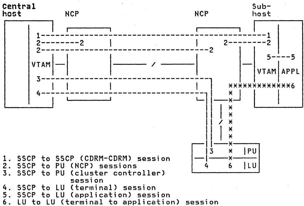
Figure 11. Sample sessions in a multiple domain configuration: The central host controls the PUs and LUs of both NCPs
