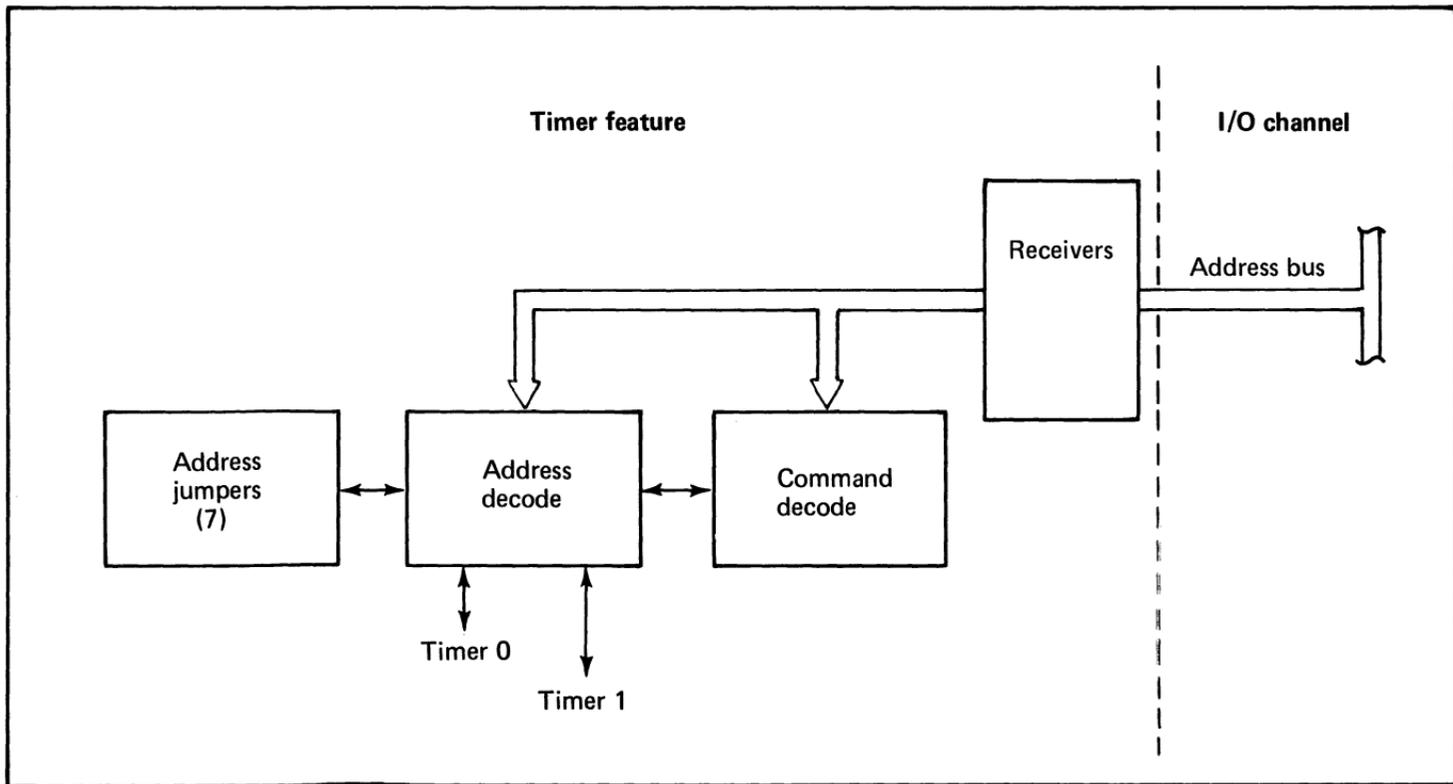
333 Figure 94. Block diagram of the timers showing their input/output channel connections and external signals for special uses (1 of 3)
