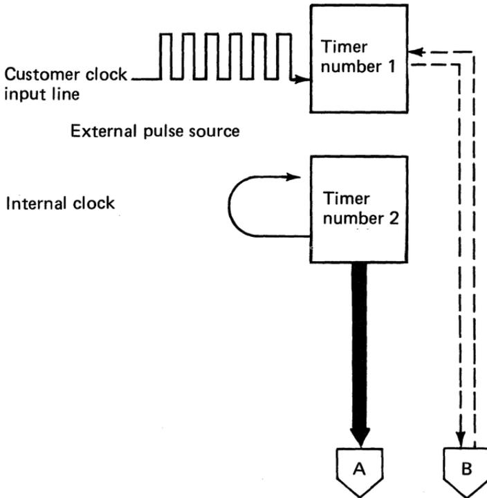
**Figure 96. Pulse rate measurement using a pair of timers (1 of 2)**
