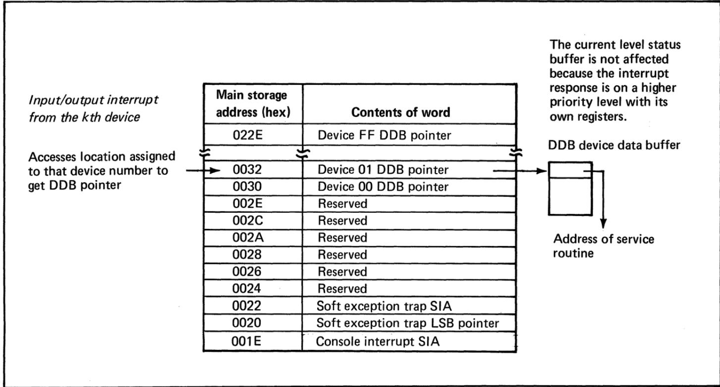
**Figure 23. Input/output and class interrupts and the response of the processor (1 of 2)**
