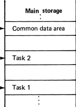
Example of two tasks, task 1 and task 2, cooperating in updating a shared data area. Address keys for fetching and writing data into the data area must be the same. Program areas use different keys and are protected against being overwritten.
