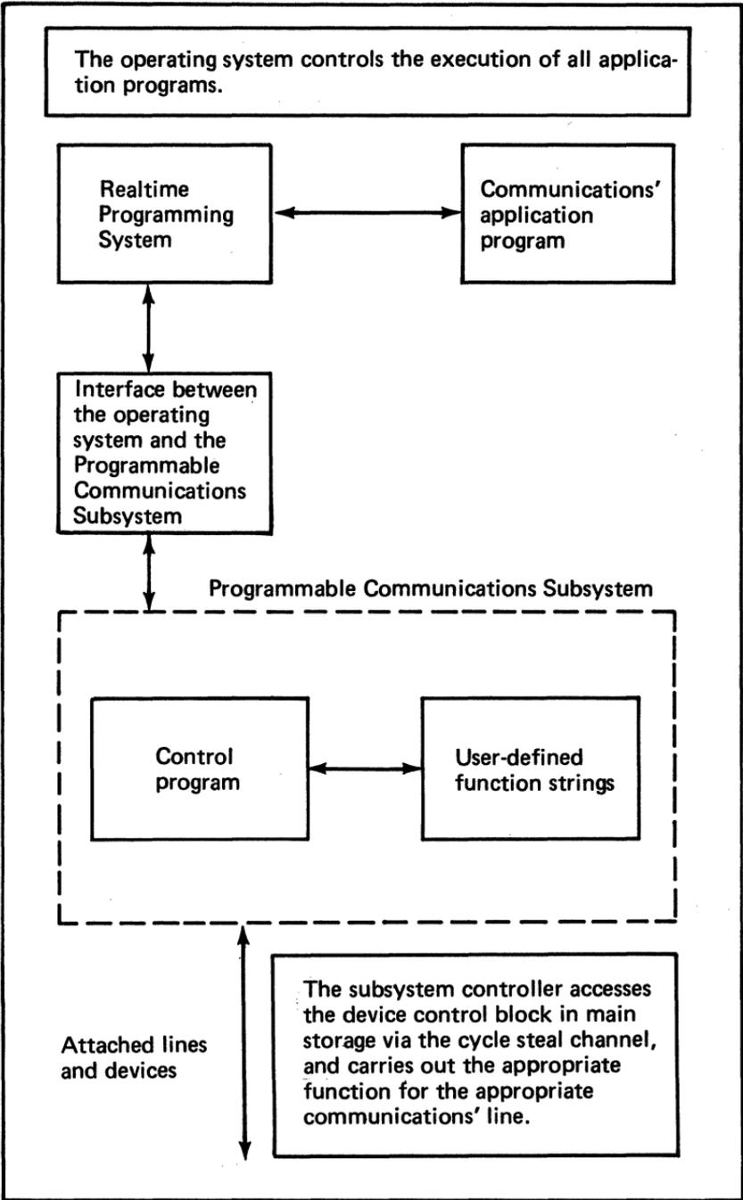
**Figure 131. Integrating software support of the Programmable Communications Subsystem into the Realtime Programming System operating system (1 of 2)**
