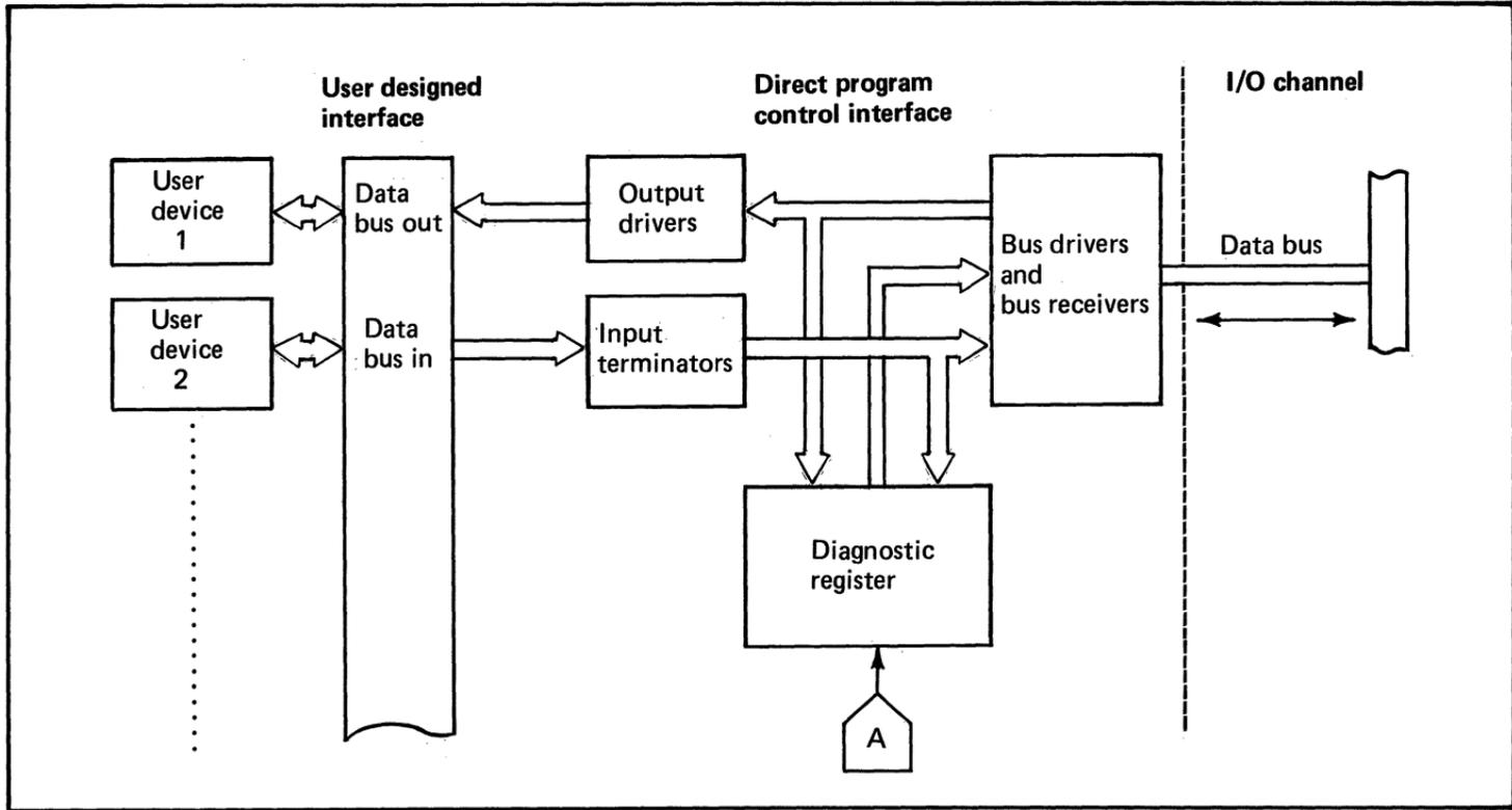
Figure 103. Block diagram of the OEM interface (1 of 3)
