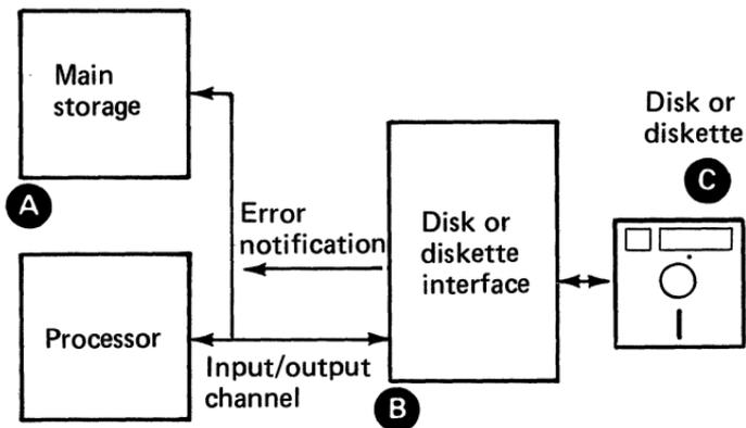
**B** Cyclic redundancy checks assist in the detection of errors due to bad data on the disk or noisy transmission.
