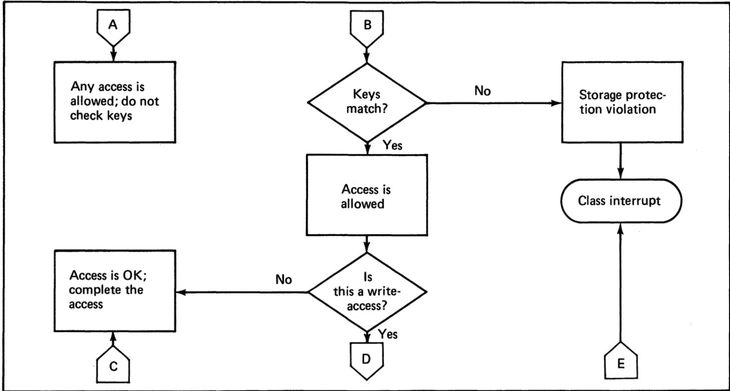
Figure 39. Operation of storage protection during an access (2 of 3)
