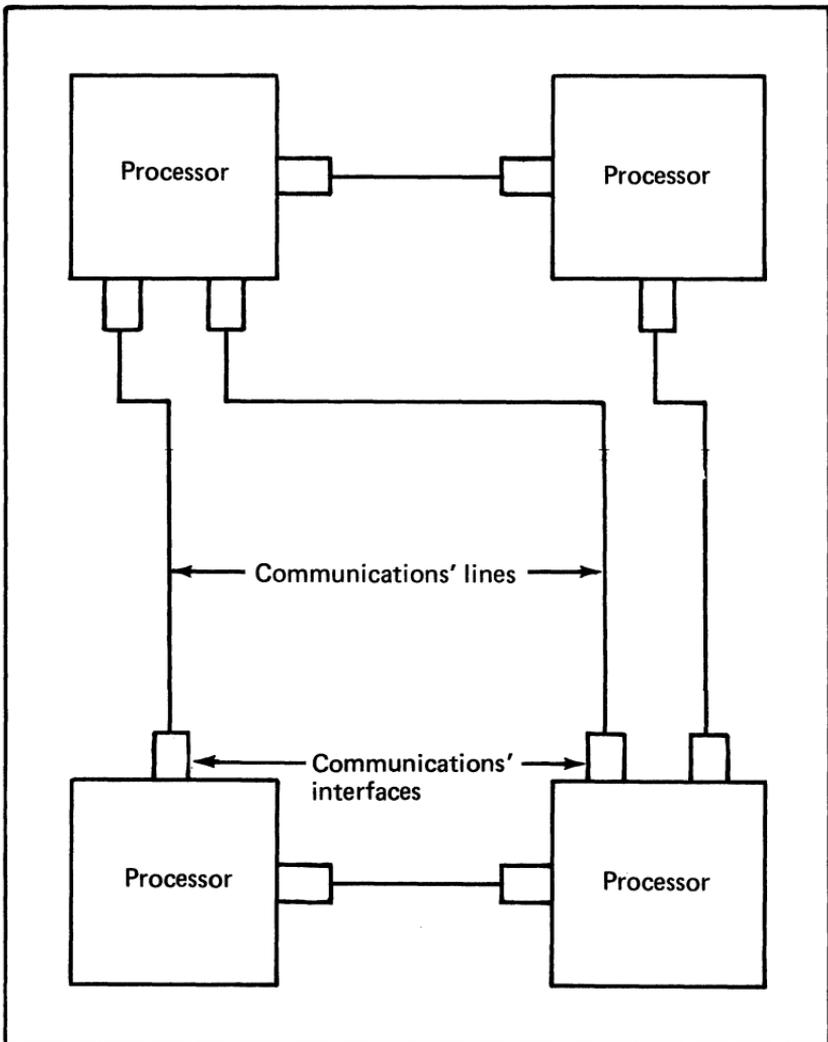
Each processor may act as a host-like processor, a concentrator, or a multifunction terminal. Data base and application processing may be arbitrarily distributed. Each processor must have communications' software to handle message routing from processor to processor in the network.
