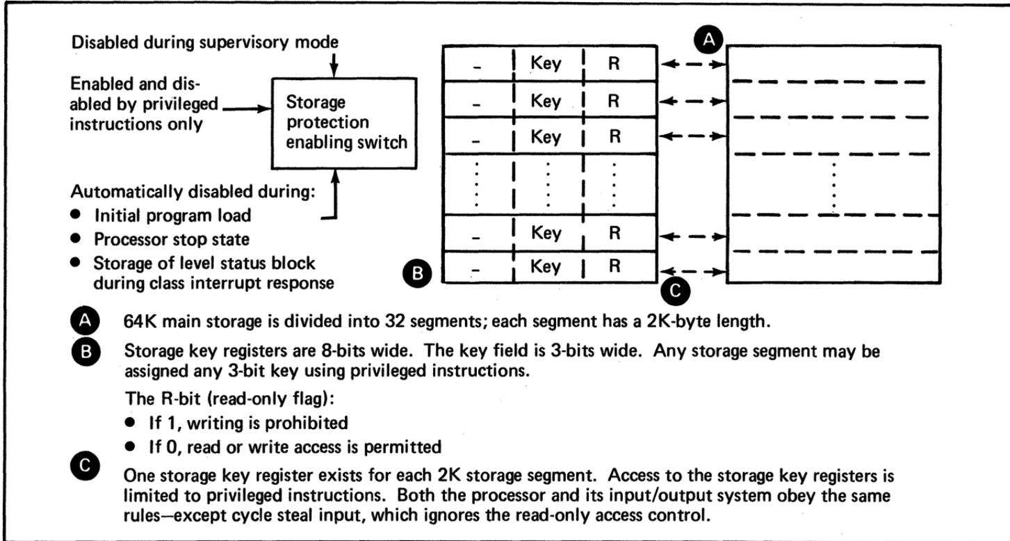
Figure 38. Storage key protection of main storage (1 of 2)
