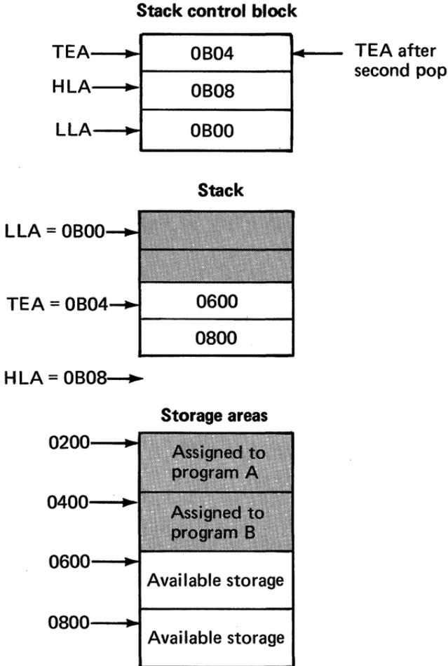
**Figure 28. Example of stack usage: allocation of storage areas to concurrent programs (3 of 4)**
