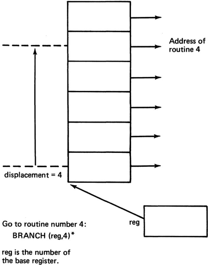
Figure 36. Combined base relative and indirect addressing mode solutions to programming problems (1 of 2)
