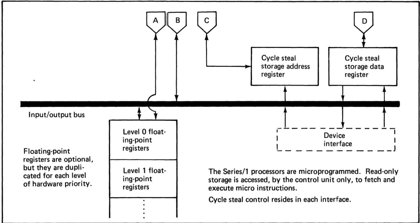
Figure 18. Overall data flow in the Series/1 processor (2 of 2)
