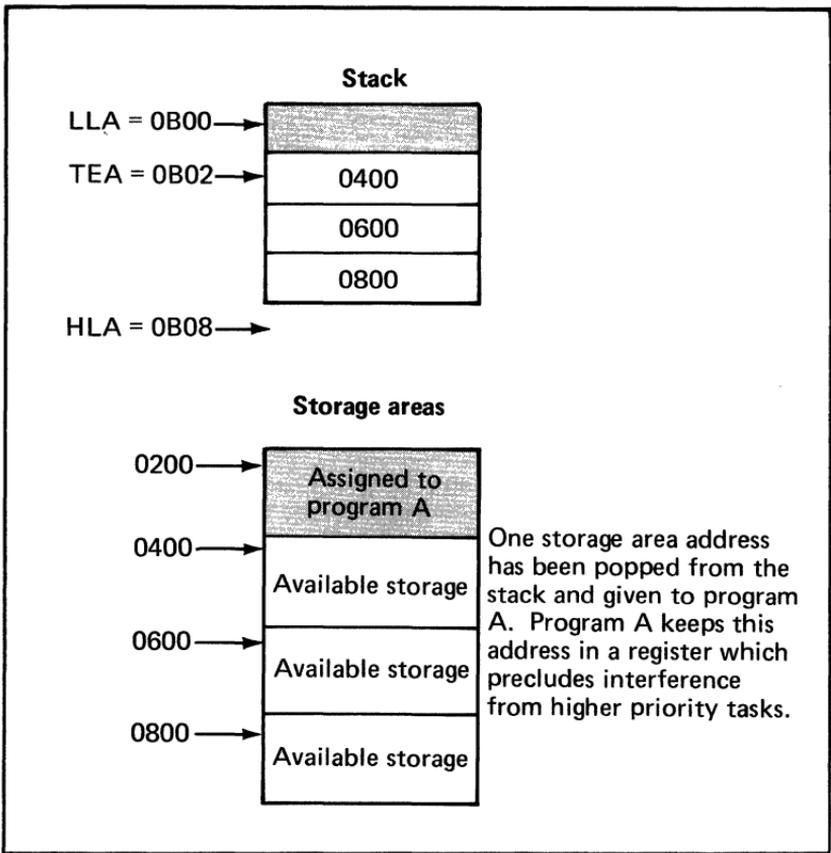
**Figure 28. Example of stack usage: allocation of storage areas to concurrent programs (2 of 4)**
