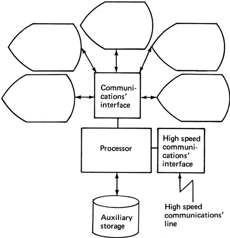
The concentrator consolidates input from a group of clustered terminals and transmits their combined data, at high speed, over a single line (or a few lines) to remote computers.
