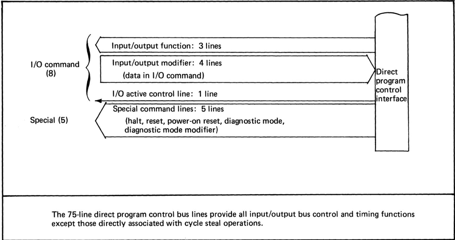
Figure 104. The direct program control interface bus (2 of 2)
