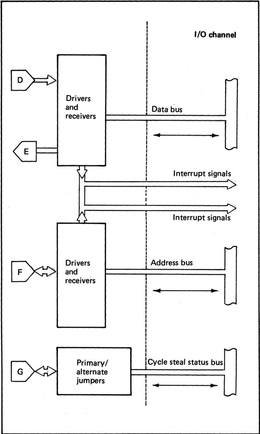
Figure 99. The teletypewriter interface block diagram (3 of 4)
