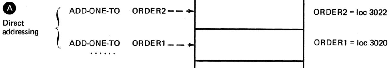
Figure 32. Storage addressing modes which do not use registers (1 of 3)
