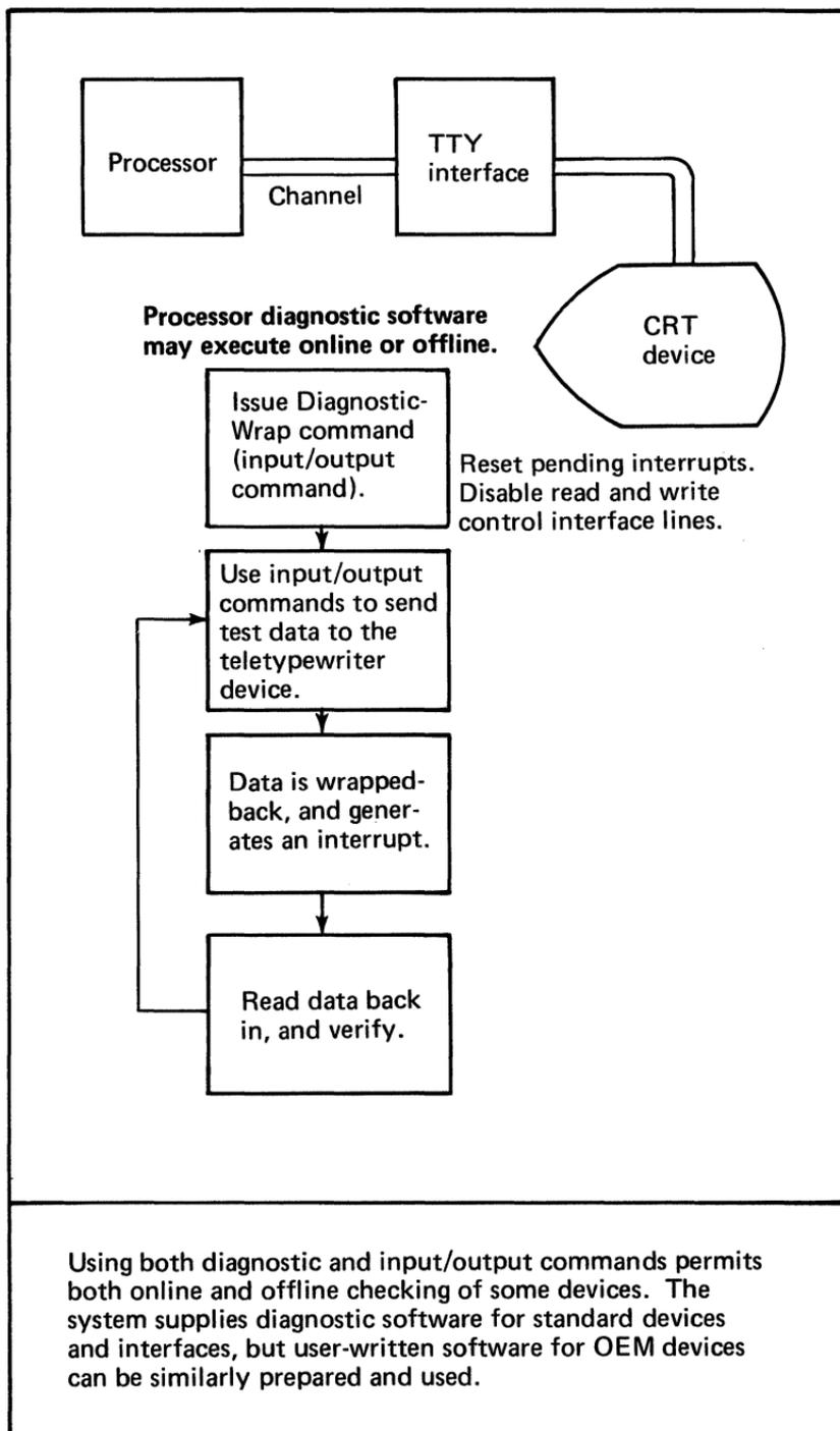
Figure 138. Teletypewriter interface design
