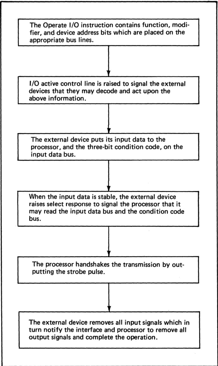
Figure 106. Data bus input sequence (1 of 2)
