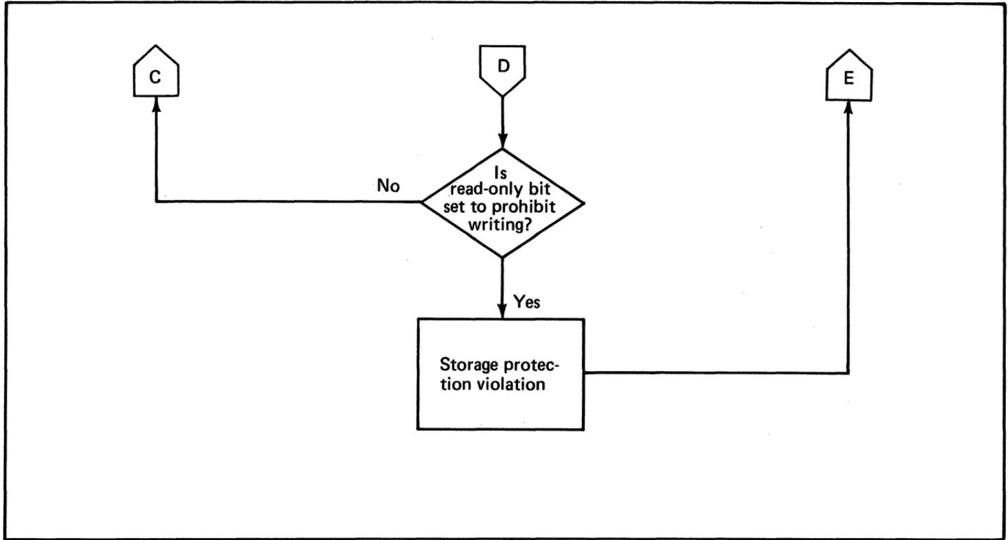
Figure 39. Operation of storage protection during an access (3 of 3)
