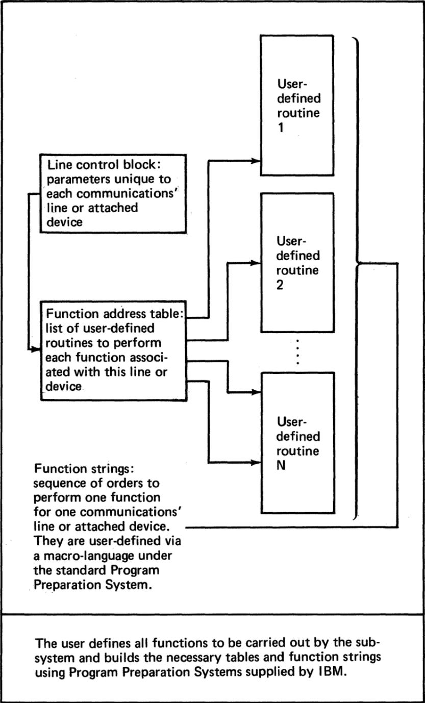
**Figure 130. Software organization within the Programmable Communications Subsystem (2 of 2)**
