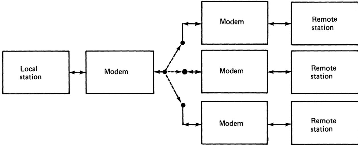
A point-to-point switched or dial-up connection of communicating stations. Only one secondary station is connected at any time. Both dial-up and responding to the dial-up with Series/1 communications' interfaces can be automatic.
