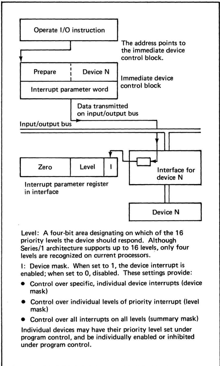
Figure 61. Individual devices under program control
