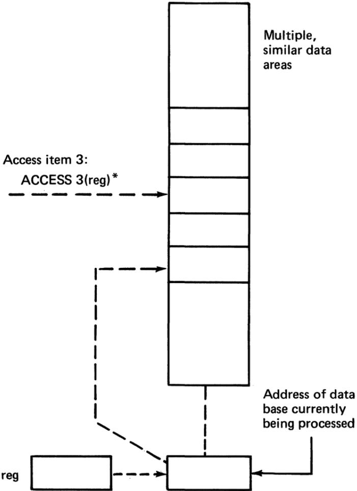
Figure 36. Combined base relative and indirect addressing mode solutions to programming problems (2 of 2)
