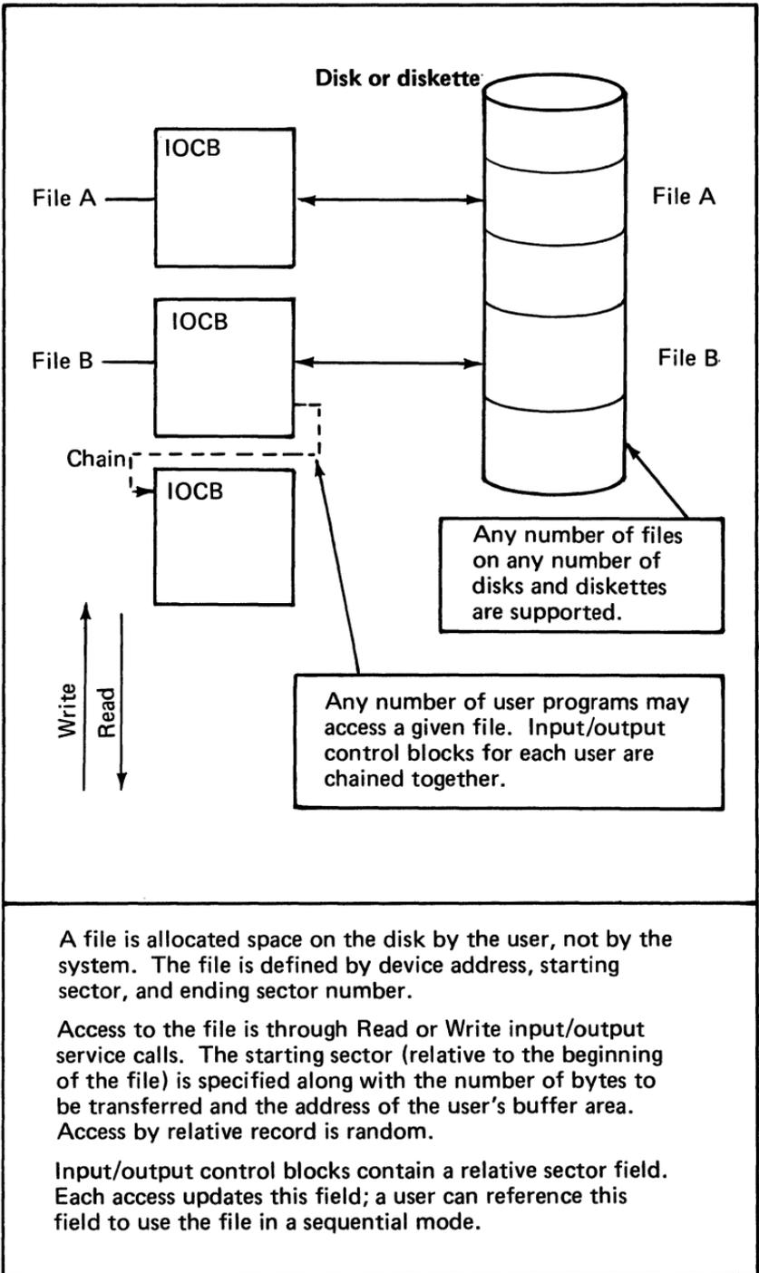
**Figure 73. Access to files using Control Program Support**
