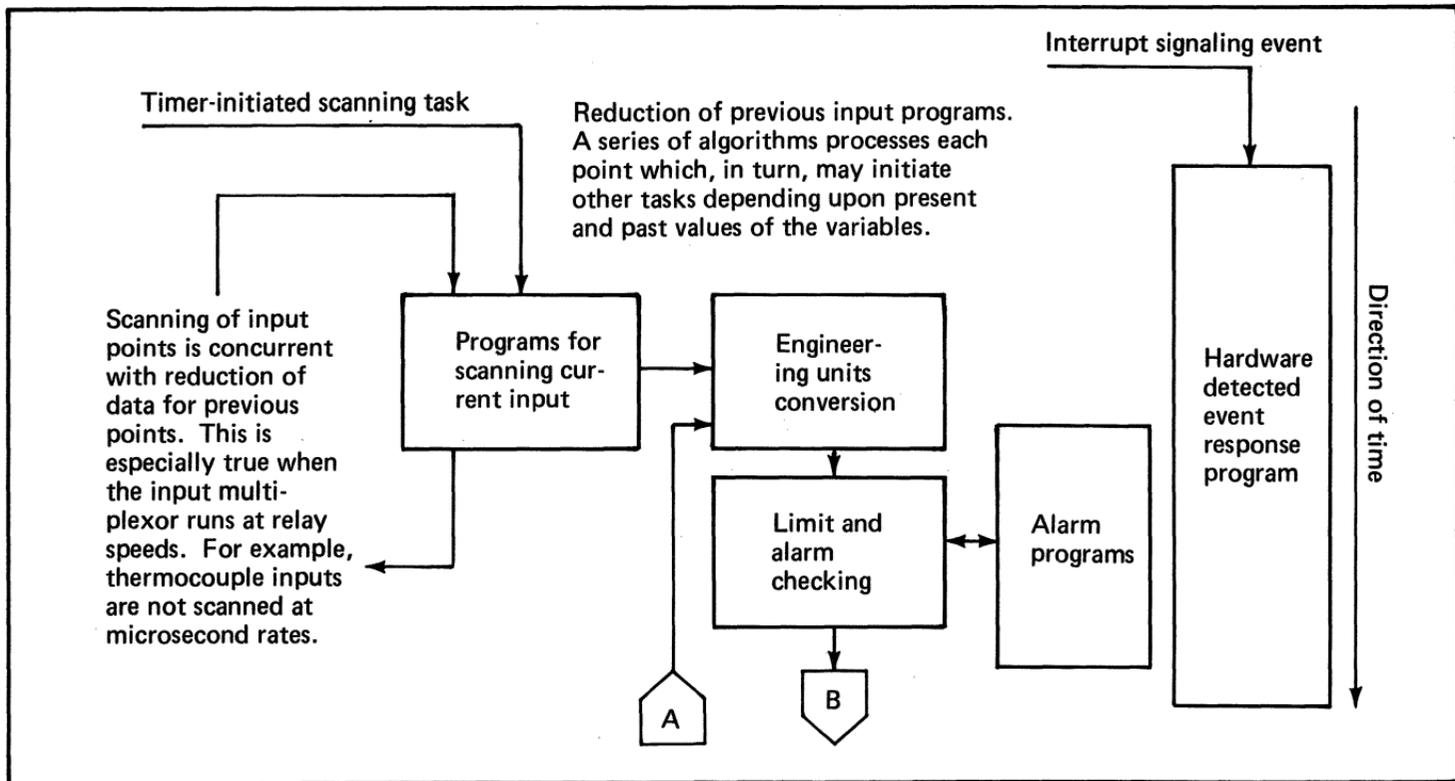
Figure 8. Set of concurrent tasks to carry out data acquisition and control (1 of 2)
