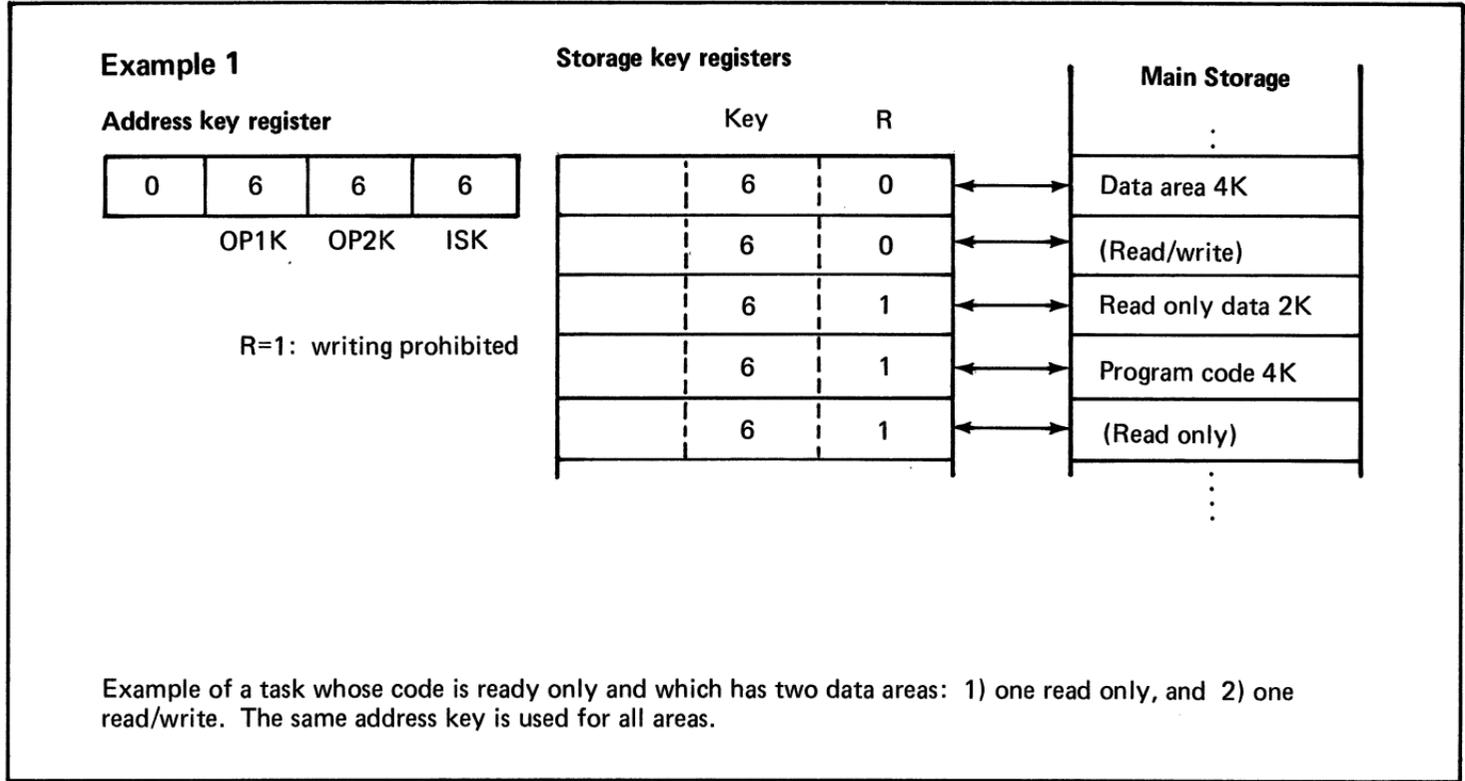
Figure 41. Three examples of address key storage protection (1 of 3)
