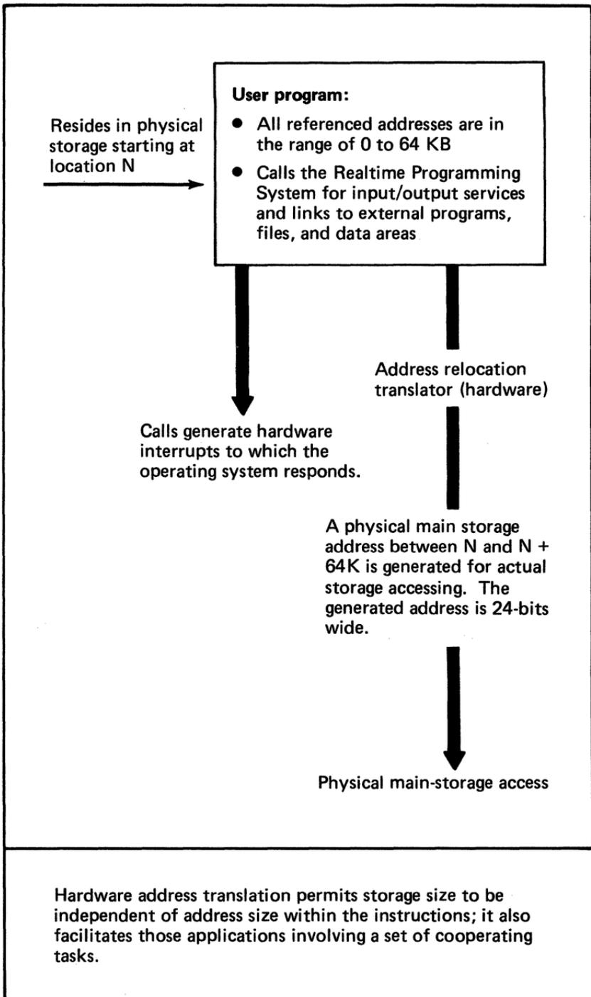
Figure 11. Address relocation for user programs
