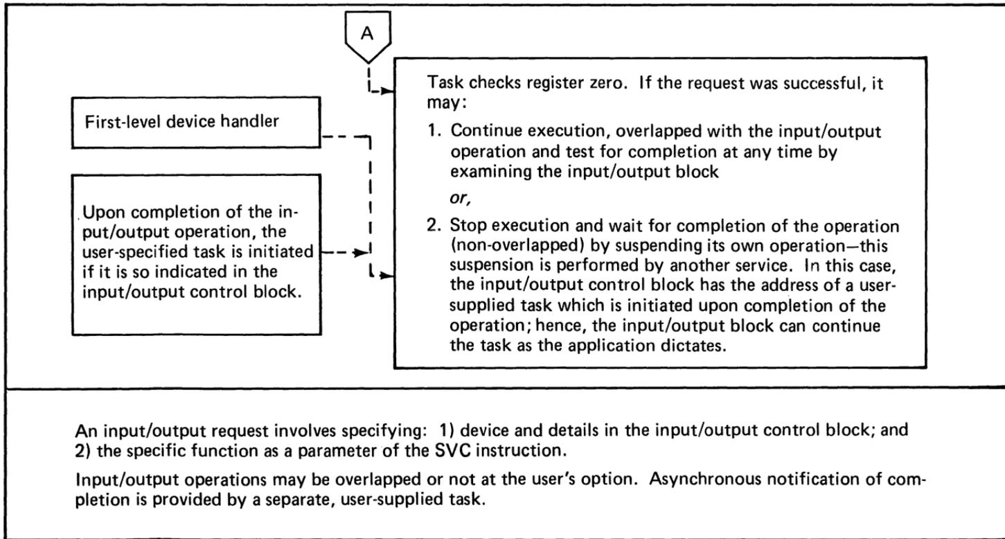
Figure 71. Overlapping and non-overlapping of input/output control (2 of 2)
