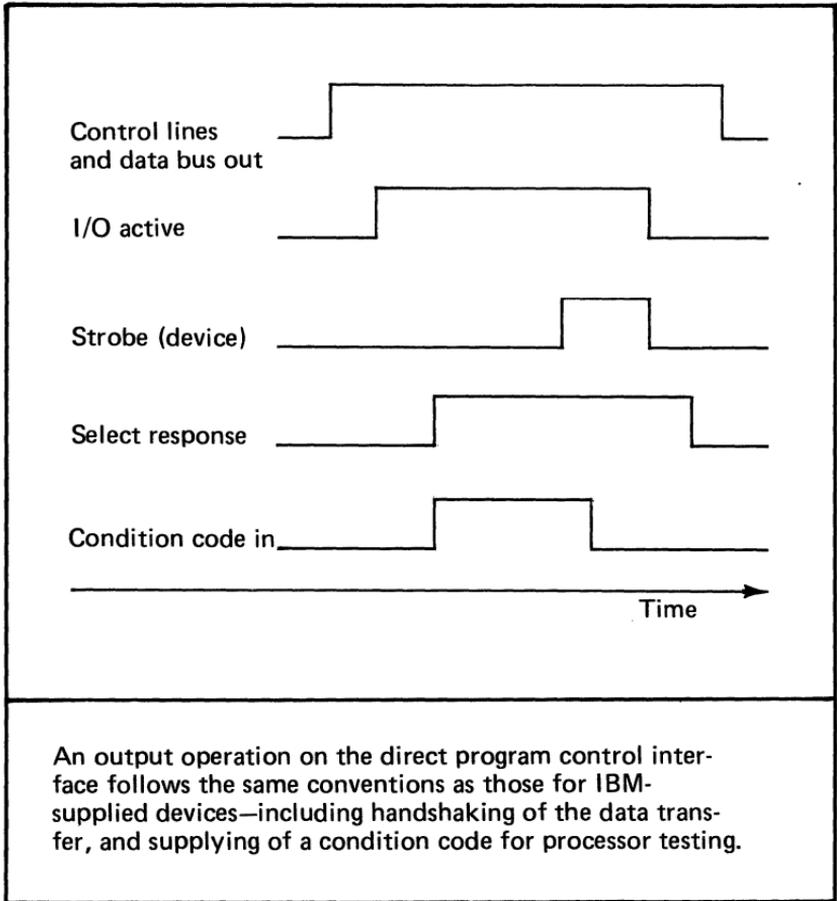
**Figure 105. Data bus output sequence (2 of 2)**
