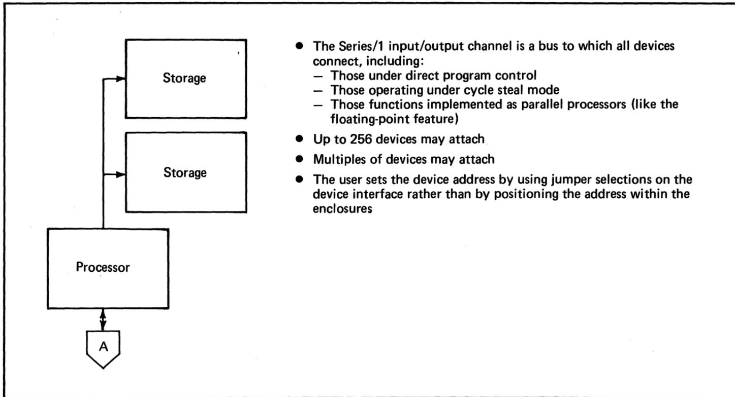
Figure 52. Input/output device combinations (1 of 4)
