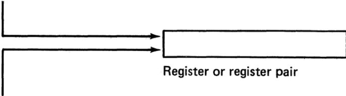
Replace vacated bits by original sign bit if shifting right *arithmetically*.
