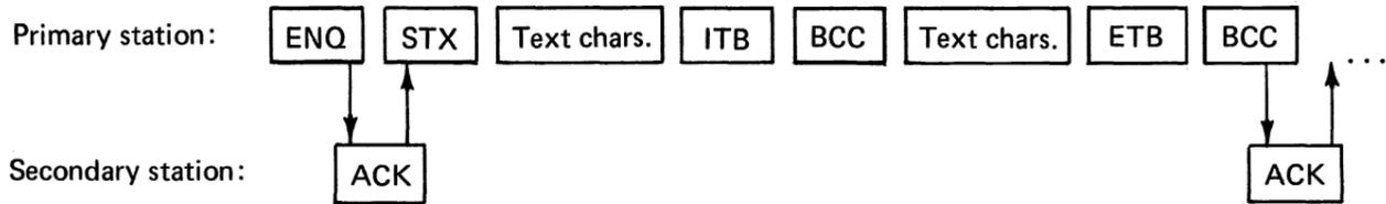
The ACK0 and ACK1 acknowledgement characters are used alternately to signal:
