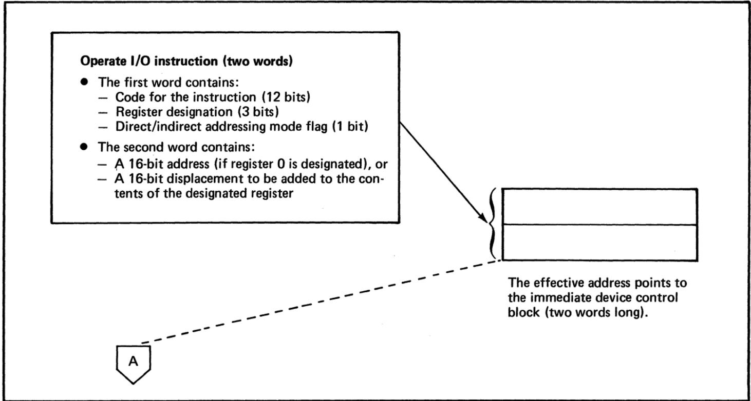
Figure 59. Direct program control performed with a single instruction—Operate I/O (1 of 3)
