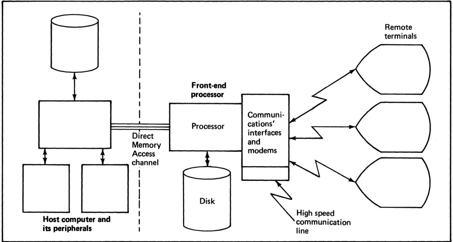
Figure 6. The front-end processor (1 of 2)
