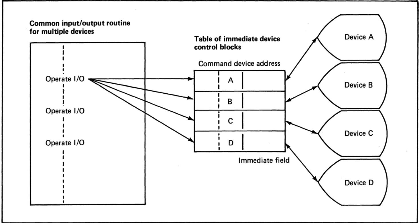
**Figure 64. A common input/output control routine addressing different immediate device control blocks (1 of 2)**
