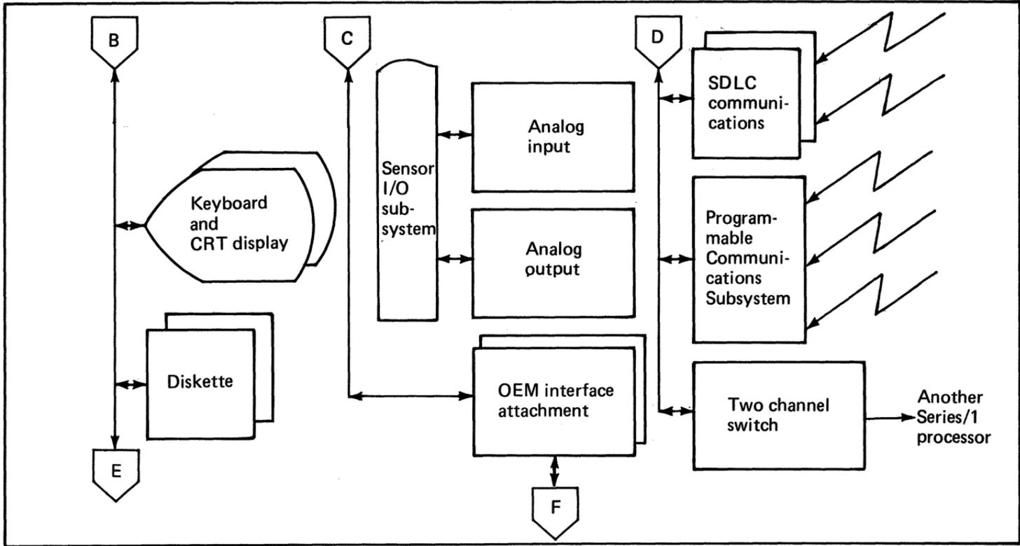
Figure 52. Input/output device combinations (3 of 4)
