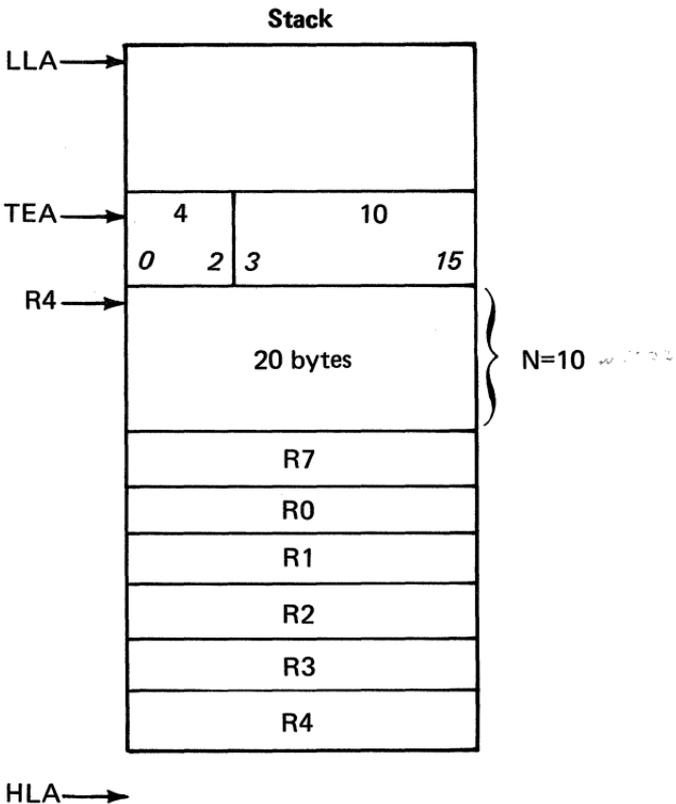
Figure 30. Example of stack usage: subroutine linkage and allocation of a work area (1 of 2)
