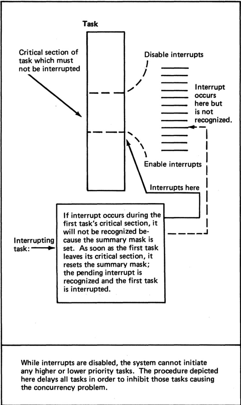
**Figure 87. Using disabling and enabling interrupts to control concurrency**
