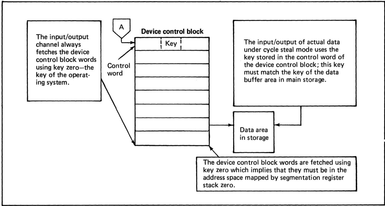
Figure 69. Input/output is consistent with storage protection of both mapped and unmapped processors (3 of 4)
