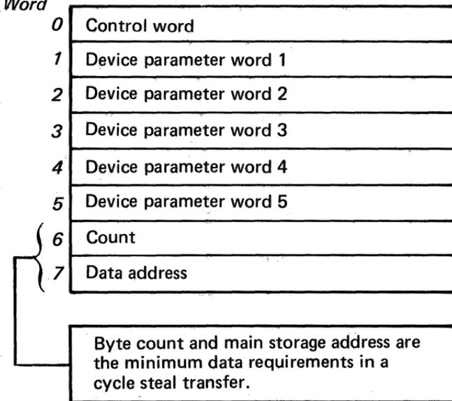
Device control block words are accessed by the device interface. Only those words needed for a specific device are actually transferred to the device interface.
