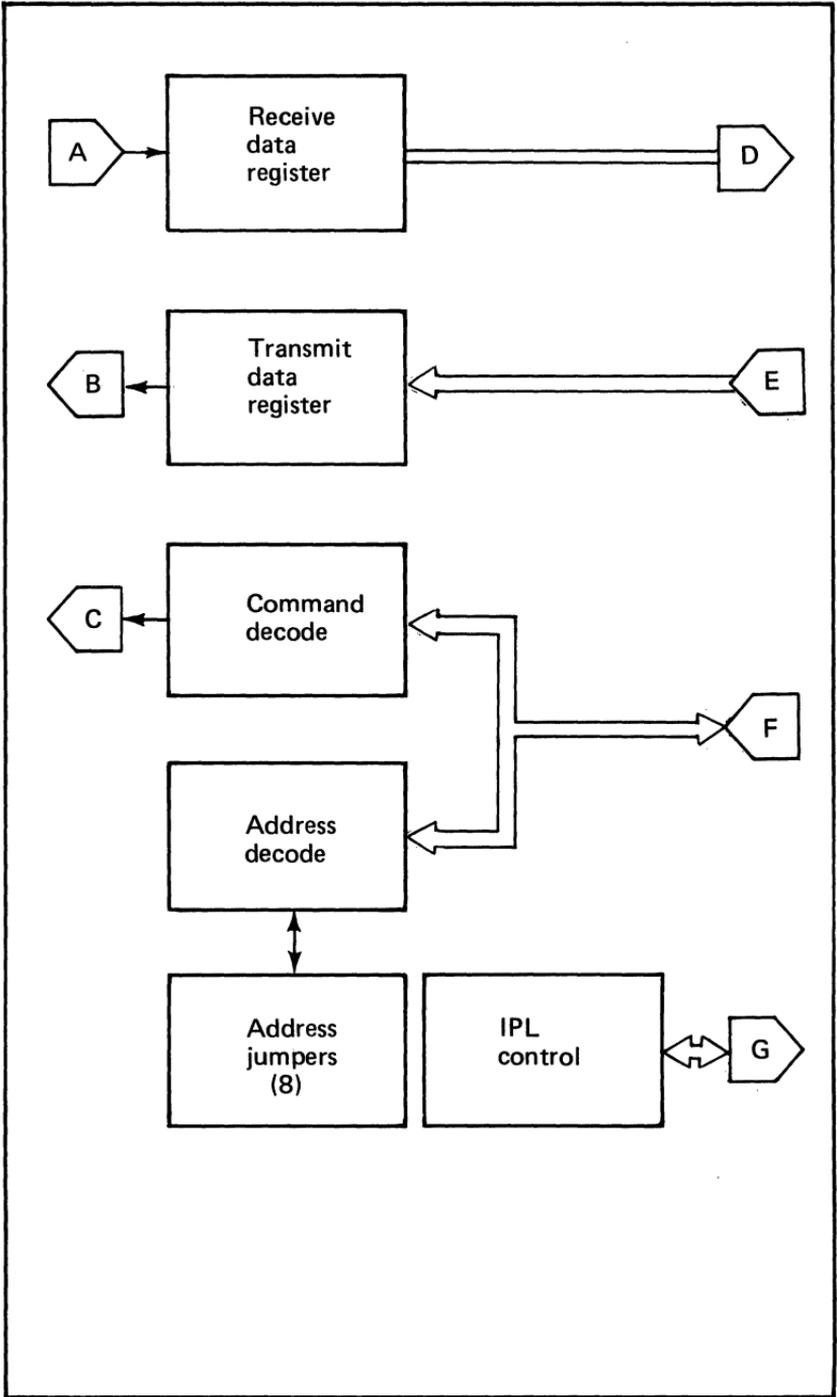
Figure 99. The teletypewriter interface block diagram (2 of 4)
