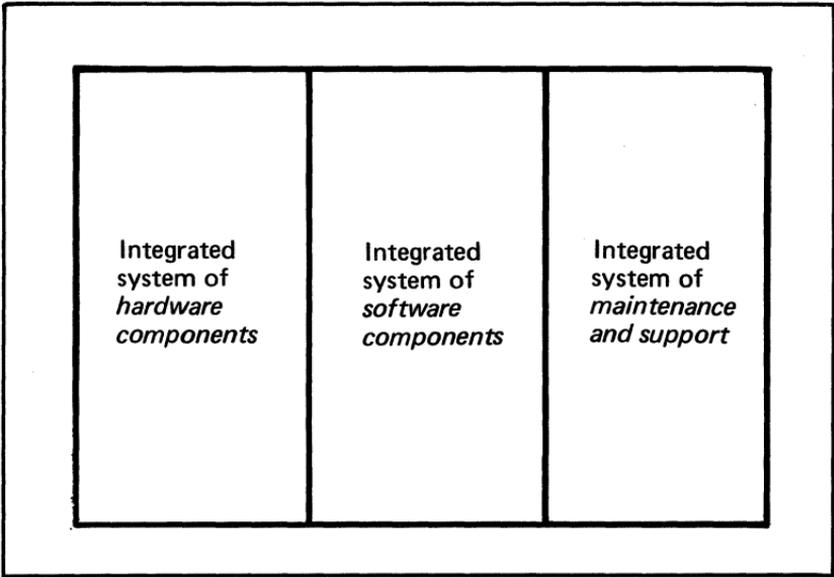
**Figure 1. Essential ingredients of a small computer system**
