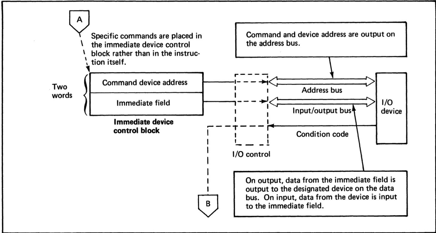
Figure 59. Direct program control performed with a single instruction—Operate I/O (2 of 3)
