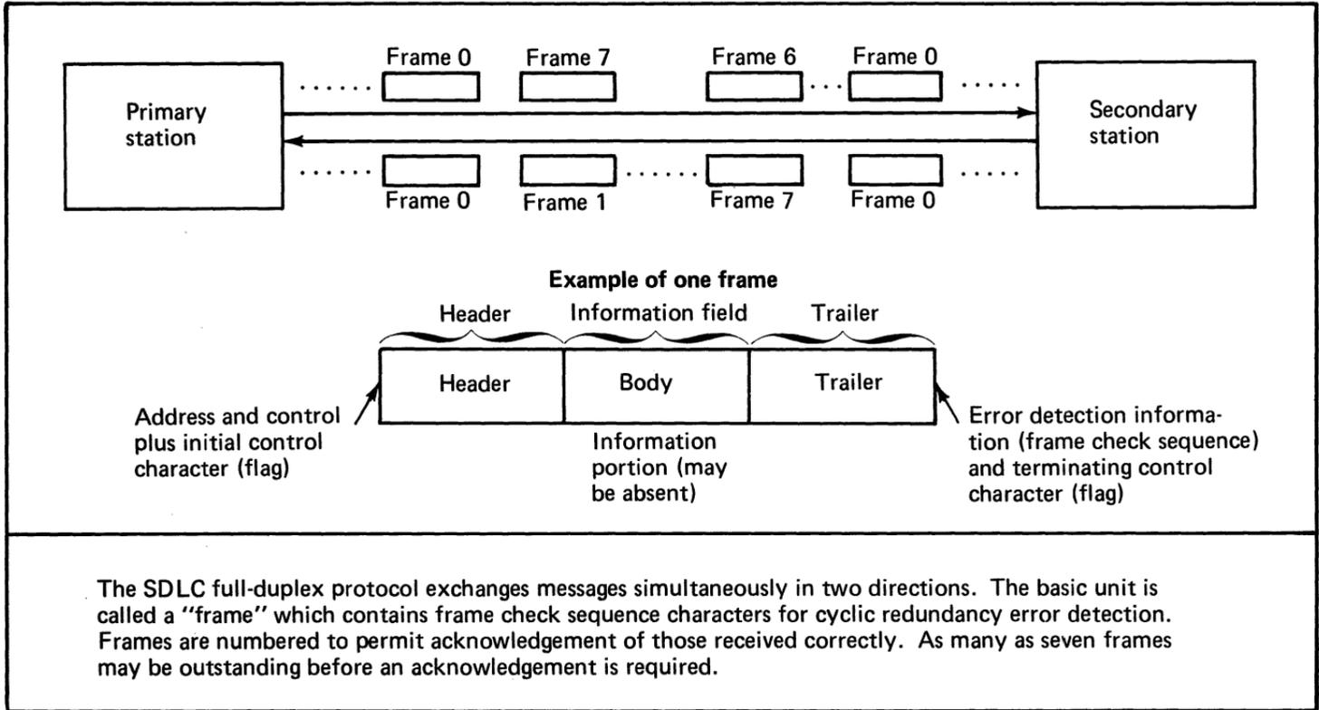
Figure 123. Basic concept of SDLC
