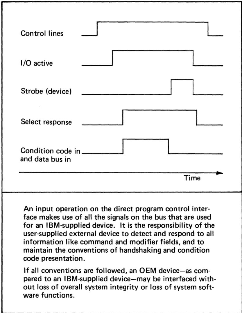
Figure 106. Data bus input sequence (2 of 2)
