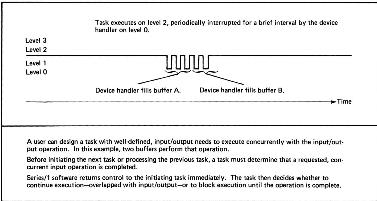
Figure 58. Direct program control and overlapped input/output (2 of 2)
