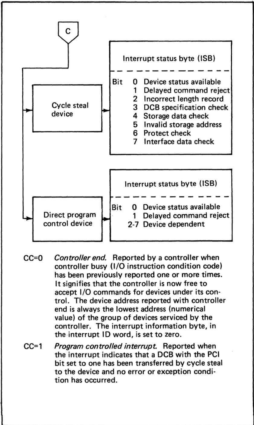
**CC=0** *Controller end.* Reported by a controller when controller busy (I/O instruction condition code) has been previously reported one or more times. It signifies that the controller is now free to accept I/O commands for devices under its control. The device address reported with controller end is always the lowest address (numerical value) of the group of devices serviced by the controller. The interrupt information byte, in the interrupt ID word, is set to zero.
