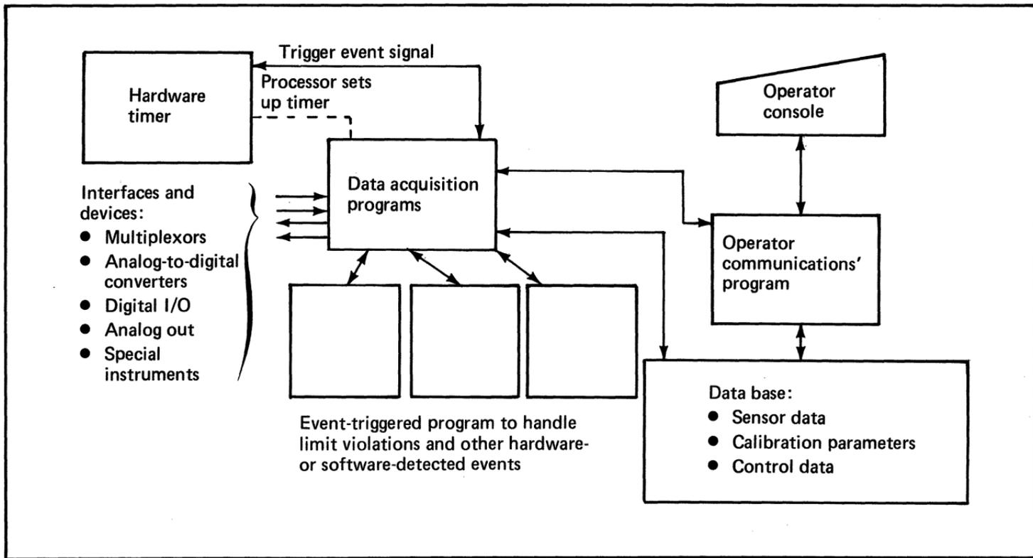
Figure 7. The data acquisition and control application (1 of 2)
