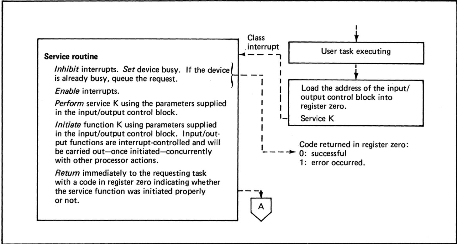
Figure 71. Overlapping and non-overlapping of input/output control (1 of 2)
