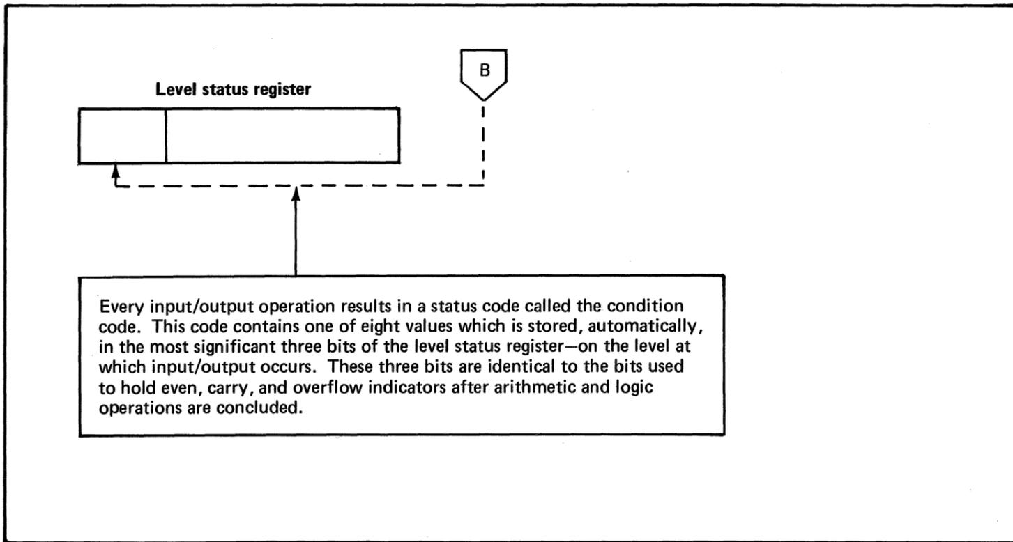
Figure 59. Direct program control performed with a single instruction—Operate I/O (3 of 3)
