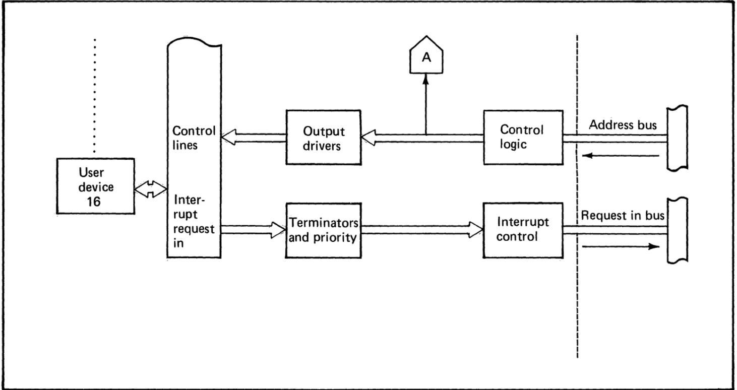
Figure 103. Block diagram of the OEM interface (2 of 3)
