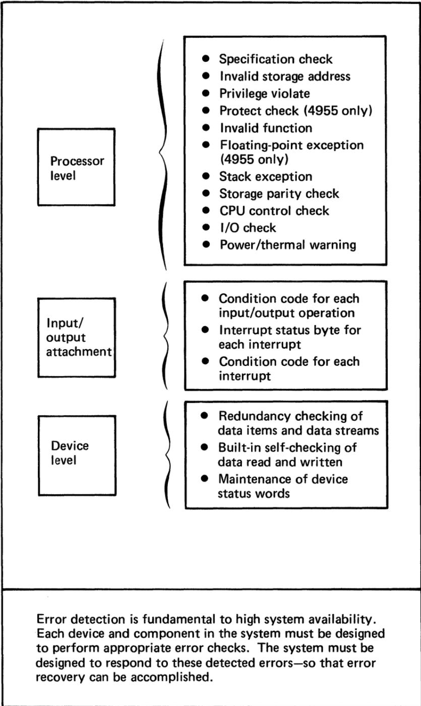
**Figure 133. Elements of error detection**
