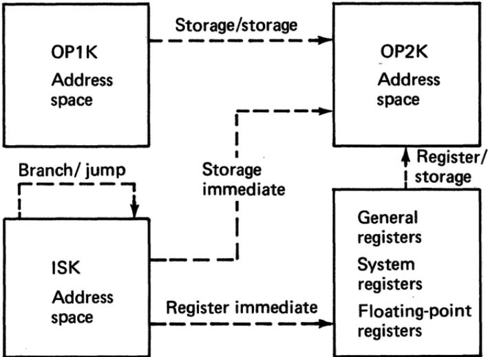
Each of the three address keys controls one type of storage access:
