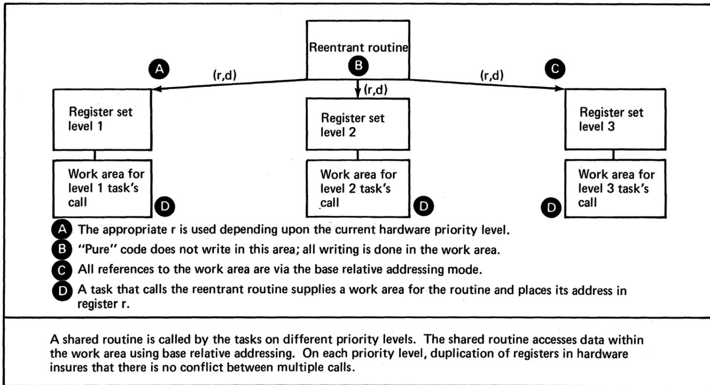
Figure 47. Addressing modes facilitate reentrant routines' use of multiple work areas
