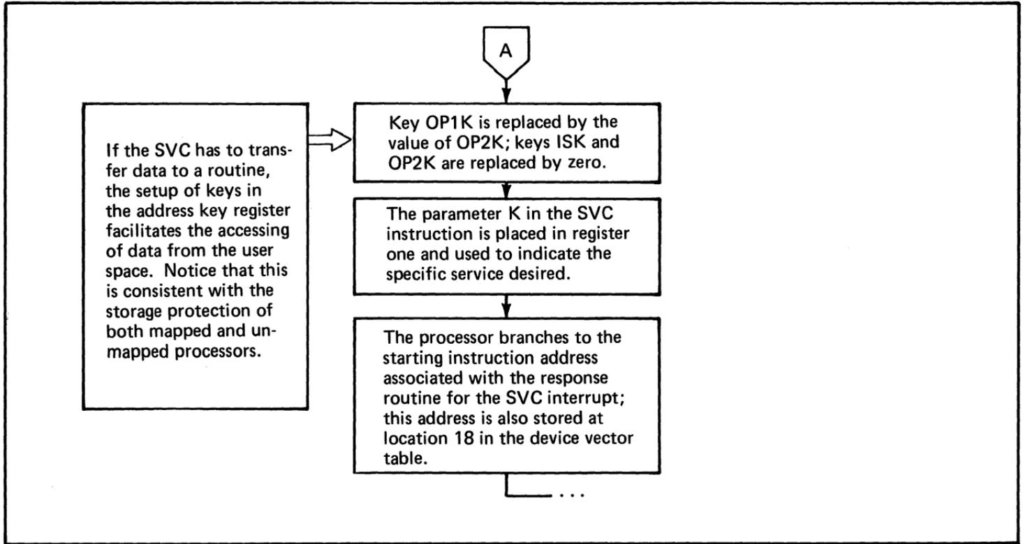
Figure 70. Communications between a task and the operating system using the Supervisor Call (SVC) convention (2 of 3)
