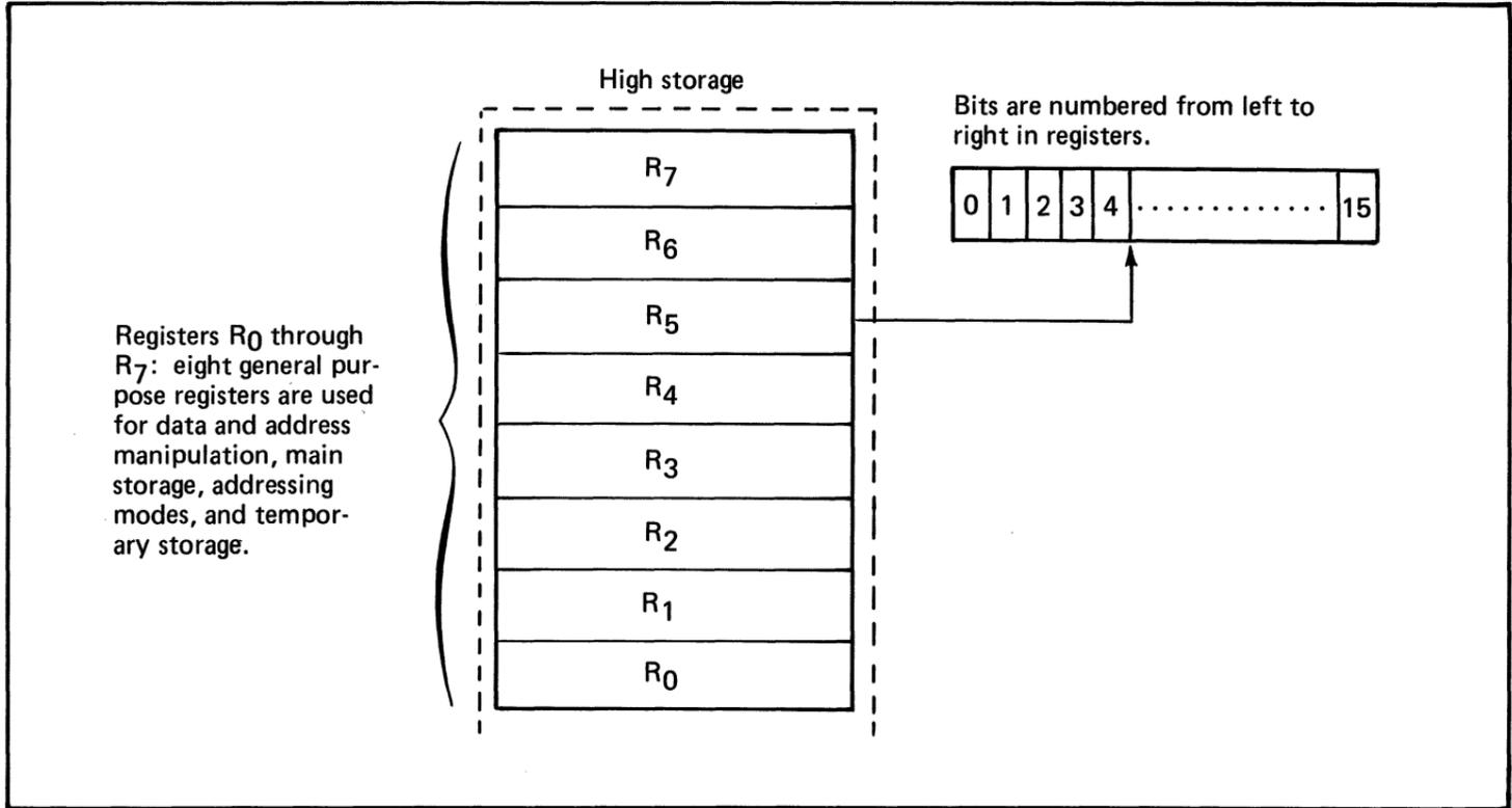
Figure 19. The level status block (1 of 2)
