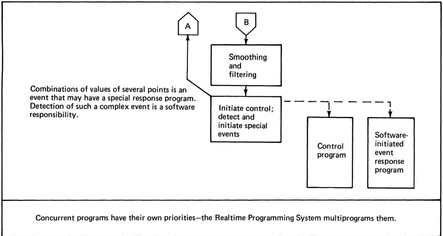
Figure 8. Set of concurrent tasks to carry out data acquisition and control (2 of 2)
