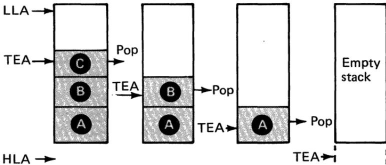
The Series/1 provides instructions for adding and deleting one-, two-, and four-byte size elements.
