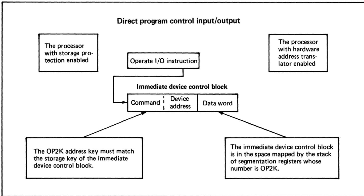
Figure 69. Input/output is consistent with storage protection of both mapped and unmapped processors (1 of 4)
