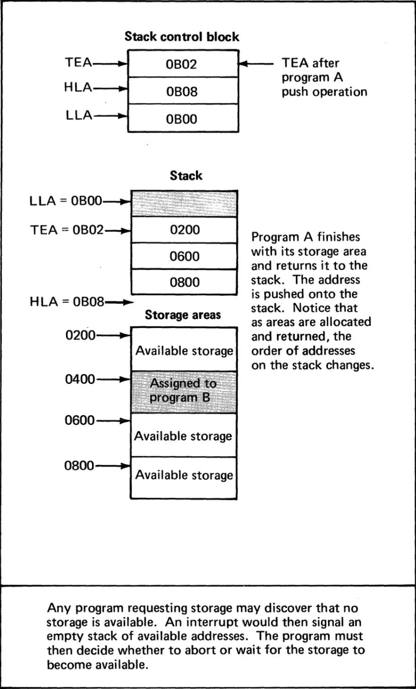
**Figure 28. Example of stack usage: allocation of storage areas to concurrent programs (4 of 4)**
