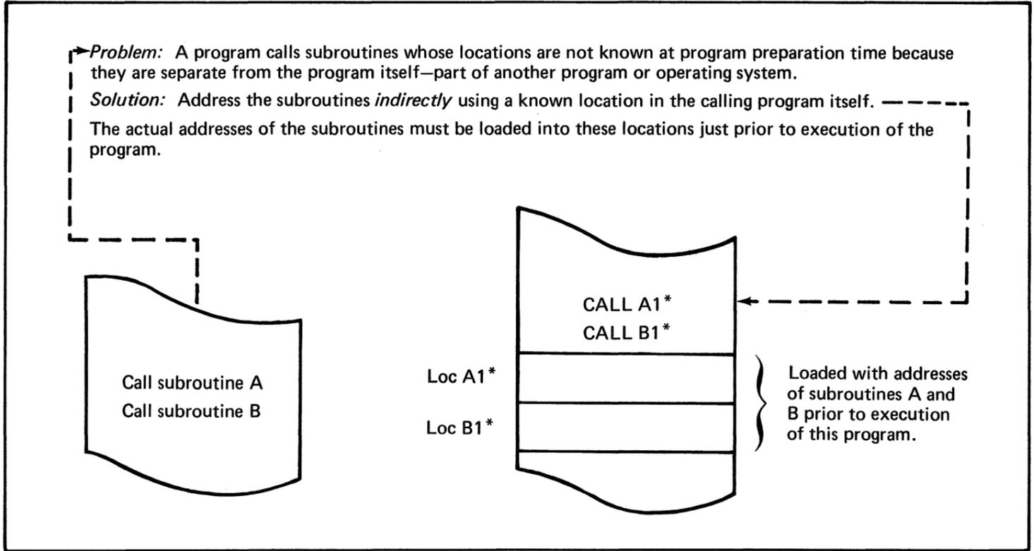
Figure 32. Storage addressing modes which do not use registers (3 of 3)
