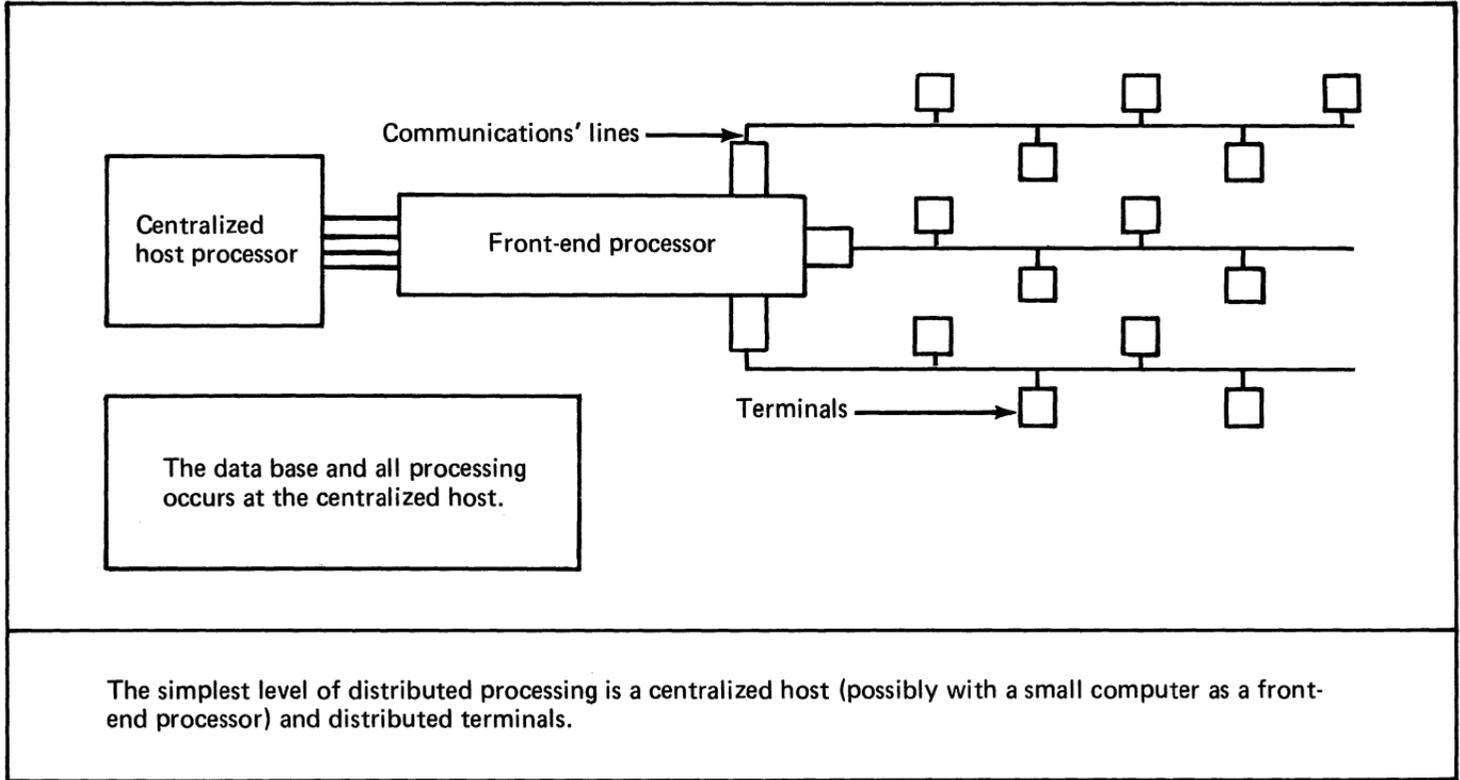
Figure 111. Centralized processing
