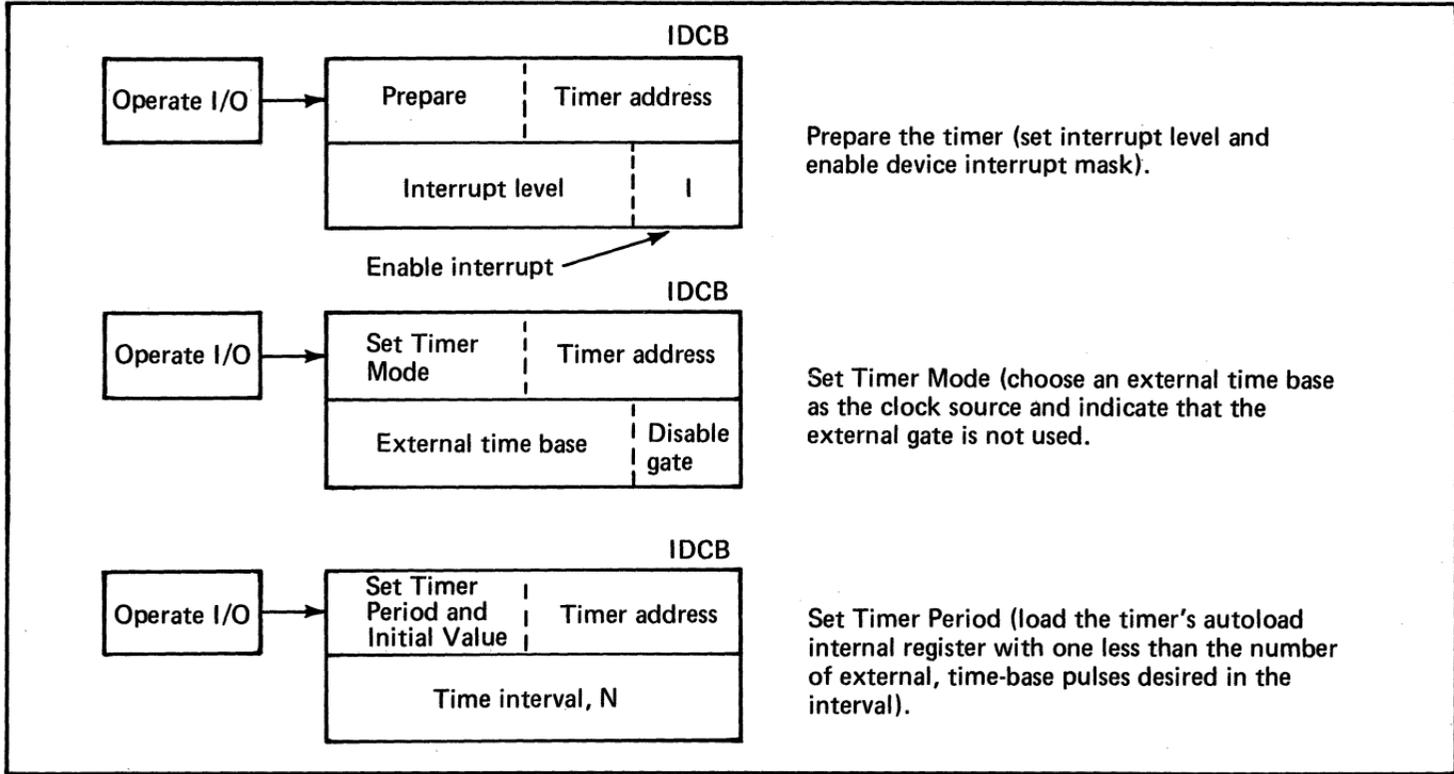
Figure 95. Using the timer to provide interval timing to the processor (2 of 3)
