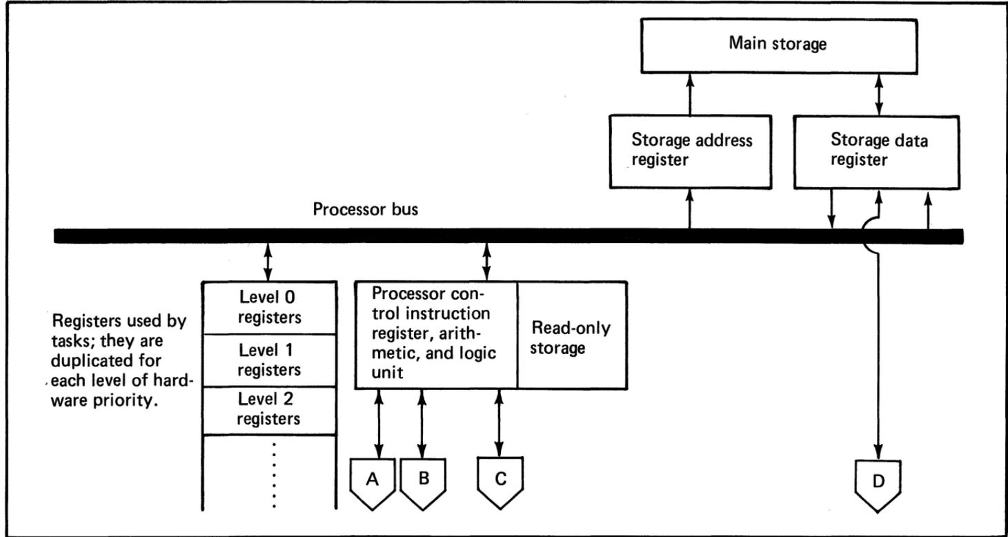
Figure 18. Overall data flow in the Series/1 processor (1 of 2)
