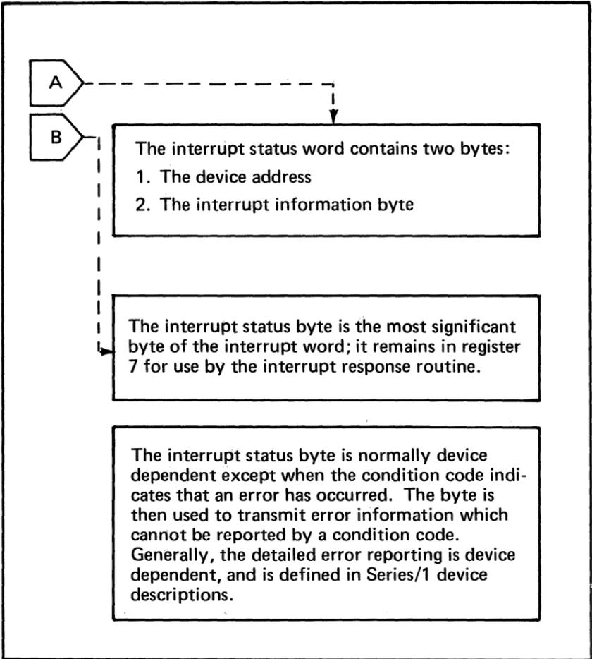
**Figure 63. Condition codes accompanying each input/output interrupt (2 of 5)**
