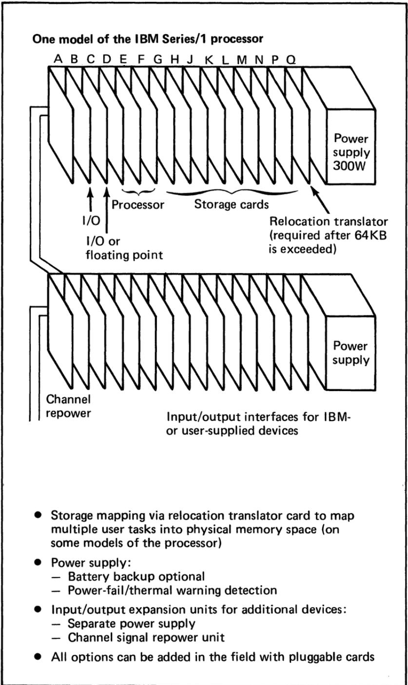
**Figure 10. Features of the IBM Series/1 processor family (2 of 2)**
