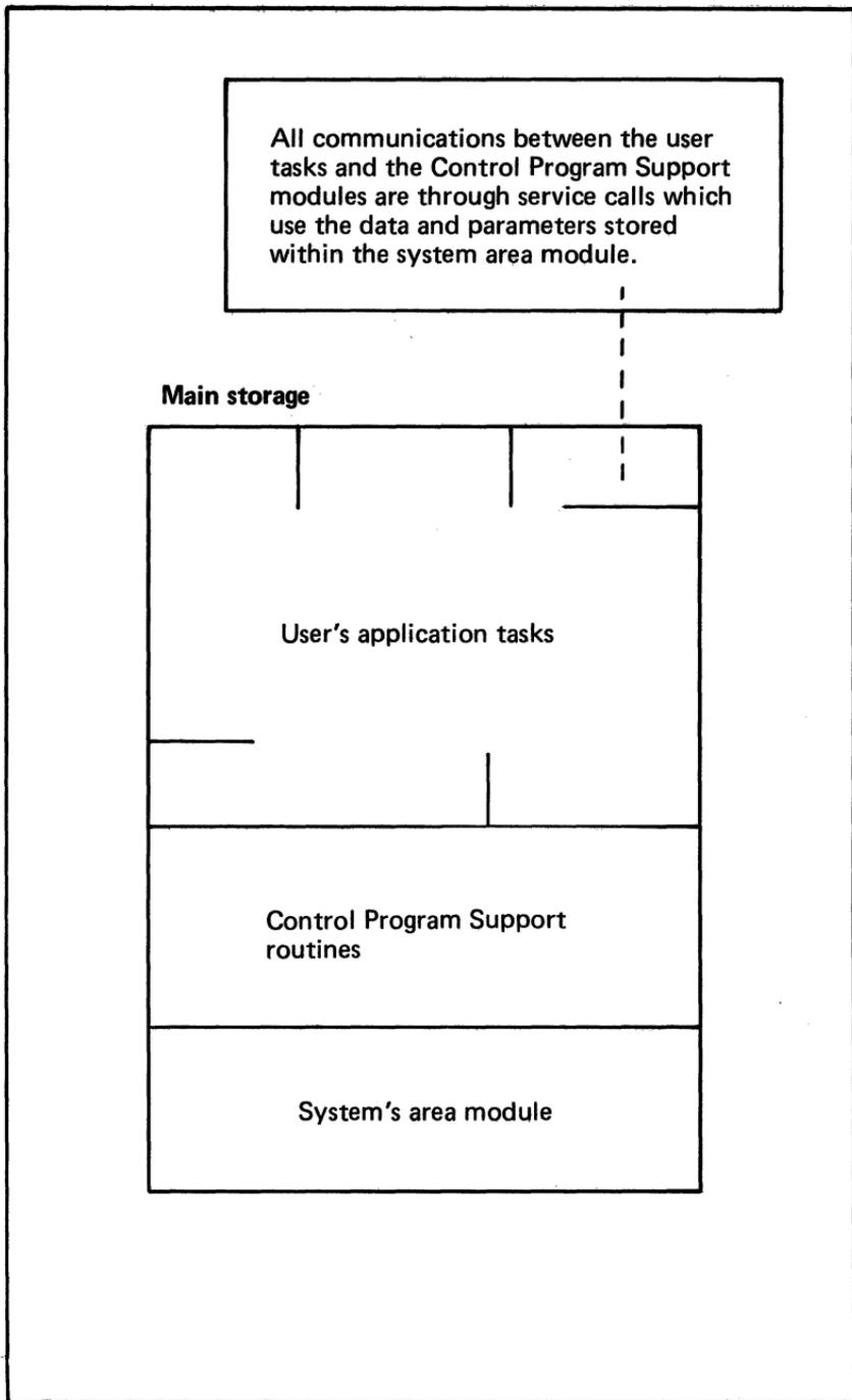
**Figure 74. Organization of main storage for a dedicated application utilizing the Control Program Support package (1 of 2)**
