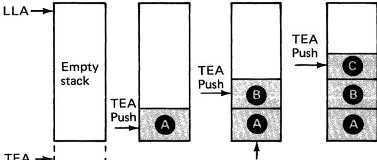
Notice that the addition of elements is from the higher addresses toward the lower addresses in main storage.
