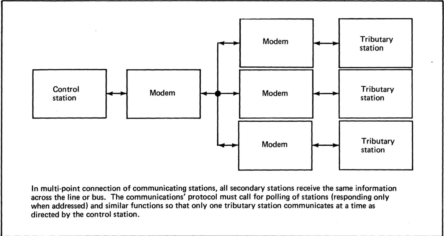
Figure 115. The structure of communications' support (3 of 3)
