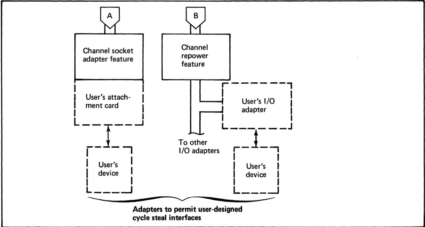
Figure 93. Options for user attachments to the Series/1 (2 of 2)
