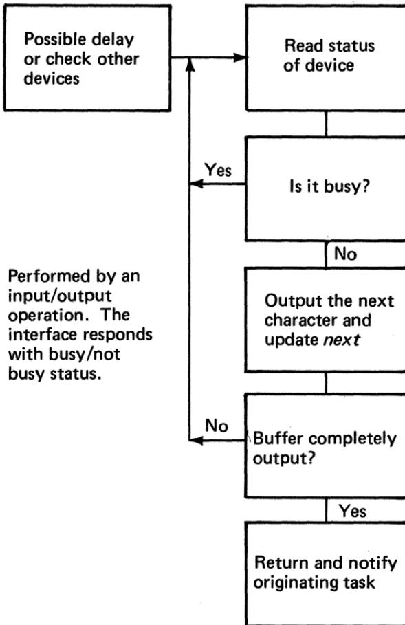
Because of the difference between the processor and the device speeds, this form of polling ties up the processor completely doing what is, essentially, a small task. By comparison, interrupt-driven input/output of this type operates with a very economical overhead.
