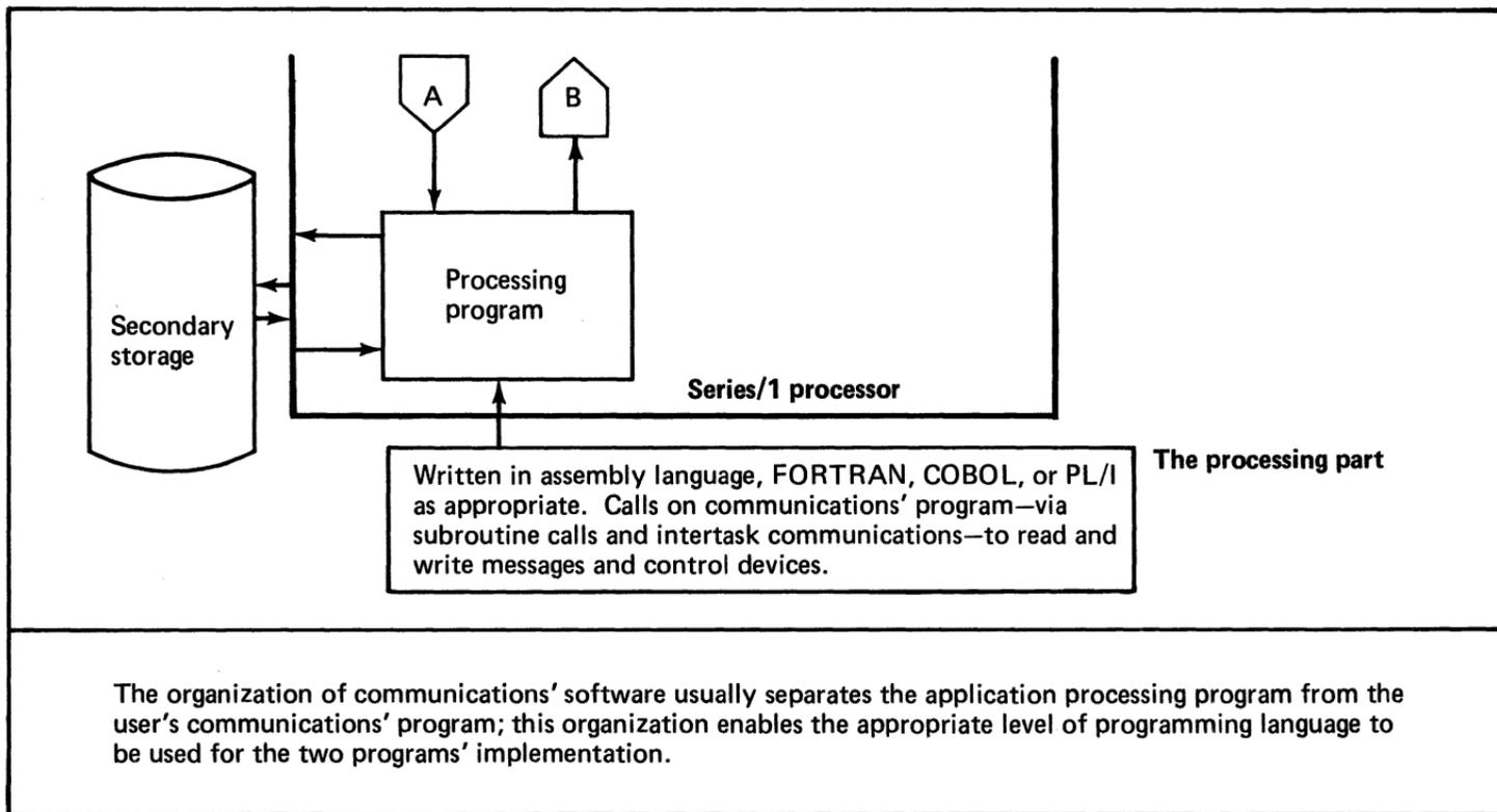
Figure 127. Software use of communications (2 of 2)
