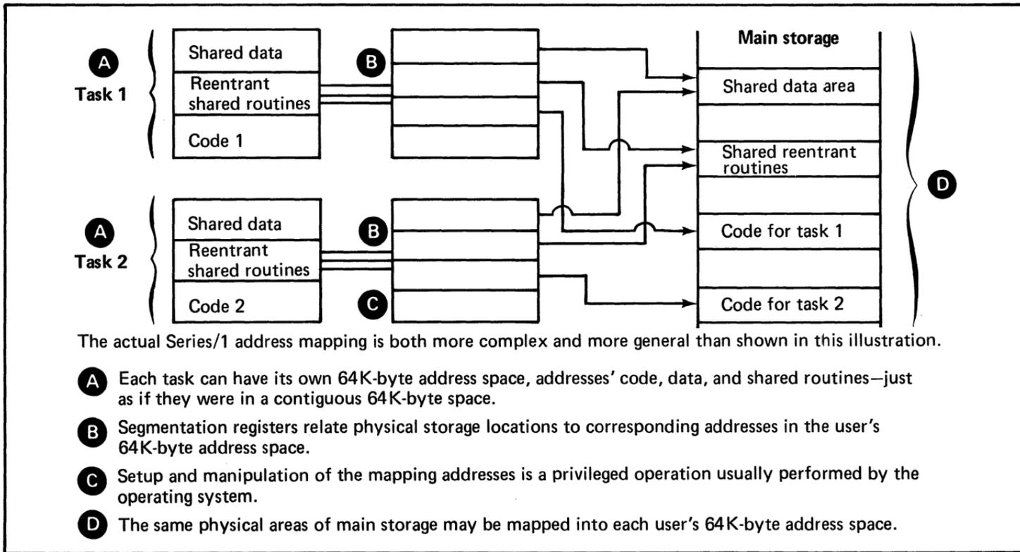
Figure 43. Conceptual mapping of main storage for two tasks sharing common data and subroutine areas
