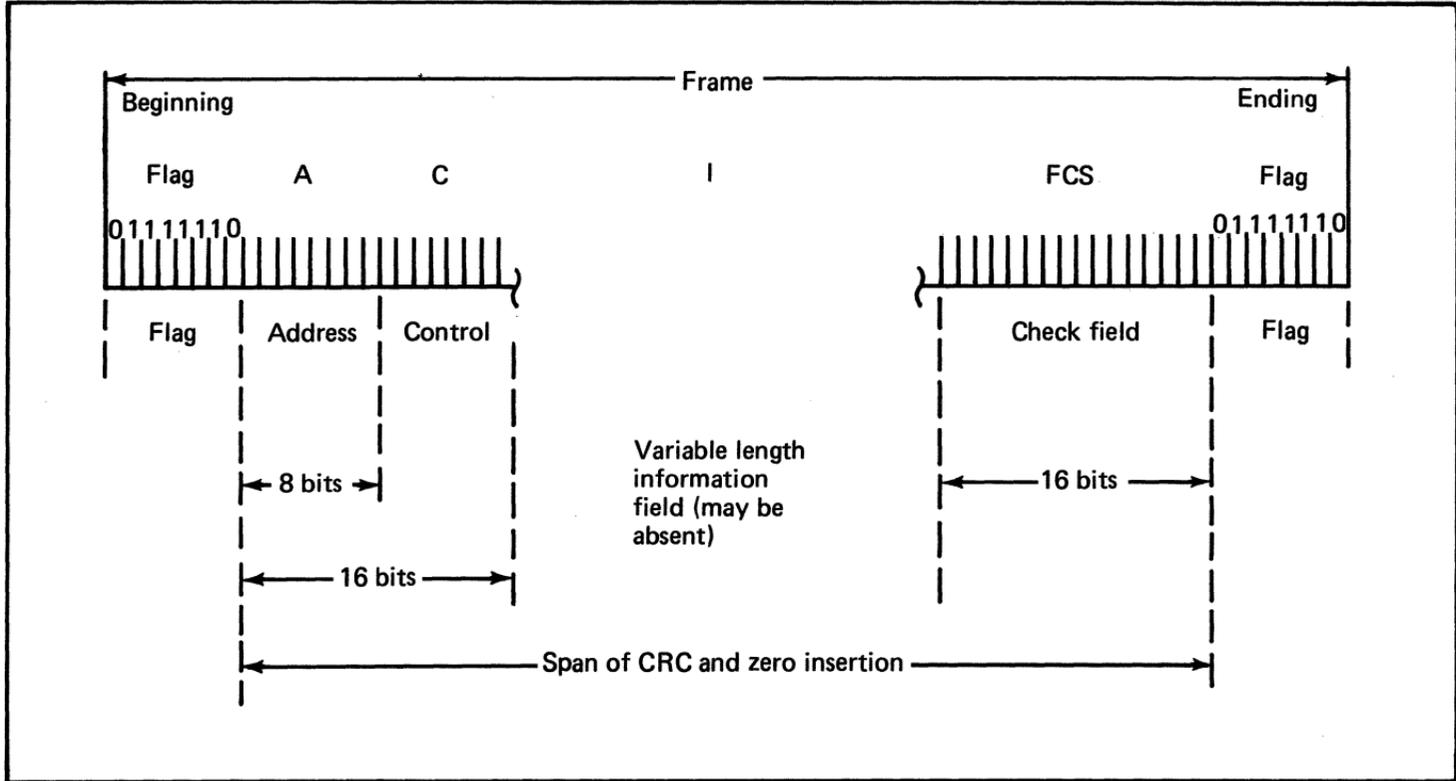
Figure 124. Detailed definition of the SDLC frame format (1 of 2)
