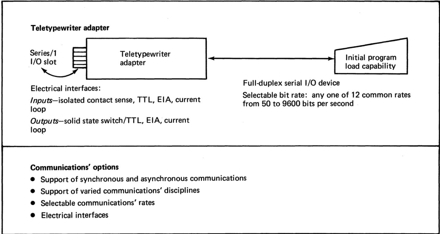
Figure 17. A subsystem can be flexibly configured to interface with a combination of analog and digital, input and output devices (1 of 4)
