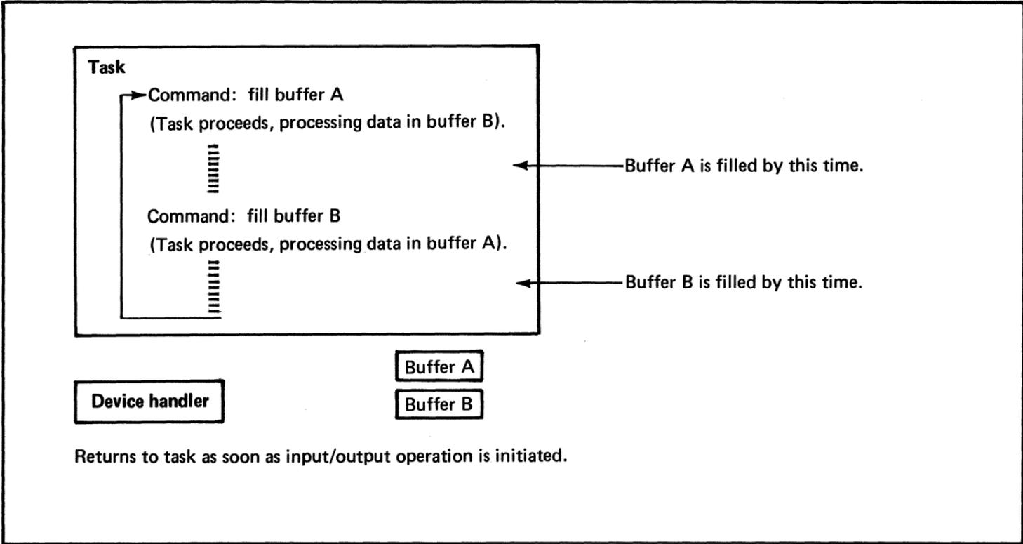
Figure 58. Direct program control and overlapped input/output (1 of 2)
