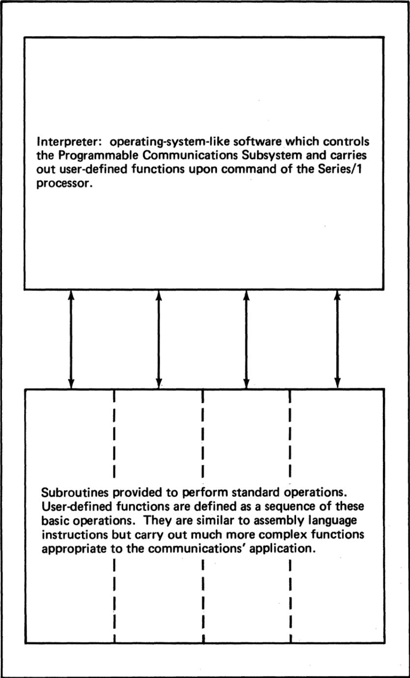
**Figure 130. Software organization within the Programmable Communications Subsystem (1 of 2)**
