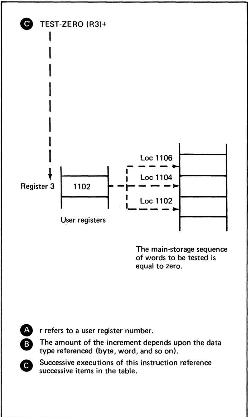
Figure 33. Storage addressing modes using registers for address storage (2 of 2)
