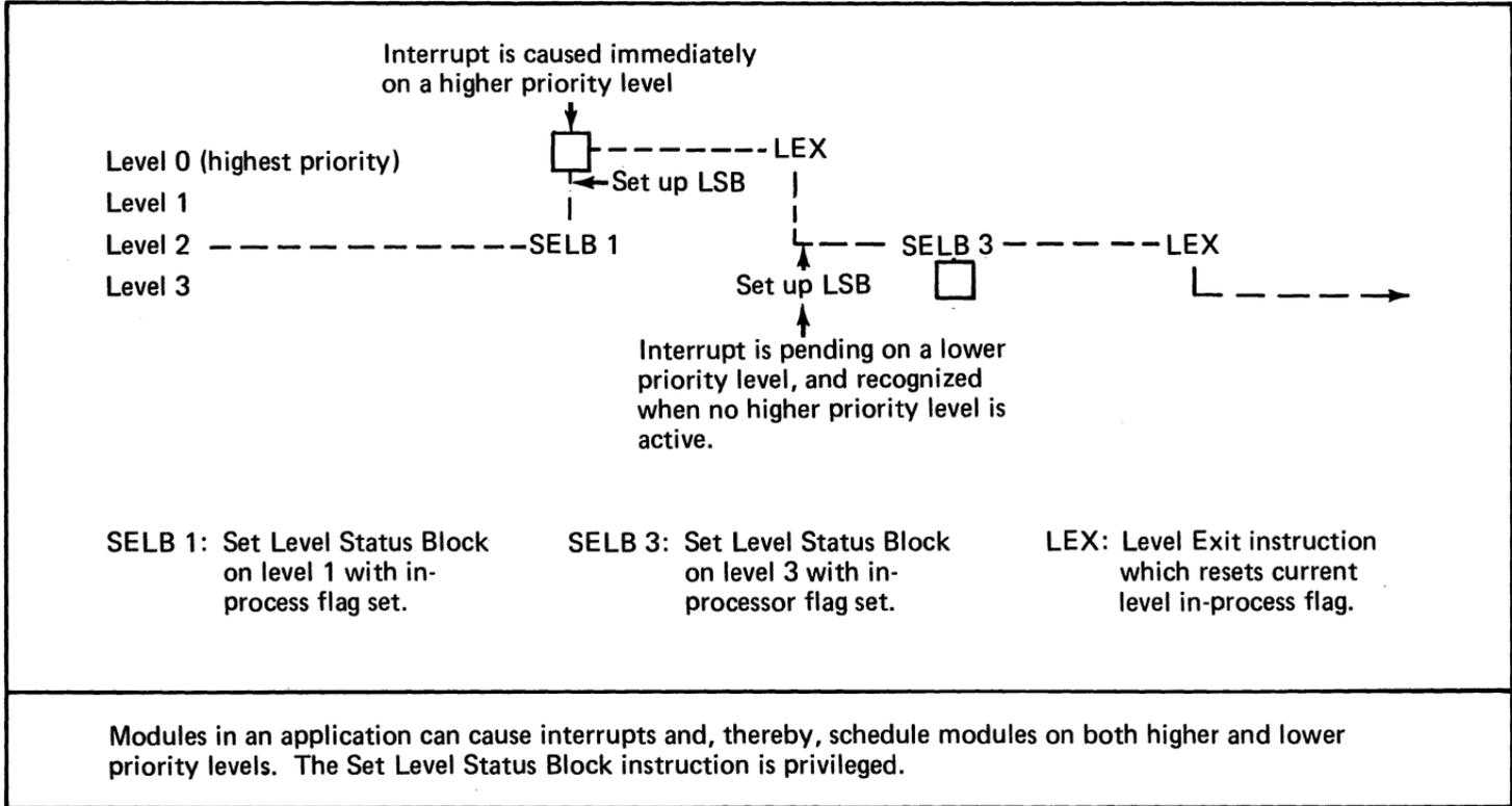
Figure 91. The level status block and module scheduling (2 of 2)
