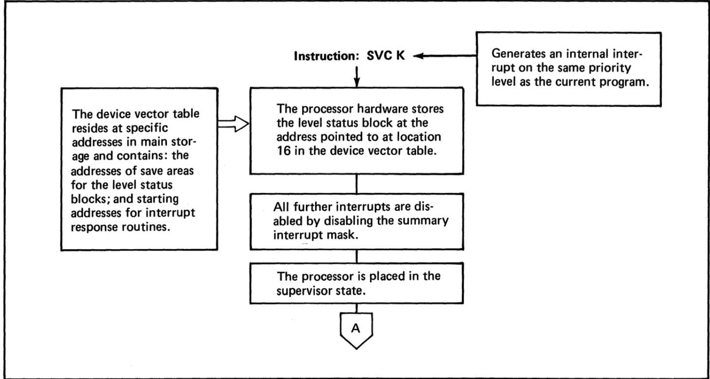
Figure 70. Communications between a task and the operating system using the Supervisor Call (SVC) convention (1 of 3)
