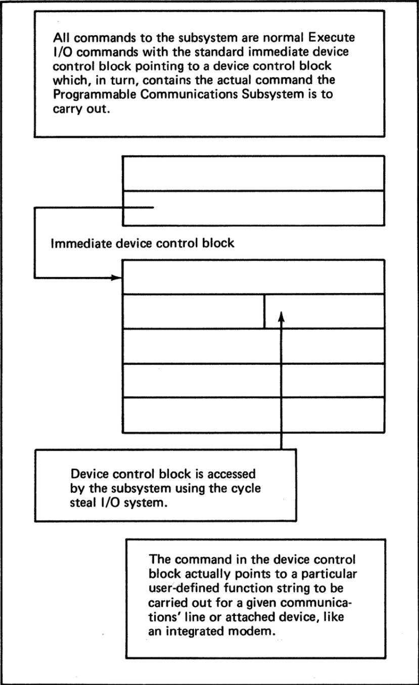
**Figure 131. Integrating software support of the Programmable Communications Subsystem into the Realtime Programming System operating system (2 of 2)**
