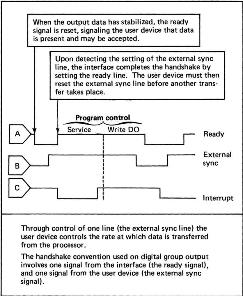
**Figure 101. The handshake convention used on digital group output (part 1)**
