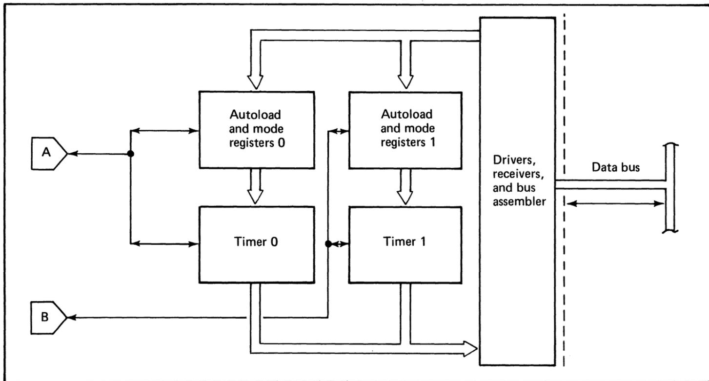
Figure 94. Block diagram of the timers showing their input/output channel connections and external signals for special uses (3 of 3)
