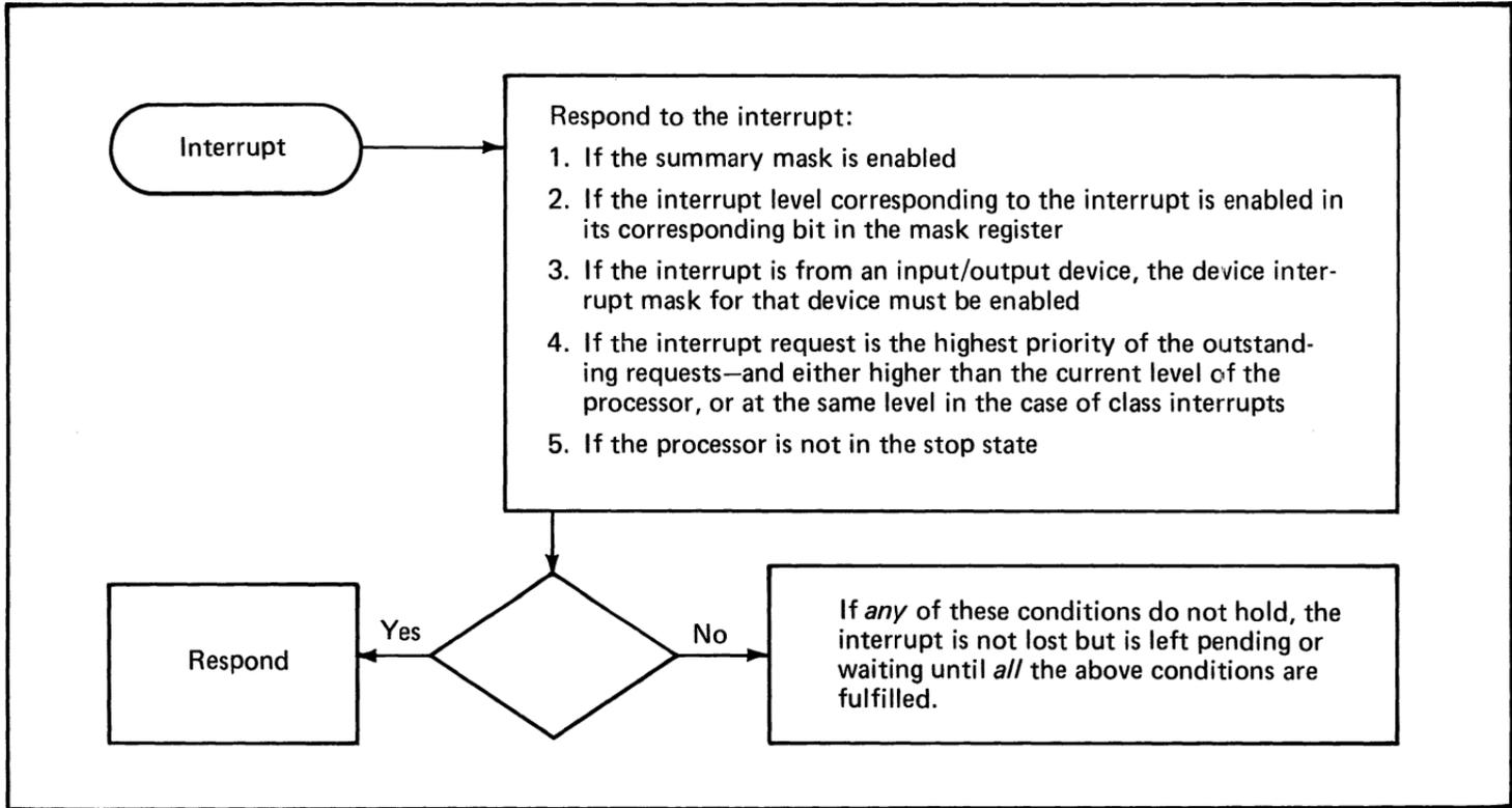
Figure 31. The priority interrupt algorithm (2 of 2)
