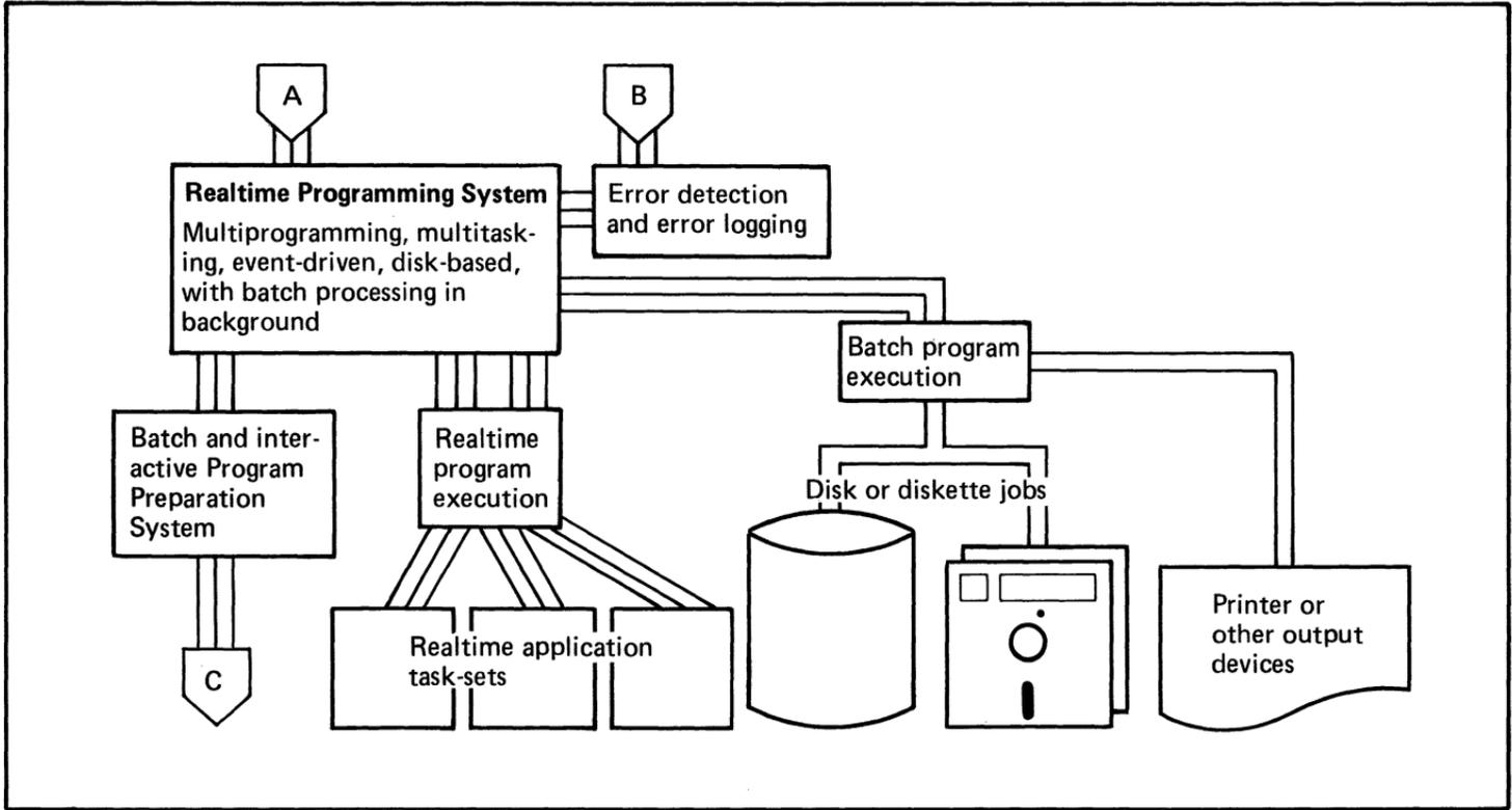
Figure 9. IBM Series/1: an integrated system of hardware, software and maintenance elements (2 of 3)
