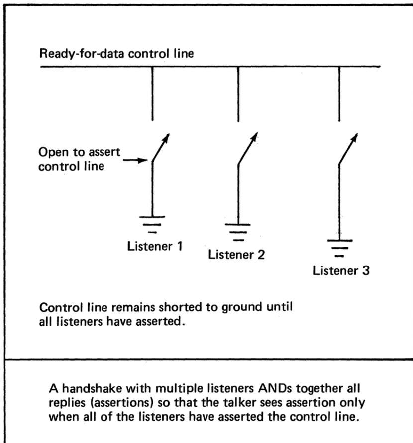
**Figure 110. Data transfers with multiple listeners**
