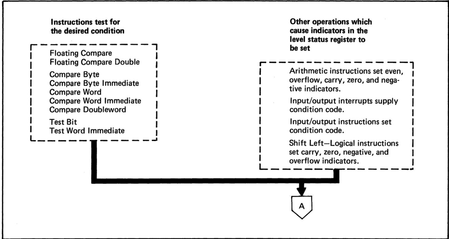
Figure 83. Operation and computation testing instructions (1 of 3)
