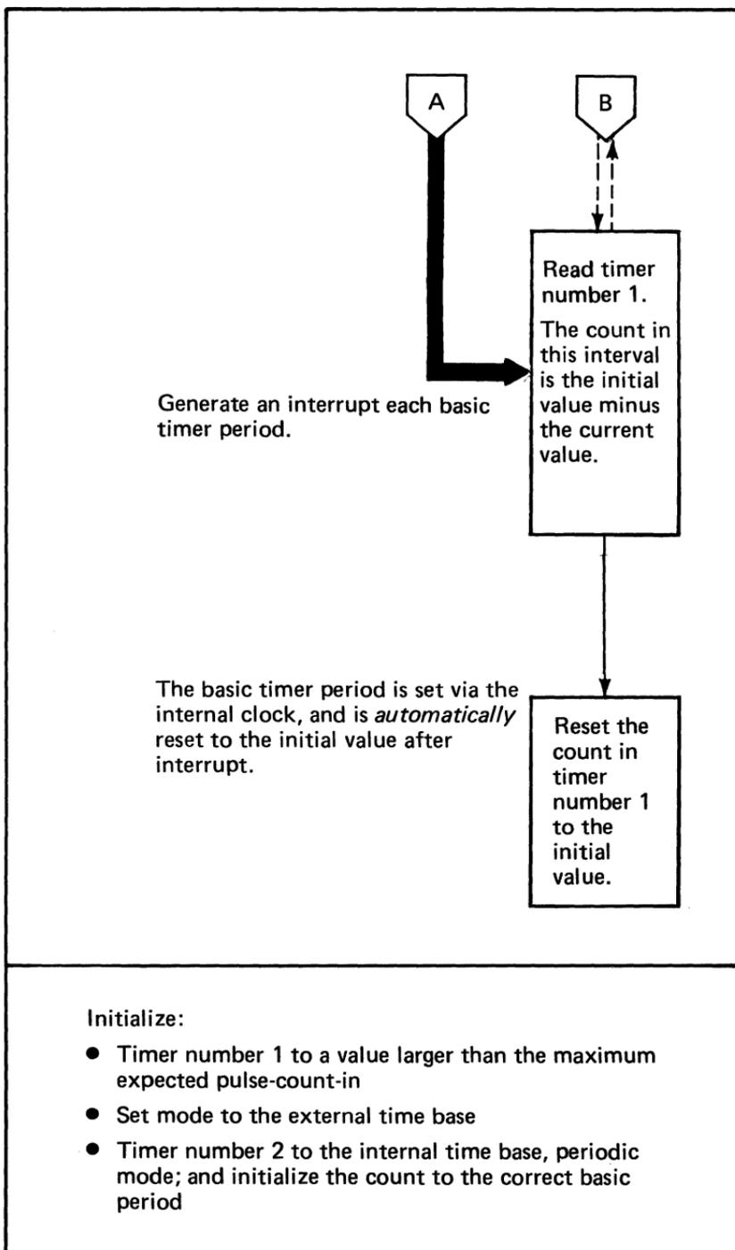
Figure 96. Pulse rate measurement using a pair of timers (2 of 2)
