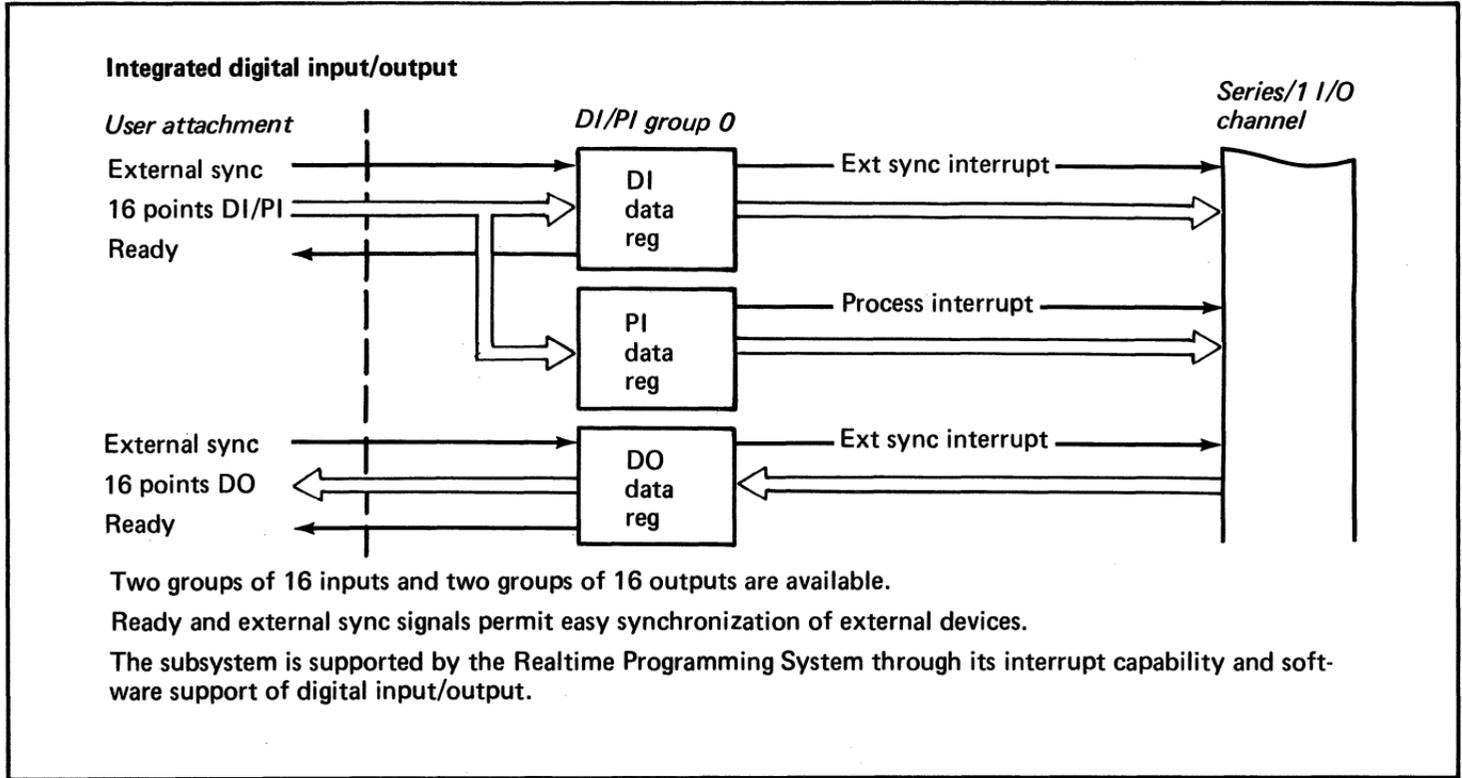
Figure 17. A subsystem can be flexibly configured to interface with a combination of analog and digital, input and output devices (3 of 4)
