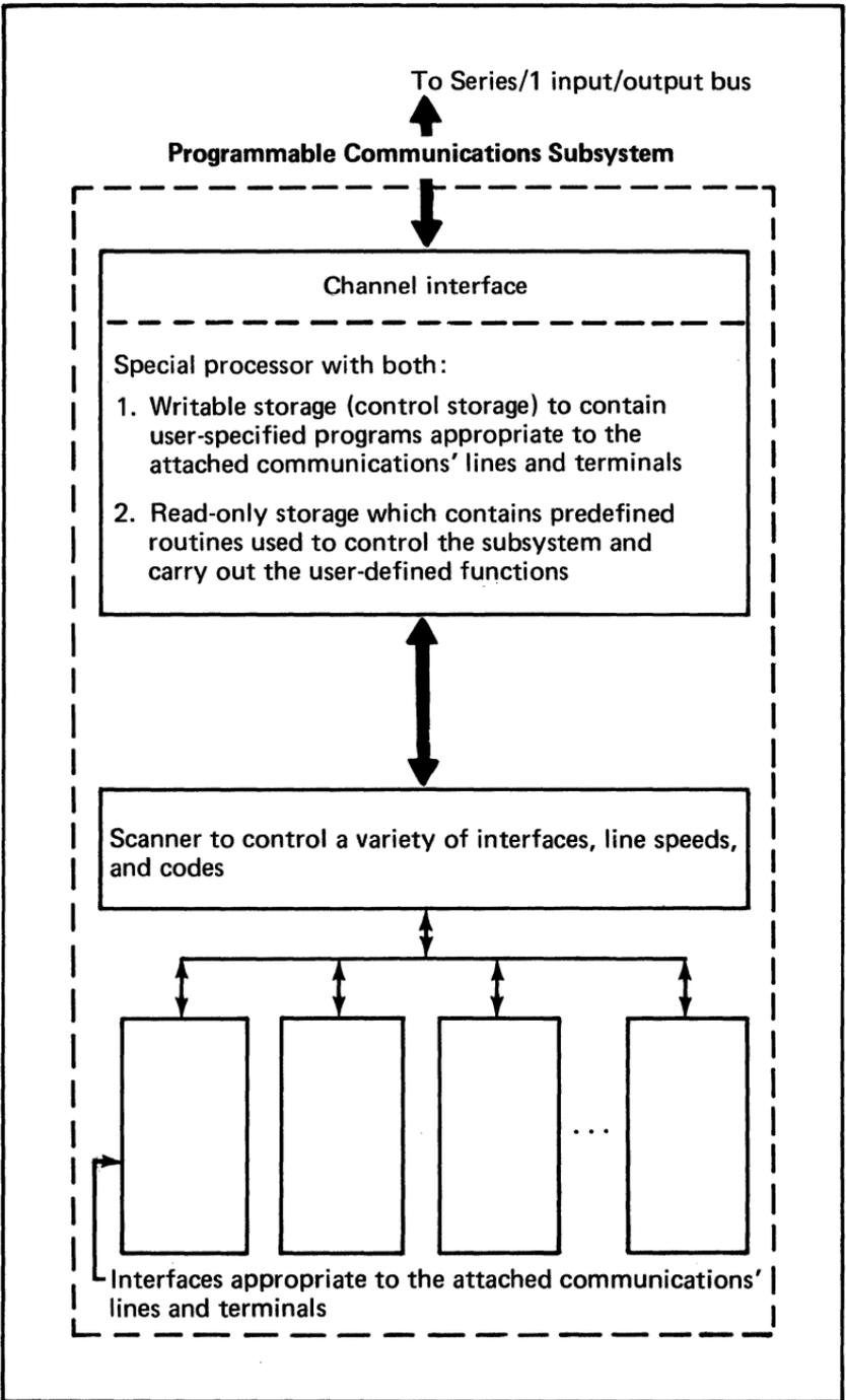
**Figure 129. Hardware organization of the Programmable Communications Subsystem**
