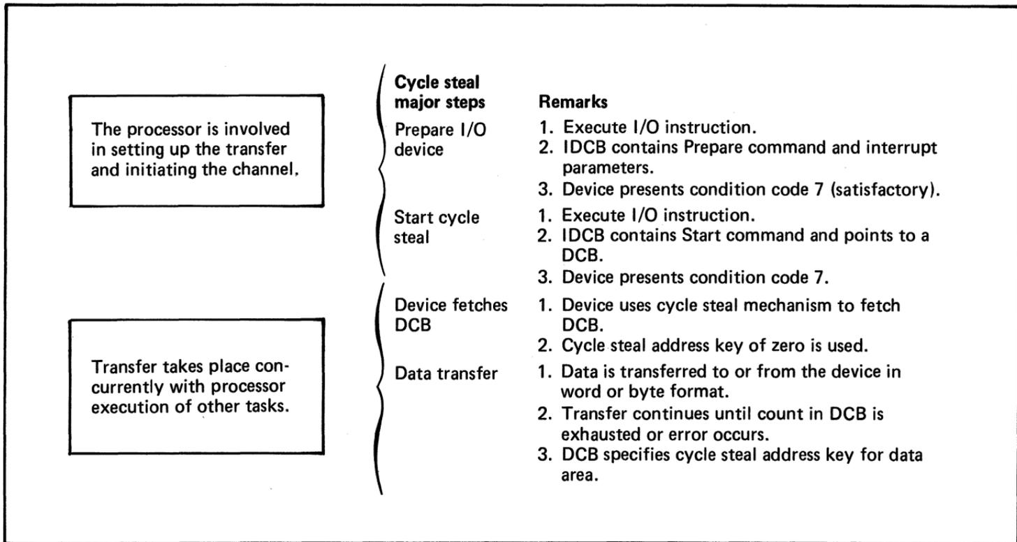
Figure 68. Sequence of operations during cycle stealing transfers (1 of 3)
