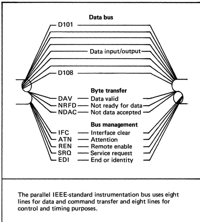
**Figure 108. The sixteen-line interface bus**
