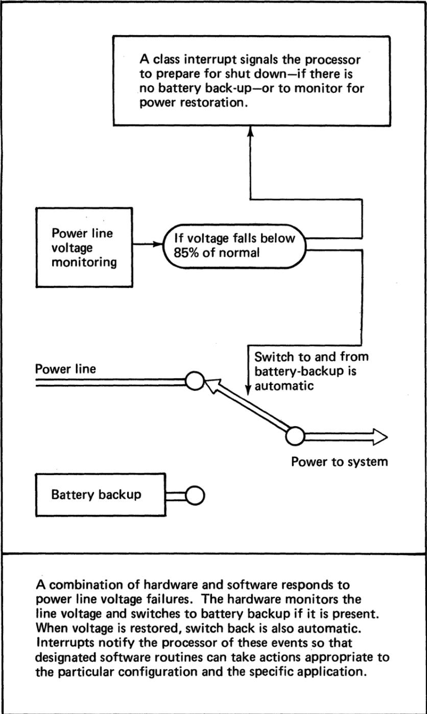
**Figure 135. Hardware and software response to a power failure**
