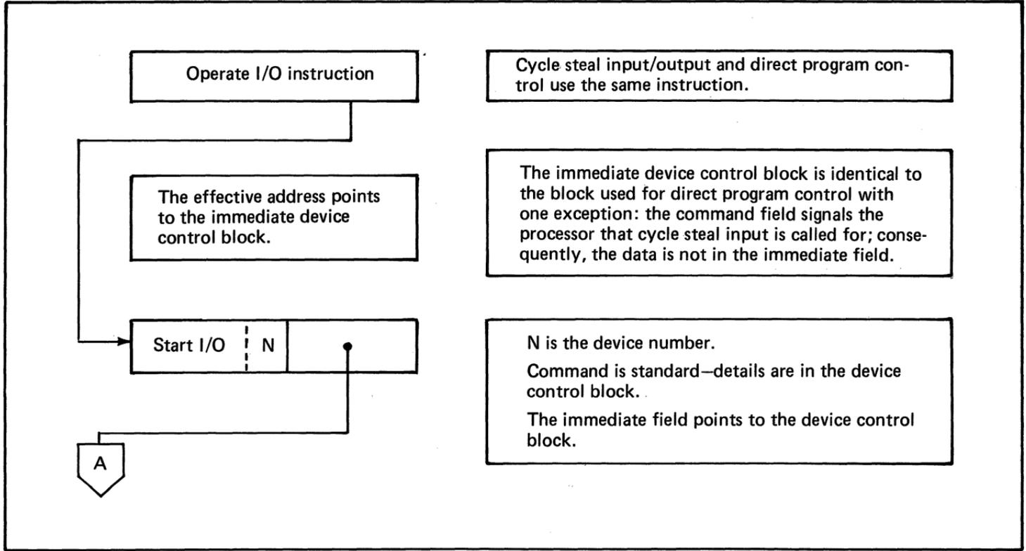
Figure 66. Cycle stealing input/output (part 2) (1 of 2)
