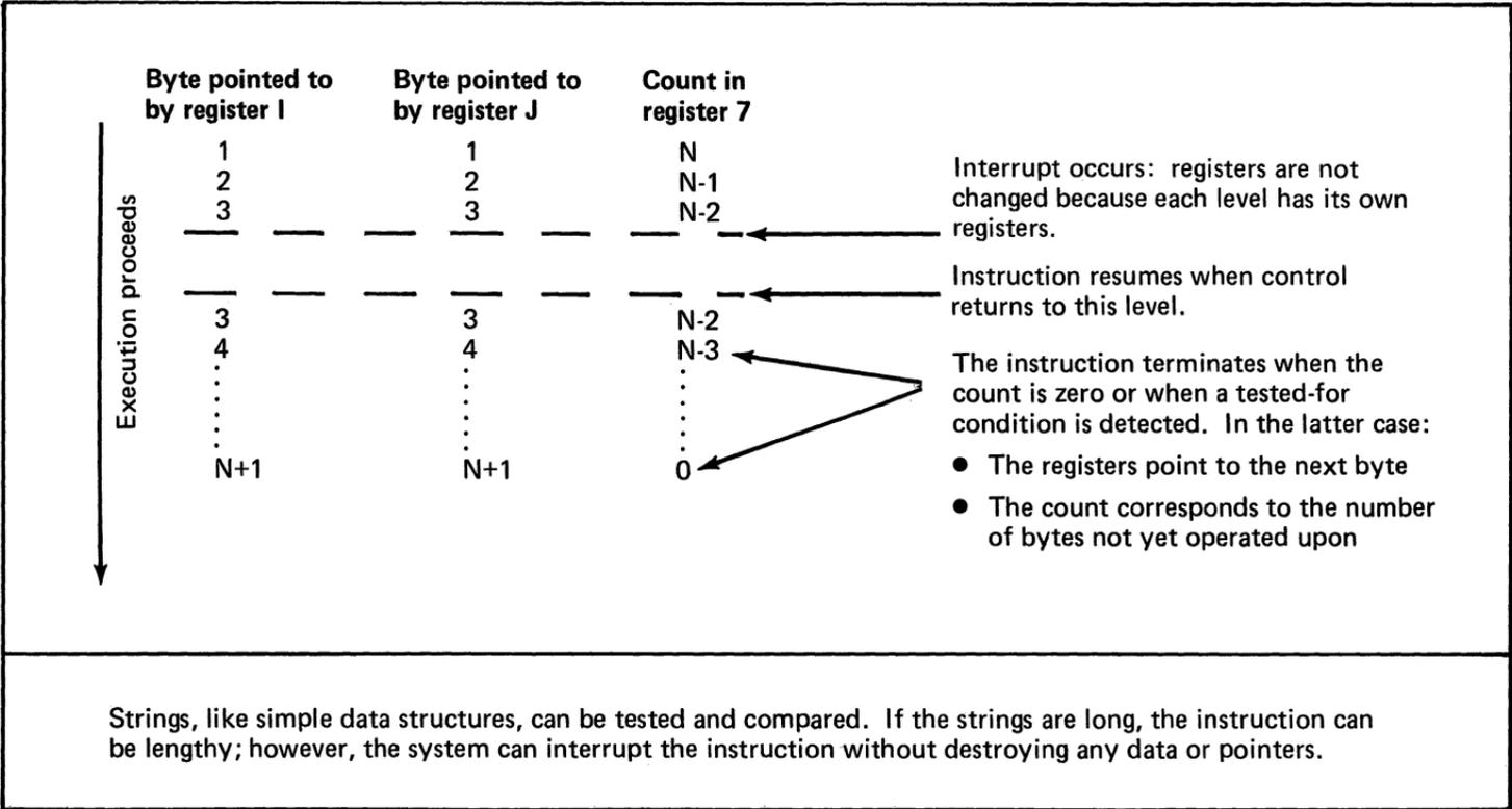
Figure 84. Comparing a string of bytes (2 of 2)
