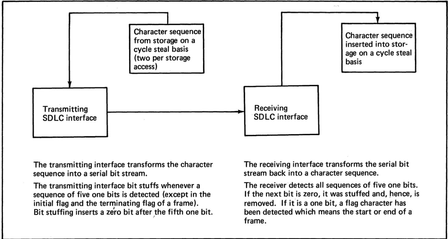
Figure 125. Bit stuffing (1 of 2)
