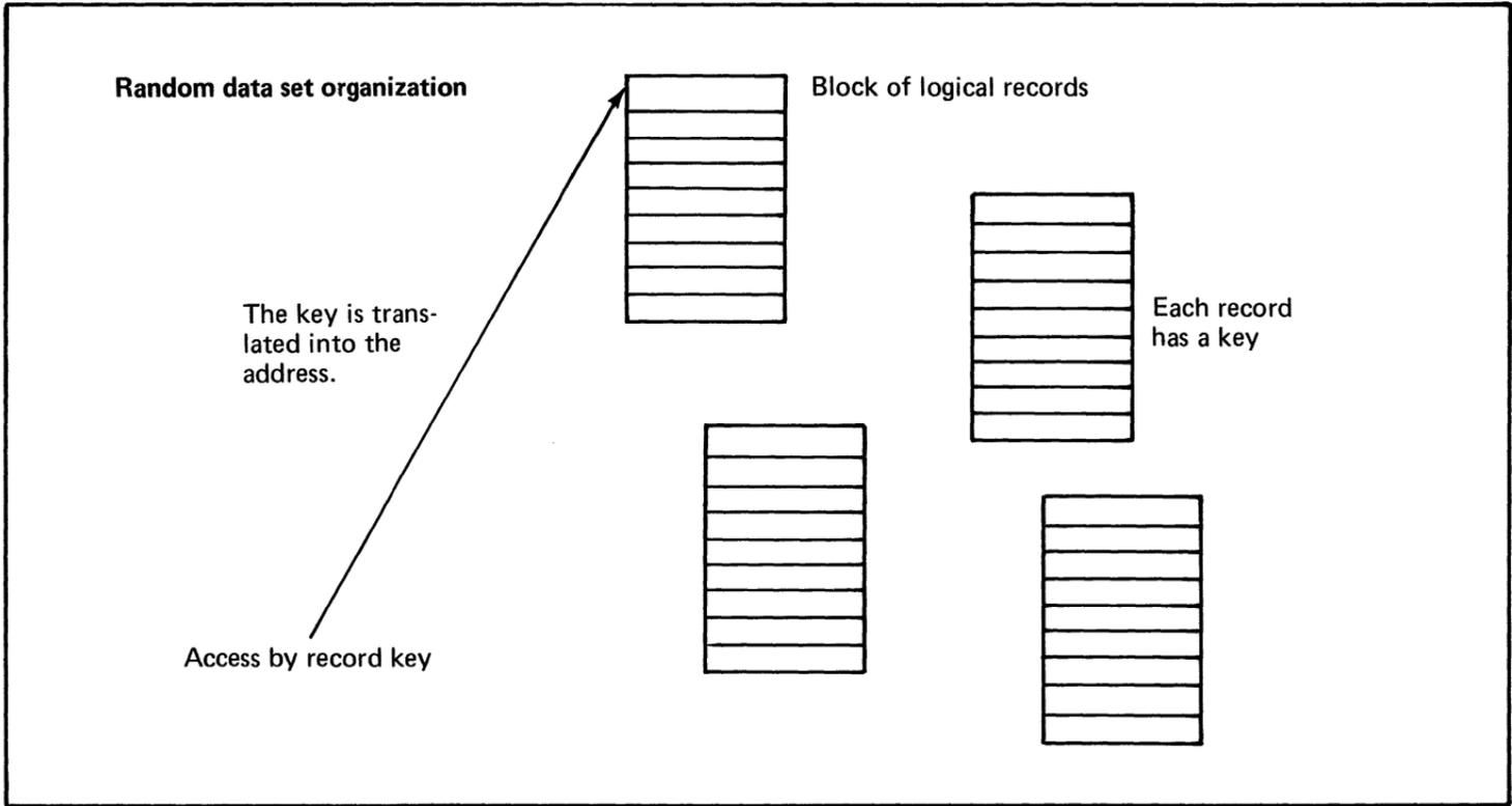
Figure 75. Four data set organizations supported under the Realtime Programming System (2 of 5)
