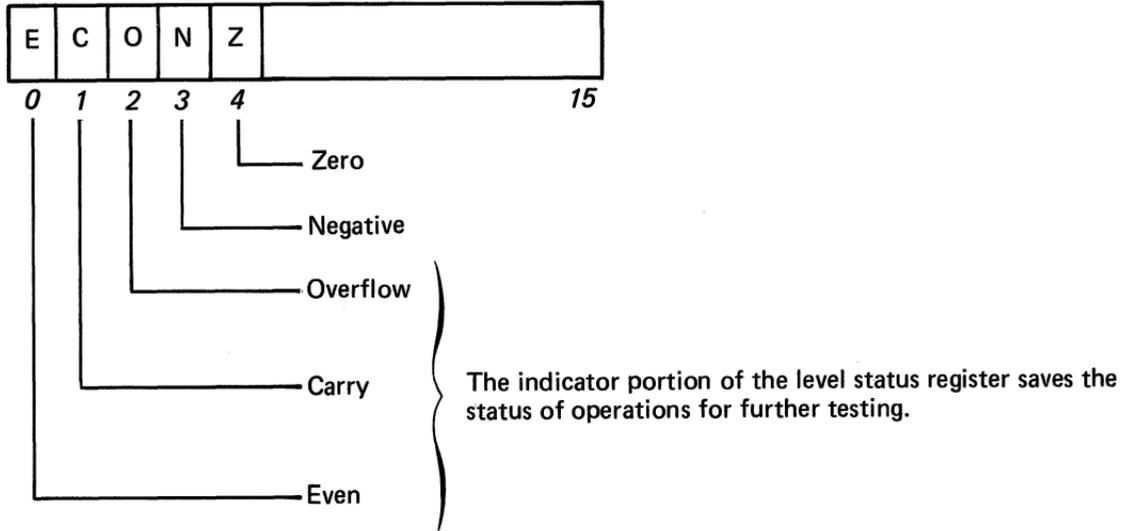
**Figure 21. Indicator set in the level status register (1 of 2)**
