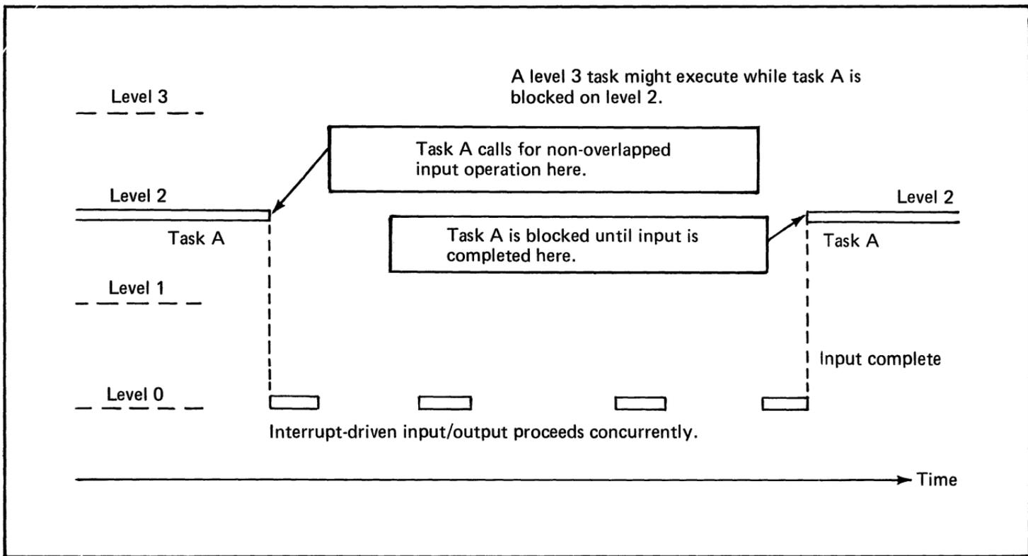
Figure 57. Effect of non-overlapped input/output on task execution (2 of 2)
