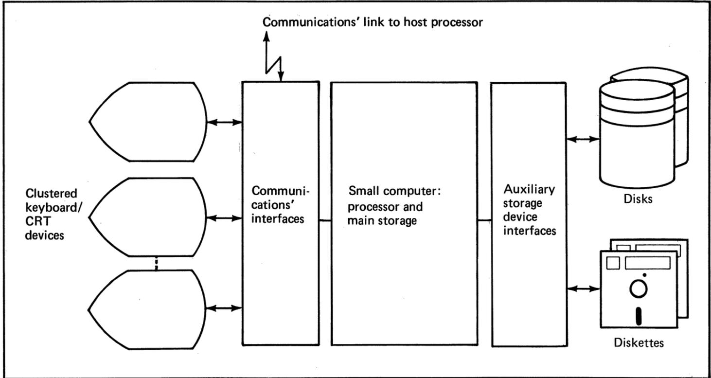
Figure 2. Common configuration for a multifunction terminal application (1 of 2)
