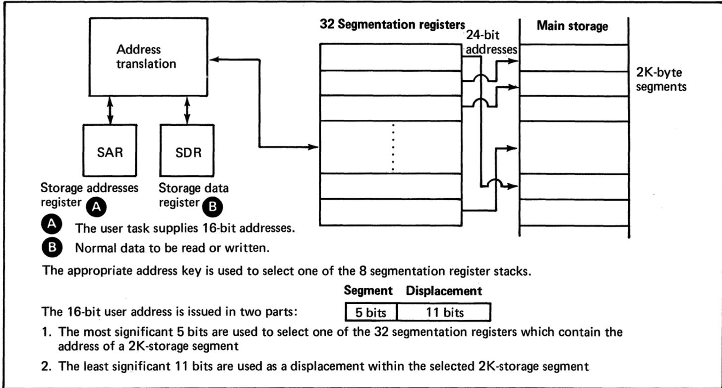
Figure 42. Conceptual basis for storage address translation
