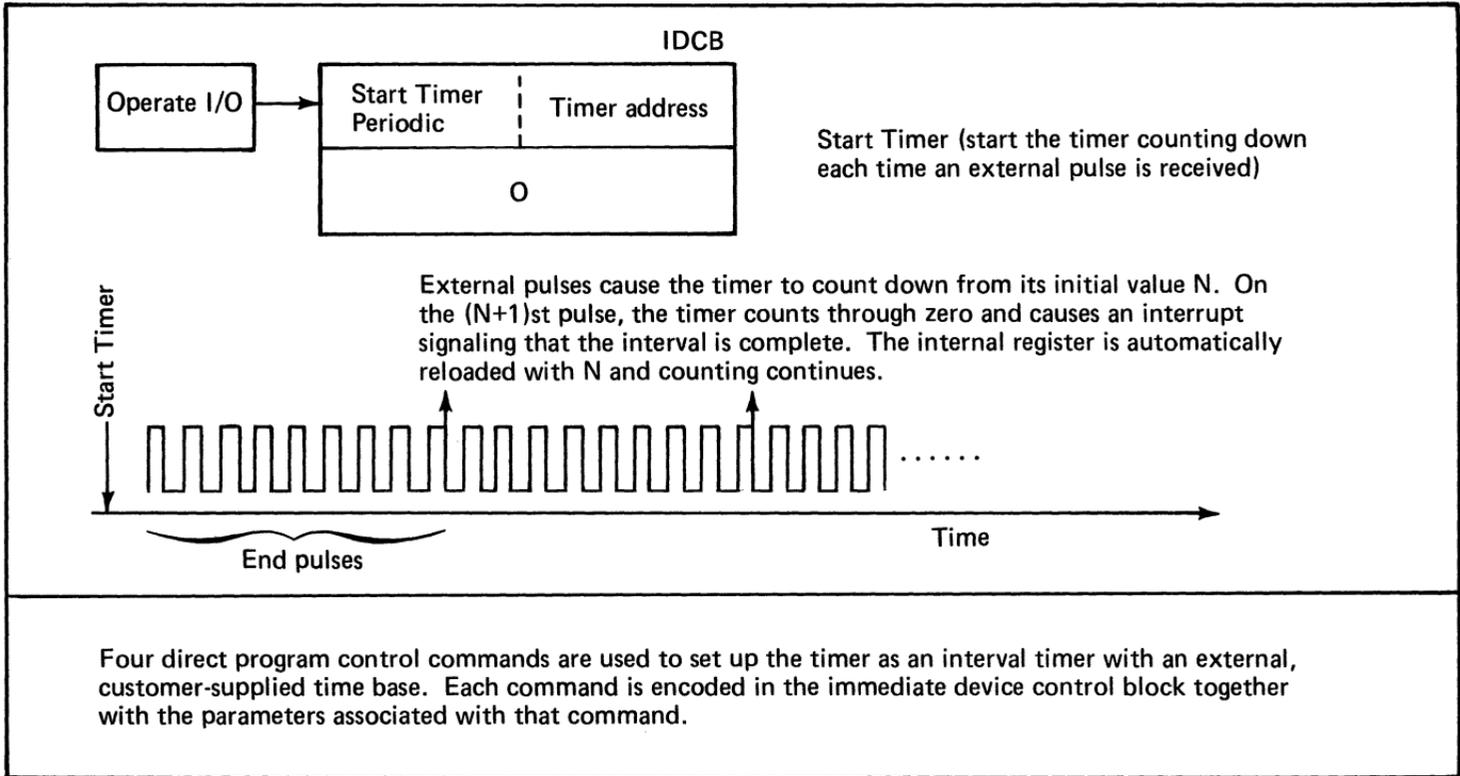
Figure 95. Using the timer to provide interval timing to the processor (3 of 3)
