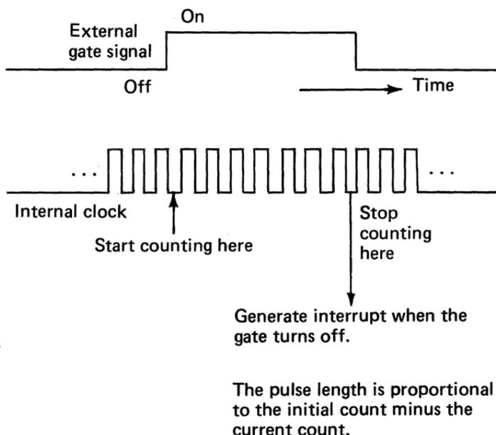
**Figure 97. Pulse duration measurement using the external signal and a timer (1 of 2)**
