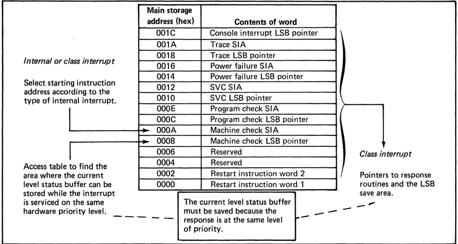
Figure 23. Input/output and class interrupts and the response of the processor (2 of 2)
