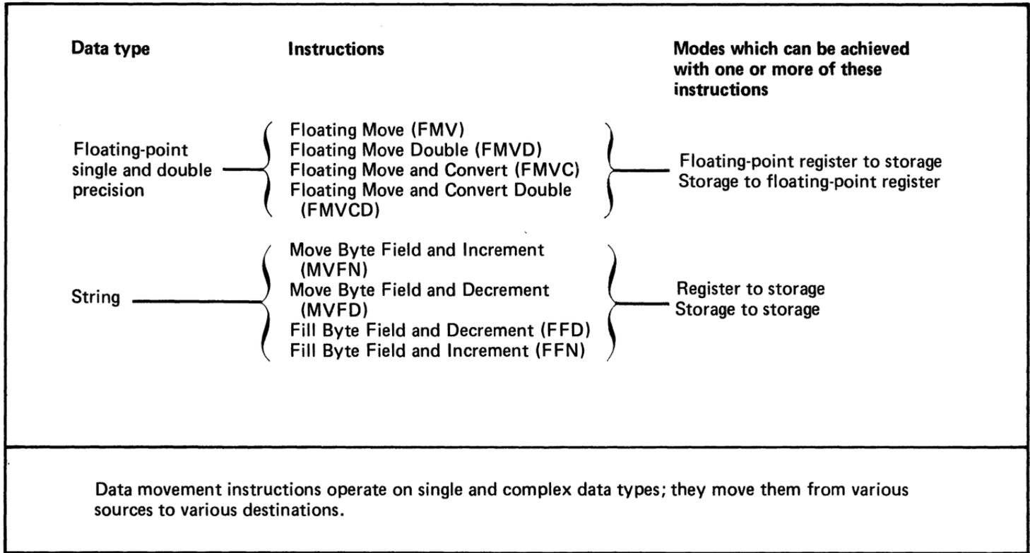
Figure 79. Series/1 instructions and modes for data movement (2 of 2)
