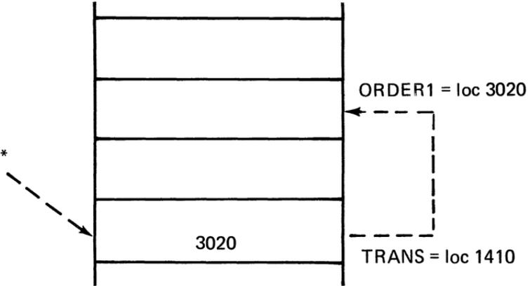
Indirect addressing allows programs to refer to different data items at different times by changing only the contents of TRANS rather than all of the addresses within the program.
