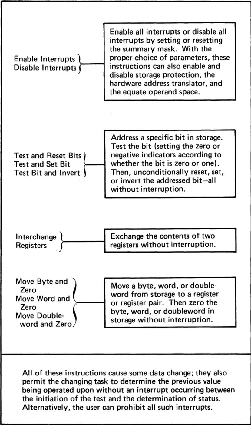
Figure 86. Instructions which can be used to control concurrency
