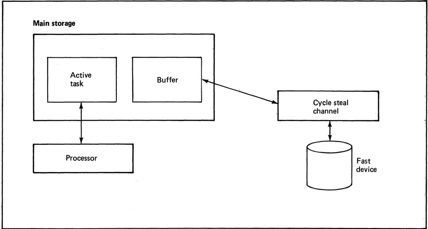
Figure 65. Cycle stealing input/output (part 1) (1 of 2)
