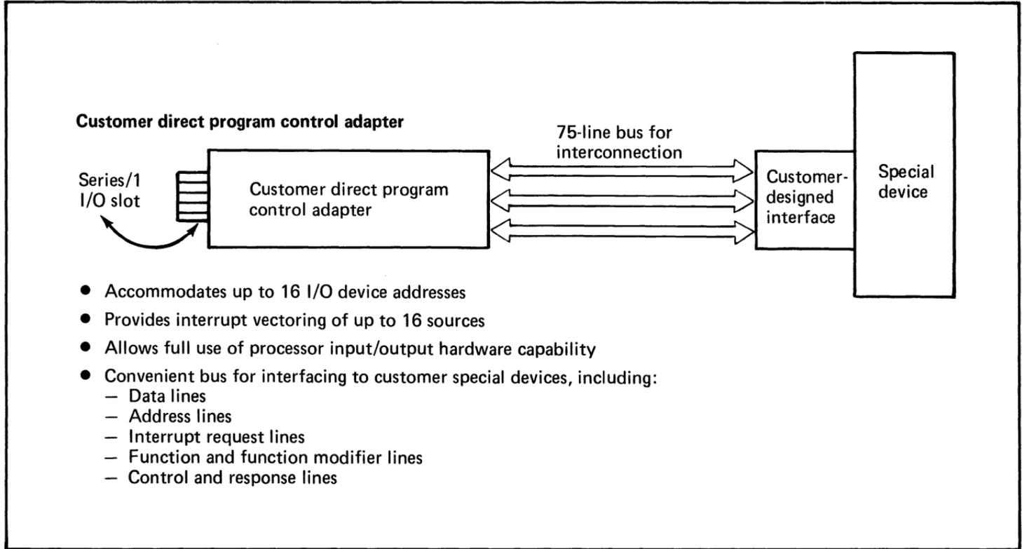
Figure 17. A subsystem can be flexibly configured to interface with a combination of analog and digital, input and output devices (2 of 4)
