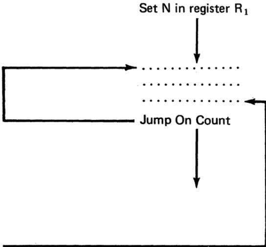
{ R<sub>1</sub> contains N during the first pass through the instructions; N-1, the second pass through, and so on.
