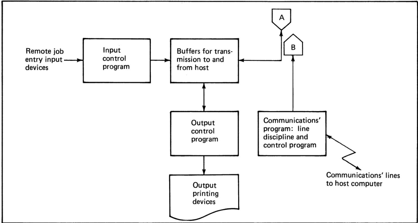
Figure 3. Multiple cooperating programs for the multifunction terminal application (2 of 3)
