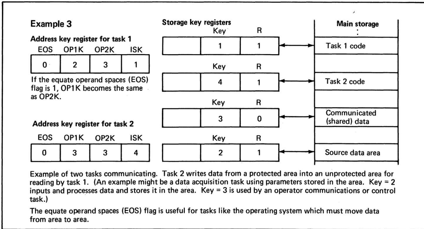
Figure 41. Three examples of address key storage protection (3 of 3)
