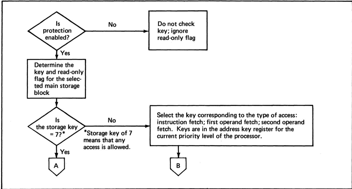
Figure 39. Operation of storage protection during an access (1 of 3)
