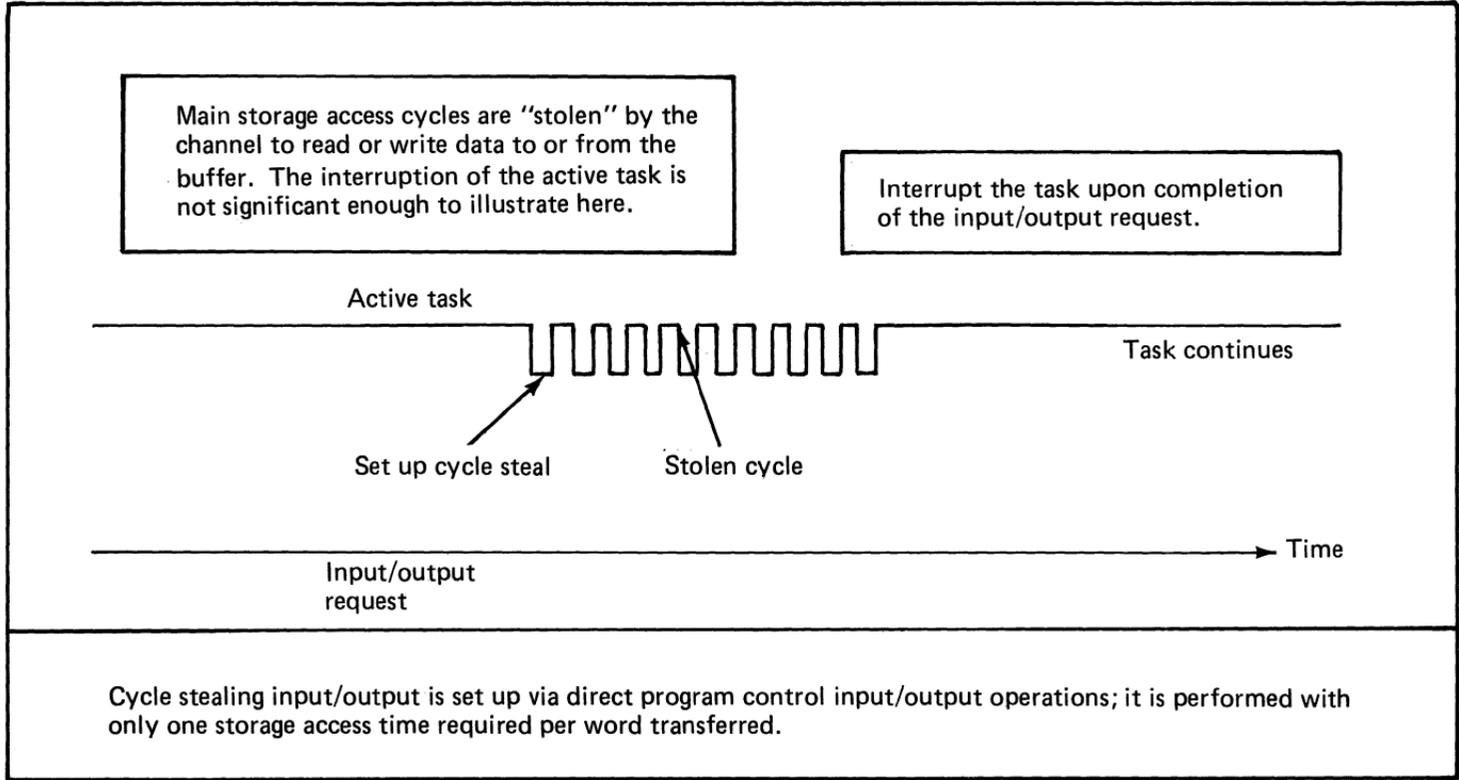
Figure 65. Cycle stealing input/output (part 1) (2 of 2)
