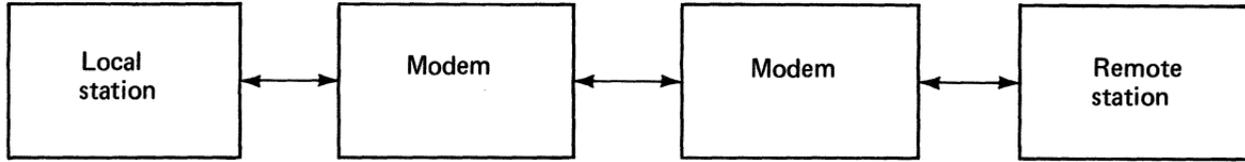
A point-to-point connection of two communicating stations. The modem is necessary only if the distance is long or the telephone communication facilities are used.
