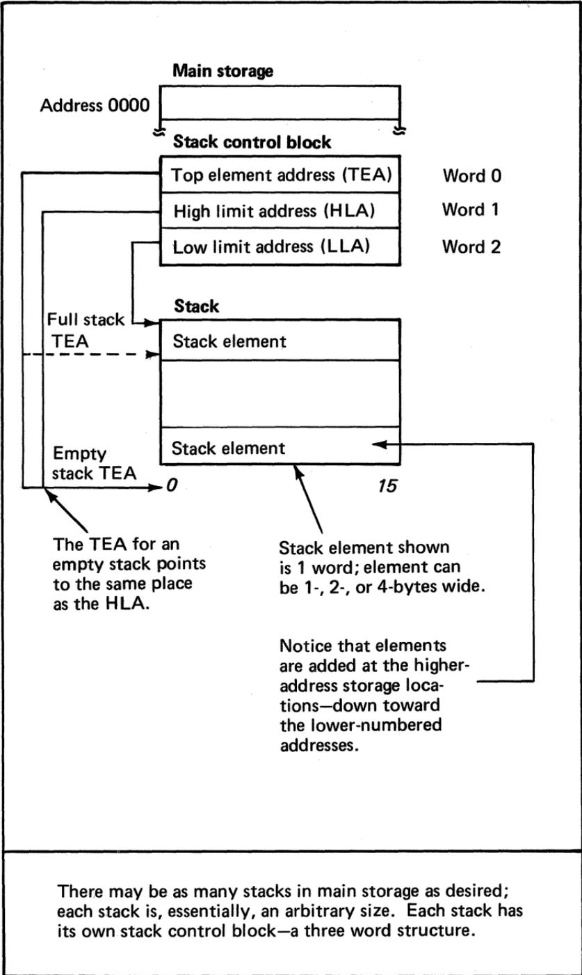
Figure 26. The relationship of the stack control block to the data stack
