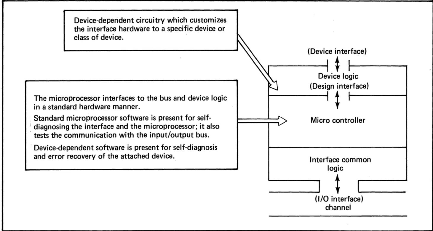
Figure 54. Organization of the microprocessor-controlled interface between the input/output channel and devices
