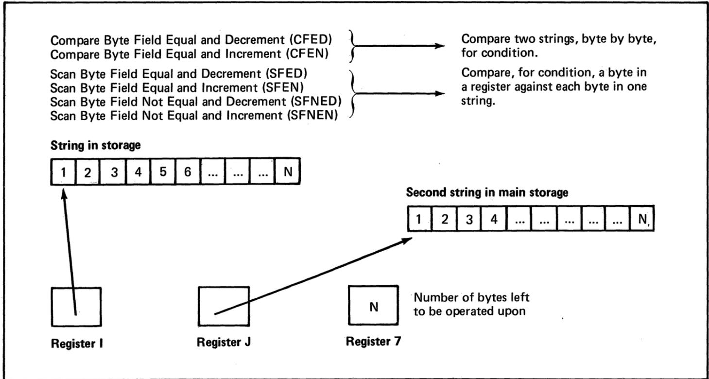
Figure 84. Comparing a string of bytes (1 of 2)
