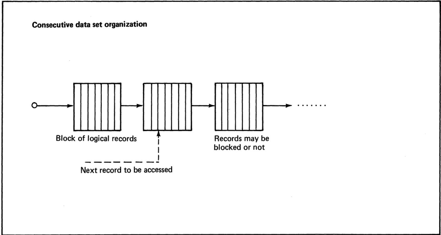
Figure 75. Four data set organizations supported under the Realtime Programming System (1 of 5)
