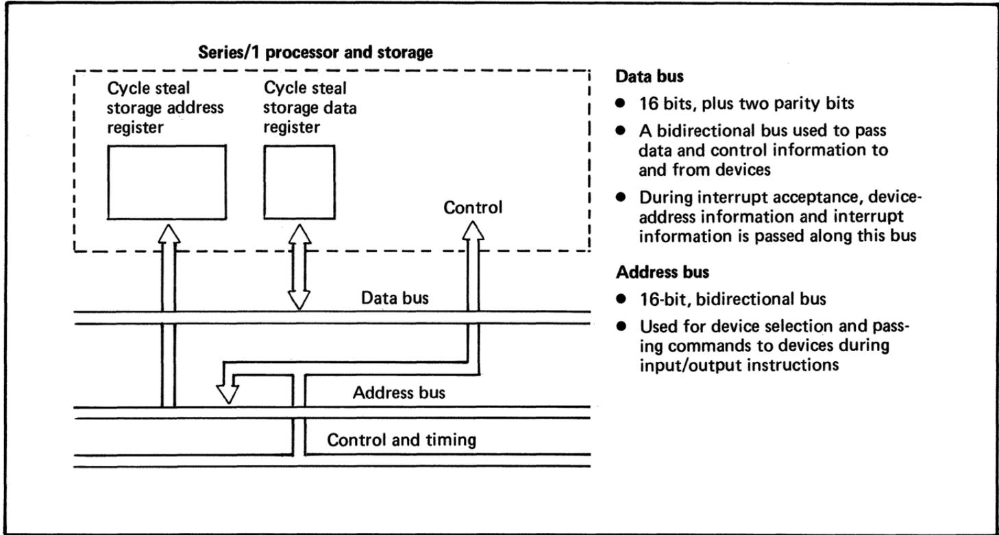
**Figure 55. The Series/1 input/output bus: asynchronous and multidropped (1 of 2)**
