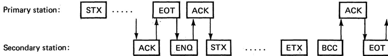
Messages may alternate in direction at times determined by control characters like end of transmission.
