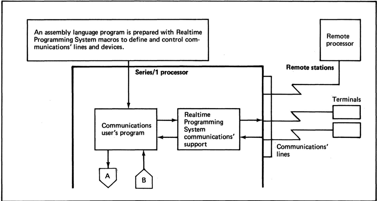
Figure 127. Software use of communications (1 of 2)
