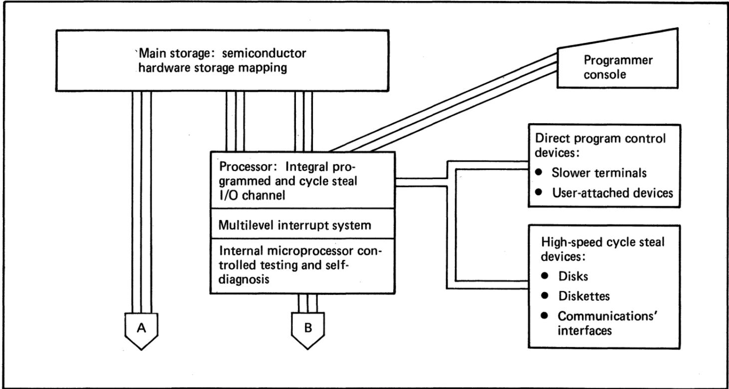
Figure 9. IBM Series/1: an integrated system of hardware, software and maintenance elements (1 of 3)
