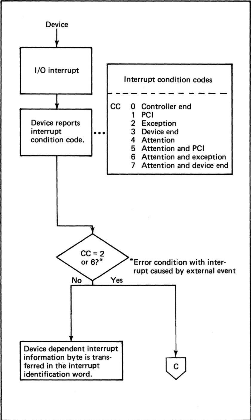
Figure 63. Condition codes accompanying each input/output interrupt (3 of 5)
