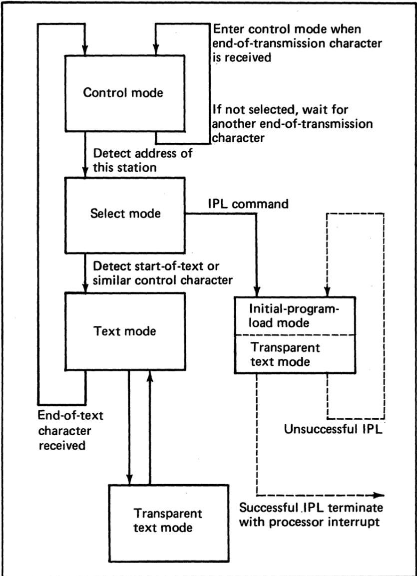
The binary synchronous interface operates in one of several modes depending upon whether it is selected by the controlling station for transmission or receiving, for initial program load, or for other functions. The mode changes are caused by detection of pre-defined control characters.
