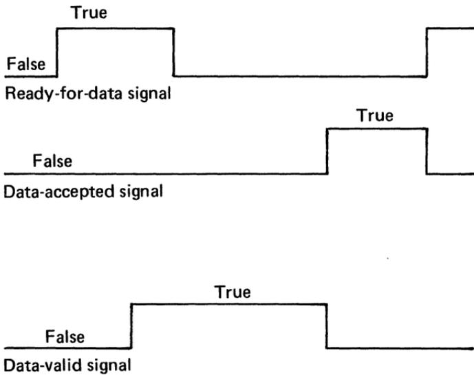
1. The talker puts data on data lines and signals data-valid after receiving the ready-for-data signal.
