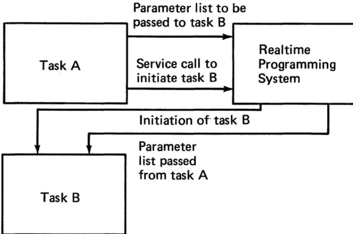
**Events:** a set of conditions detected by one or more tasks, the occurrence of which can cause execution of other tasks. Interacting tasks can easily synchronize with the event mechanism.
