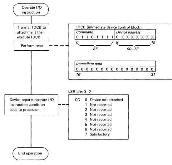
Figure 2-5. Device reset command operation
