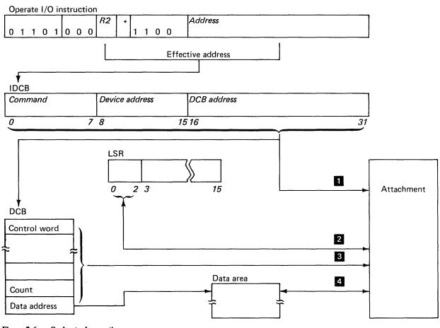
Figure 2-6. Cycle steal operation
