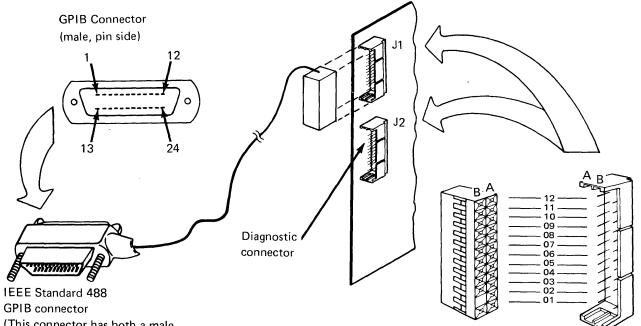
(This connector has both a male and a female to permit stacking.)
