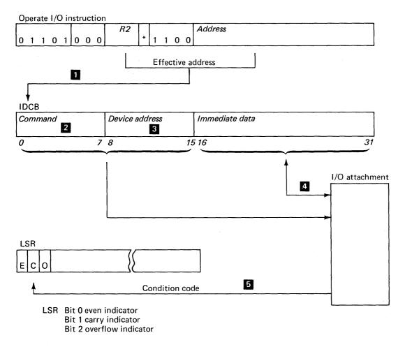
Figure 2-2. Direct program control I/O operation
