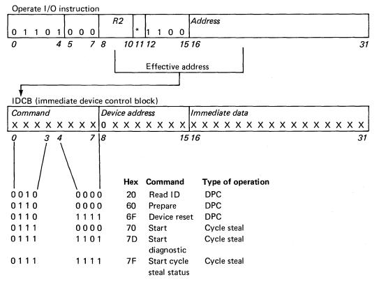
Figure 2-1. Operate I/O instruction and IDCB formats
