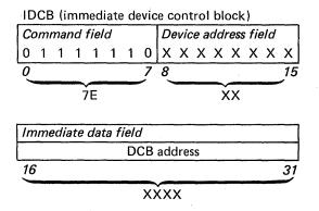
In the DCB control word, bit 2 must equal 1, bits 5–7 can equal either 0 or 1 and all other bits must equal 0. The byte count must be 0002 (for both single-line and multiple-line attachments), and the data address must be even. If any of these conditions are not met, the attachment presents an exception interrupt request and reports DCB specification check in the interrupt status byte.
