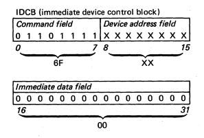
A Device Reset command issued to the attachment causes the attachment to become busy while the reset functions are carried out. There are differences between the single-line attachment and the multiple-line attachment are:
