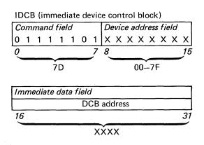
The byte count for this operation must be 12 (hex 000C) and the data address must be even; otherwise, a DCB specification check will occur. The DCB control word should be hex 2000.
