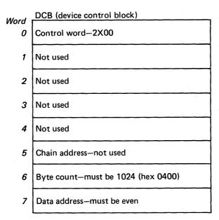
This operation begins if DCB word 0 bit 2 equals 1 and the byte count is 1024. Starting at the address specified in DCB word 7, the attachment cycle steals 1024 bytes of data from the attachment into storage. A device-end interrupt request is presented when the cycle stealing is completed.
