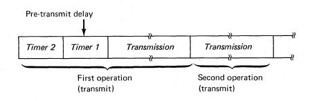
Timer 1 should be set for a pre-transmit delay of approximately 9 milliseconds when the receiving station is a program-controlled device and is directly connected or is connected through a full-duplex modem. Timers 1 and 2 should always be activated to prevent excessive turnaround and noise.
