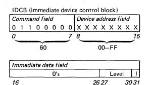
Level. This four-bit field specifies the priority interrupt level assigned to the device. Bits 27 through 30 indicate priority levels.
