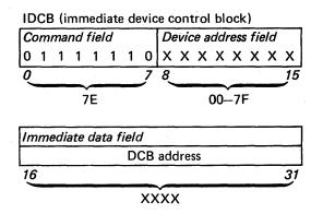
The byte count for this operation must be 12 (hex 000C) and the data address must be even; otherwise a DCB specificaiton check will be transmitted. The DCB control word should be hex 2000. For this command to operate properly, the attrachment must be disconnected from the modem and a wrap connector must be plugged into the modem end of the cable that goes from the attachment to the modem.
