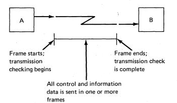
The higher level of grouping, a frame sequence, is checked by the program for missing or duplicated frames. At a station that transmits sequenced frames, the program counts and numbers each sequenced frame; this count is called Ns. At a station receiving sequenced frames, the program counts each error-free sequenced frame that it receives; this count is called Nr.
