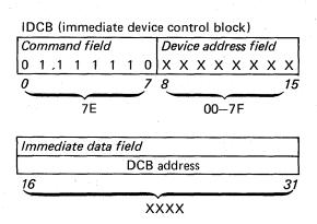
When a Start Diagnostic 2 command is issued to the attachment, various operations as defined in the DCB are executed. These operations are terminated with a device-end interrupt request after the attachment cycle steals the Start Diagnostic 2 words into storage. The operations and words are described below.
