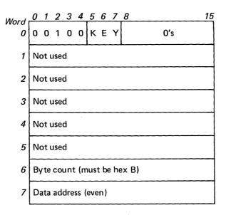
The diagnostic first performs an attachment storage test, which consists of writing/reading 1's and 0's through all the storage locations. If the test is successful, a hex FF is written into data word 5, high-order byte. If the test fails, a hex 00 is written into data word 5, bits 0-7.
