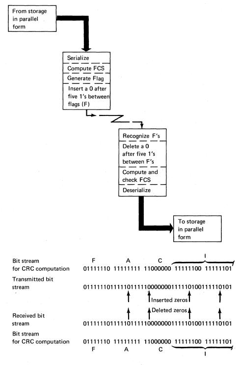
Data Link Control Functions and Zero Insertion/Deletion
