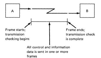
In the higher level of grouping, a frame sequence is checked by the program for missing or duplicated frames. At a station that transmits sequenced frames, the program counts and numbers each sequenced frame; this count is called Ns. At a station receiving sequenced frames, the program counts each error-free sequenced frame that it receives; this count is called Nr.
