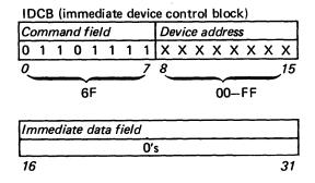
A Device Reset command issued to the attachment causes the attachment to become busy while the reset functions are carried out. The amount of time that the attachment is busy is a function of the microcode program. The attachment presents a busy after reset (CC2) if an Operate I/O immediately follows a Device Reset.
