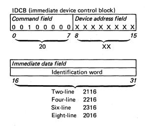
*Note:* If the controller card has jumpers installed for addresses that are not valid, the controller responds to commands as though the 4-line adapter card was present; therefore, the ID of the controller should match the number of attachment lines present to prevent errors. For example, an ID of 2016 or 2316 defines a controller with two 4-line attachments. If there is only one 4-line attachment present, the ID is 2216 or 2116.
