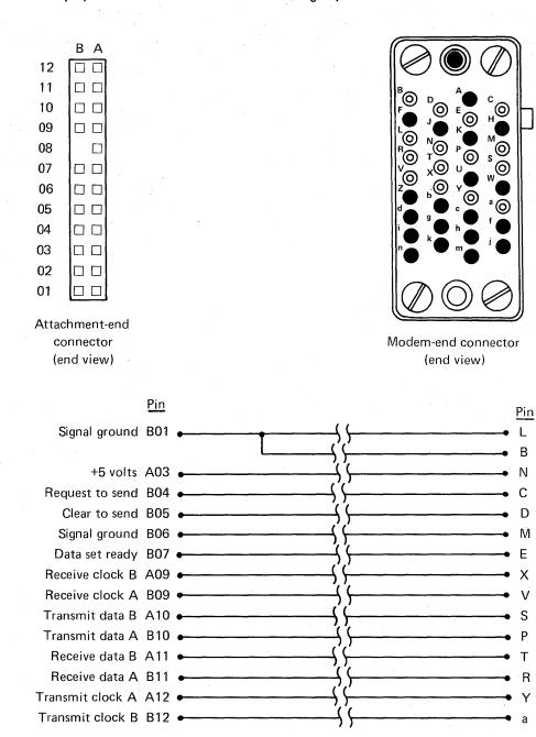
Binary Synchronous Communications V .35/High Speed DDN Cable
