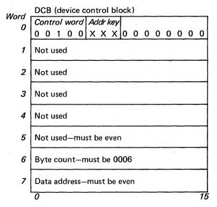
Figure 2-5. Format of the DCB for a Start Cycle Steal Status command
