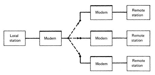
An X.21 leased network consists of a station connected to one or more remote stations by a data circuit terminating equipment (DCE), synchronous communications single line control (SCSLC), and leased-line connecting the stations.
