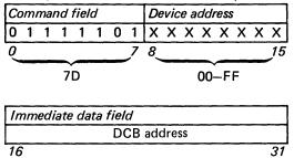
Start Diagnostic 1 causes two types of tests to occur in the attachment, with the results placed in processor storage beginning at the address specified in word 7 (data address) of the DCB. The byte count for this operation must be equal to 11 and the data address must be even; otherwise, an exception interrupt is presented with bit 3 (DCB specification check) set in the interrupt status byte.
