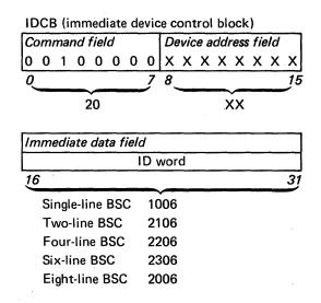
*Note:* If the control-feature card has jumpers installed for addresses not present, the controller responds to commands as if the hardware is present. Consequently, the ID of the controller should match the number of attachment lines present to prevent errors. For example, an ID of 2006 defines a multiple-line controller with two 4-line attachments (all eight lines in use). If there is one 4-line attachment present, the ID is 2206 (or 2106 if only two of the four lines are in use).
