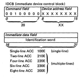
*Note:* If the controller card has jumpers installed for addresses that are not present, the controller responds to commands as though the 4-line adapter card was present; therefore, the ID of the controller should match the number of attachment lines present to prevent errors. For example, an ID of 200E defines a multiple-line controller with two 4-line attachments (8 lines). If there is only one 4-line attachment present (4 lines), the ID is 220E.
