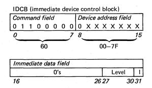
Level This four-bit field specifies the priority interrupt level assigned to the device. The binary value of bits 27-30 indicates priority levels of 0-3.
