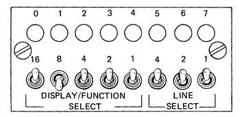
The indicator panel can be used with any of the communication features. The panel's cable plugs into a connector on a feature control card, and the panel can be moved between processor units and input/output (I/O) expansion units; it is not necessary to have more than one indicator panel. The panel does not attach to the half-width model of the processor.
