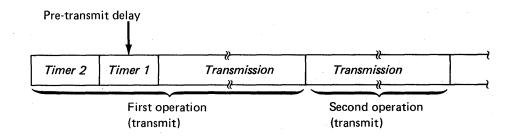
*Note:* Timer 1 should be set for a pre-transmit delay of approximately 9 milliseconds when the receiving station is a program-controlled device and is directly connected or connected through a full-duplex modem. Timers 1 and 2 should always be specified to prevent excessive turnaround times and noise.
