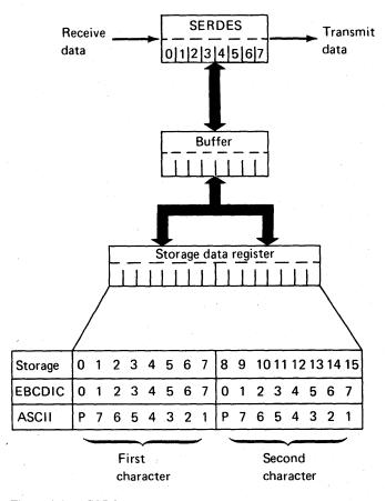
Figure 4-1. SDLC attachment data flow
