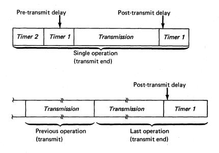
**Transmit Allow Break.** This operation is the same as the transmit operation, except that it allows the receiving station to stop the transmission. To do this, the receiving station "breaks" the line by driving its transmit line to a "space" condition for at least 150 milliseconds. If the attachment detects this condition, it presents an exception interrupt request with bit 0 equal to 1 in the interrupt status byte. Status word 1 bit 6 is equal to 1 to indicate a break.
