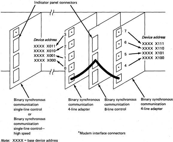
**Binary Synchronous Communications Control Feature**
