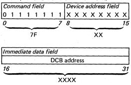
The byte count in the DCB (word 6) must be equal to 6 and the data address (word 7) must be on a word boundary (bit 15 off) or an exception interrupt request (CC2) will occur with DCB specification check bit (bit 3) equal to 1 in the interrupt status byte.
