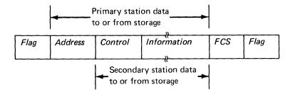
The accumulation of frame-check sequences starts with the address and includes the frame-check sequence (FCS) received.
