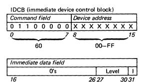
*Level - bits 27-30:* This four-bit field specifies the priority interrupt level assigned to the device. The binary value of bits 27-30 indicates priority levels of 0-3.
