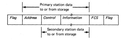
The accumulation of frame-check sequences starts with the address and includes the frame-check sequence received.
