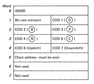
**COD1/EOA.** When the first end-of-address (EOA) (1) character is received, the attachment begins longitudinal redundancy check (LRC) character accumulation, starting with the next character received. The EOA character is placed into storage. Any characters received between the first EOA and the COD 5 (2) character that have the same bit configuration as the EOA are treated as data.
