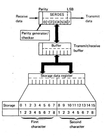
*Note:* The programmable attachment transmits by sending out the low-order bit of the byte first. The received characters are stored in the same manner; that is, the first bit received is the low-order bit of the byte. If the character is less than 8 bits, it must be right justified. If the data address (DCB word 7) is odd, only one character is moved in or out of storage on the first data transfer.
