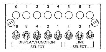
The indicator panel can be used with any of the communication features. The panel's cable plugs into a connector on a feature control card, and the panel can be moved between processor units and input/output (I/O) expansion units; it is not necessary to have more than one indicator panel. The panel does not attach to the half-width model of the processor.
