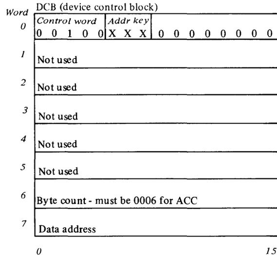
Figure 2-3. Format of the DCB for a start cycle steal status command
