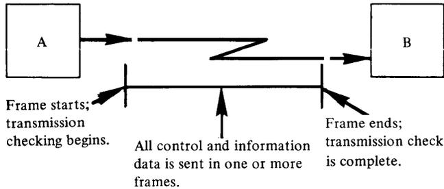
The higher level of grouping, a frame sequence, is checked by the software for missing or duplicated frames. The software at a station transmitting sequenced frames counts and numbers each sequenced frame. This count is known as *Ns*. The software at a station receiving sequenced frames counts each error-free sequenced frame that it receives; the receiver count is called *Nr*.
