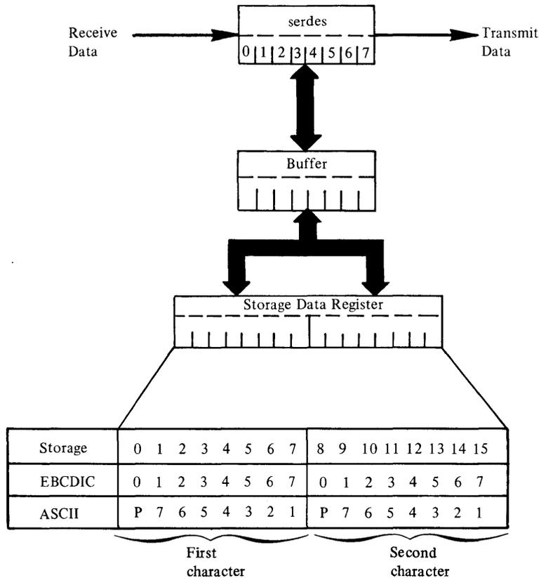
Figure 4-1. SDLC Attachment Data Flow
