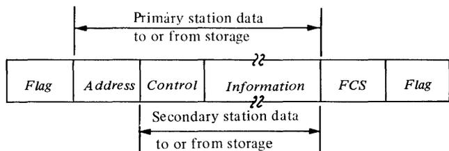
The FCS accumulation starts with the address and includes the FCS received.
