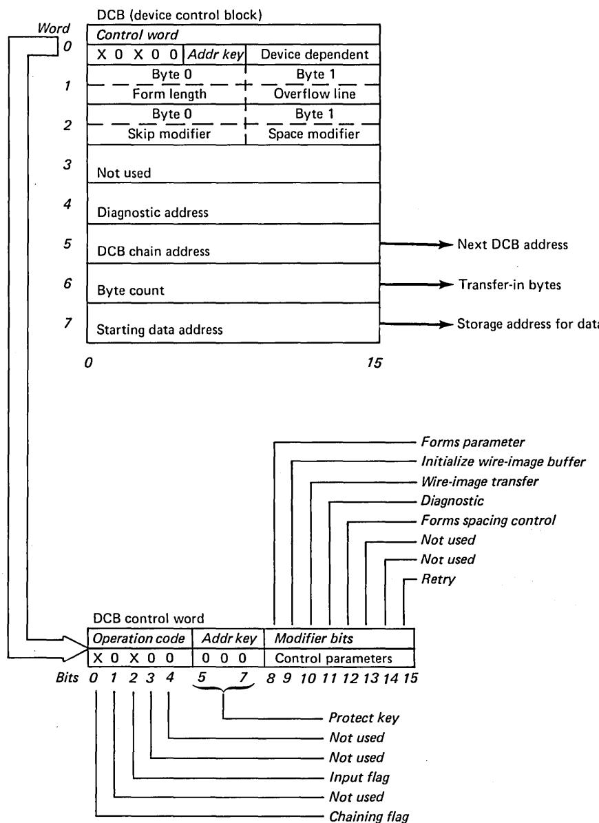
Figure 2-4. Device control block
