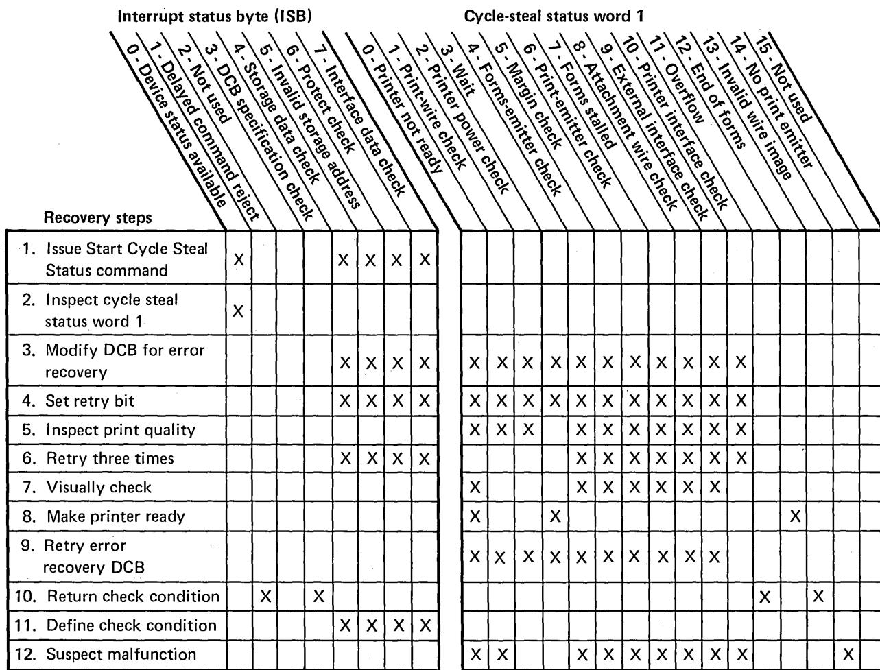
**Figure 2-8.** Error recovery procedure
