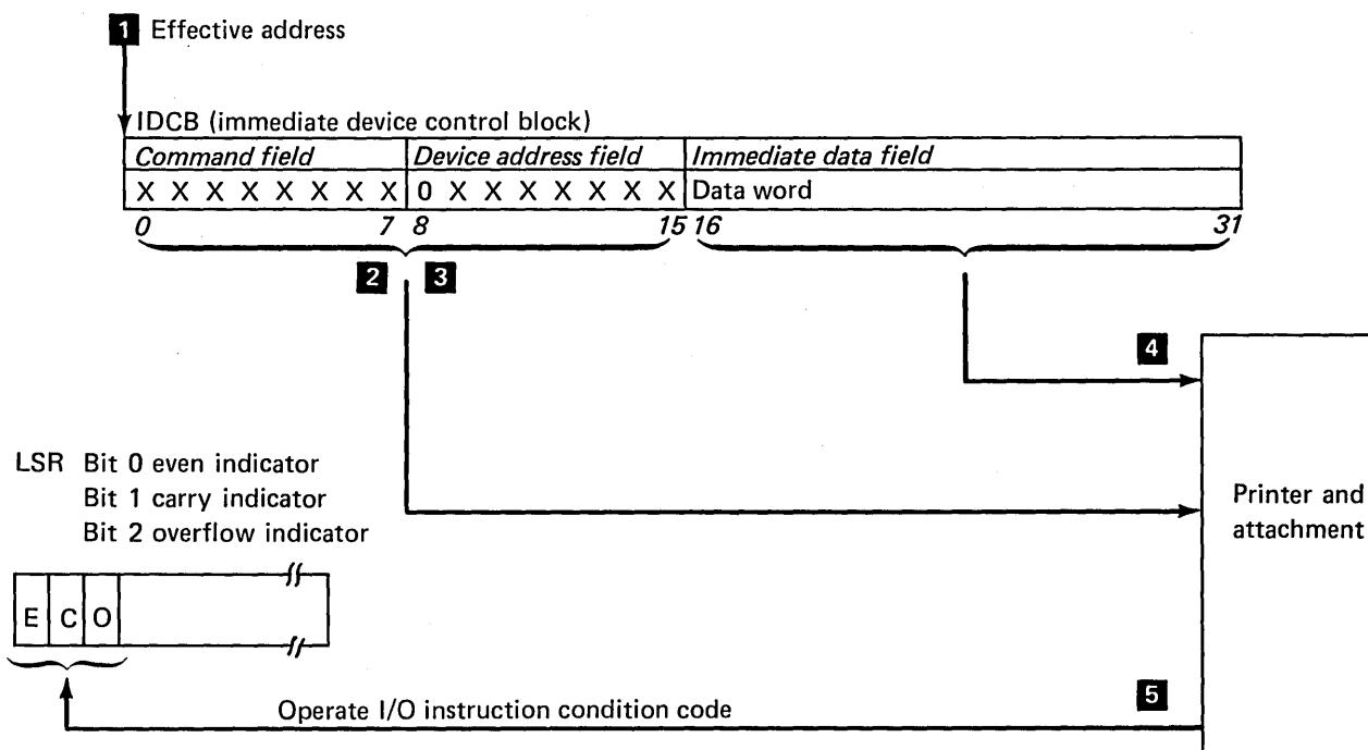
Figure 2-2. Direct program control (DPC) operation
