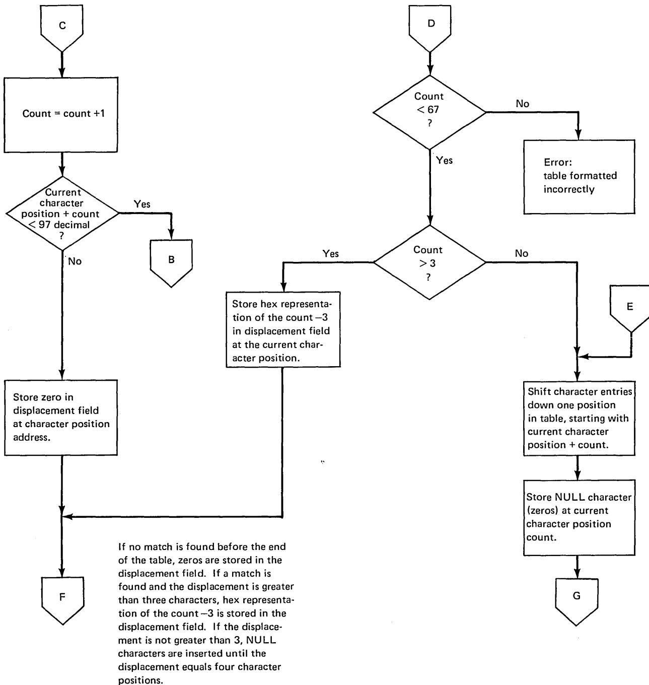
**Figure 2-14 (Part 2 of 3).** Flowchart for calculating displacement fields for characters in the wire-image table
