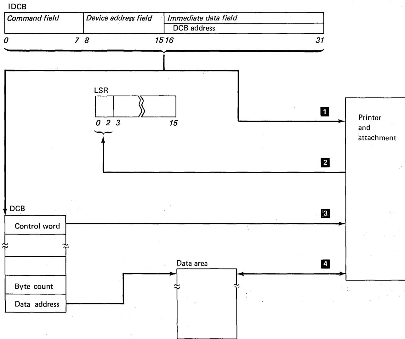
Figure 2-3. Cycle-steal operation
