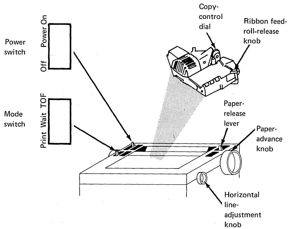
Figure 1-5. Printer controls
