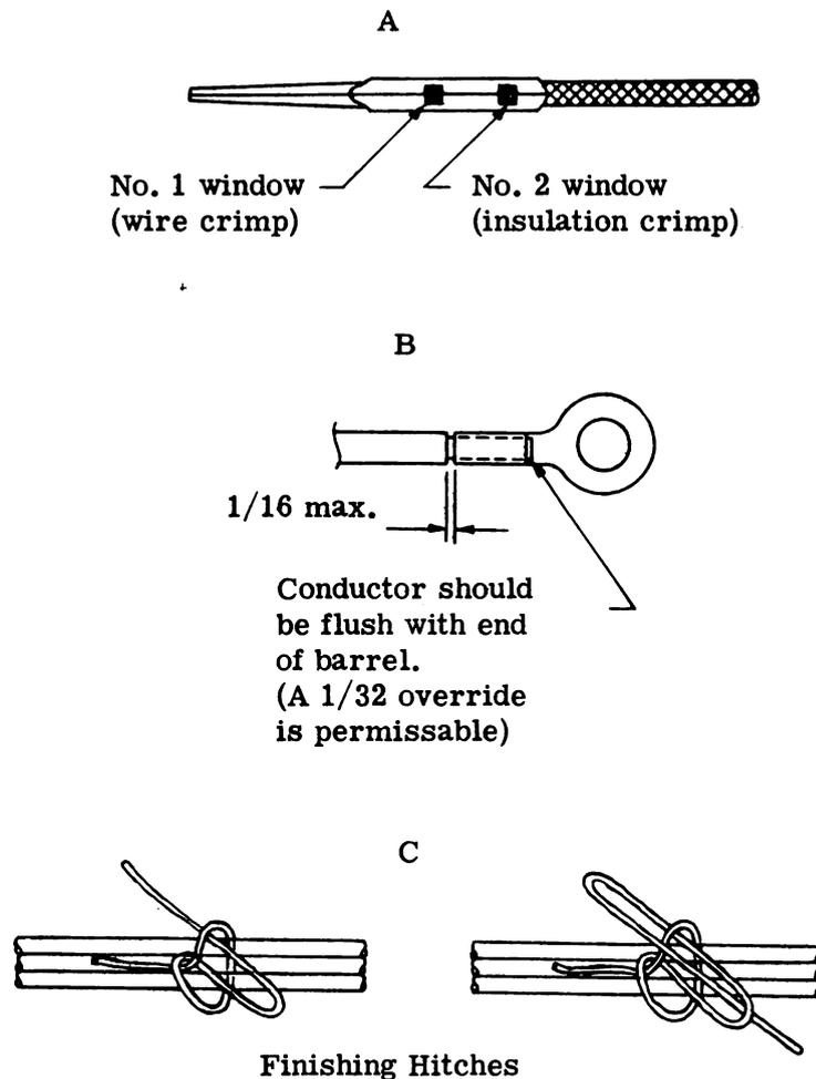
Figure 4-1. Cabling Crimps and Hitches
