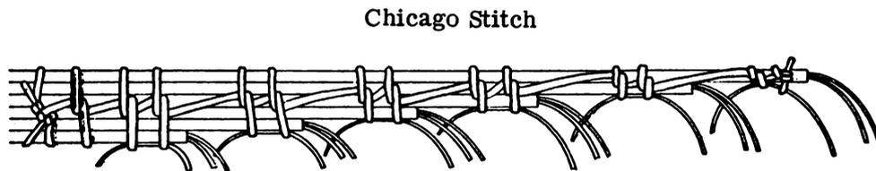
Figure 4-2. Lacing Stitches and Knots
