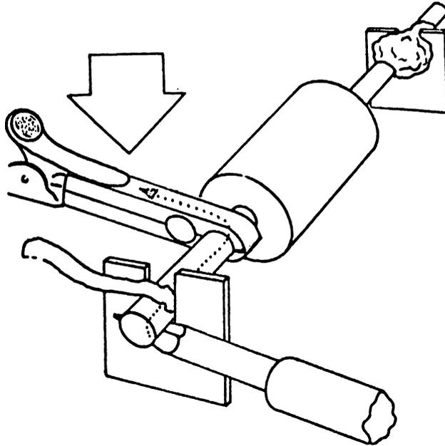
Electrical components that may be adversely affected by excessive heat should be protected by a heat shunt.
