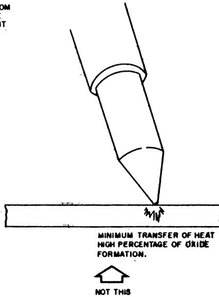
Figure 1-3. Correct and Incorrect Soldering Methods
