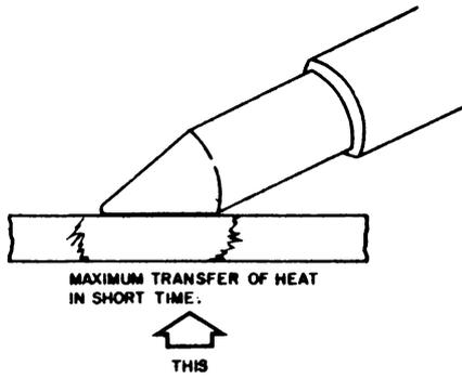
SINCE WE MUST HEAT THE JOINT QUICKLY TO PREVENT OXIDES FROM FORMING...THE POSITION OF THE IRON ON THE WORK IS IMPORTANT
