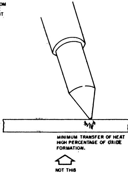
Figure 1-3. Correct and Incorrect Soldering Methods
