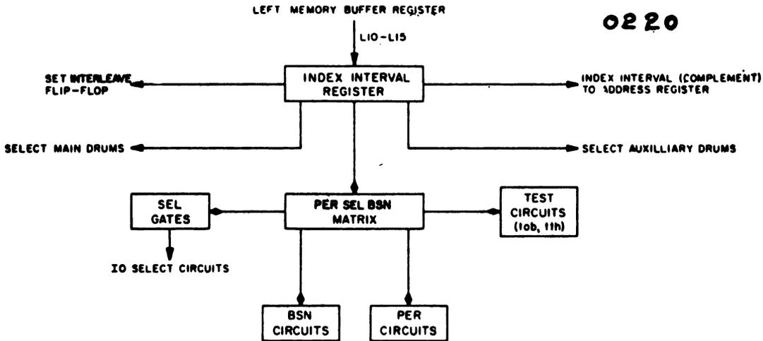
Figure 5-1. Selection Element, Simplified Block Diagram
