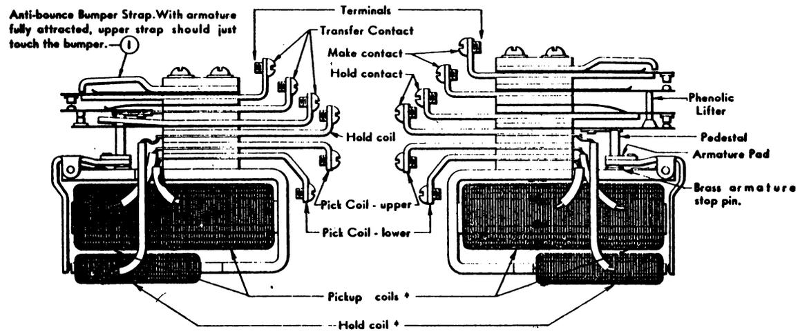
Three - Coil Duo Relay - Double Core
