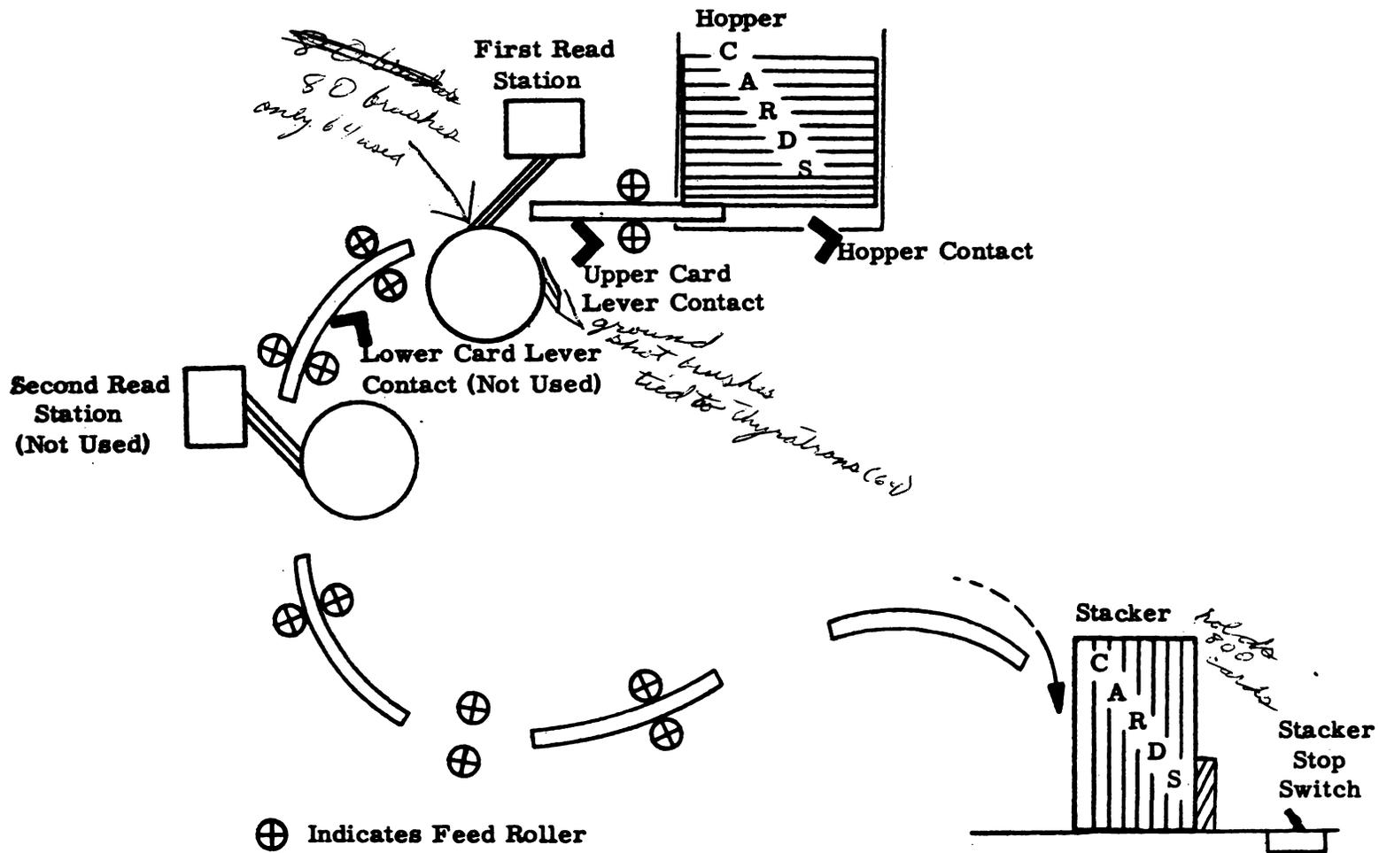
Figure 9, Card Feed Unit Of Card Reader
