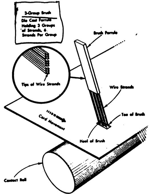
Figure 3-9. Brush, Card, and Contact Roll
