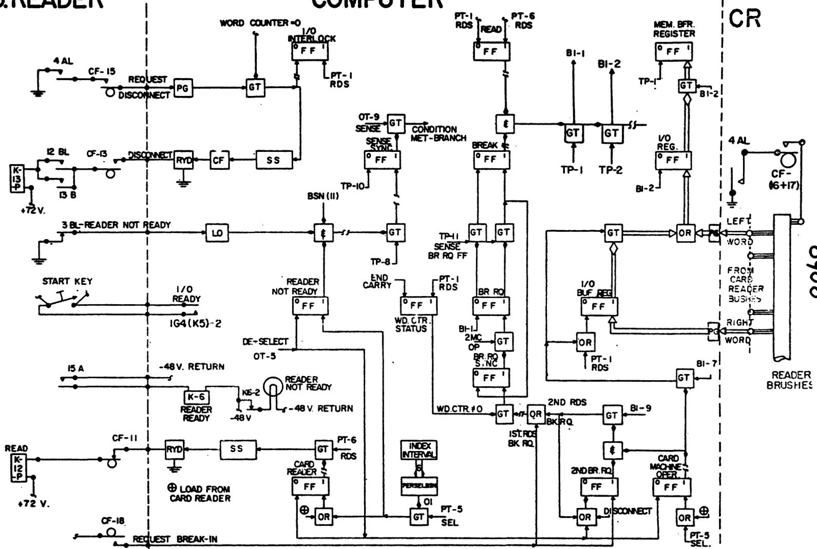
Figure 13, Computer Control Of Card Reader
