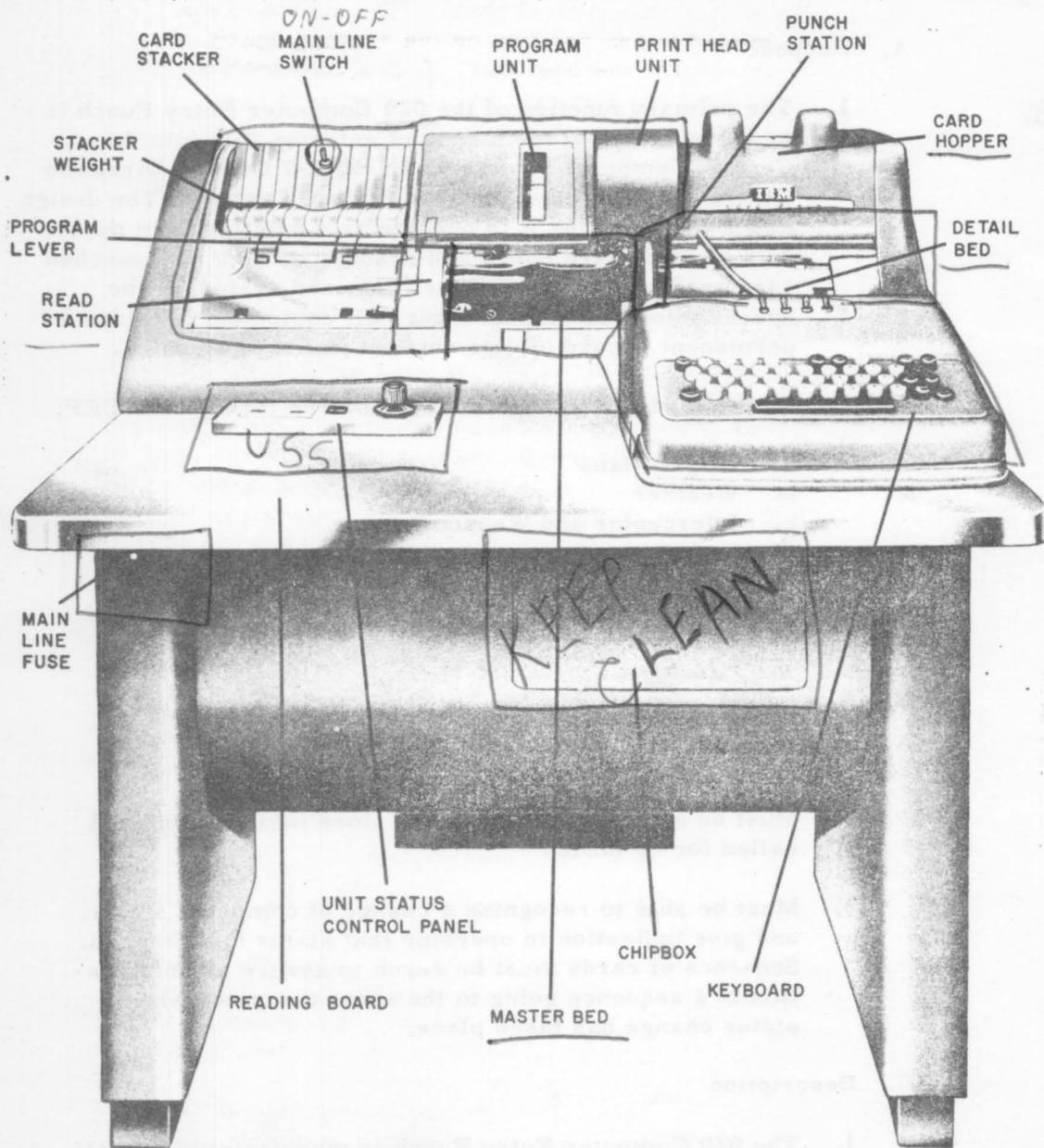
Figure 2-1. 020 Computer Entry Punch, Detailed Front View
