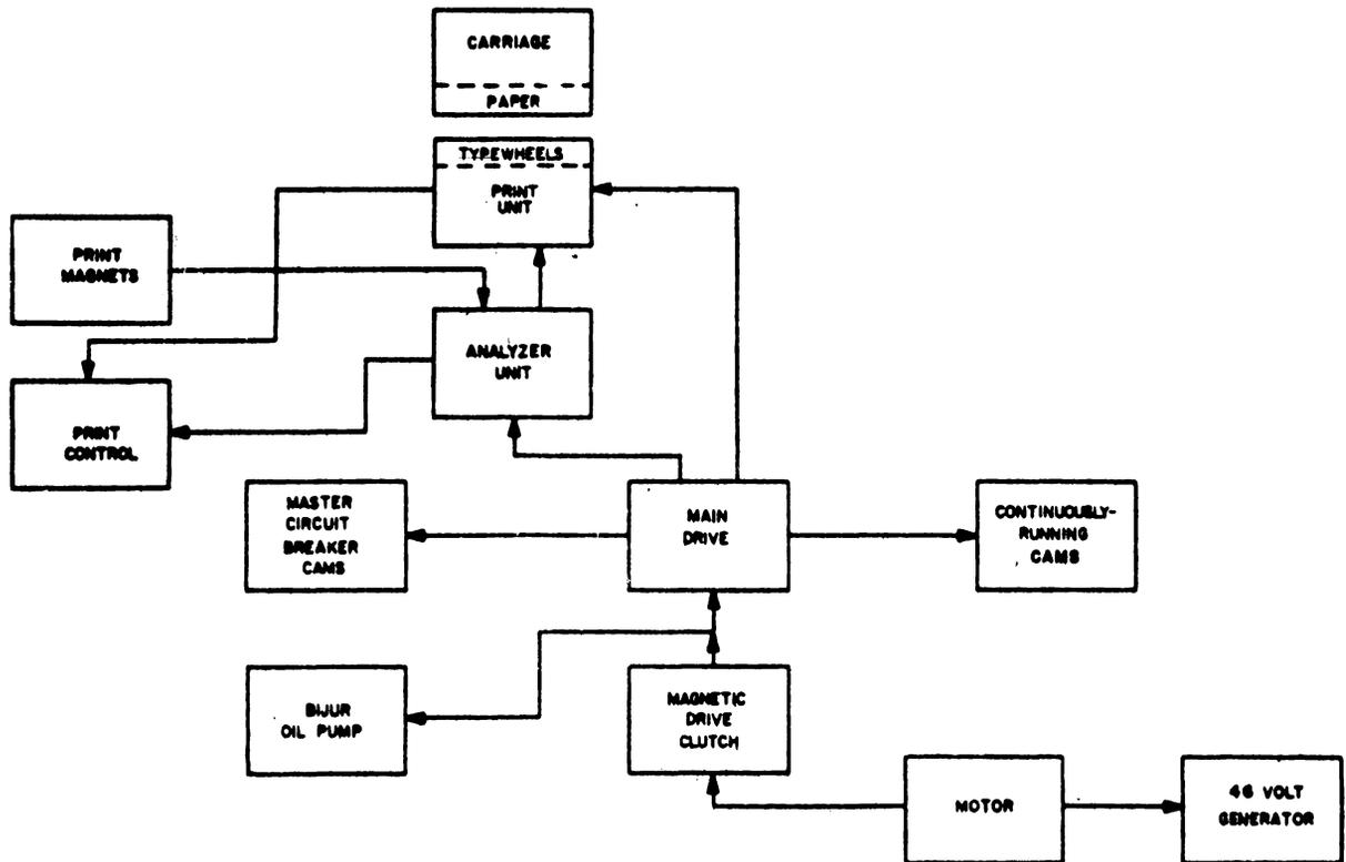
Figure 3-1. 718 Printer Mechanical Drive, Block Diagram
