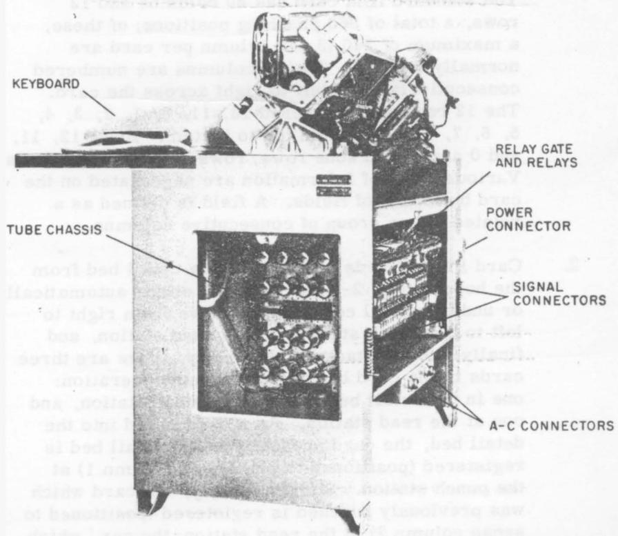
Figure 2-5. Computer Entry Punch, Right Side
