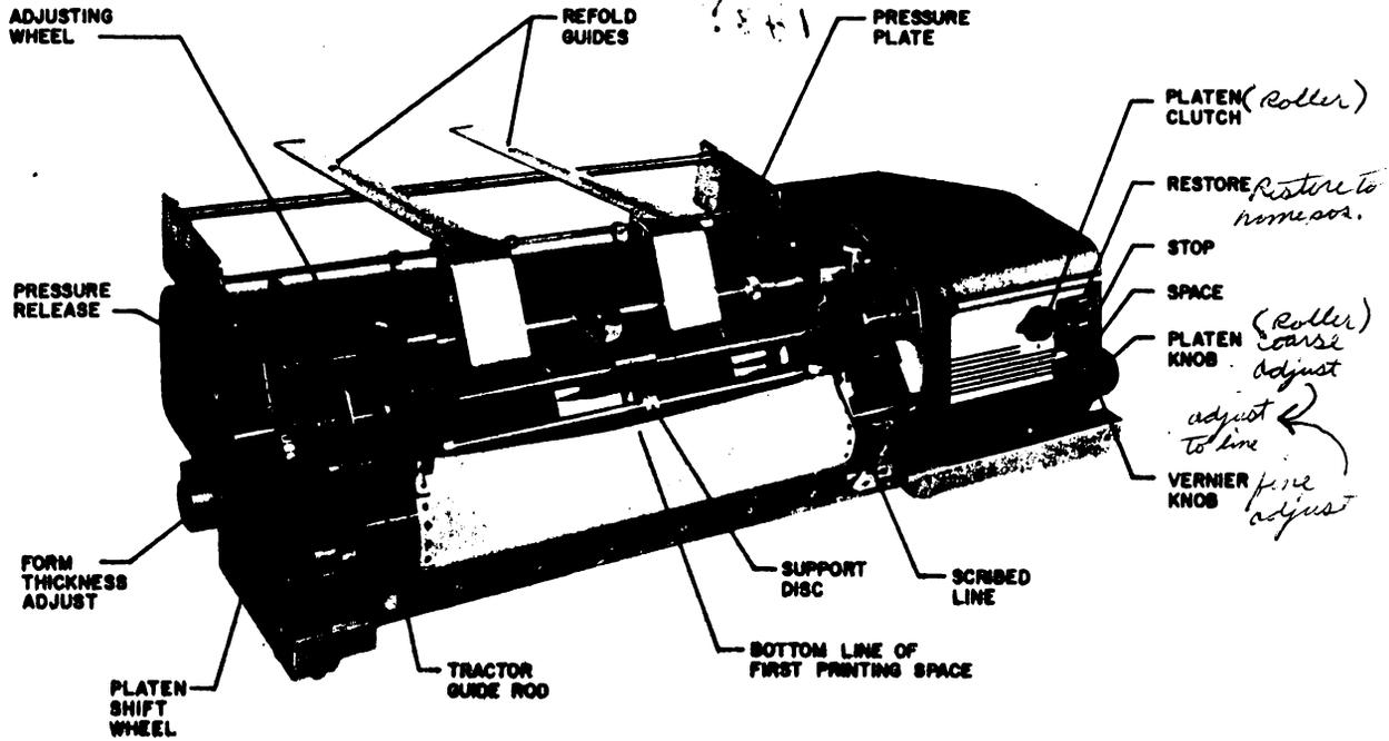
Figure 6-2. Carriage Controls
