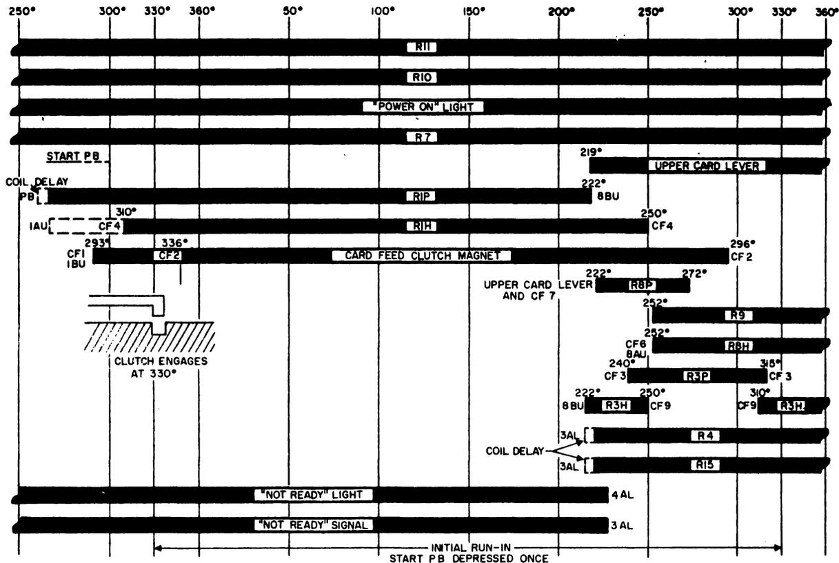
Figure 3-18. Relay Sequence for Initial Run-In
