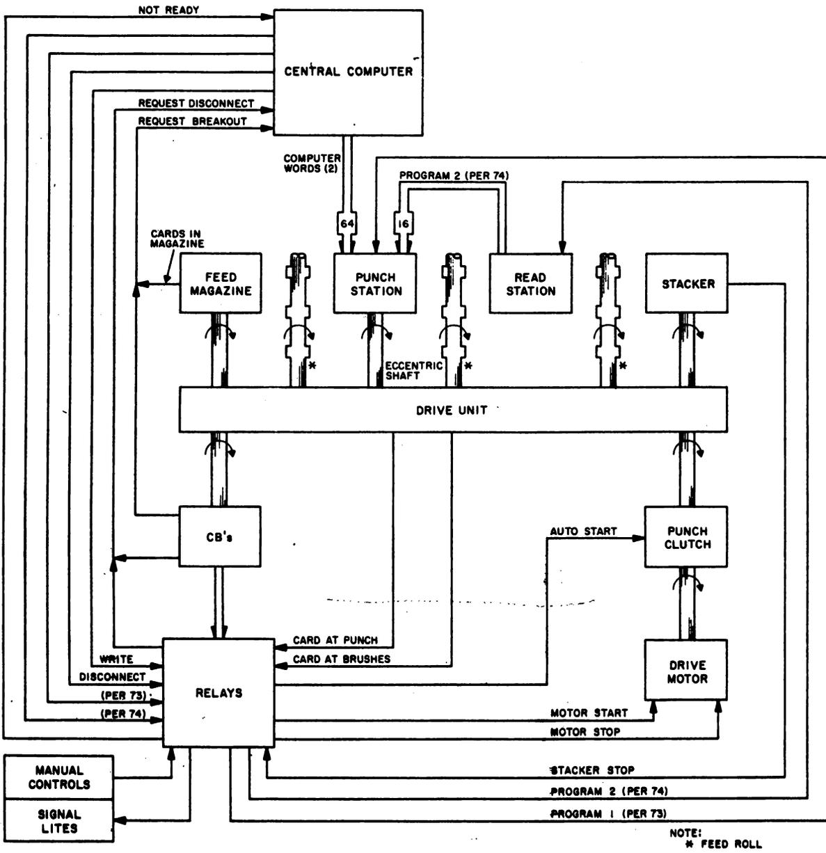
Figure 3-1. 723 Card Recorder, Block Diagram
