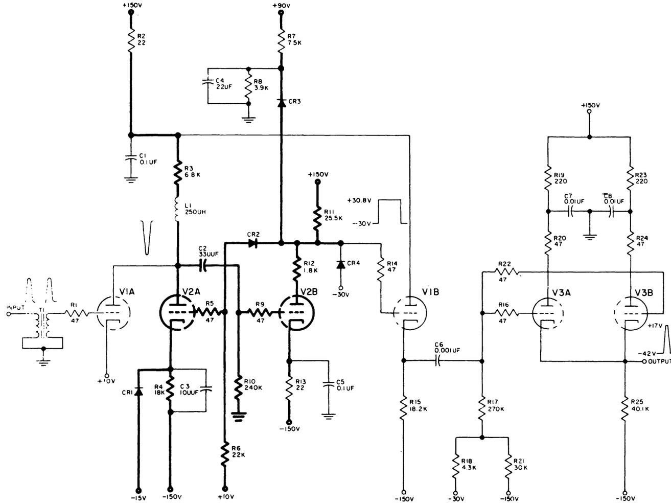
Figure 4-55. Single-Shot, Model D, Schematic Diagram
