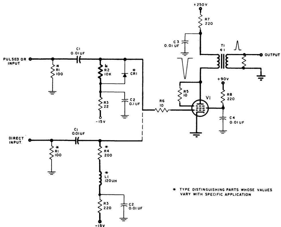
Figure 4-25. Pulse Amplifier, Model B, Schematic Diagram
