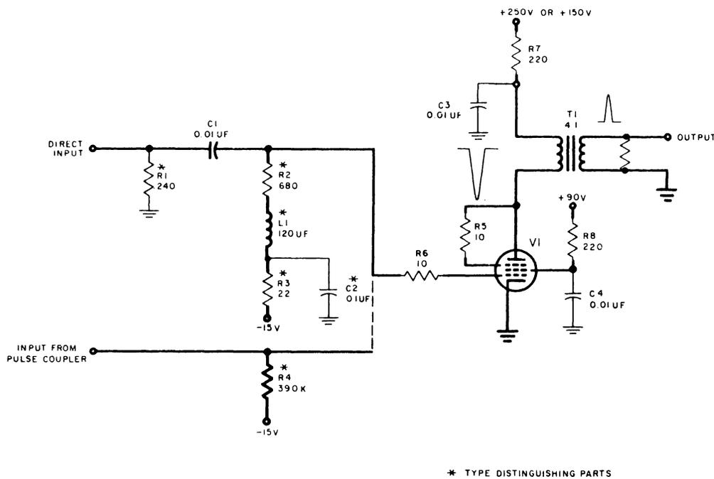
Figure 4-26. Pulse Amplifier, Model C, Schematic Diagram
