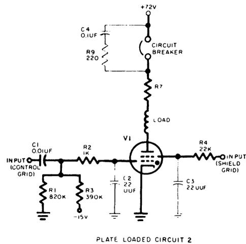
Figure 4-37. Thyratron Relay Driver, Model A, Schematic Diagram
