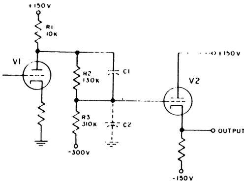
Figure 4-9. Compensated D-C coupling Network, Simplified Schematic Diagram
