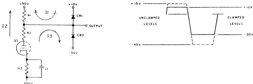
Figure 4-8. Diode Clamped Output Levels, Simplified Schematic Diagram
