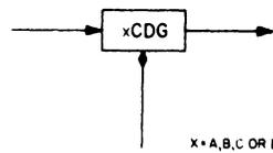
Figure 4-64. Capacitor-Diode Gate, Logic Block Symbol
