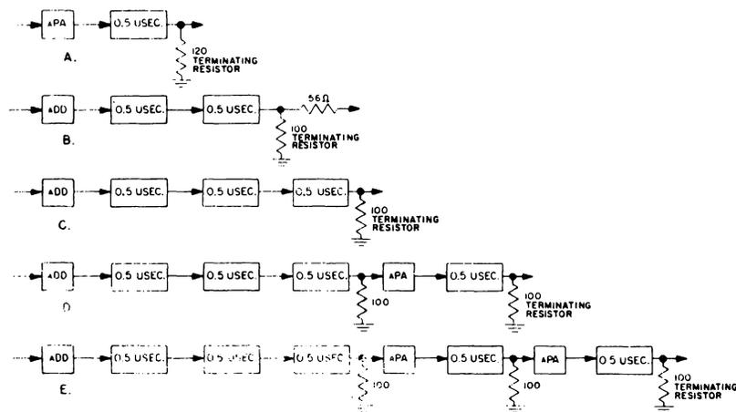
Figure 4-60. Typical Arrangements of Delay Units
