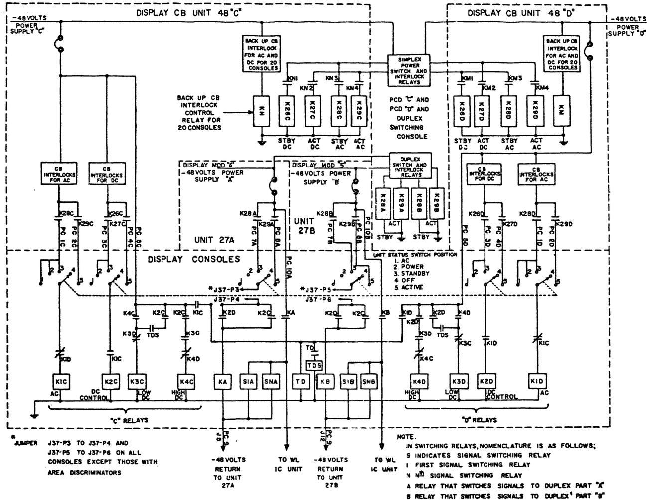
**SIMPLEX POWER AND SIGNAL CONSOLE SWITCHING**
