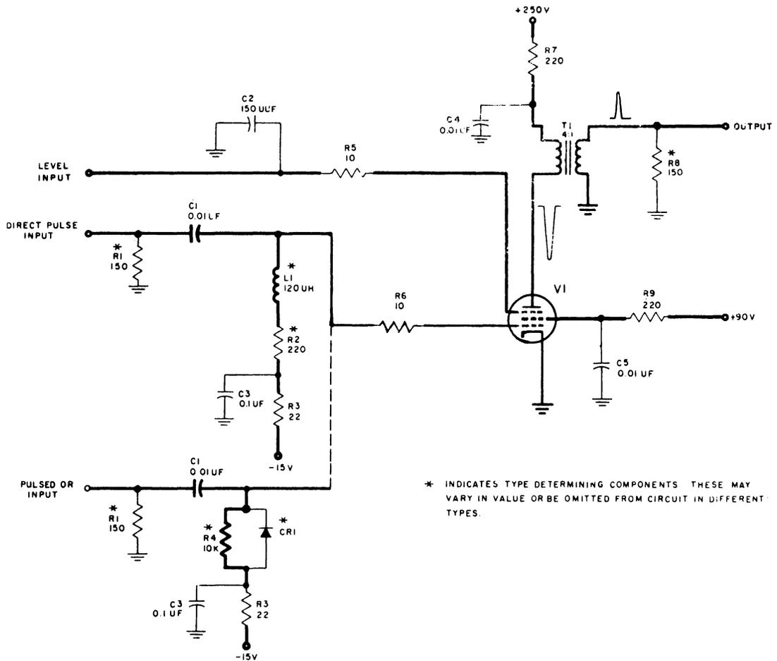
Figure 4-23. Gate Tube, Model A, Schematic Diagram
