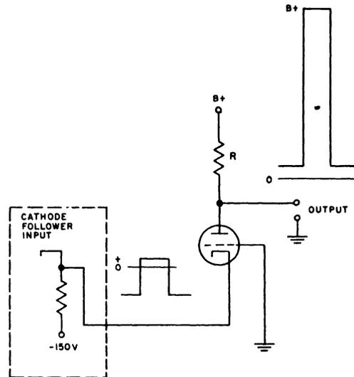
Figure 4-36. Grounded Grid Amplifier, Simplified Schematic Diagram
