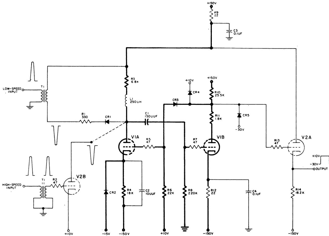
Figure 4-53. Single-Shot, Model B, Schematic Diagram
