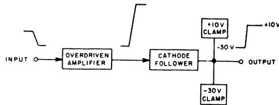
Figure 4-42. D-C Inverter, Simplified Block Diagram
