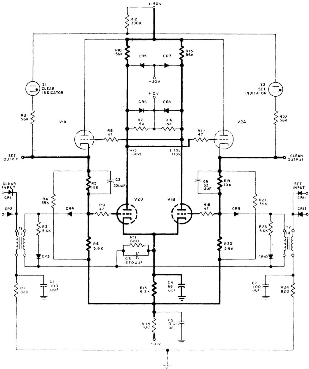
Figure 4-47. Flip-Flop, Model A, Schematic Diagram
