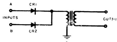
Figure 4-20.  $Y_{OR}$  Circuit Schematic Diagram
