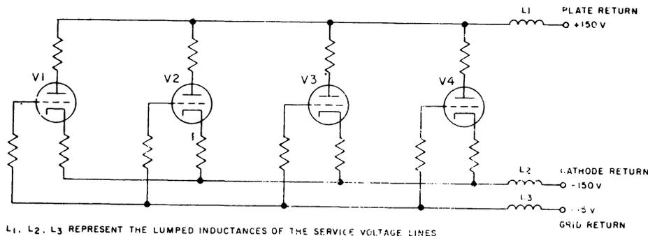
Figure 4-6. Common Return Paths, Simplified Schematic Diagram
