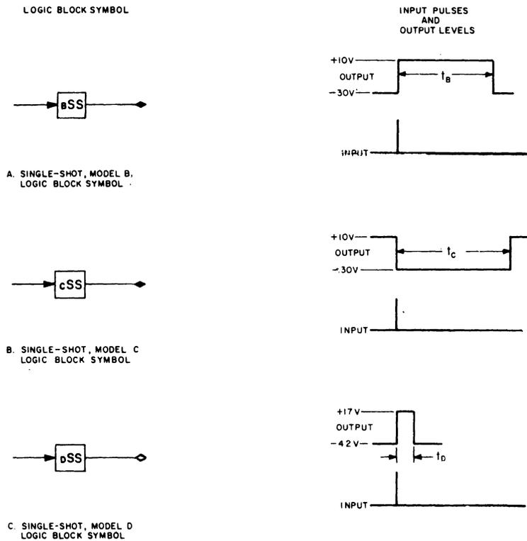
Figure 4-48. Single-Shot, Logic Block Symbols and Output Waveforms
