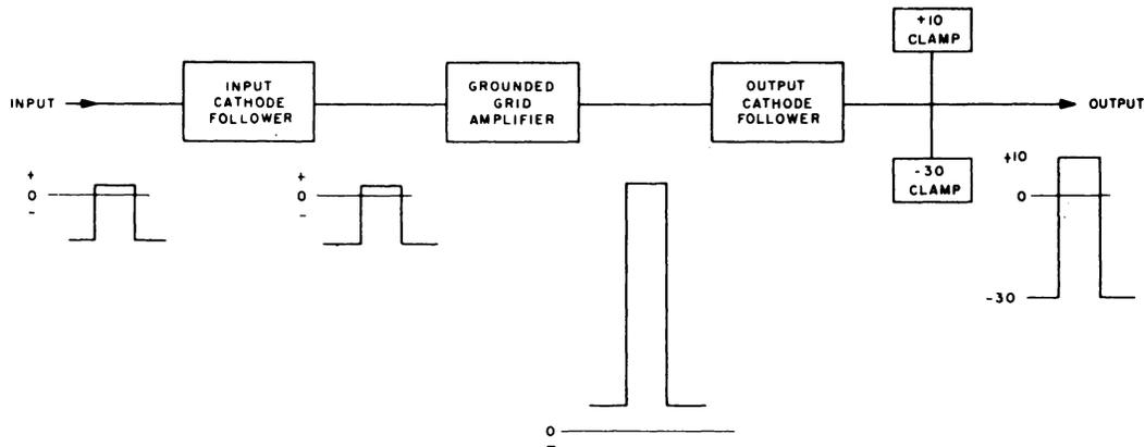
Figure 4-35. D-C Level Setter, Block Diagram
