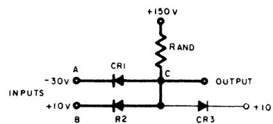
Figure 4-16. Two Way AND Circuit
