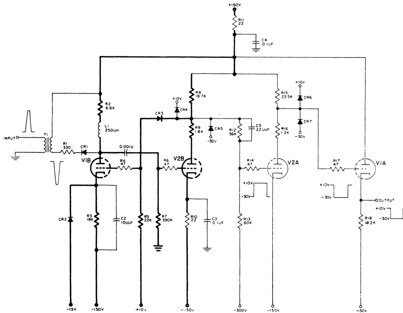
Figure 4-54. Single-Shot, Model C, Schematic Diagram
