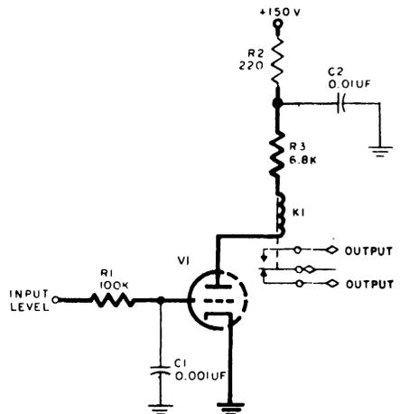
Figure 4-40. Vacuum-Tube Relay Driver, Model B, Schematic Diagram
