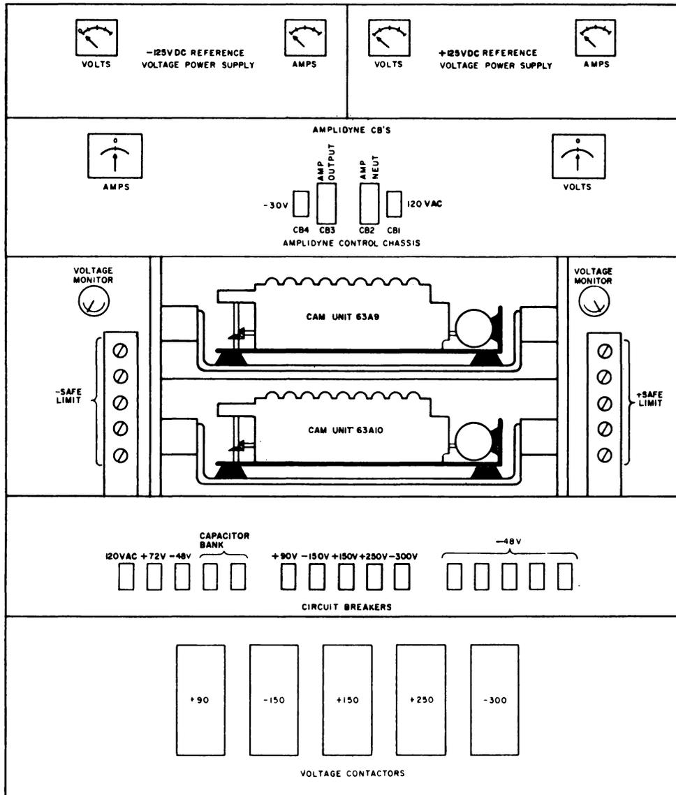
Figure 7-30. Controls and Indications, Module A, PCD Unit 63
