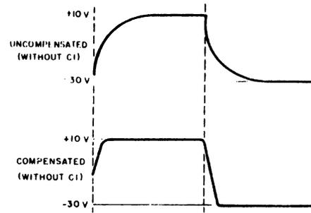
Figure 4-10. Output Waveform (V2 in Figure 4-9.)
