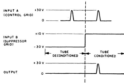
Figure 4-22. Gate Tube, Model A, Input-Output Relationship
