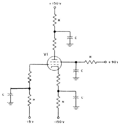
Figure 4-7. RC Decoupled Returns, Simplified Schematic Diagram
