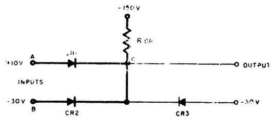
Figure 4-18. Two-Way OR Circuit,
