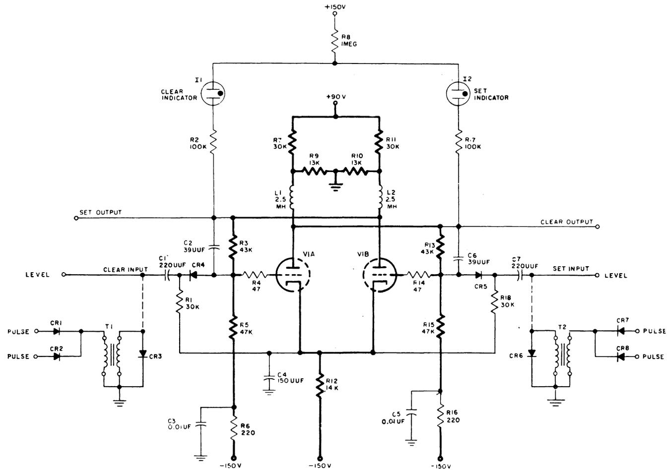
Figure 4-45. Flip-Flop, Model B, Schematic Diagram
