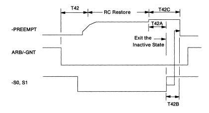
Figure 1-17. Exiting from the Inactive State
