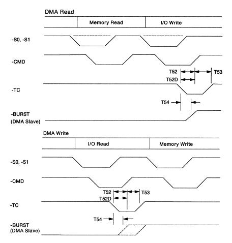
Figure 1-52. Burst DMA Transfer (DMA-Controller Terminated)
