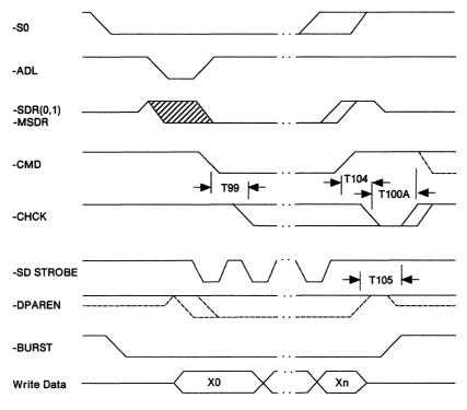
Figure 1-82. Channel Check - Streaming Data Write Cycle
