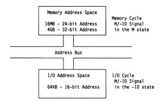
Figure 1-3. I/O and Memory Address Space
