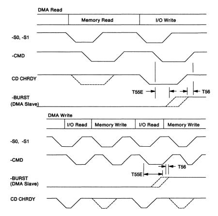
Burst DMA Transfer (DMA-Slave Terminated - Synchronous-Extended Cycle, 300 ns)
