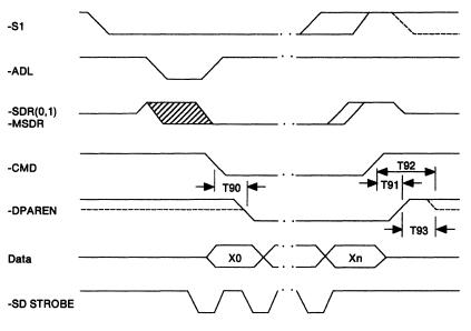
Figure 1-69. Data Parity Read Cycle - Streaming Data Transfer
