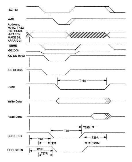
Figure 1-27. Asynchronous Extended Cycle (≥ 300 ns)
