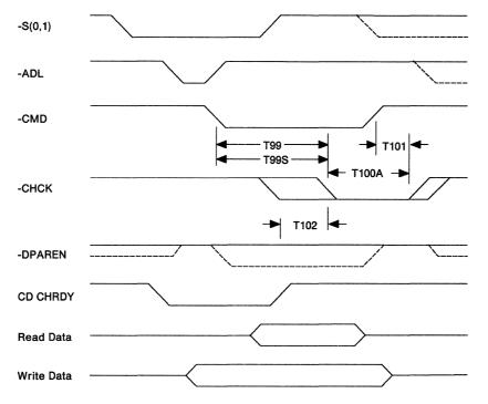
Figure 1-78. Channel-Check - Extended Cycle
