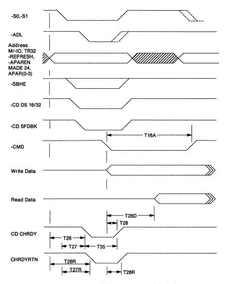
Figure 1-25. Synchronous-Extended Cycle (300 ns Minimum)
