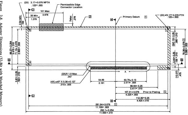
Figure 2-8. Adapter Dimensions (32-Bit with Matched Memory)
