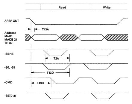
The following are the timing parameters for the first cycle after ARB/-GNT goes to the -GNT state.
