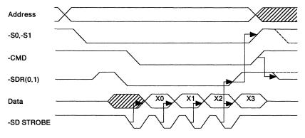
Figure 1-42. Slave-Terminated Streaming Data Cycle
