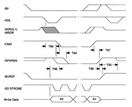
Figure 1-72. Data Parity Write Cycle - Streaming Data Transfer
