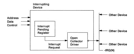
Figure 1-60. Typical Adapter Interrupt Sharing Implementation
