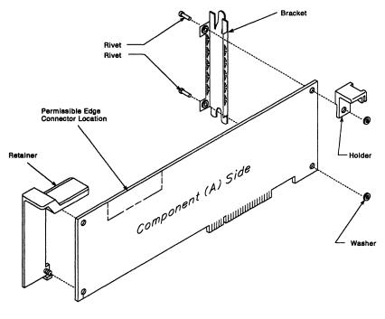
Materials: Holder and Retainer - Polycarbonate UL 94 V-0 Bracket - AISI Type 302 1/4 Hard Stainless Steel
