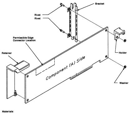
Holder and Retainer - Polycarbonate UL 94 V-0 Bracket - AISI Type 302 1/4 Hard Stainless Steel
