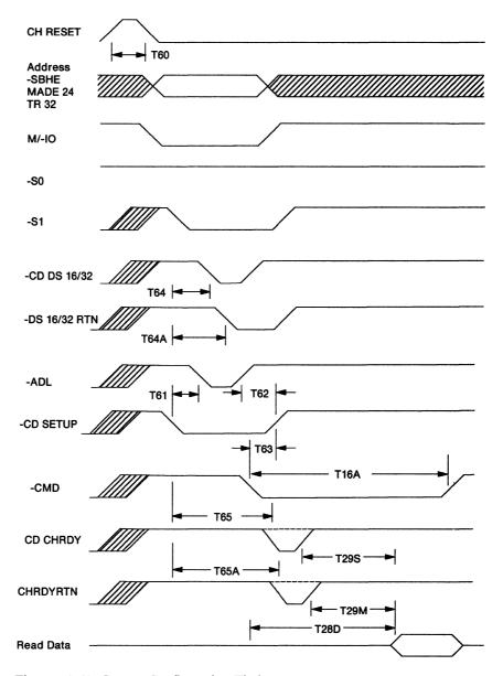
Figure 1-65. System Configuration Timing
