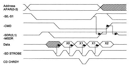
Figure 1-40. Master-Terminated Streaming Data Cycle
