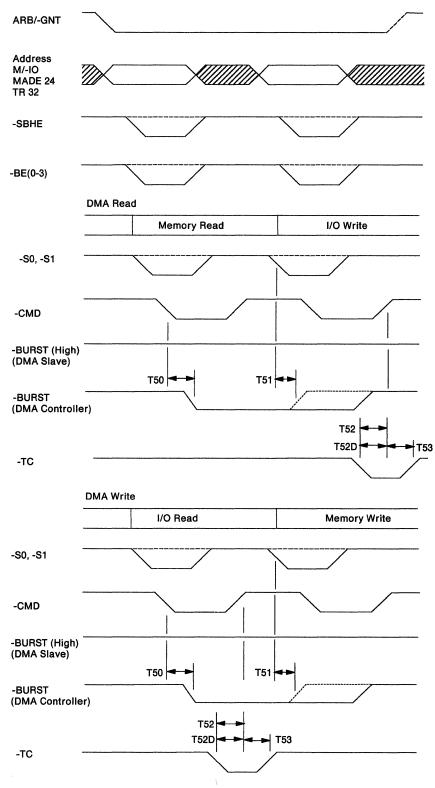
Figure 1-50. Single DMA Transfer (DMA-Controller Controlled)
