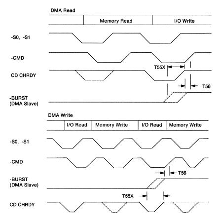
Figure 1-58. Burst DMA Transfer (DMA-Slave Terminated - Asynchronous-Extended Cycle, ≥300 ns)
