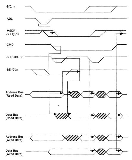
Figure 1-37. 64-Bit Streaming Data Cycle Overview
