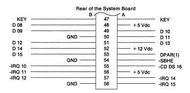
The following are the signals and voltages assigned to the channel connector 16-bit section.
