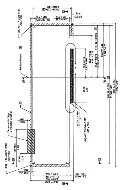
Figure 2-6. Adapter Dimensions (32-Bit)
