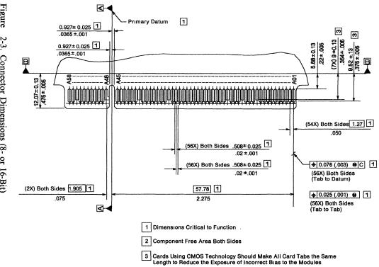
Figure 2-3. Connector Dimensions (8- or 16-Bit)
