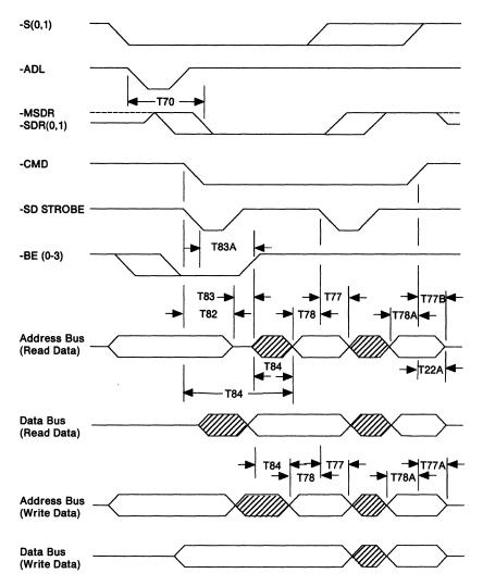
Figure 1-48. Streaming Data Clocking (64-Bit)
