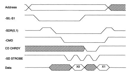
Figure 1-41. Master-Terminated Streaming Data Cycle (Slave Not Ready)
