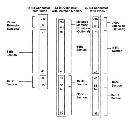
Figure 1-85. Micro Channel Connectors
