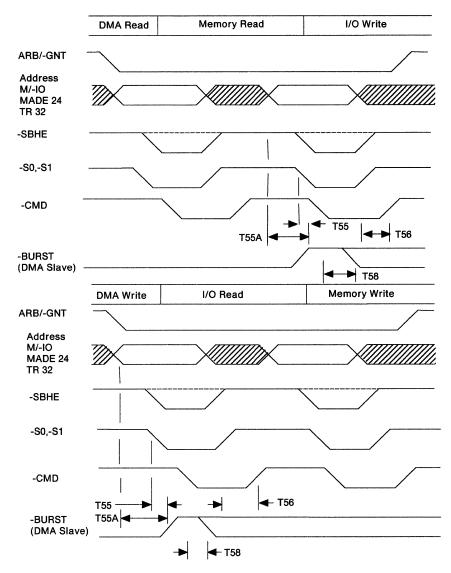
Burst DMA Transfer (DMA-Slave Terminated - Default Cycle, 200 ns)
