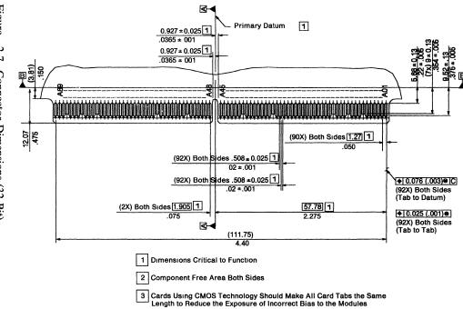
Figure 2-7. Connector Dimensions (32-Bit)
