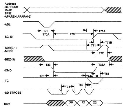
Figure 1-43. Streaming Data Cycle
