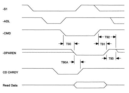
Figure 1-67. Data Parity Checking Read Cycle - Basic Transfer
