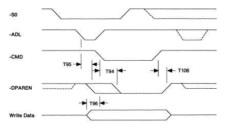
Figure 1-70. Data Parity Checking Write Cycle - Basic Transfer
