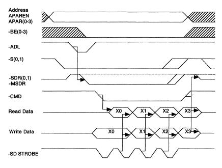
X0, X1, X2, and X3 represent a data transfer of 16 or 32 bits. Figure 1-36. 16- and 32-Bit Streaming Data Cycle Overview
