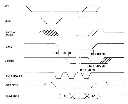
Figure 1-80. Channel Check - Streaming Data Read Cycle
