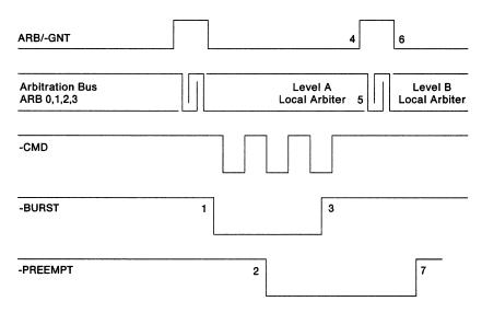
Figure 1-16. Preempted Burst Transfer
