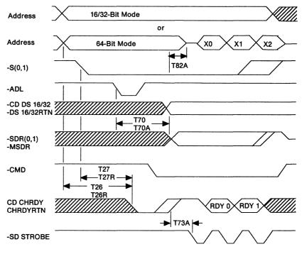
Figure 1-44. Streaming Data Cycle - Deferred Start
