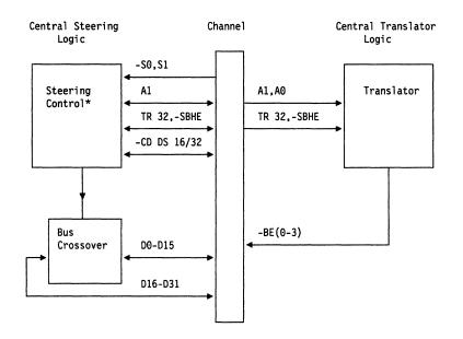
The following block diagram shows the implementation of data steering.
