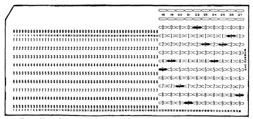
Figure 20-Mark Sensed Card. This card has been mark sensed with the numbers "5479024218." This number can be punched into a field of the same card by passing it through the document originating machine. No key punching is necessary.
