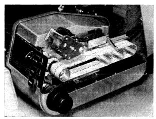
Figure 34–IBM Carriage Tape in Operating Position. Continuous punched paper tape governs the feeding of continuous forms through the tabulator. Holes punched in channels 1, 5, and 12 are read by carriage brushes and transmitted internally to the control panel where wiring starts and stops skipping and ejecting. (Courtesy of International Business Machines Corporation)
