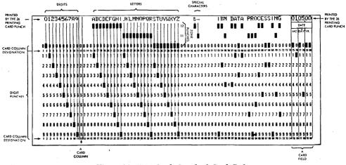
Figure 96-IBM Card-Standard Card Code
