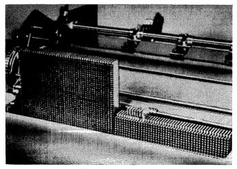
Figure 56–Print Unit IBM Type 402
