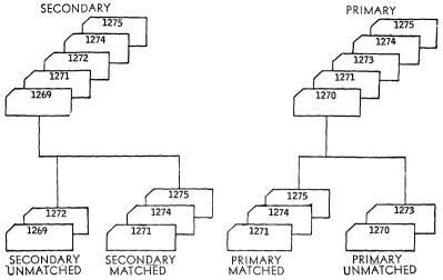
Figure 29-Matching Operation on the Collator. Cards with the same employe punched in them drop into the two center stackers. Cards in either feed that do not have a corresponding number in the other feed drop into the outside stackers.
