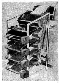
Figure 64–Power Feed Vertical Separator. Multicopy report is placed in center section. One carbon winds around a spindle and one copy folds in a side rack. The other copies fold in the opposite side rack. These copies are then placed in the center section and the process is repeated until all carbons have been removed. (Reprinted by permission of The Standard Register Co.)
