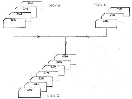
Figure 27-Merging. Decks A and B are merged together to form Deck C. Numbers written on the cards indicate employe number which is punched in the cards.
