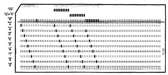
Figure 5-IBM Punched Hole Codes. Zone portion of card is above line; numeric portion below it. Names of the 12 horizontal rows are indicated at left.
