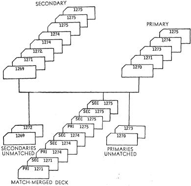
Figure 30-Match-Merging Operation on the Collator. Same as the matching operation except cards with corresponding numbers are merged together in one of the center stackers.
