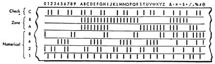
Figure 101-Magnetic Tape-Seven-Bit Alphameric Code
