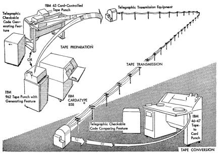
Figure 79-Machine-to-Machine Communication
