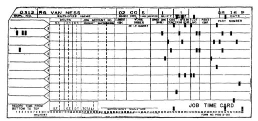
Figure 21–IBM Type 552 Interpreter Printing. Job time cards are prepunched and distributed to all direct workers in the company each day to be used to record their time spent on each job. The IBM 552 Interpreter is used to print the top line with the data that is punched in the card so that it can be read by human beings.
