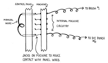
Figure 18-Circuit Completed Between Control Panel and Machine
