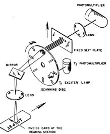
The scanner makes a rapid vertical scan. Due to document motion (or in some cases the motion of a sweep mirror) the vertical scans progress across the character. Output of the scanner is a video signal.
