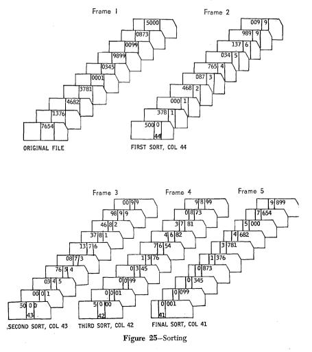
name field might comprise 20 columns which would require 40 sorts. The sorting can be accomplished in twelve passes by sorting the initials and the first four positions of last name.
