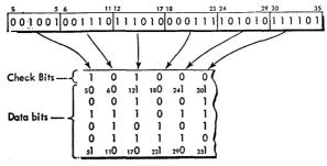
Figure 102-Magnetic Tape-Binary System
