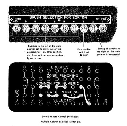
Figure 46. Control Panel Wiring - Zero Elimination
