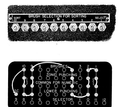
Selection of a predetermined digit occurring in any one or more of brush positions, 1, 2, 4, 9, or 10. Selecting commutator contact bar our for digit value desired. All others IN. All brush selection for sorting switches set to SELECT. Zero-eliminate and MCS control switches - OFF.
