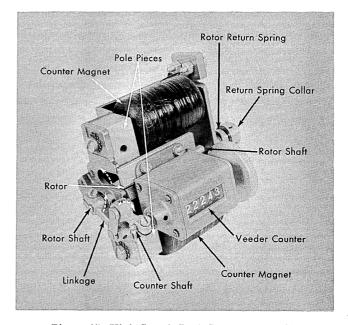
Figure 37. High Speed Card Counter Assembly
