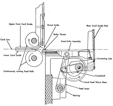
Figure 17. Feed Knife Operation
