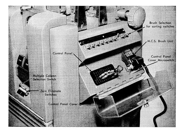
Figure 43. Multiple Column Selection Device, Type 82
