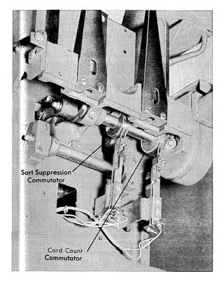
Figure 36. Auxiliary Card Count and Sort Suppression Commutators
