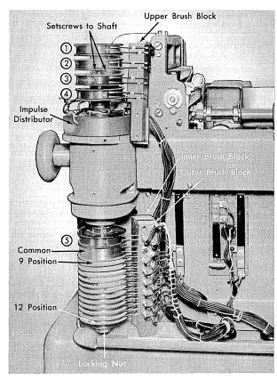
Each of the upper five commutators are individually adjustable since each one is fastened to the shaft by means of set screws. Two brushes ride on each of the 17 commutator surfaces to make and break contact at timed intervals.
