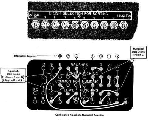
Zero eliminate control switches OFF Multiple column selection switch on All brush selection switches set to SELECT
