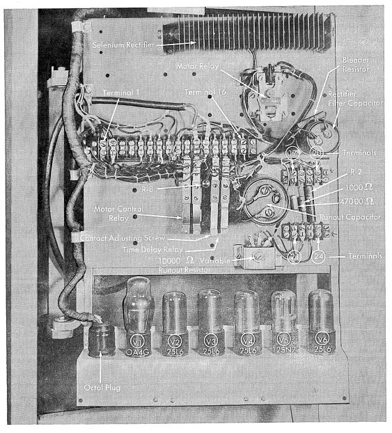
Figure 22. Relay Gate and Electronic Chassis
