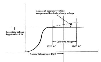
Figure 60. Schematic of Filament Transformer Output
