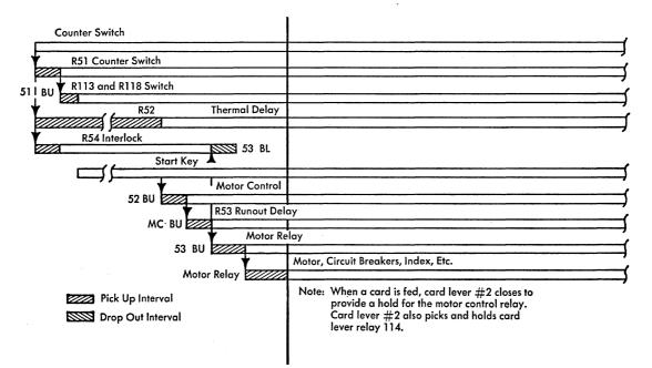
Figure 62. Conditioning Circuits (Sequence Chart)
