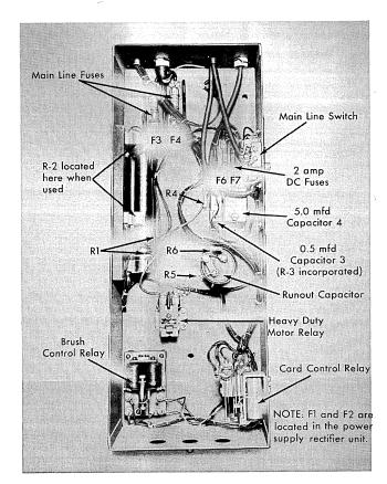
Figure 33. Type 75 Sorting Relay Cabinet
