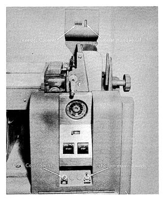
Figure 35. Auxiliary Card Counting Device
