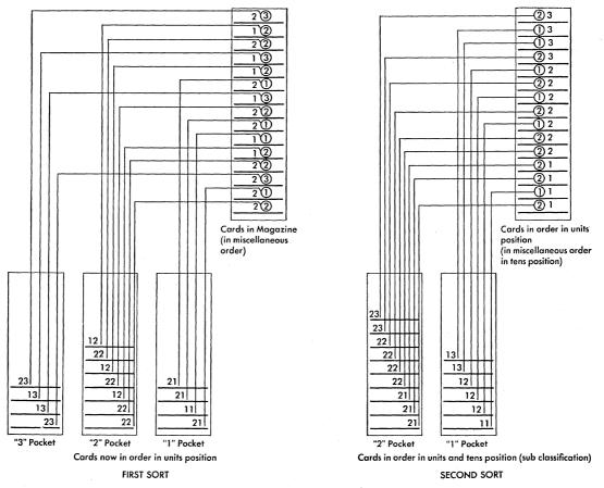
Figure 2. Principle of Sorting
