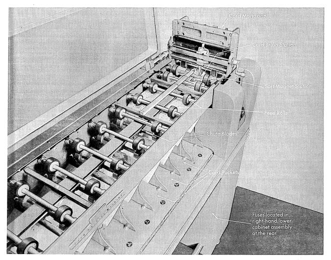
Figure 1. Card Transport Through the Machine
