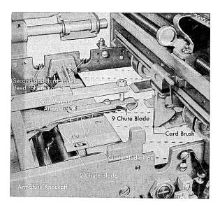
Figure 5. Sensing the Card
