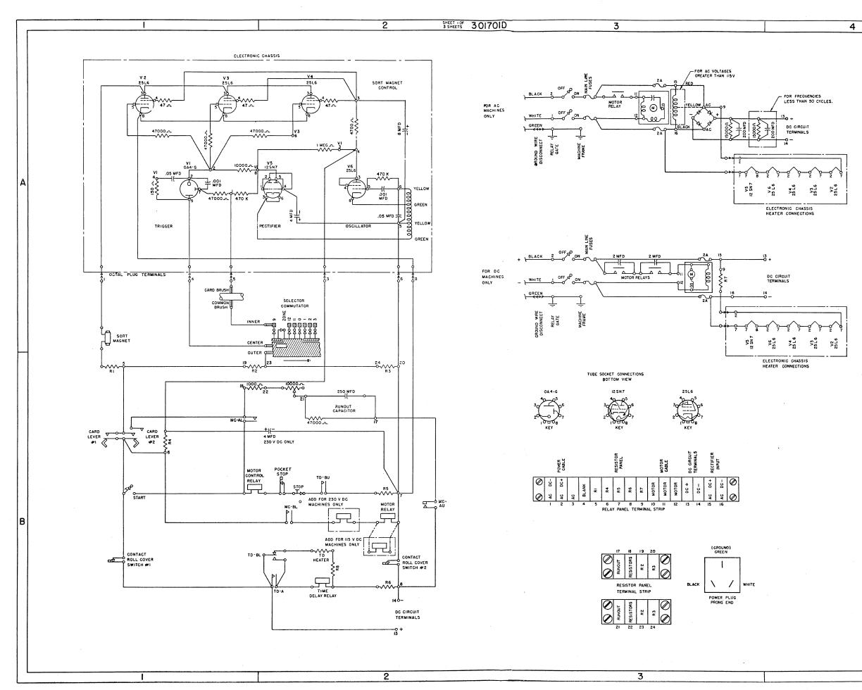
Figure 66. IBM 82 Wiring Diagram and Time Chart
