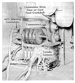
Figure 47. Internal Controls - MCS Device
