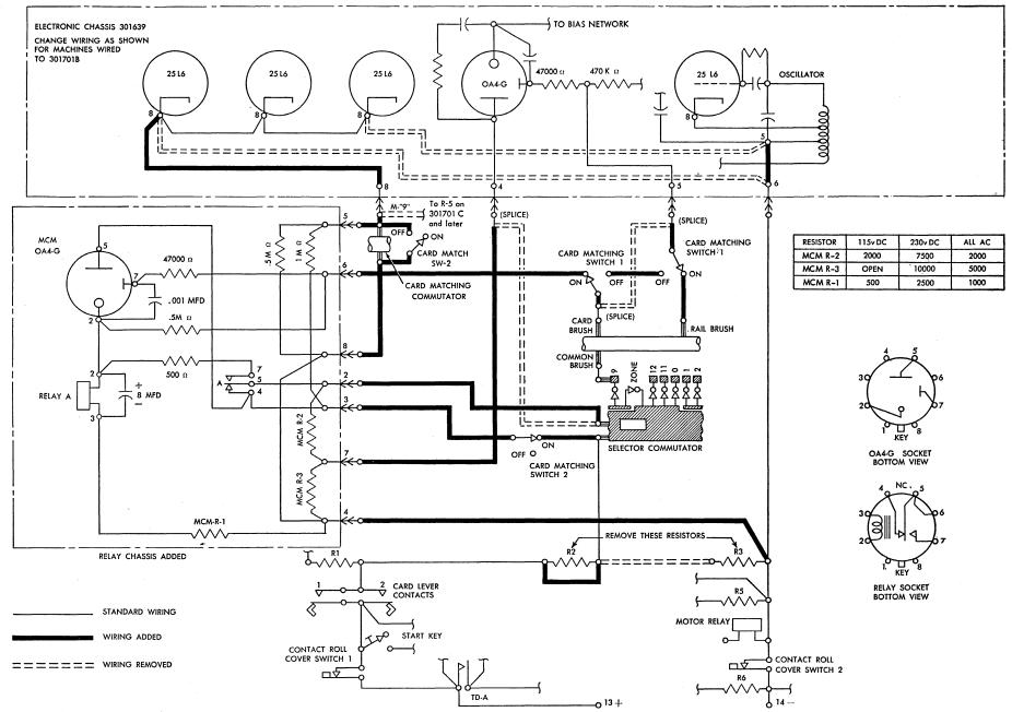
Figure 41. Wiring Diagram - Card Matching, Type 82
