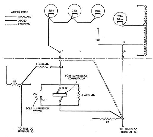
Figure 39. Wiring Diagram - Sort Suppression Device, Type 82
