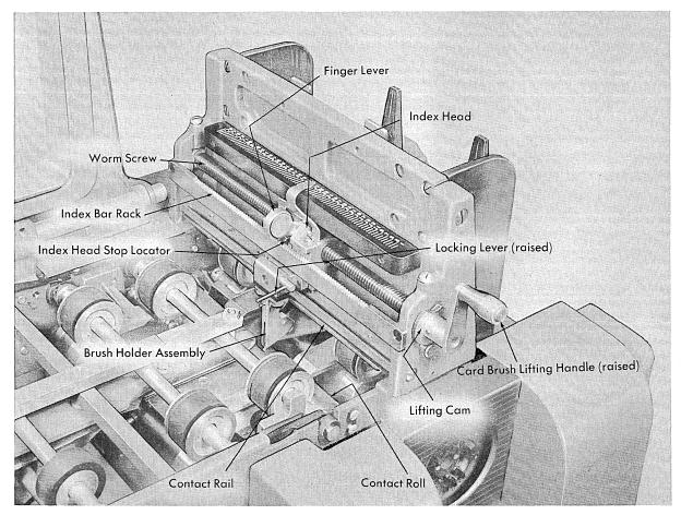
Figure 9. Removing the Card Brush Assembly
