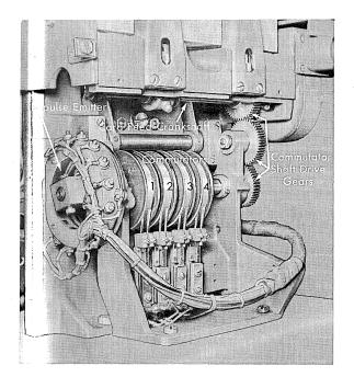
Figure 52. Internal Controls - Group Sorting Device
