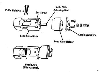
Figure 18. Feed Knite Slide Assembly
