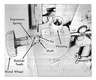
Figure 14. Declutching Hand Wheel
