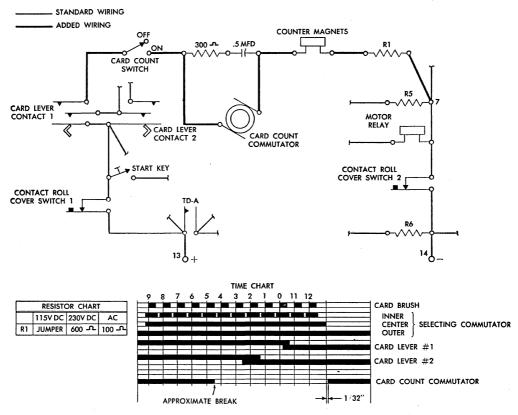
Figure 38. Wiring Diagram - Auxiliary Card Count Device, Type 82
