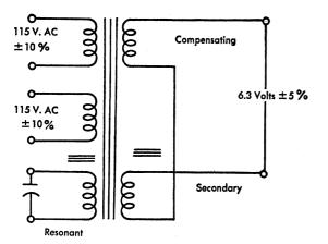
Figure 58. Filament Voltage Transformer (Schematic)
