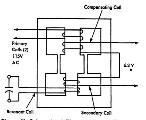
Figure 59. Schematic of Filament Voltage Transformer
