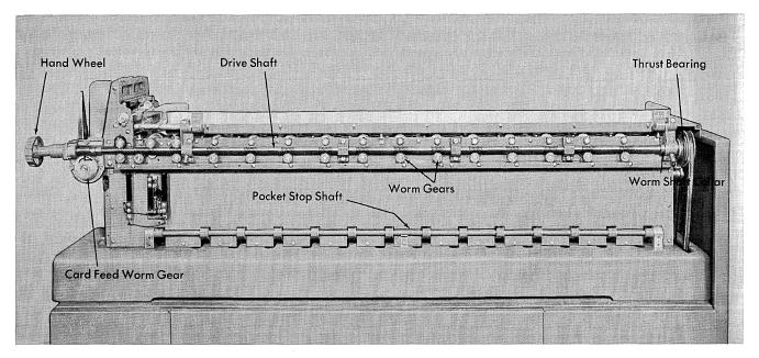
Figure 13. Main Drive Shaft and Pocket Stop Shaft
