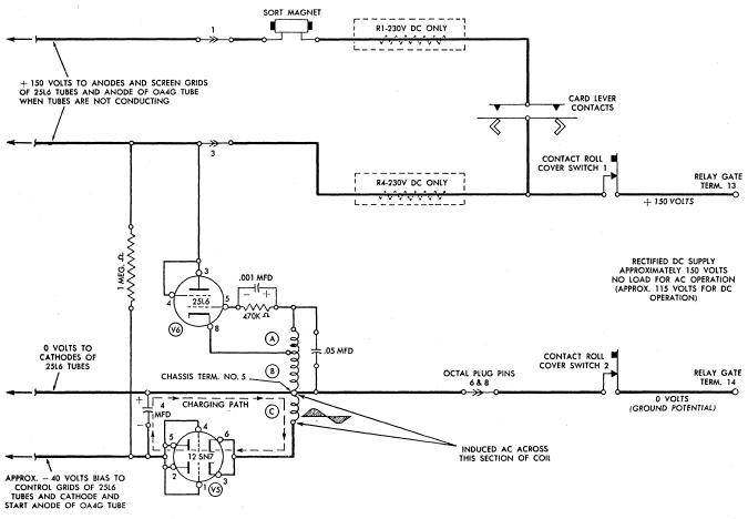
Figure 24. Schematic of Oscillator and Rectifier
