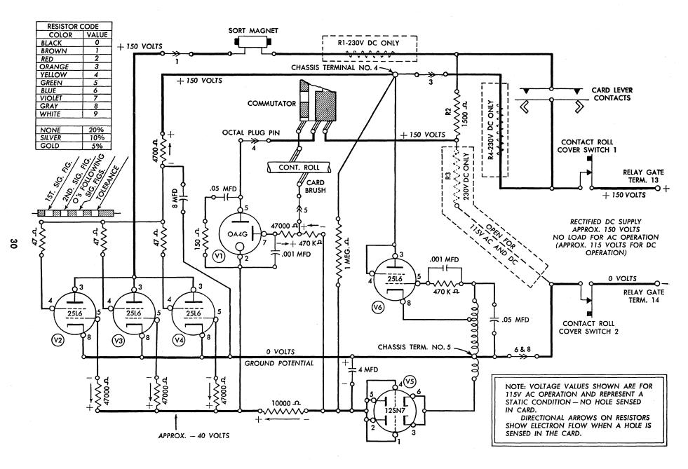
Figure 25. Schematic of Type 82 Sorting Circuits
