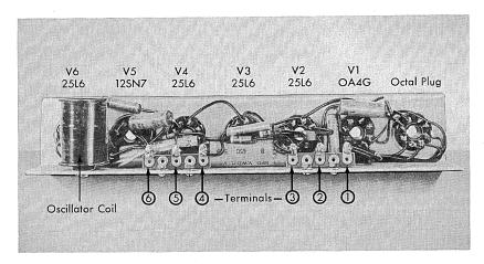
Figure 23. Bottom View of Electronic Chassis
