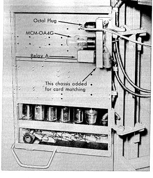
Figure 42. Card Matching Tube Chassis
