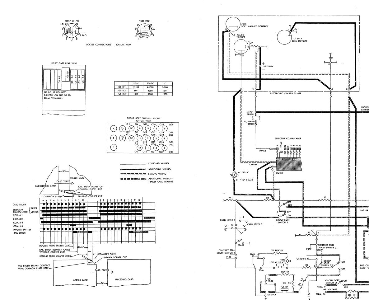
Figure 54. Wiring Diagram - 82 Group Sort Device
