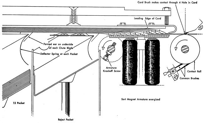
Figure 7. Position of Chute Blades After Sort Magnet Energization
