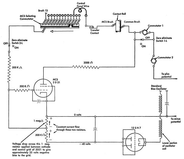
Figure 50. Schematic Wiring of MCS Control Tube
