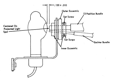
Figure 4-18. Fiber Optic Bundles and Light Source Adjustment
