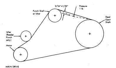
Figure 4-1. Drive Belt Adjustments
