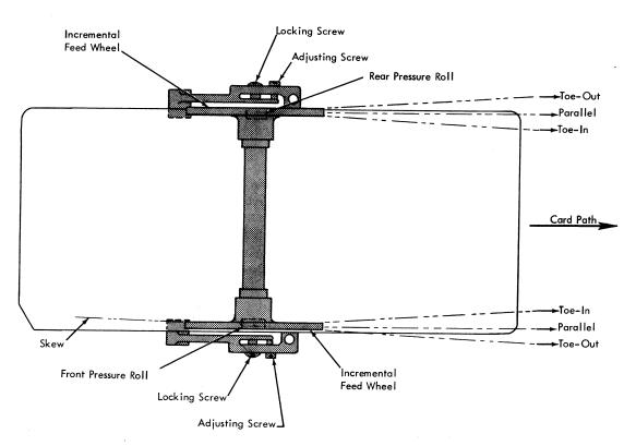
• Figure 4-38. Skew Adjustment (Viewed from Underside of Punch Unit)
