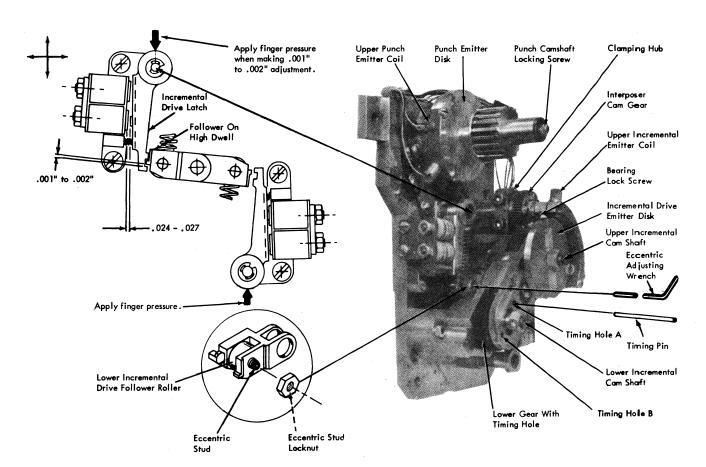
Figure 4-47. Incremental Drive Adjustments
