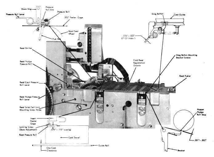
Figure 4-8. Preread and Read Station Adjustments
