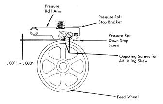
Figure 4-39. Downstop Adjustment
