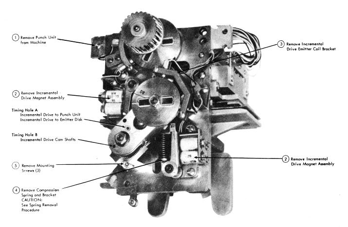
Figure 4-49. Incremental Drive Unit Removal
