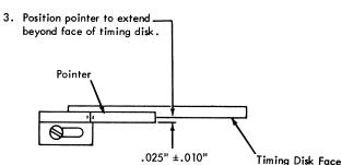
Figure 4-43. Index Pointer Adjustment
