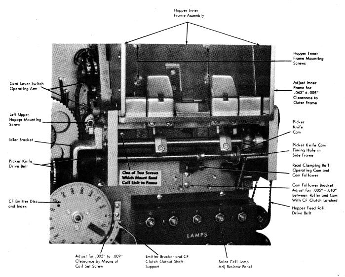
Figure 4-6. Hopper and Pickerknife Camshaft
