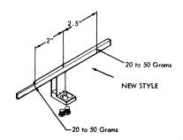
• Figure 4-9. Read Clamping Rail Adjustments
