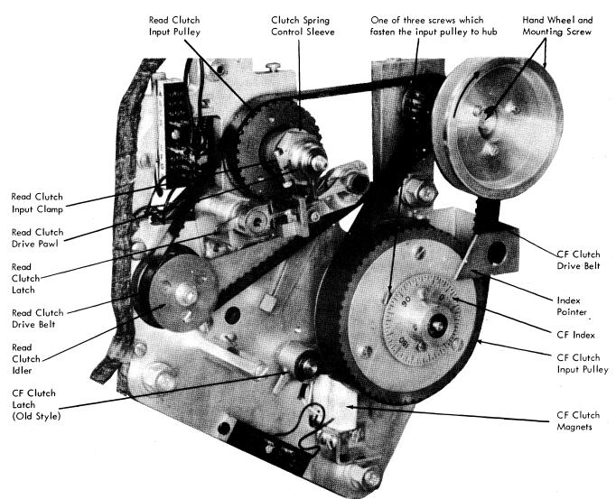
Figure 4-5. Card Feed Clutch and Read Clutch Removals
