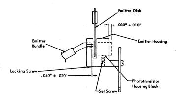
Figure 4-19. Emitter Bundle and Phototransistor Adjustment
