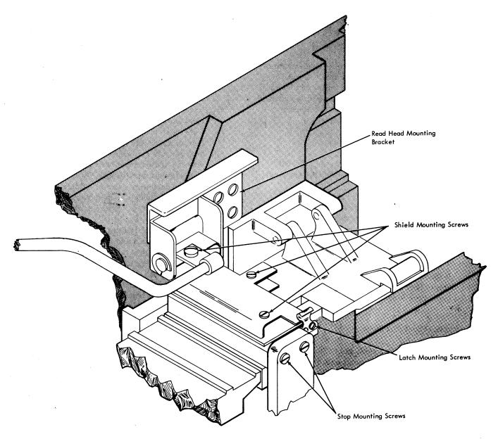
Figure 4-17. Front Mounted Read Head
