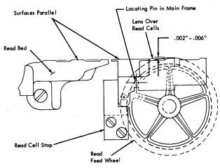
Figure 4-10. Read Cell Unit Adjustment
