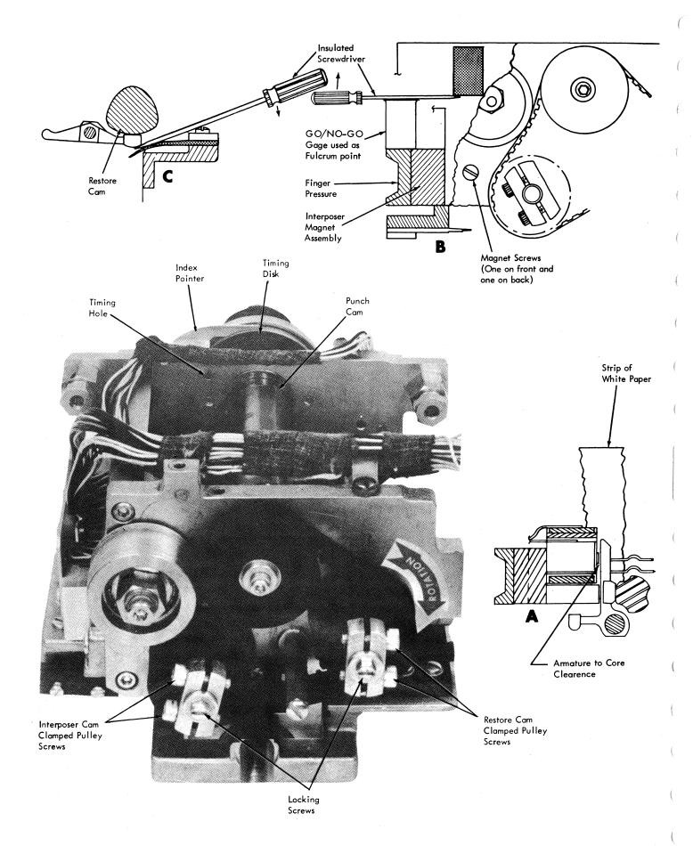
Figure 4-45. Cam Timing
