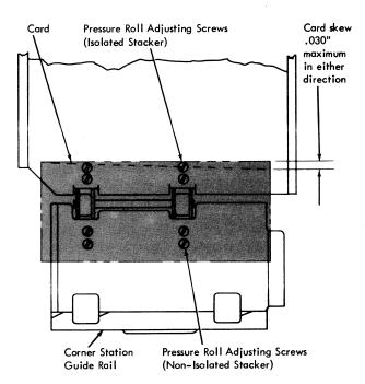
Figure 4-25A. Pressure Roll Adjusting Screw Locations
