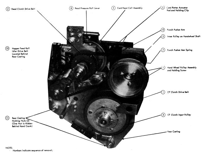
Figure 4-3. Rear Casting Removal
