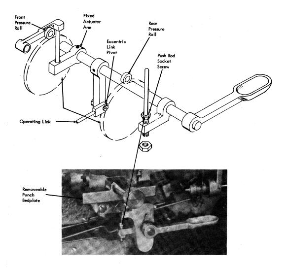
Figure 4-24. Punch Feed Pressure Roll Adjustment
