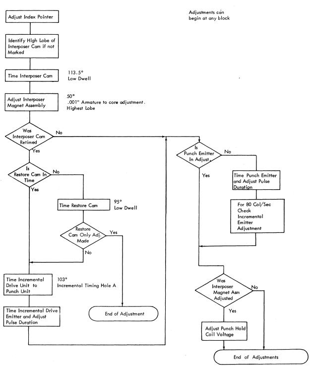
Figure 4-44. Cam and Emitter Adjustment Sequence
