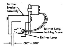
Figure 4-14. Read Emitter Lamp Adjustment
