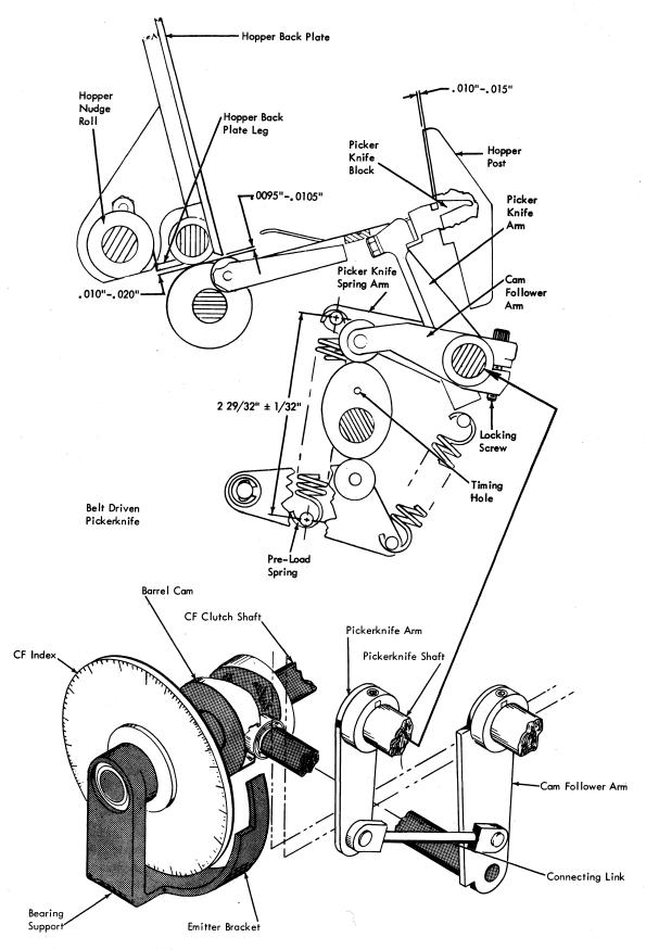
Figure 4-7. Pickerknife and Throat Adjustments
