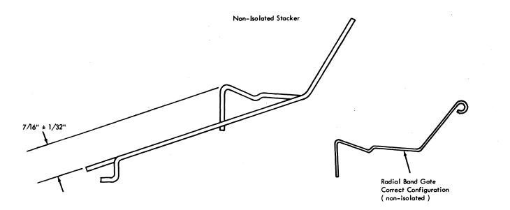
Figure 4-28. Radial Guide Gate Adjustment
