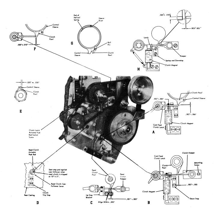
Figure 4-4. Card Feed Clutch and Read Clutch Adjustments
