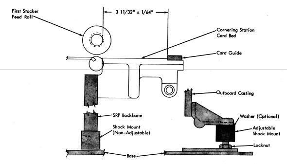
Figure 4-34. Stacker Alignment
