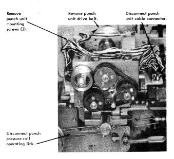
Figure 4-36. Punch Unit Removal
