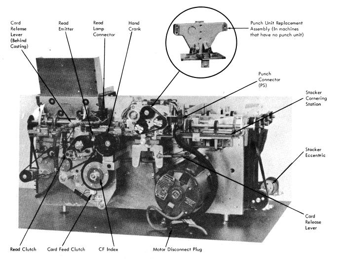
Figure 5-2. Serial Reader Punch, Rear View
