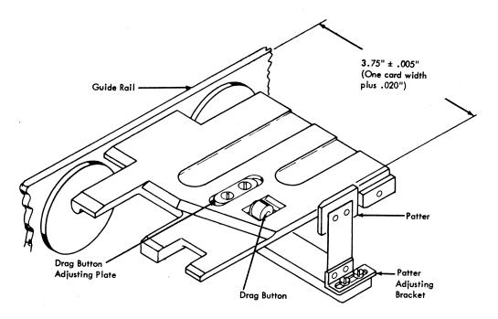
Figure 4-22. Punch Drag Button and Card Patter Adjustment
