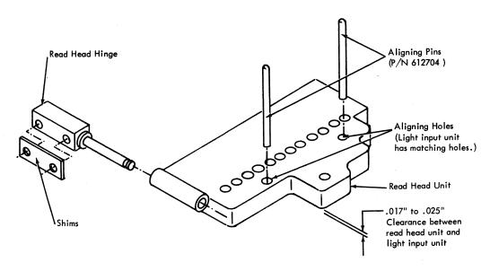
• Figure 4-16. Read Head Unit Adjustment
