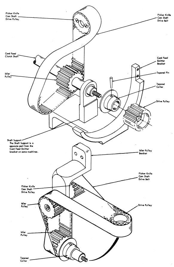
Figure 4-2. Pickerknife Camshaft Drive Belt Installation
