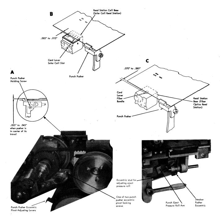
• Figure 4-21. Punch Station Transport Adjustments
