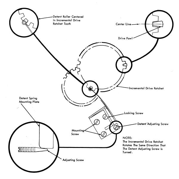
Figure 4-48. Incremental Drive Ratchet Detent Adjustment
