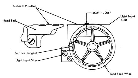
Figure 4-15. Light Input Unit Adjustment
