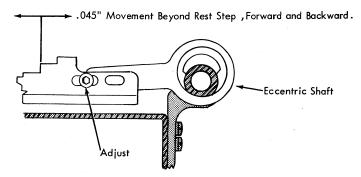
Figure 4-33. Joggler Operating Arm Slide (Isolated)
