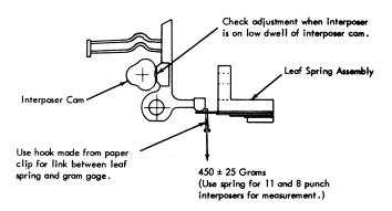
Figure 4-40. Interposer Leaf Spring Assembly Adjustment
