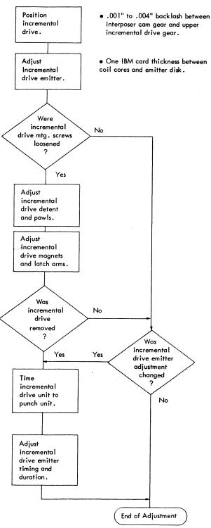
Figure 4-46A. Incremental Drive Unit Adjustment Sequence
