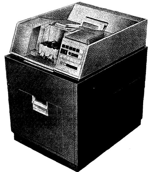
Figure 58. IBM 542 Card Read Punch
