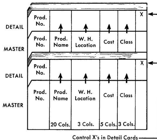
Figure 38. Automatic Coding by Gangpunching
