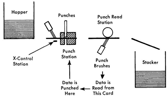
Figure 29. Schematic of Gangpunching
