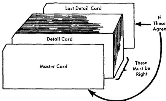
Figure 31. Verification of Gangpunching.
