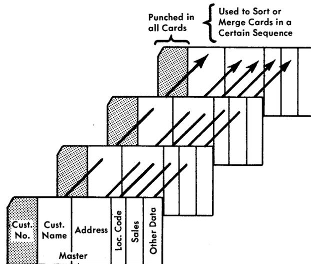
Figure 5. Coding by Gangpunching
