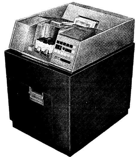
Figure 57. IBM 541 Card Read Punch
