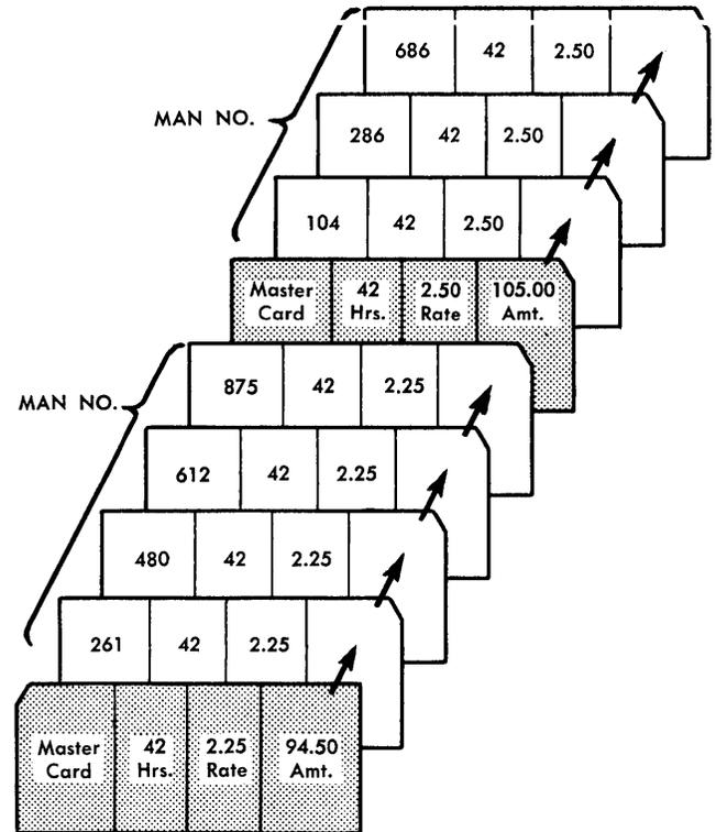
Figure 39. Automatic Extending by Gangpunching
