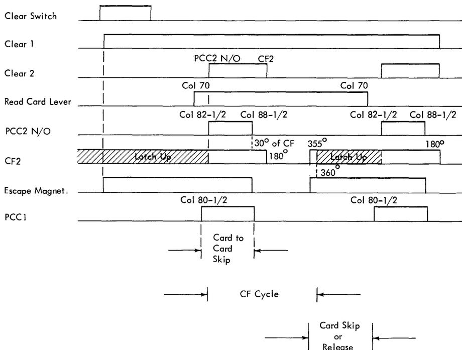
Figure 3-17. Clear Operation (With Card in Detail Station)
