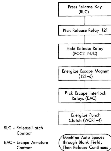
Figure 3-11. Release Key Operation (Blank Field)
