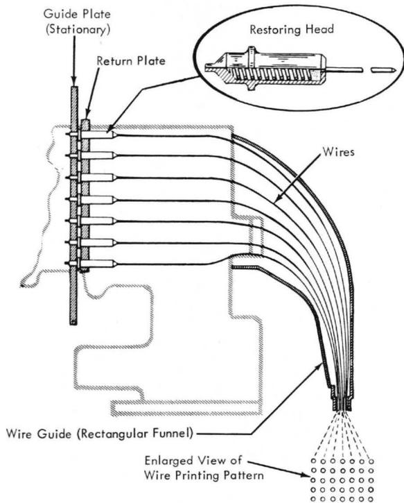
Figure 2-55. Print Wires
