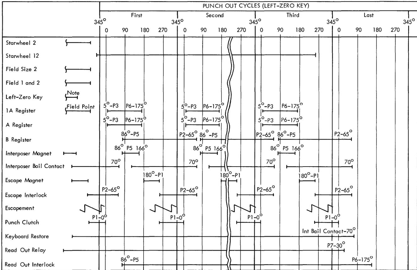
NOTE: The left-zero key picks the read out relay and the first interposer magnet to start the punch out operation.
