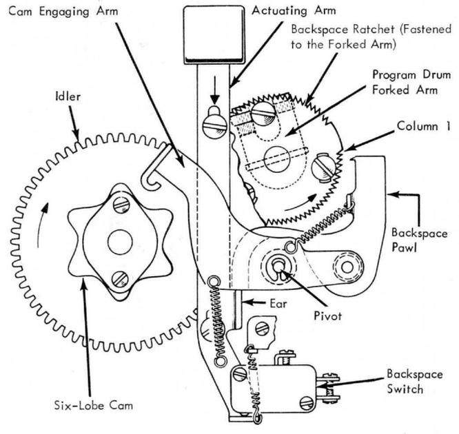
Figure 2-10. Backspace Mechanism
