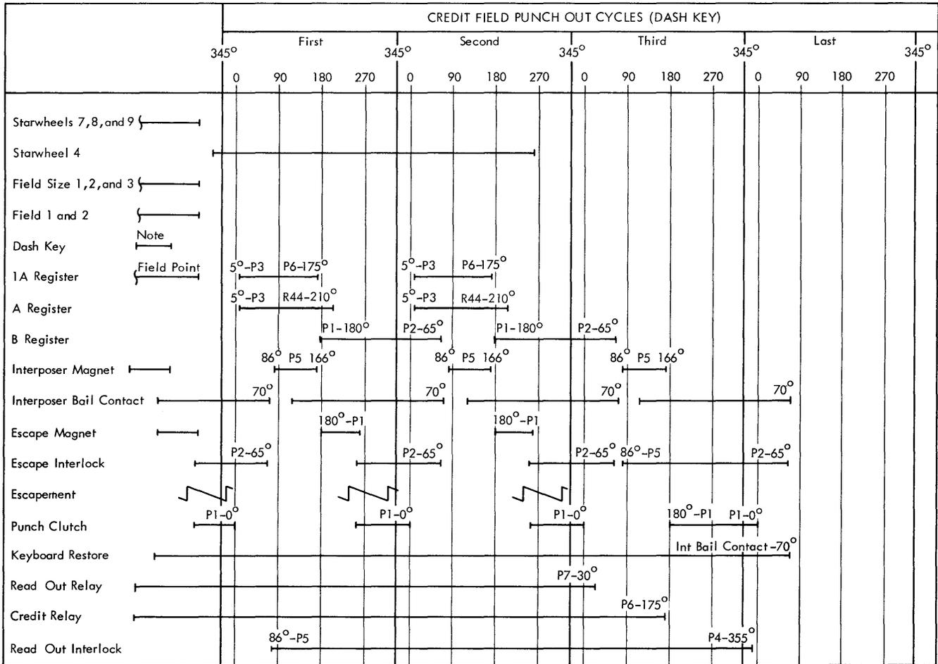
NOTE: The dash key picks the credit relay, the read out relay, and the first interposer magnet to start the punch out operation.
