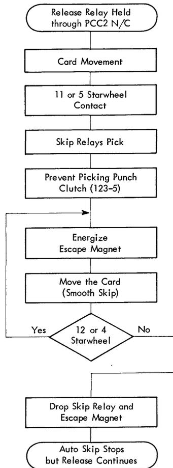
Figure 3-13. Release Key Operation (Auto Skip Field)
