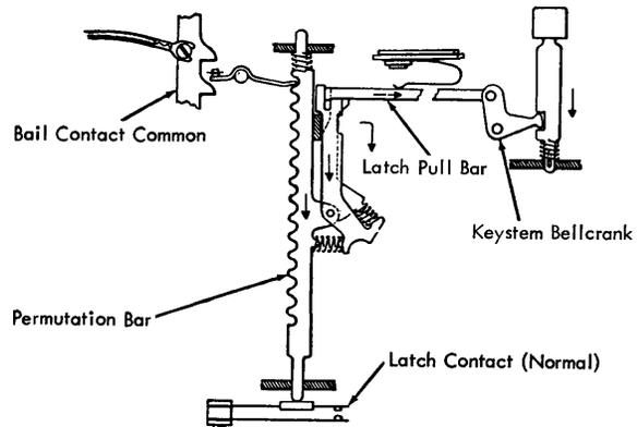
Figure 2-26. Permutation Bar and Keyboard Latch (Normal)
