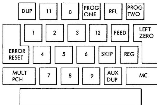
Figure 6-1. Numeric Keyboard and Switch Panel (Model B11)
