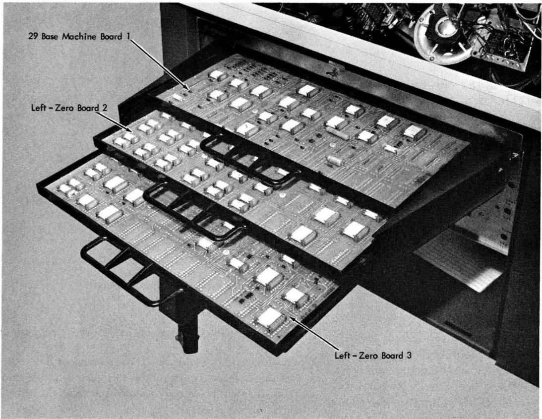
Figure 4-2. Left-Zero Relays ( Reed Relay Machines )
