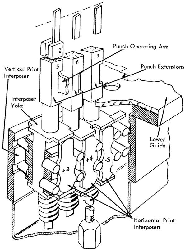
Figure 2-60. Punch Extensions and Print Interposers
