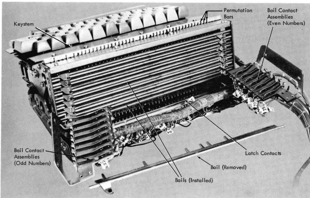
● Figure 2-28. Permutation Unit and Keystem Numbering Chart
