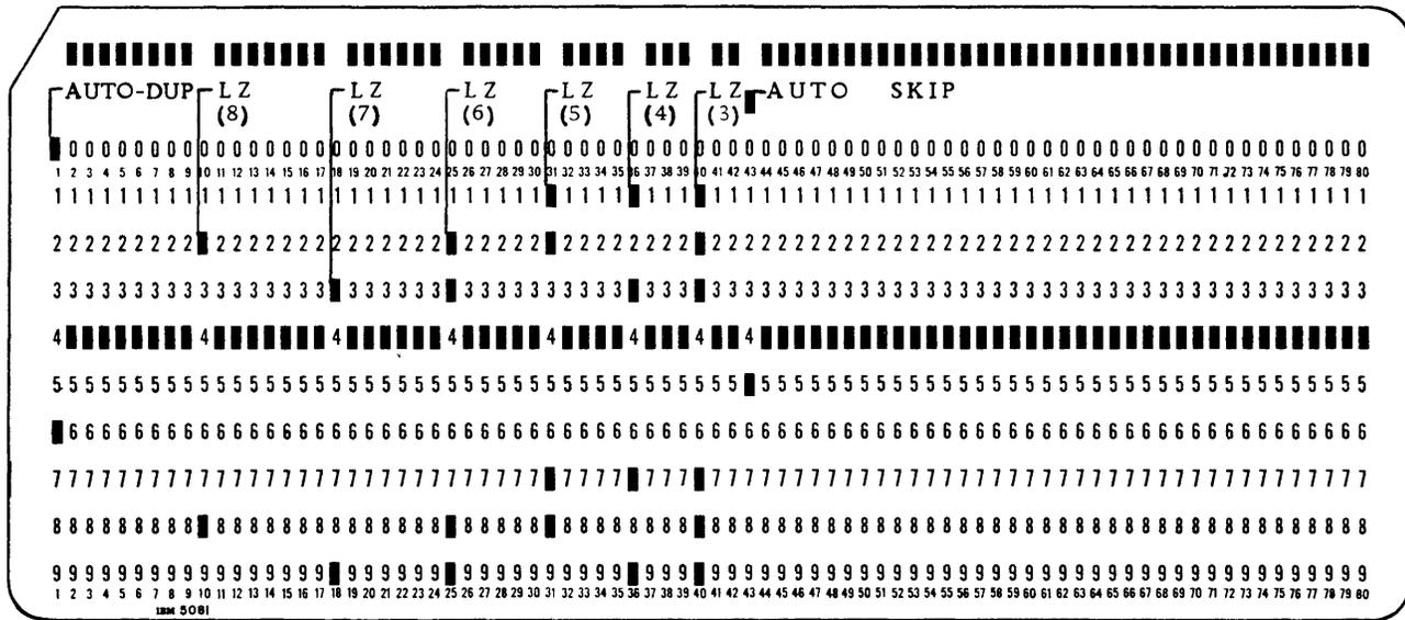
Figure 4-13. Left-Zero Program Card, Wire Contact Relay Machines
