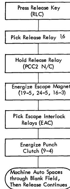
Figure 3-28. Release Key Operation (Blank Field)
