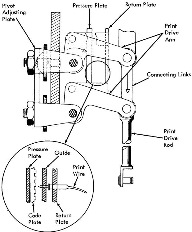
Figure 2-62. Print Drive Rod and Pressure Plate
