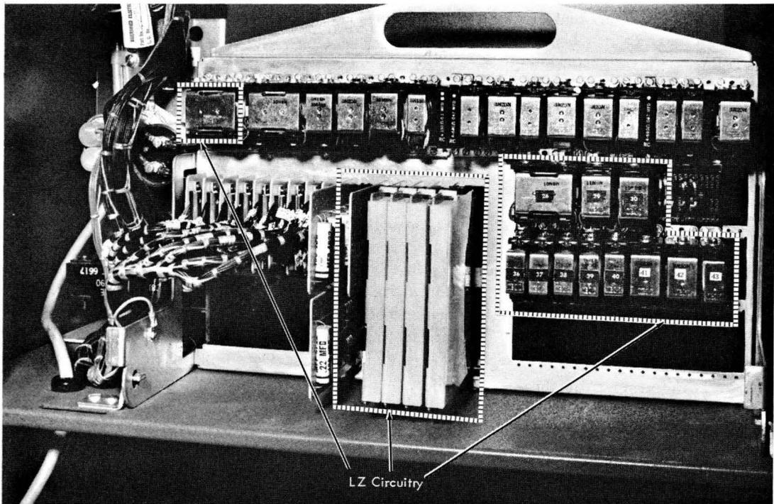
Figure 4-3. Left-Zero Relays ( Wire Contact Relay Machines )
