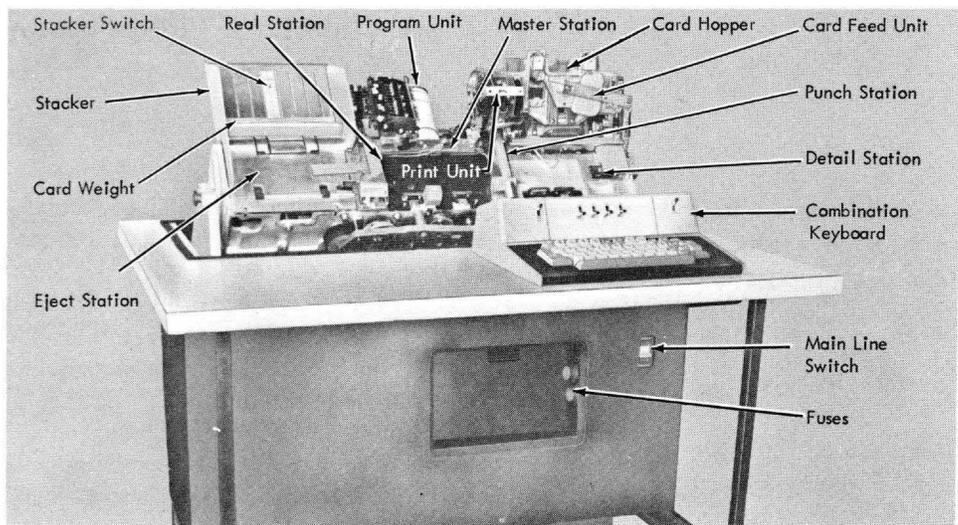
Figure 1-2. IBM 29, Front View (Covers Off)
