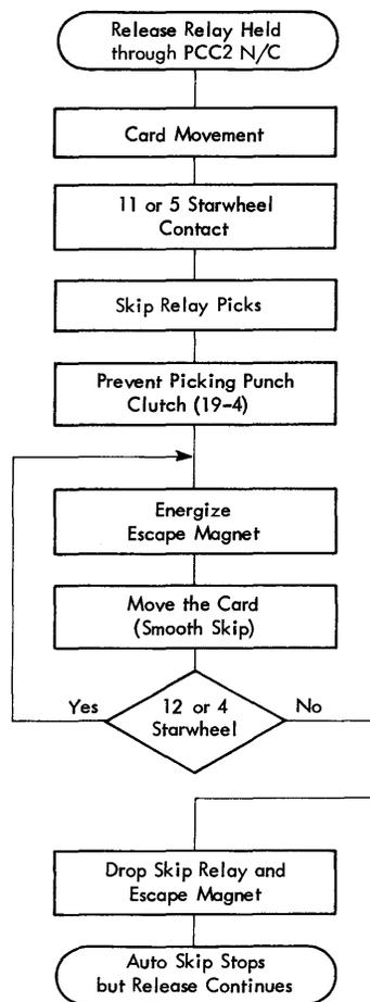
Figure 3-30. Release Key Operation (Auto Skip Field)
