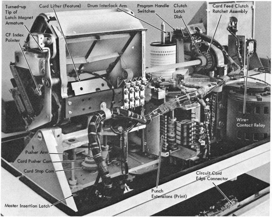
Figure 2-12. Card Feed Unit (Right Rear View)
