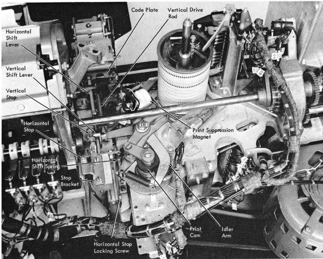
Figure 2-54. Print Unit (Rear View)
