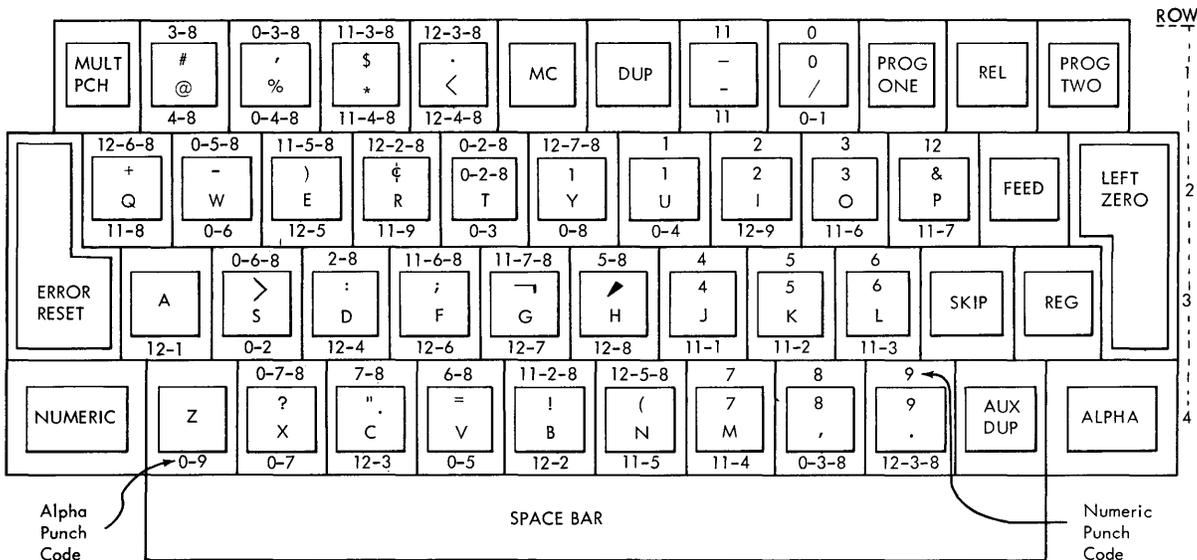
Figure 6-2. Combination Keyboard and Switch Panel (Model B22)
