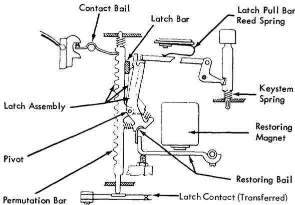
Figure 2-27. Permutation Bar and Keyboard Latch (Tripped)
