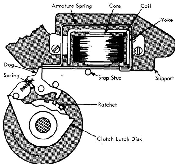
Figure 2-5. Card Feed Magnet and Clutch Assembly
