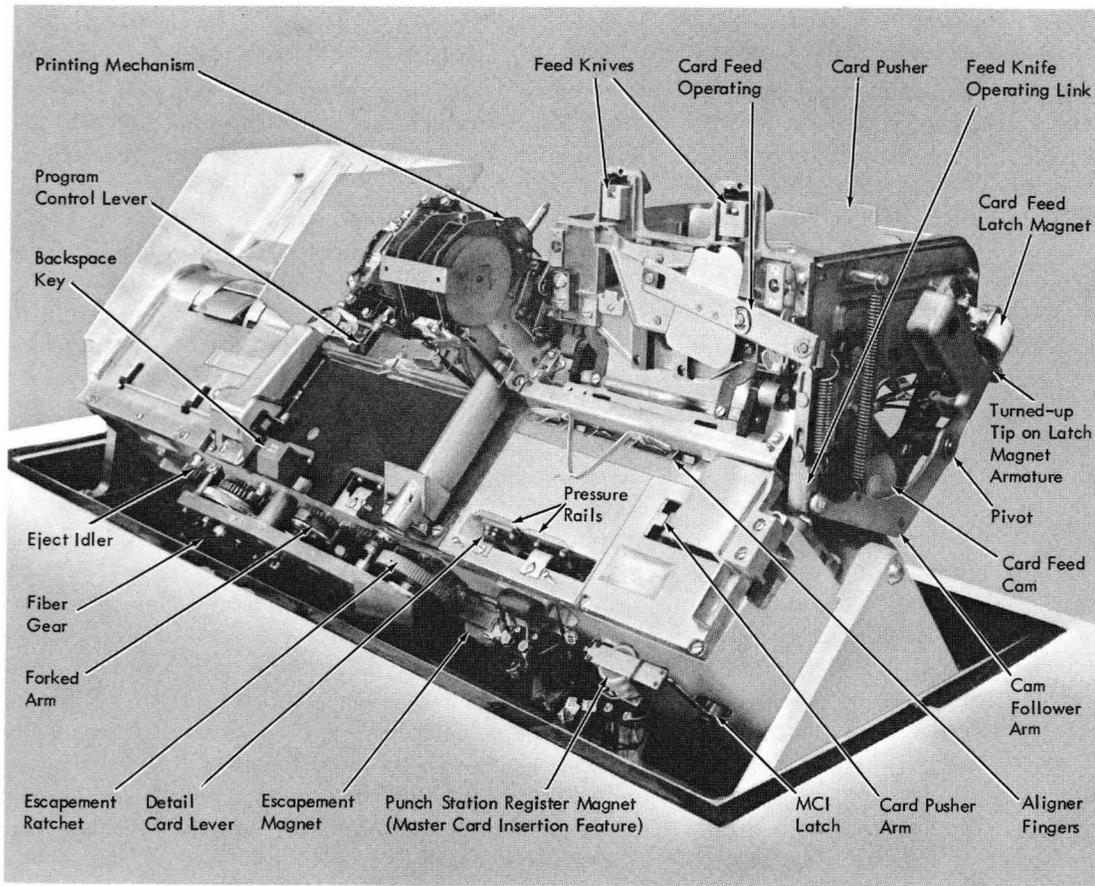
Figure 2-11. Card Feed Unit (Right Front View)
