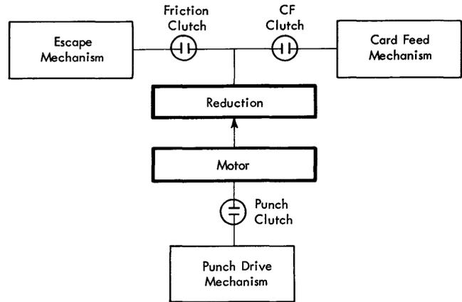
Figure 2-2. Clutch Function
