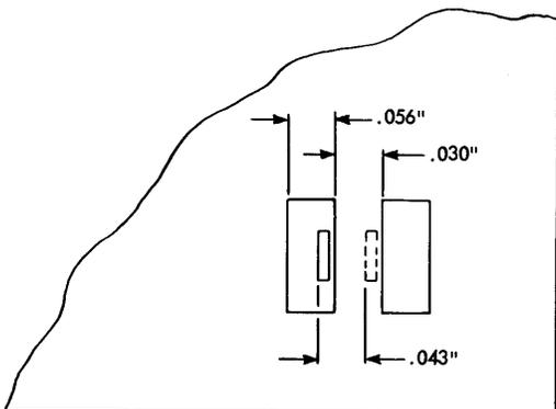
Figure 2-47. Incorrect Sensing Pin Card Registration (Read Station)
