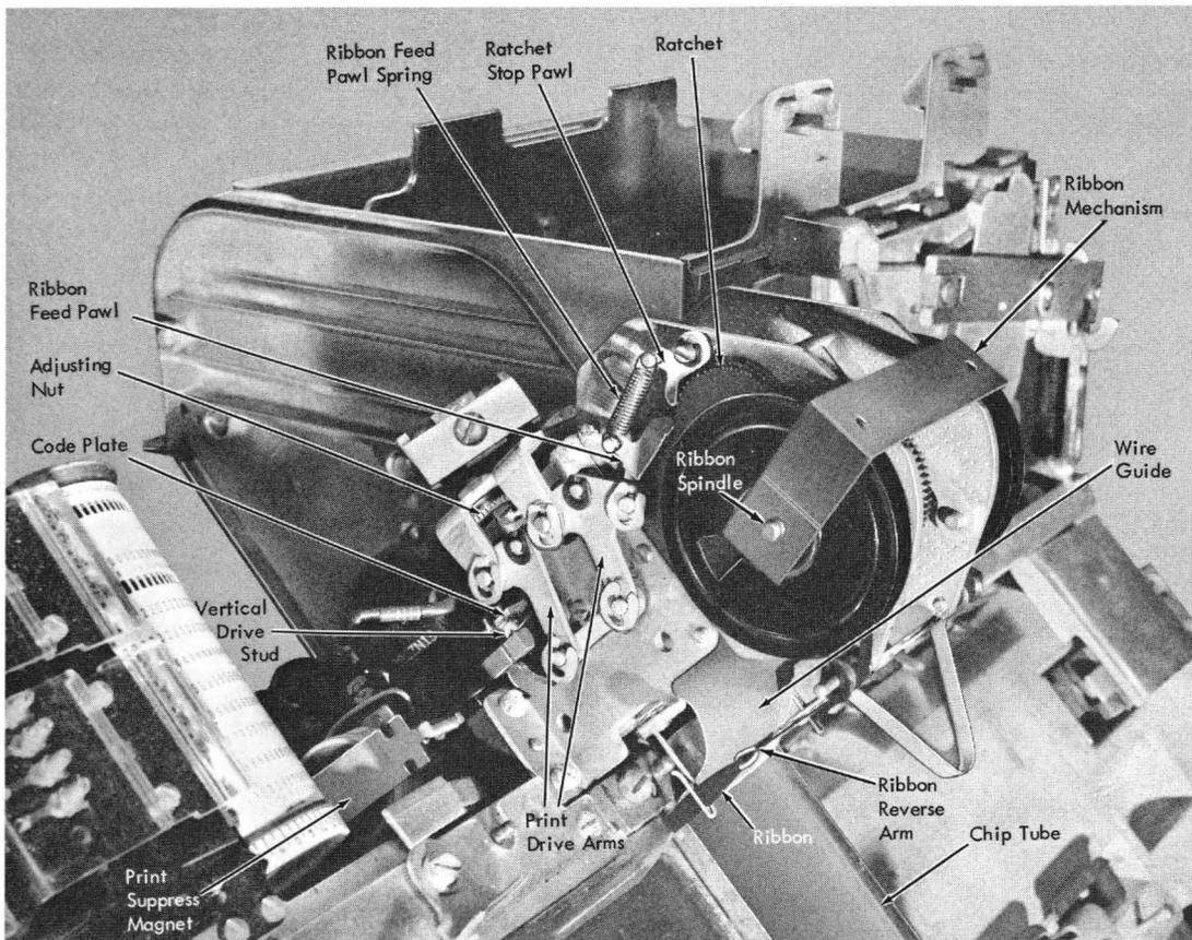
Figure 2-53. Print Unit (Left Front View)
