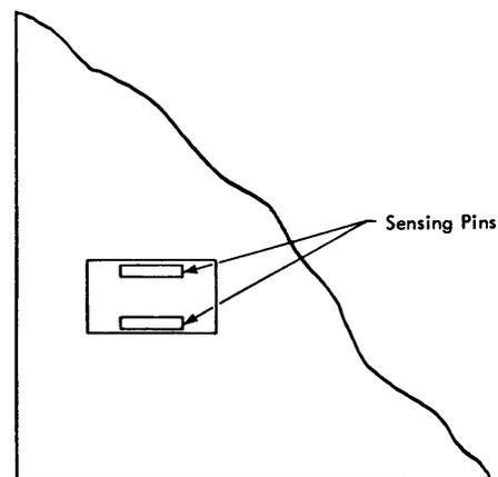
Figure 2-46. Correct Sensing Pin Card Registration (Read Station)
