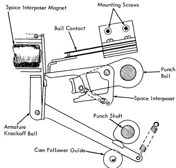
Figure 2-37. Space Interposer and Armature Knockoff Bail
