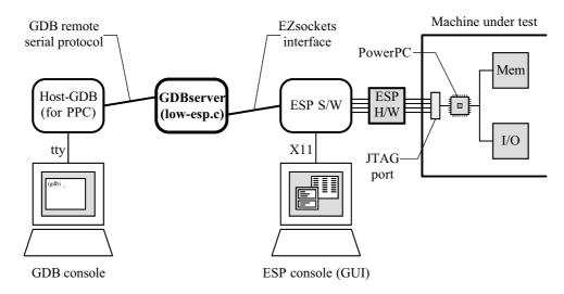
Figure 1: Debugging environment using the GDBserver for ESP
