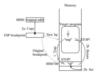
Figure 4: Stopping the target program by means of a trap
