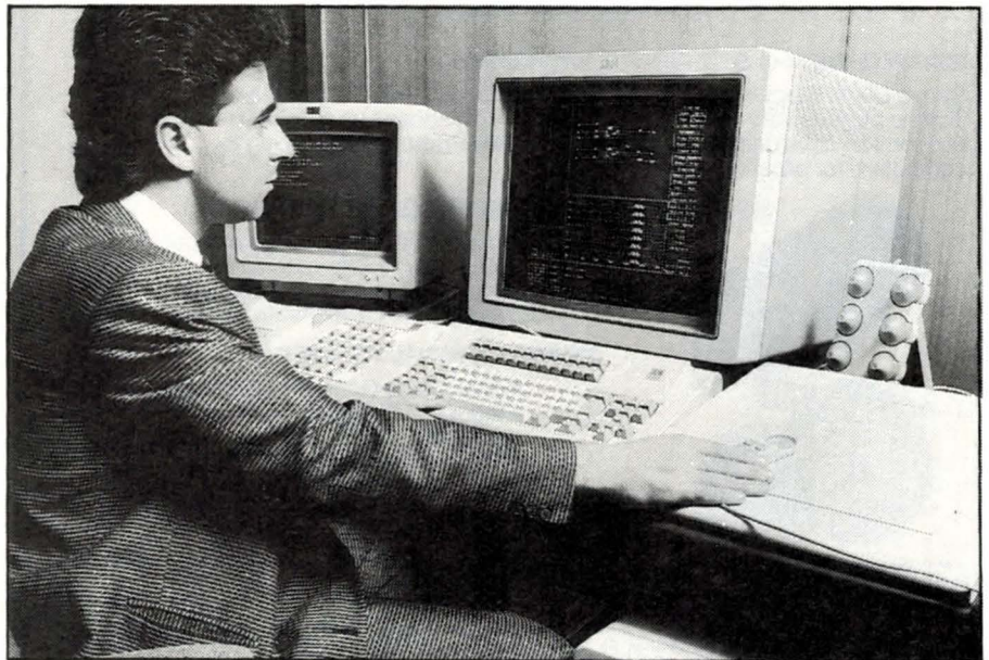
IBM systems engineer Dino Calapai uses a mouse to help him review the schematic of a printed circuit board he is designing on CIEDS/CBDS.
