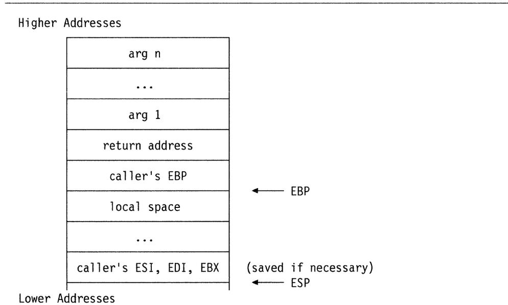
Figure 6-1. Typical Stack Frame
