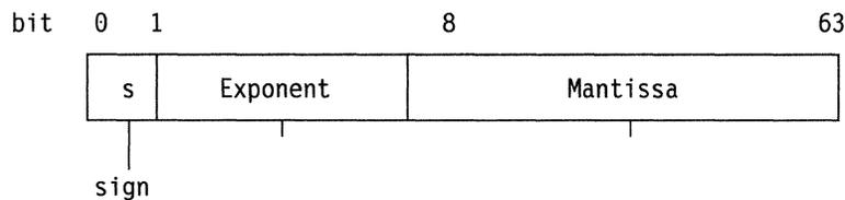
The three fields of a **double**-precision floating-point number are:
