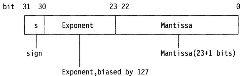
The three fields of a single-precision floating-point number are:
