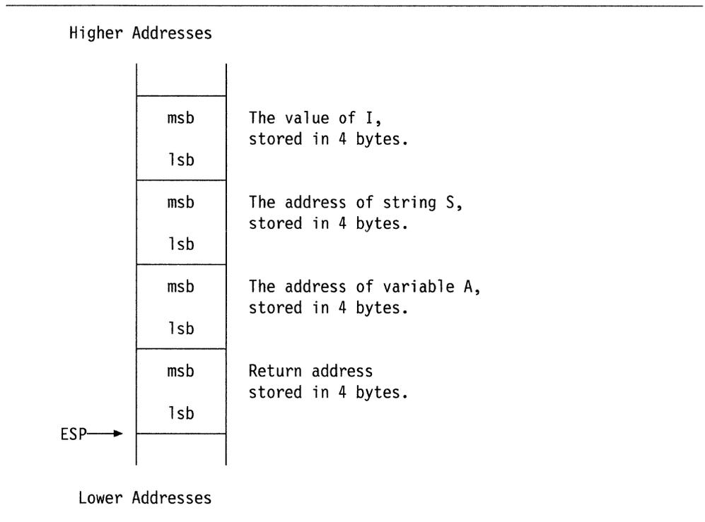
Figure 6-3. Stack After Call in Example C
