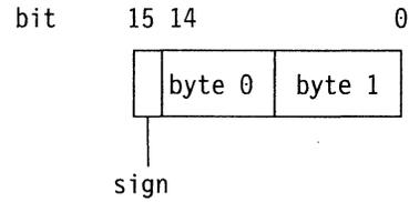
**Note:** An external short data type is fullword aligned.
