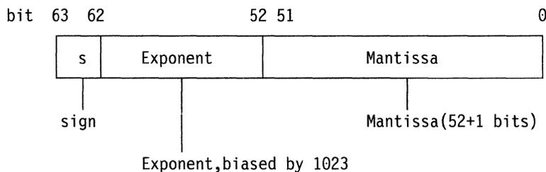
The three fields of a double-precision floating-point number are:
