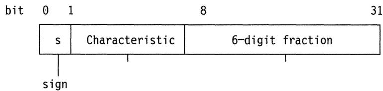
The three fields of a single-precision floating-point number are:
