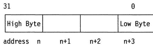
The RT PC microprocessor requires alignment of data. For this reason, the AIX RT PC C Compiler aligns 2-byte entities on even addresses and 4-byte entities on addresses which are multiples of 4; 8-byte entities are aligned on addresses which are multiples of 4.
