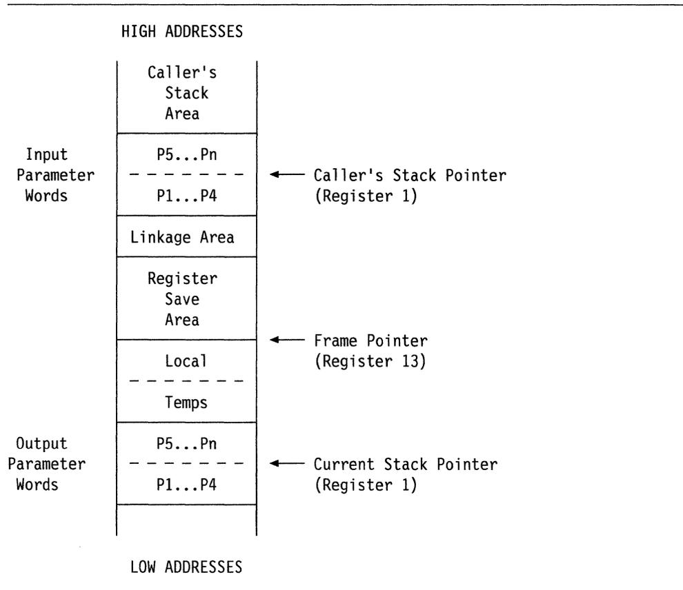
Figure 7-1. Contents of a Stack Frame
