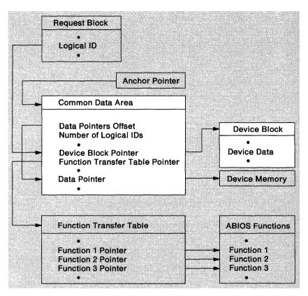
Figure 2-5. Flow of Device Block
