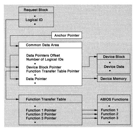
Figure 2-1. Flow of Common Data Area
