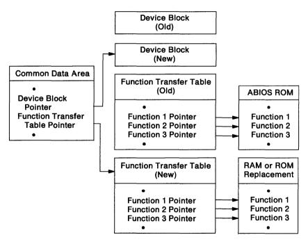
Figure 5-8. Replacing ABIOS
