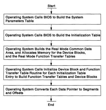
Figure 3-1. Flow of Real Mode Common Data Area Initialization
