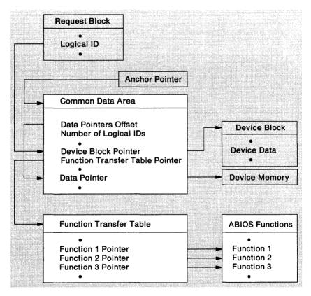
Figure 2-3. Flow of Function Transfer Table
