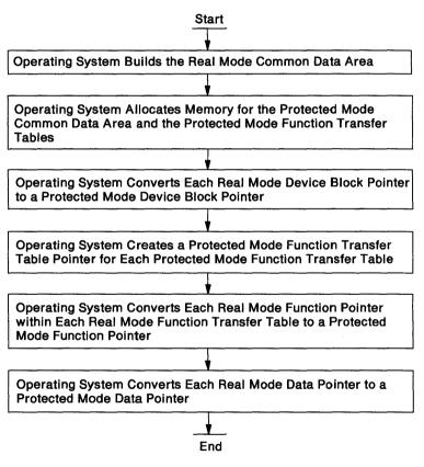
Figure 3-9. Flow of Protected Mode Common Data Area Initialization
