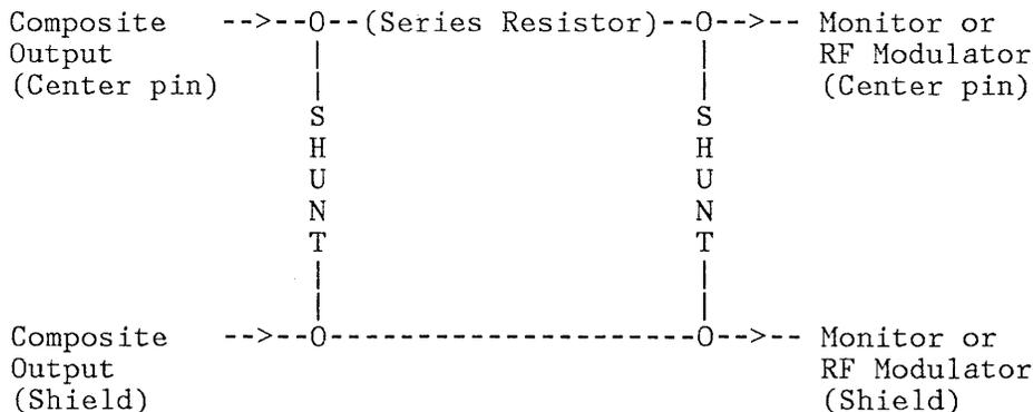
This circuit presents about a 75 Ohm impedance and should be used with 75 Ohm coax (such as RG 59 or TV coax) to minimized reflections (ghosting) that can reduce the sharpness of the picture. You must determine what level of attenuation you need, and that will be dependent on the input level needed by the device that you are connecting. A good guess would be in the 3 dB area for about a 1.0 volt p/p signal.
