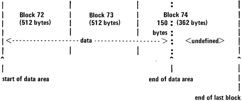
**Figure 3-7. State of Blocks on Disk After a Write**
