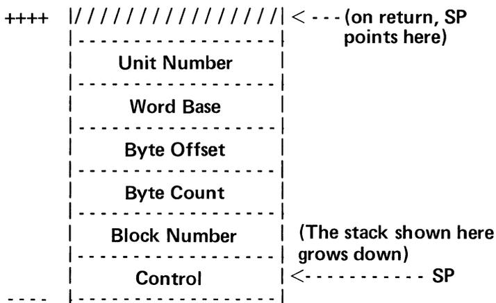
**Figure 3-5. Stack State on Entering UNITREAD or UNITWRITE**
