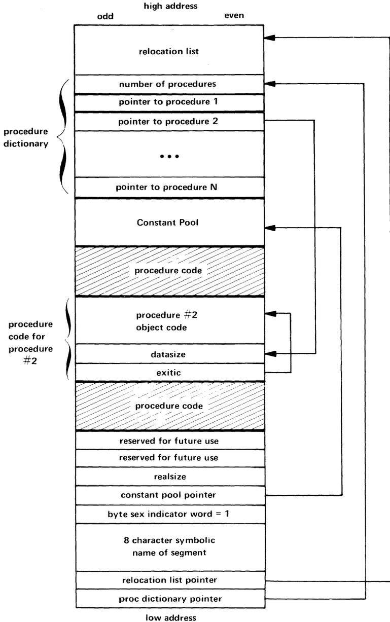
Figure 2-1. Executable Code Segment Format
