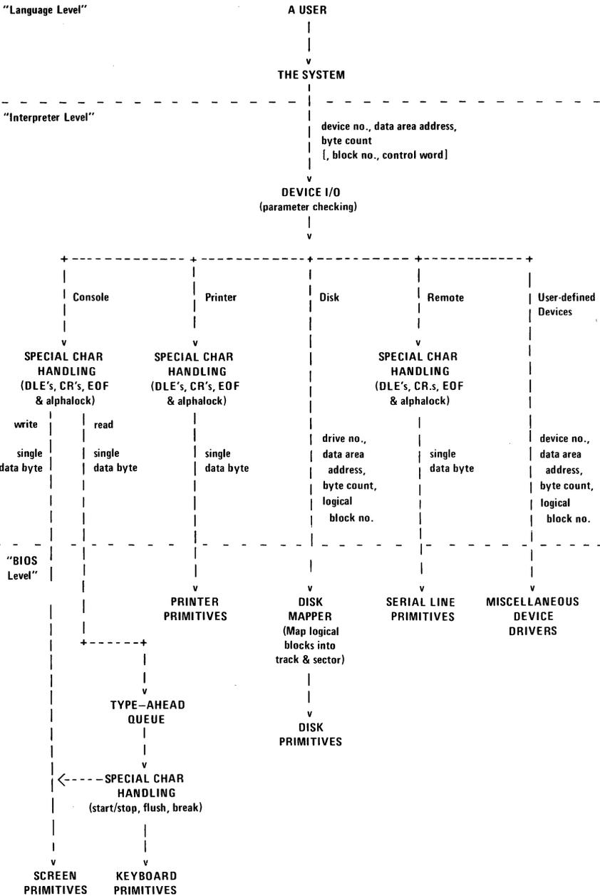
Figure 3-1. I/O Subsystem Hierarchy
