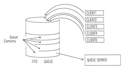
Figure 5.1 Diagram of a queue.
