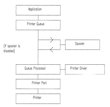
Figure 28.1 A view of the print subsystem.
