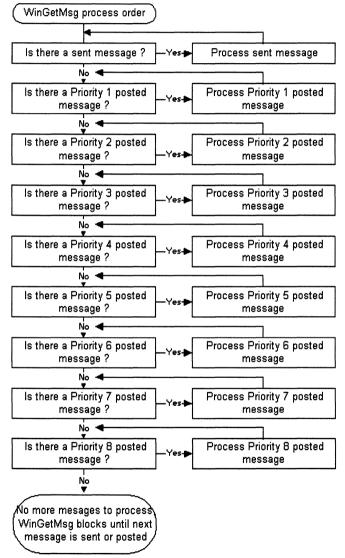
Figure 11.2 WinGetMsg message processing order
