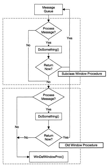
Figure 27.2 Subclassed window procedure calling chain.
