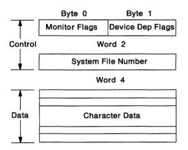
The printer device driver passes the code page information to the monitors in data packets. The code page information in the data packets is preceded by control information.
