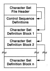
The Font File Header defines the printer which the font file supports and has pointers to the Control Sequence Definitions section of the file and to the first Font Definition Block. The Font Definition Blocks are a linked list throughout the rest of the file. Each of these sections of the font file are described in more detail below:
