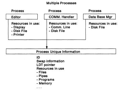
For a solution to an application where multiple asynchronous execution threads are needed, the following diagram demonstrates how the various threads might operate, each using different devices to accomplish a portion of the overall solution.
