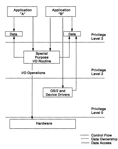
For a module to be loaded at protection level 2, the CONFIG.SYS IOPL=yes command must indicate this is to be allowed. Protection level 2 modules cannot use dynamic link, and cannot make OS/2 function calls.
