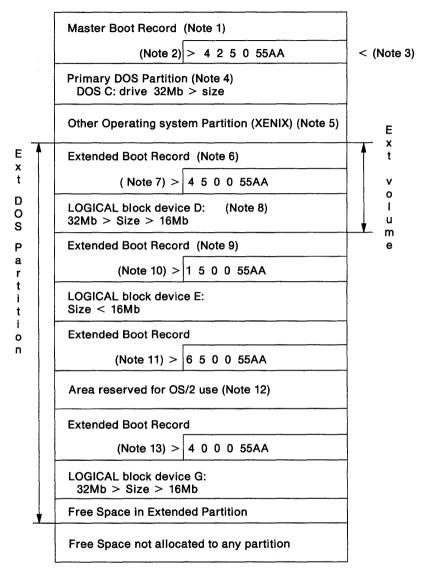
Note 1 Master start-up (boot) record code, starting at Trk 000, Hd 00, Sec 01 of disk 80H or 81H.
