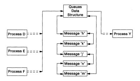
As with pipes, the sending processes can send data independently of one another. However, unique to queues, outstanding elements can be ordered by priority or by arrival order, first-in first-out (FIFO) or last-in first-out (LIFO). Also, process Y can examine each element in the queue and remove them whenever, and in any order, desired.
