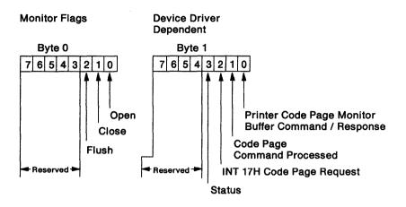
When the Status bit is set to 1 (byte 1, bit 3), this indicates that the monitor buffer is a status packet from the printer device driver. In this case, the next six bytes are:
