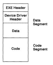
The data segment must be the first segment after the .EXE file header. This allows the device header to be located immediately
