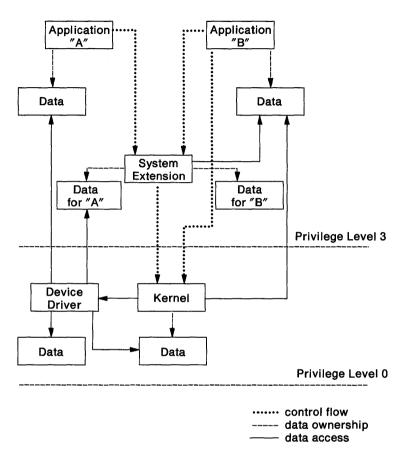
For processing of the request under a separate process, interprocess communications techniques may be implemented using semaphores, queues, signals, or shared memory.
