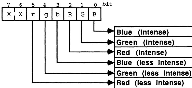
*EGA palette registers when connected to EGA or multisync monitor*
