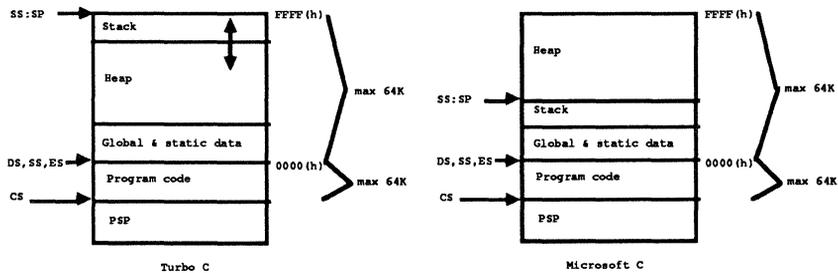
*Structure of a small model program (Turbo C/Microsoft C)*
