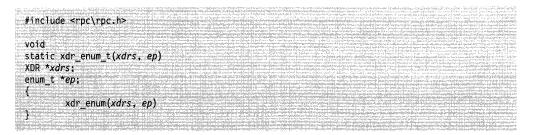
The xdr\_enum\_t procedure is used as the *inproc* and *outproc* in both the client and server RPCs.
