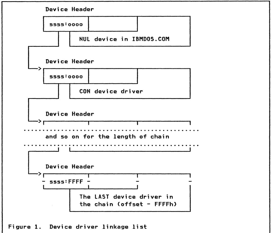
Figure 1. Device driver linkage list
