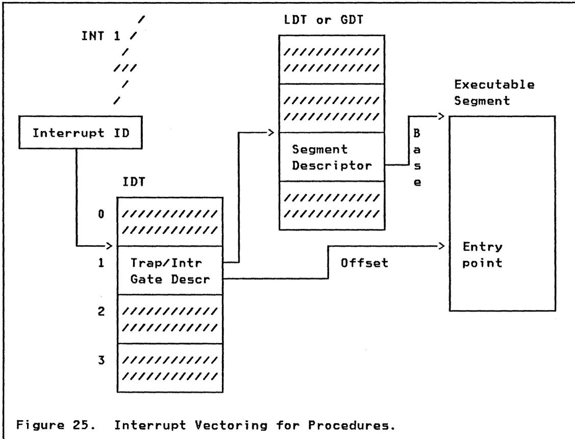
Another way of implementing interrupt handling routines is to have a task gate descriptor in the IDT. Refer to Figure 26 on page 163.
